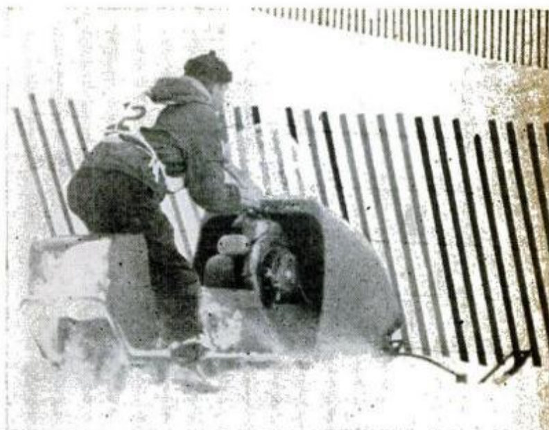
KNEELING ON THE SEAT enables the driver to shift his weight quickly from side to side for turns and also stand up to absorb the shocks with his legs
