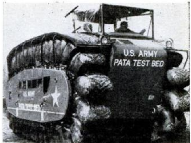
Pneumatic-tired track supports and propels a new Army amphibious cargo carrier over all terrains, normal hard surfaces, swamps and marshland, tundras and open water. Each inflated cell has cleats for better traction over soft surfaces.
