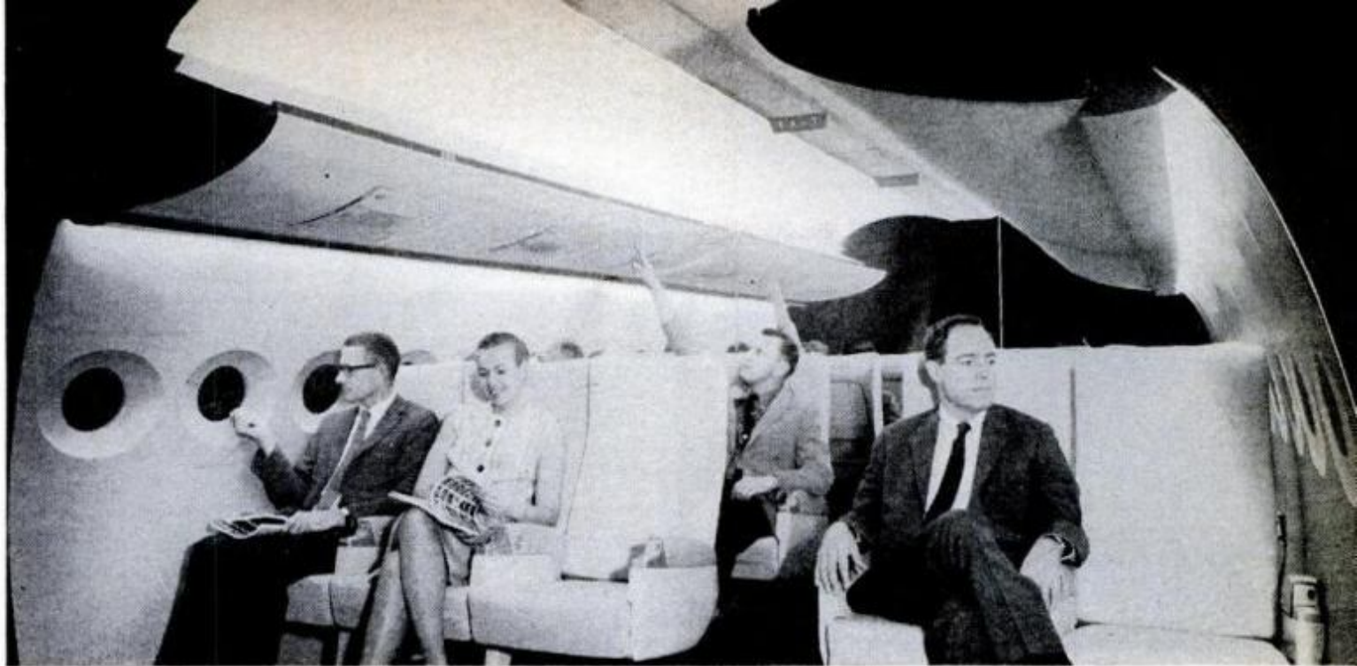
CABIN INTERIOR emphasizes tunnel-like construction. SSTs will be longer but narrower than current subsonic jets. Seats, five across, will be smaller and lighter but provide more space for each individual passenger
