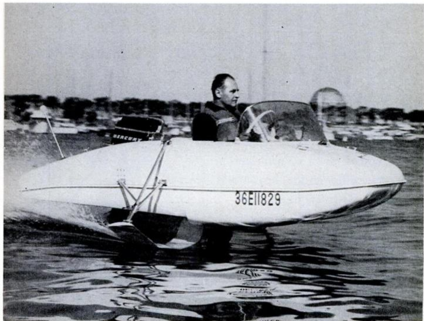
FLYING above the surface on its foils, the pod picks up speed rapidly. Running flat out, the boat rides on only 15 square inches of the foil surface
