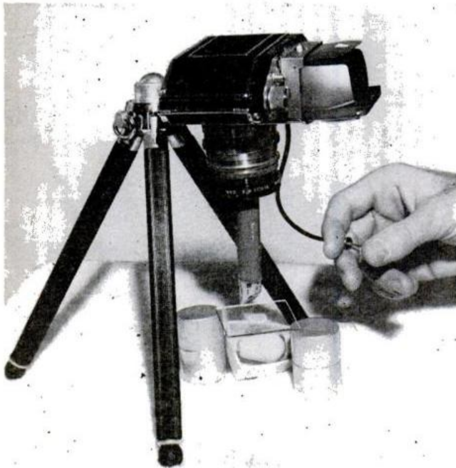
HERE IS HOW cardboard disc, sandwiched between adapter and retaining rings, is used to attach microscope to camera
