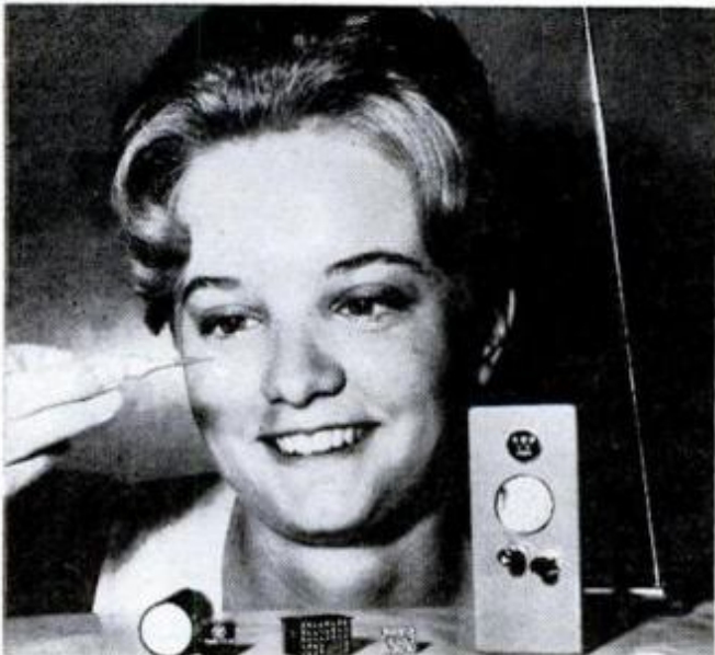
Shirt-pocket TV. A mere 3½ inches high, 4½ inches long and less than 2 inches wide with a 1-inch diameter picture tube, this Westinghouse TV is a true pocket portable. It works off batteries or can be plugged into a wall outlet. Built with microcircuits, the set dramatically shows how small, small can be. This TV is the only one of its kind and will not be sold commercially.
