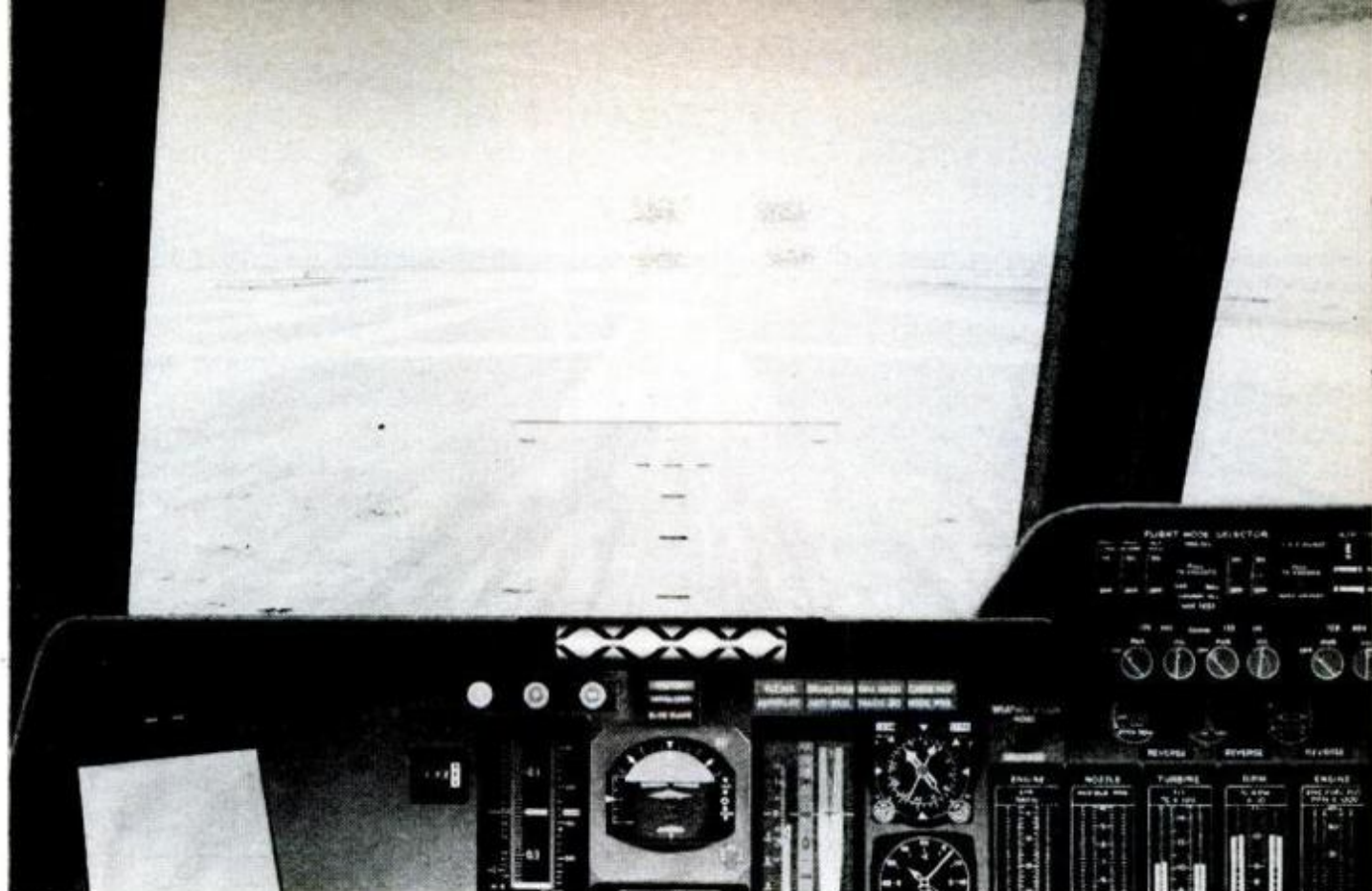
PILOT'S EYE VIEW from cockpit of supersonic transport. When nose is up during cruising, his vision is partially obscured (left). When nose is down for takeoffs and landings (above), he has normal vision. Instrument panel will also dispense with round dials, displaying information on moving tapes
