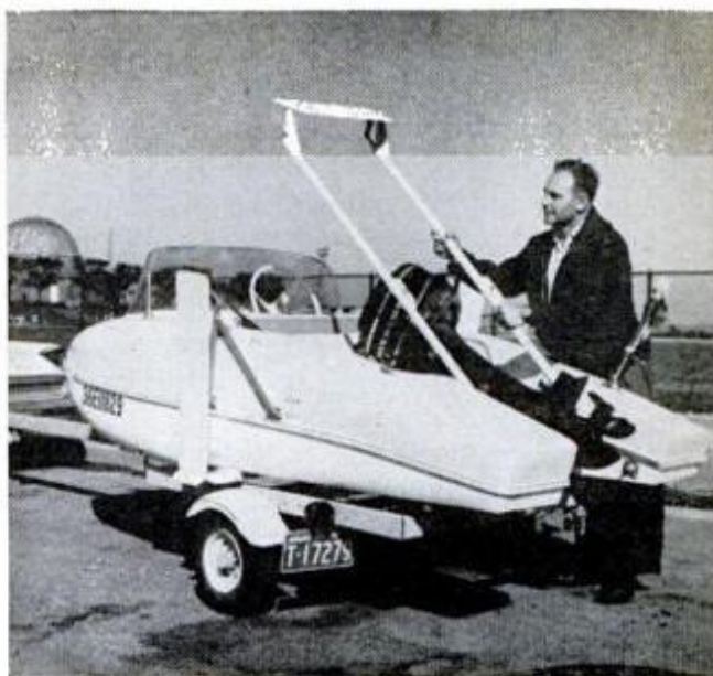
EVERYTHING FOLDS up snug to the hull so that the tiny flyer can be transported on a normal boat trailer. The stabilizer swings over into the cockpit
