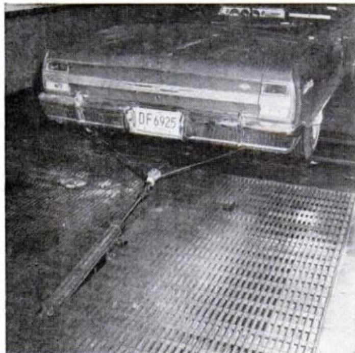
RETAINER keeps wheels from hopping on dynamometer rollers, which would give an inaccurate reading, and prevents the car from running off the machine
