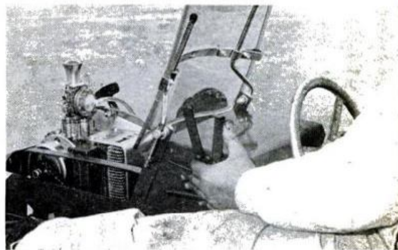
DEAD MAN THROTTLE is a safety device. It must be held forward to activate the engine; when it is released it automatically cuts off the power
