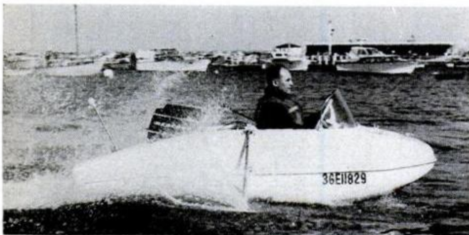
CLIMBING to a planing attitude as power is applied, the foil struts kick up a fine spray. This disappears once the hull breaks free of the water
