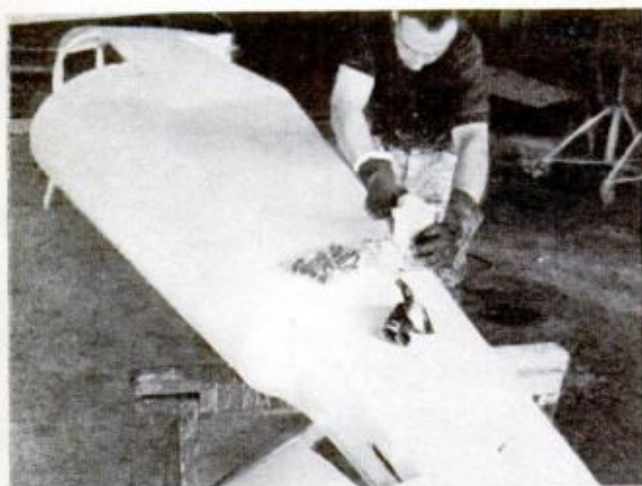
METICULOUS WORKMANSHIP , exemplified by wet sanding of plywood fuselage, is boasted by RF-3 makers. Model is near-handmade version of original
