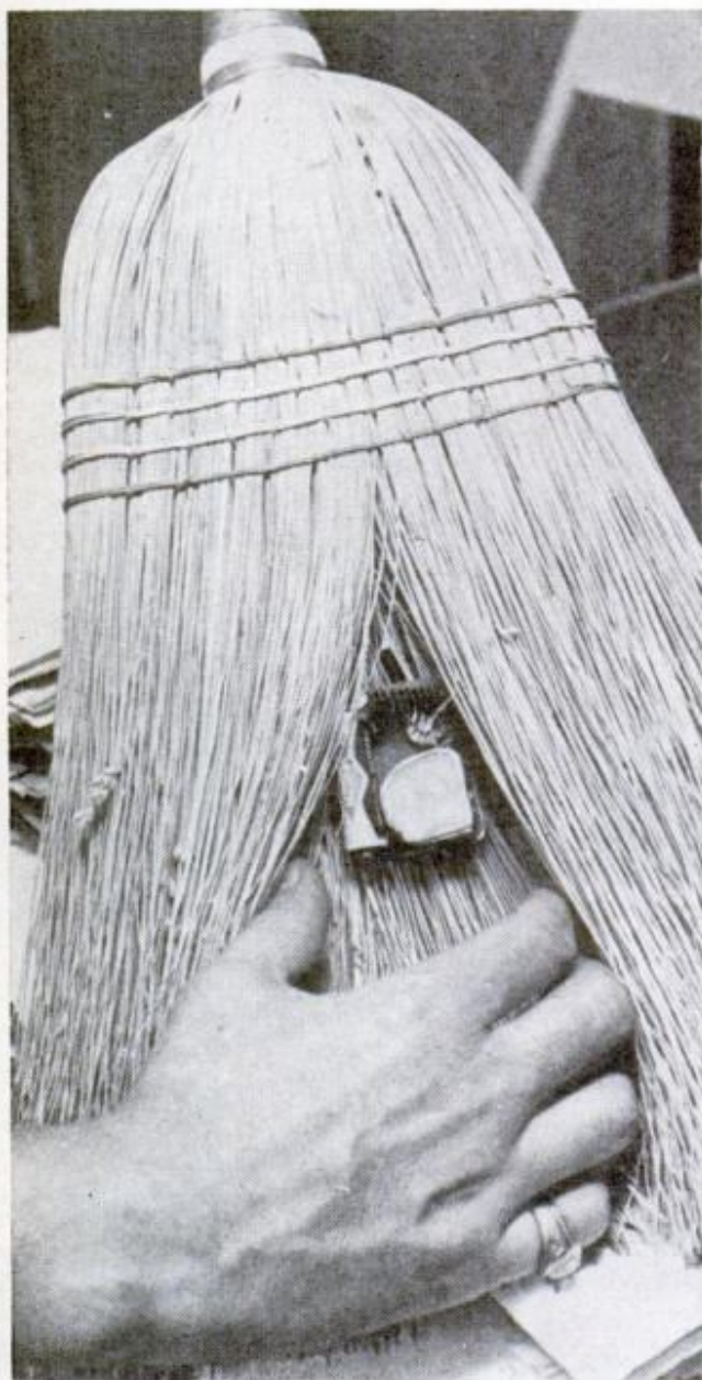
TRANSMITTER IN A BROOM is only one example of how a listening ear can be concealed in your office. Any piece of office furniture would work as well
