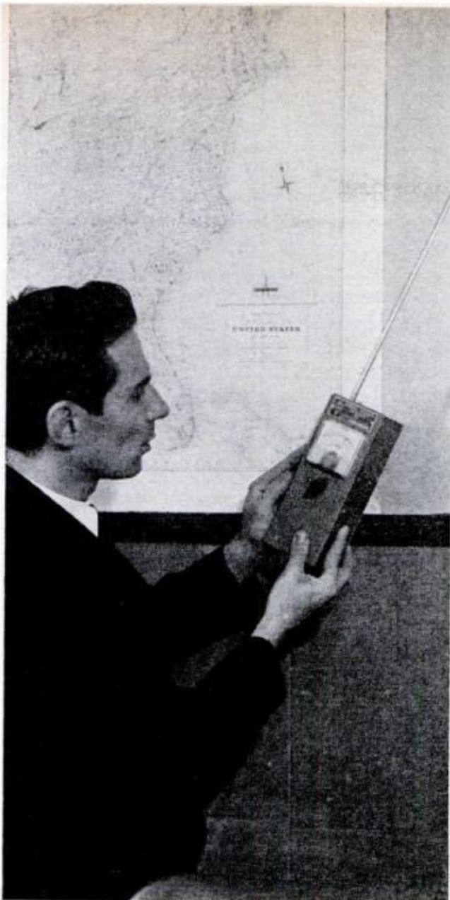
SNIFFER finds transmitters hidden in conference room. Every inch of wall, floor and ceiling must be checked methodically or low-power bug might be skipped
