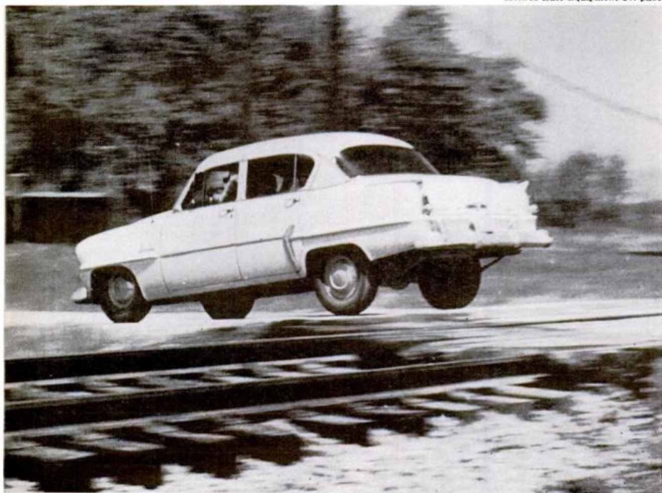
A GOOD EXAMPLE of bad shock absorbers is the bounced-up rear end of this car as it crosses a track
