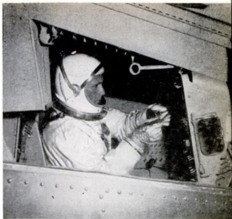
CONTROLS ON FULL-SCALE MODEL allow astronaut to move spacecraft vertically and sideways in practicing simulated docking maneuver in darkened hangar
