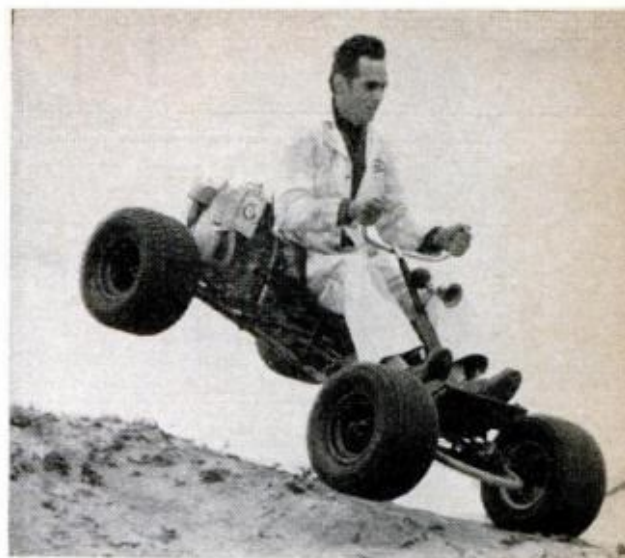
RUGGED STEEL FRAME is welded at all joints so Terra-Tiger will withstand the jolts of high-speed game of hare and hounds in cross-country terrain
