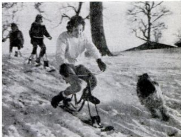
Snow-going bike. Mount an old bicycle frame on a pair of plywood skis and you've got a Jack Jumper, a midwest version of an old New England sport. The skis are two feet long and six inches wide, and when you sail down a snow-covered slope you steer with the front ski and balance with your feet.
