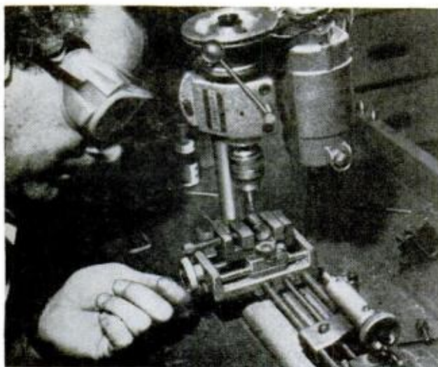
BOON TO MODELMAKERS is the Unimat, a multi-purpose power tool designed specifically for machining and drilling miniature parts with minute tolerances
