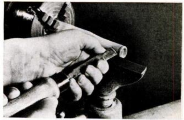
TO TURN HALOS, hollow out end of 3/4-in. round, leaving 1/8-in. thick wall, then cut off 1/8-in. ring
