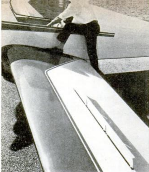
SPEED BRAKES on upper panel are demonstrated by Fournier. Brakes serve to slow plane down and increase its rate of descent for picking landing spot
