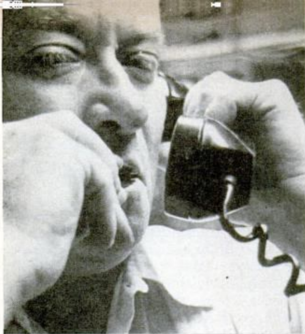
TOOT YOUR HARMONICA and it can turn on remote microphone that has been connected to bugged telephone. Emanuel Mittleman developed this system
