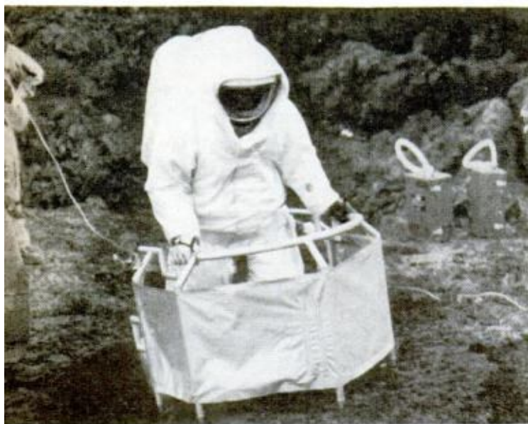
USING LUNA-WALKER stabilizing device, spaceman trudges up slope near McKenzie Pass, Ore., closely attended by members of medical and technical teams
