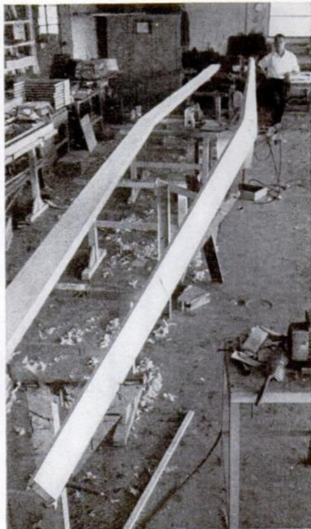
MAIN BEAM of Canadian spruce is wing's backbone and largest individual piece of the RF-3. Even in kit form, beam would not be broken down for shipment
