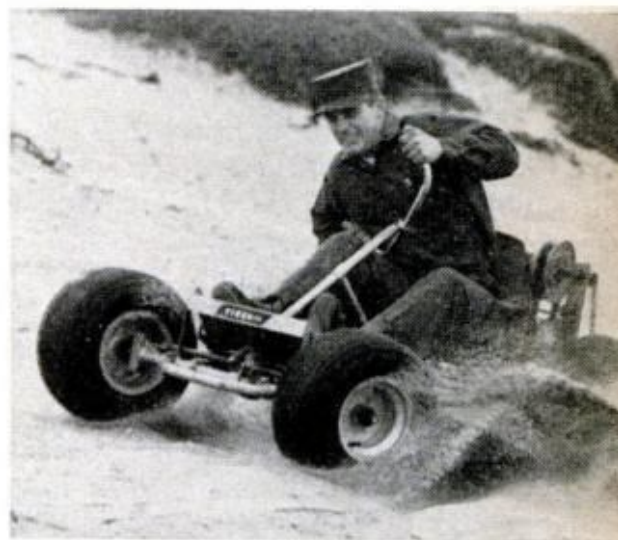
RESPONSIVE STEERING ARM and rear engine allow for sharp, sudden turns. Low, squat frame and wide tires give sand buggy amazing stability
