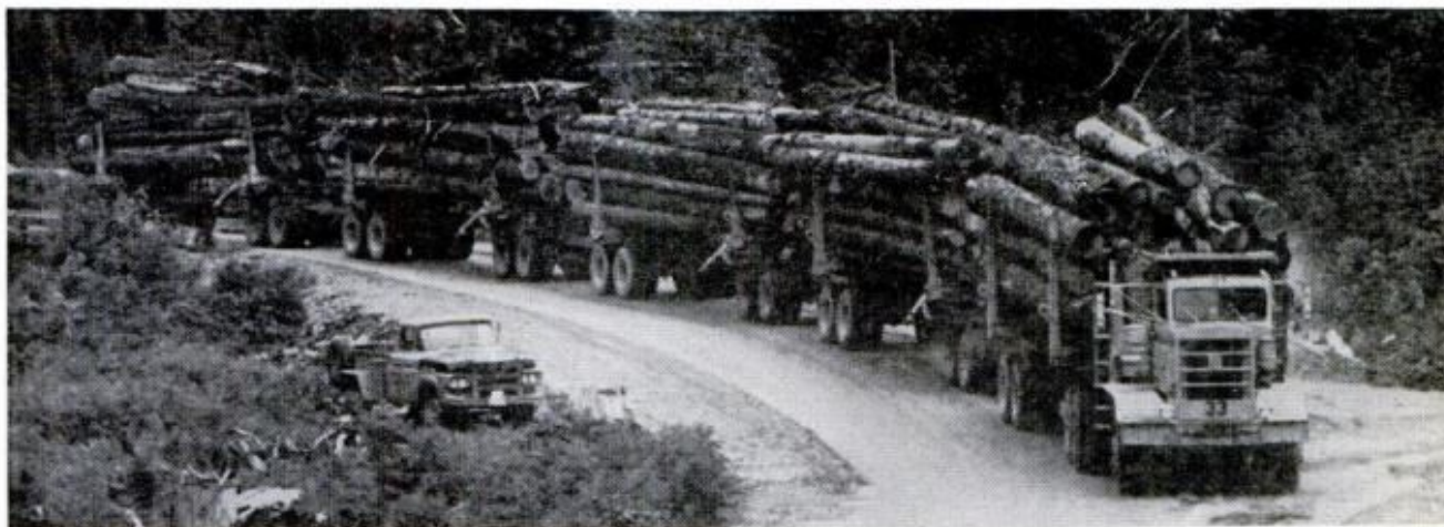
Loggers' wagon train. Experimenting with the extreme in highway hauling, Crown Zellerbach Canada Ltd., a wood pulp company, hitched together a train of five trailers loaded with 32-foot-long logs and hauled by a single 370-hp tractor for the seven-mile trip from the forest to the log dump. The caravan of 50,000 board feet of logs weighs 350,000 pounds.
