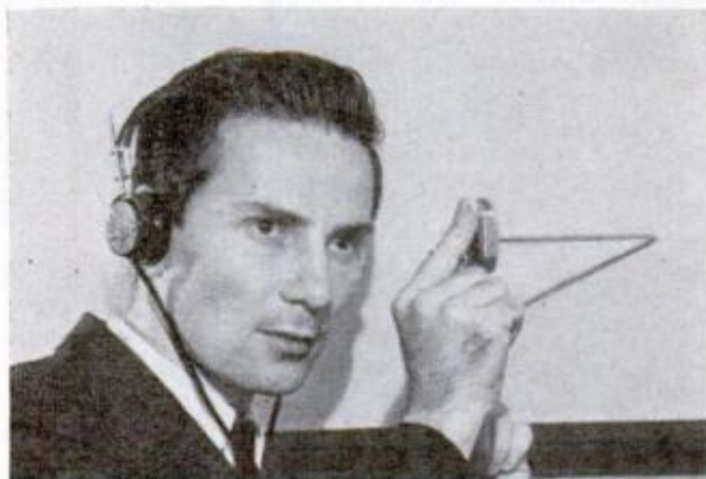
VIBRATION MICROPHONE in hands of criminal research expert Bill Eaton picks up whispers through wall of room. It's small enough to carry in pocket
