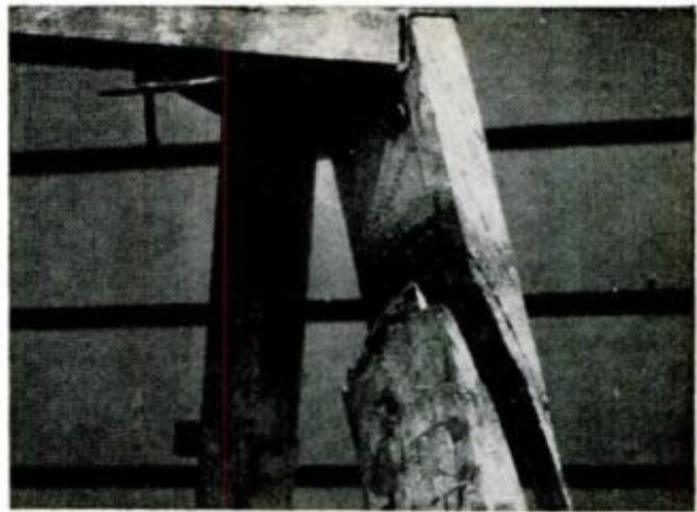
WHY STRAIGHT GRAIN is important: Break in this ladder followed the grain where it ran from edge to edge on the side rail, instead of from end to end
