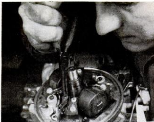
AFTER REMOVING the retainers, pull out the movable point and the spring which holds the points closed
