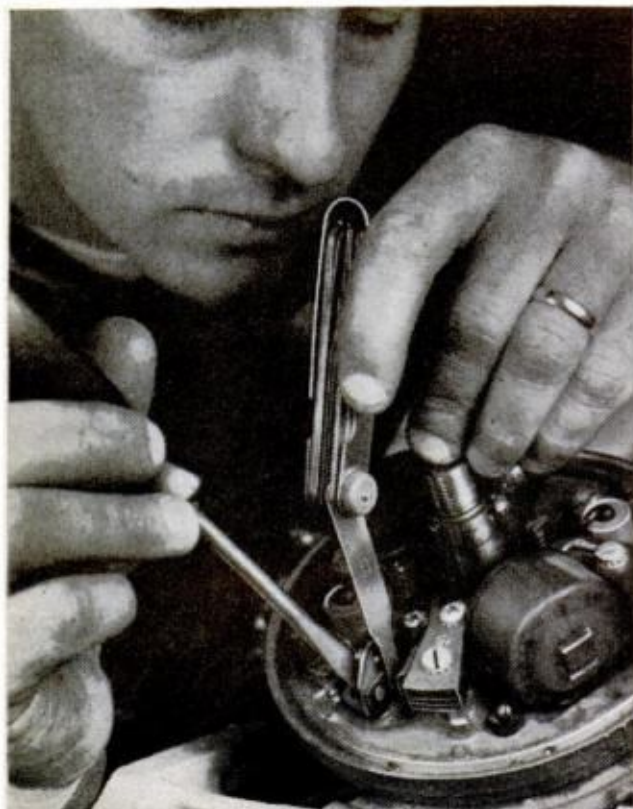
BE METICULOUS as a jeweler when setting point gap. Adjust until you feel a slight drag on the gauge
