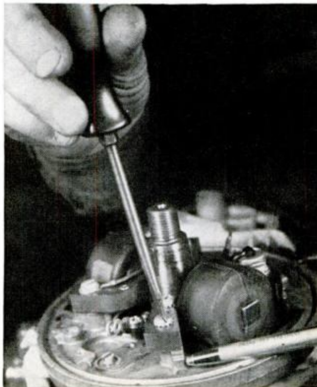
CHECK THE MAGNET for streaks which indicate that the core laminations are probably out of alignment
