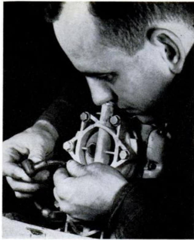
PLUG BOOTS should be checked for cracks since these mean that the plug isn't getting proper protection
