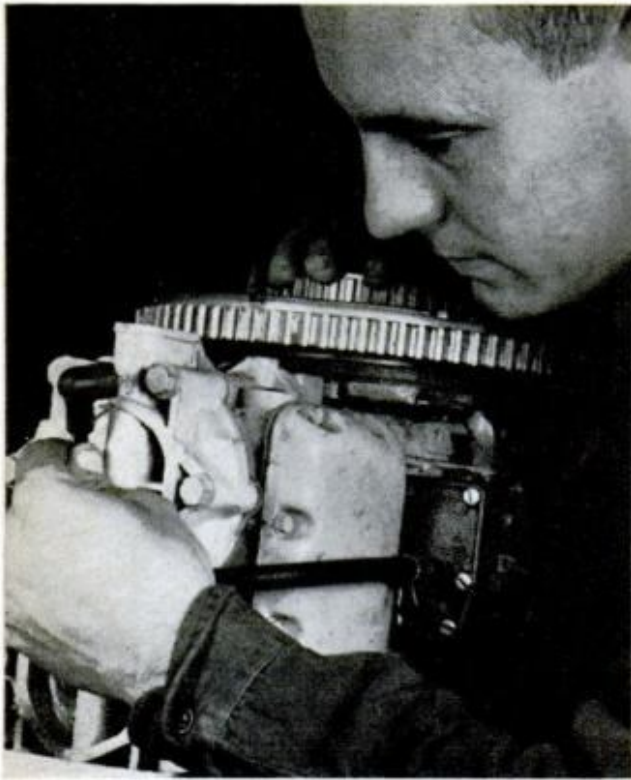
SIMPLE TEST to determine whether you have a mag problem involves pulling plug wire to check spark
