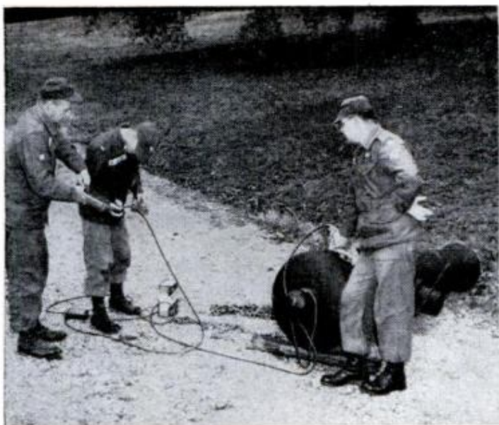
LOADED GUNS created another problem. Ordnance men pumped oil at high pressure into barrel and also tried explosive charge. Both attempts failed
