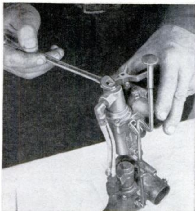
FUEL FILTER on this Mercury carburetor is hidden under a cover which must be removed for servicing
