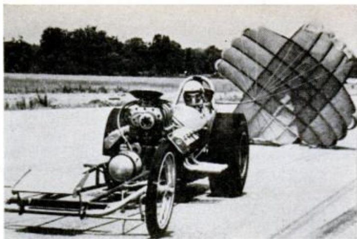
DRAG CHUTE is main deceleration device for unlimited dragsters. Its 4.5-G surge throws driver up against shoulder harness when it first pops open
