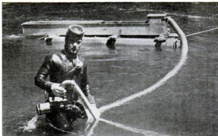
SURFACE DREDGE has a sluice box mounted on Styrofoam floats. The diver works underwater using the suction head like a vacuum cleaner to remove sand and gravel from the bedrock and expose the cracks and crevices where it is possible to discover the nuggets of gold
