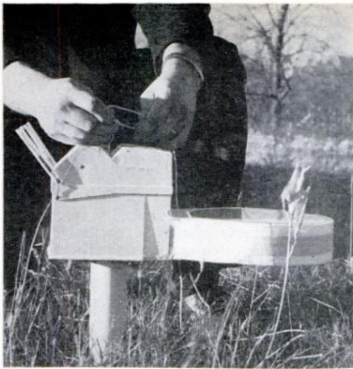
INSTRUMENT PACKAGE is tied to parachute before launching. About 50 percent of the packages are found undamaged and are returned to researchers
