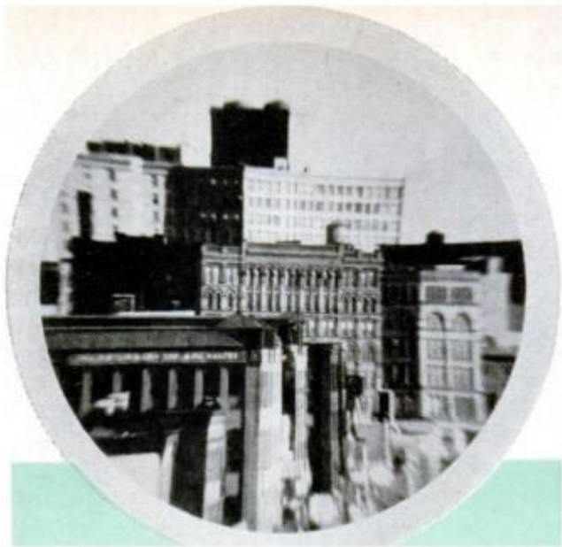
EXCESSIVE DISTORTION is evident in this glass. Note how image blurs and vertical and horizontal lines are being twisted out of shape to the point where this instrument is useless
