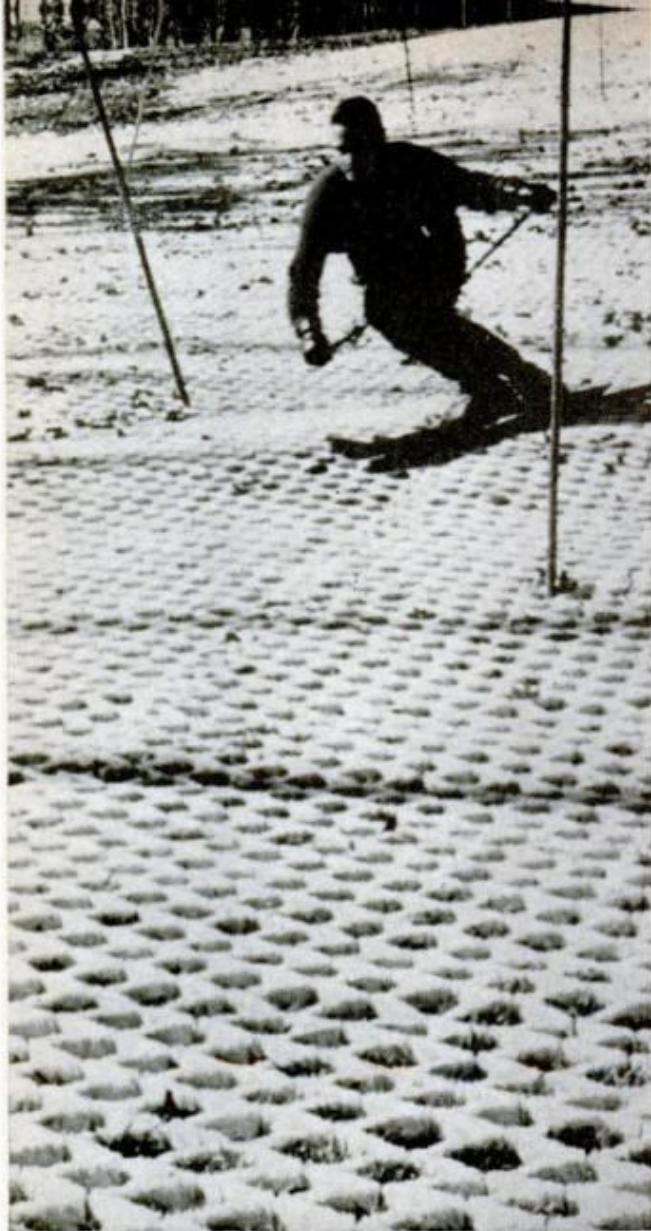
HONEYCOMB OF VINYL bristles provides surface that skiers say "gives" enough to permit the same edging and weight control that are used on the real thing
