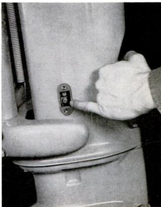
SHIFT ROD mechanism on this Gale is located under a cover plate on the housing. You'll have to loosen this before lower unit can be removed from motor
