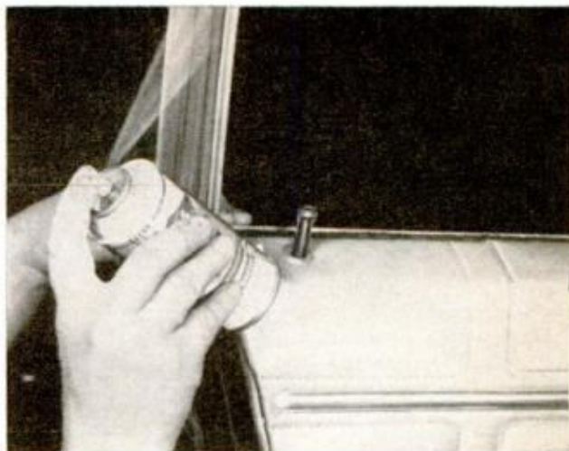
DRIED-OUT WEATHERSTRIPPING on a door can produce an irritating squeak when door is opened. Keep it pliable and noise-free with silicone spray lubricant
