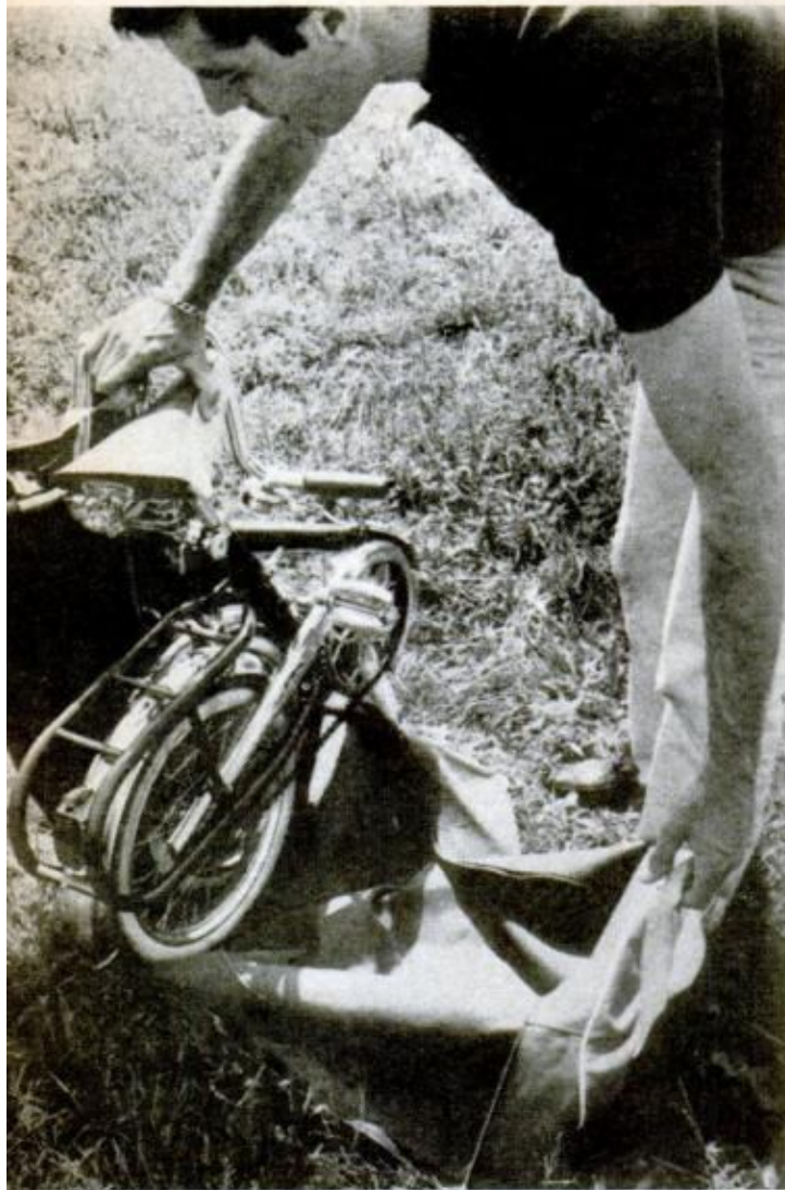
TRANSPORTATION around the camp ground is afforded by an Italian folding bicycle that is carried in a zippered case and can be assembled in 30 seconds
