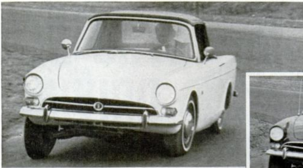
AIMING AT HOLDING THE INSIDE shoulder as a marker, we found the Tiger (above) could do better at four mph faster than the standard Alpine (right). Tiger rack and pinion steering is slightly heavier than the Alpine recirculating ball system
