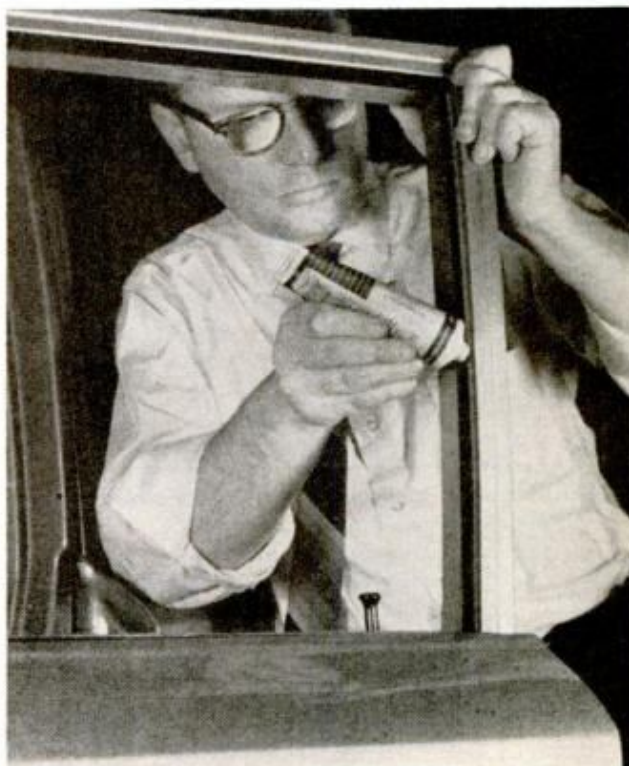
DON'T FORGET WINDOW CHANNELS. Silicone spray or grease lube will assure continued smooth operation
