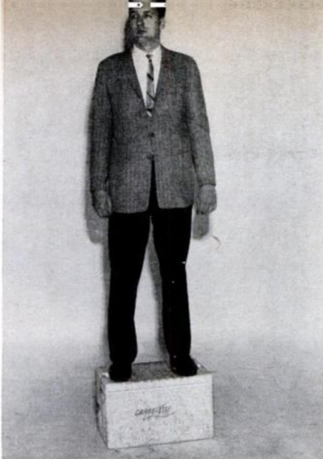
PLASTIC-COVERED polystyrene cooler that sells for $14 proved remarkably strong, surviving drop test and easily supporting the weight of a 230-pound man
