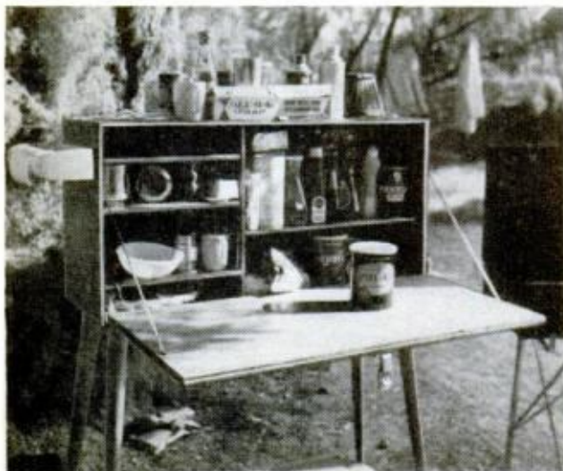
PORTABLE CUPBOARD was designed by boat camper for on-shore use. To build one, first assemble all the items you wish to store and mock it up in cardboard
