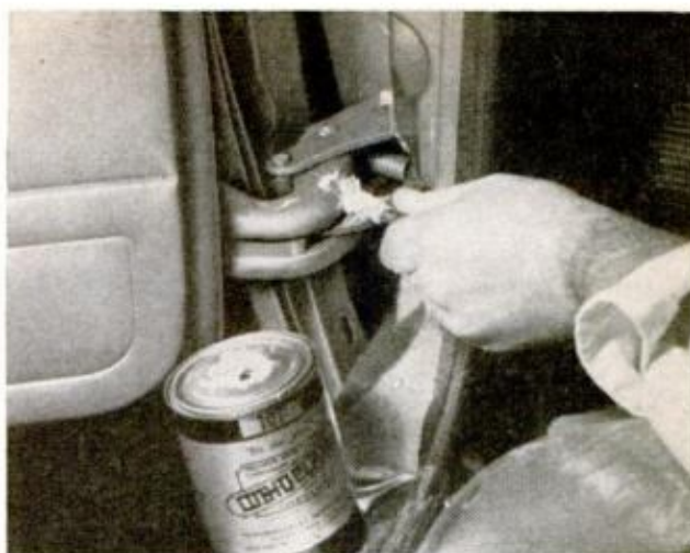
ON DOOR CHECK MECHANISMS , be sure to hit all sliding surfaces and pivot areas with grease or oil
