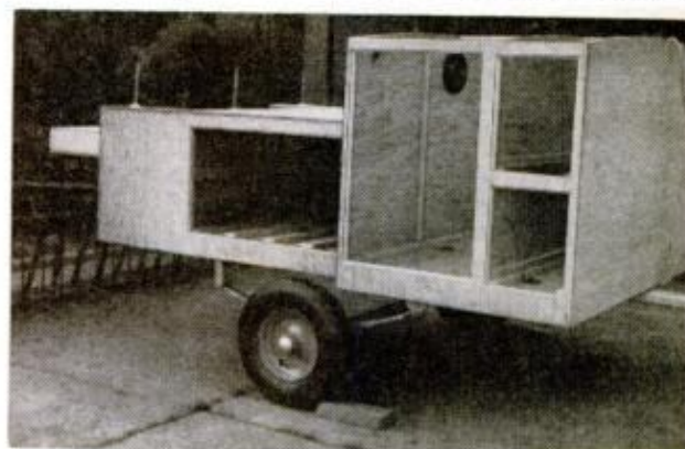
FRONT PARTITIONS are anchored to bed with screws through framing feet (above); add lateral bracing, then apply side panels with glue and screws (below). Rear deck laps all verticals, ties assembly together
