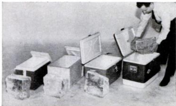
PLACING 25-POUND chunks of ice in four different type coolers, we sealed coolers for three days. Only the $3 Styrofoam chest contained ice when opened
