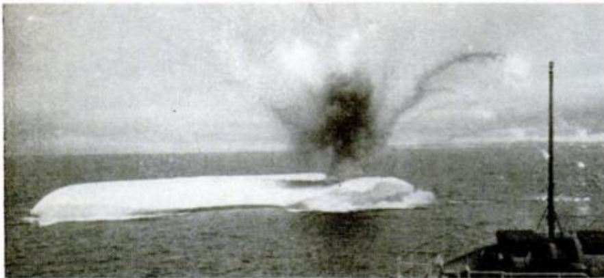
THERMITE BOMBS , which produce temperatures up to 4000° F. when they burn, were used in another experiment to melt or disintegrate icebergs. Thermite explosion made pretty pictures, but did nothing to berg
