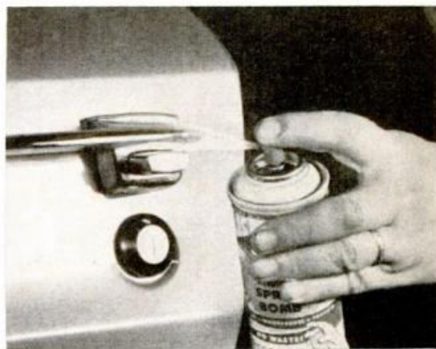
DOOR LOCKS , often ignored as lube points, should be treated with spray or motor oil and flake graphite
