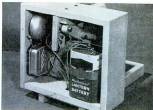
UNDERSIDE VIEW of toy shows how components fit inside base. Scoreboard wiring enters hole in back
