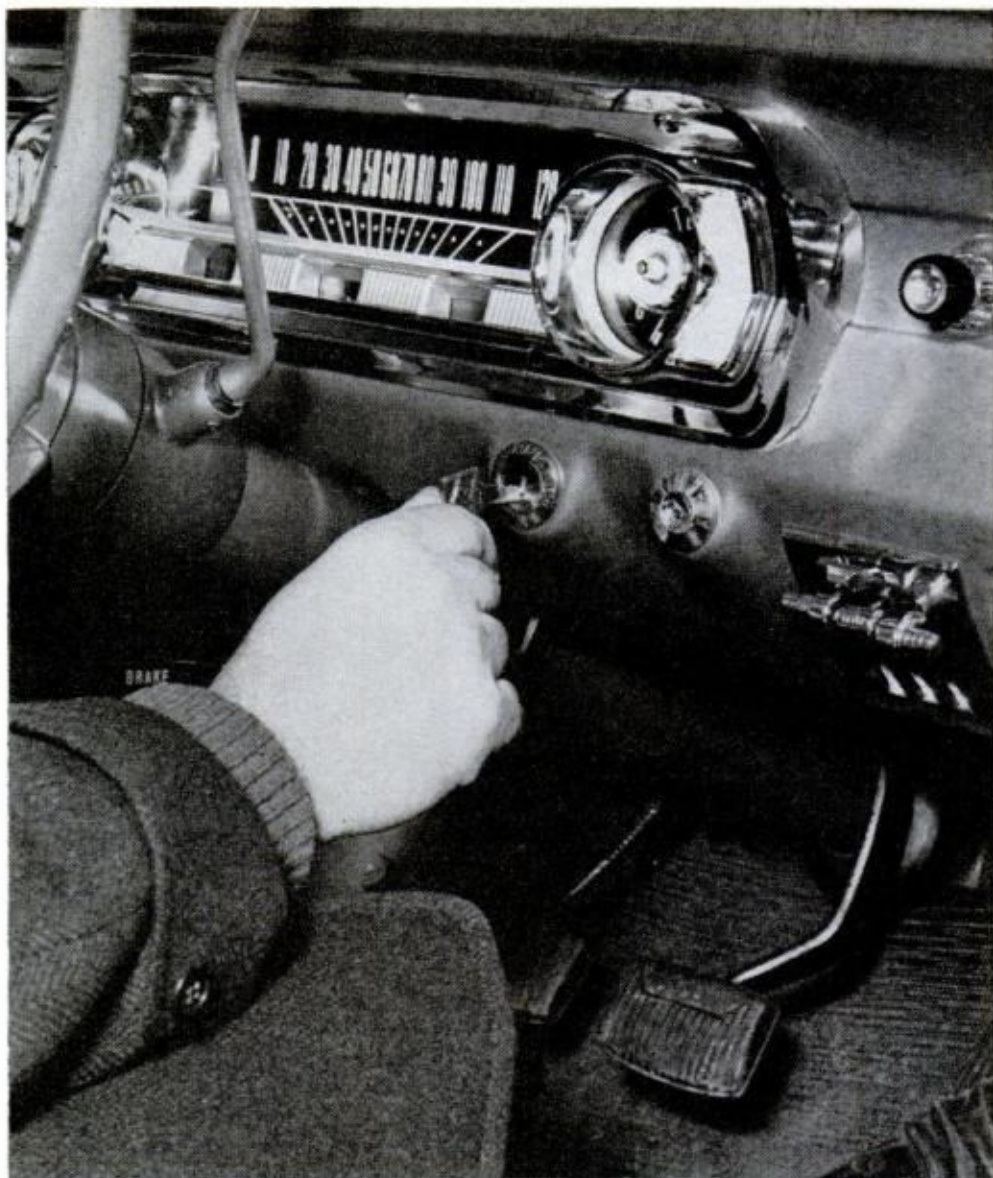
INSTRUMENT CLUSTER houses Christmas-tree speedometer and idiot lights, but owners were pleased with uncluttered instrument layout and attractive padding
