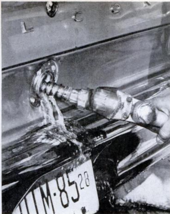
GASOLINE GEYSERS COMING FROM THE sharply kinked Falcon fill pipe got a full measure of protests by owners. Some also found the trunk sill too high
