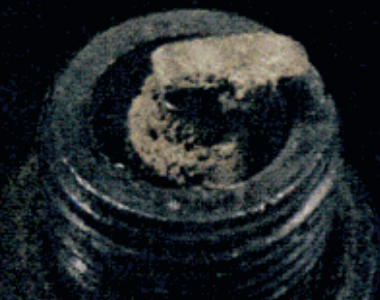
DEPOSIT FOULING —variously-colored powdery deposits caused by combustion of fuel and oil additives . . . may cause missing under high speed and heavy load conditions.
