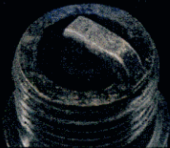
CARBON FOULING —dry fluffy black carbon deposits caused by over-rich fuel mixture, excessive choking, poor ignition, or excessive idling.
