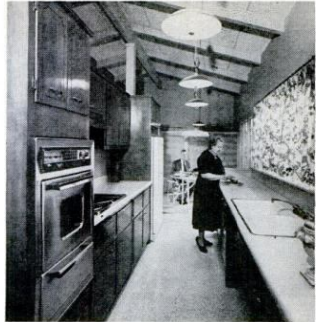
NO BEND, NO STRETCH is the aim of retirement-house kitchen planners. Lights pull down and cabinets and ovens can all be reached without stooping
