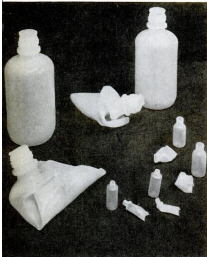
POLYETHYLENE BOTTLES shown have just been taken from boiling water. Those that had been irradiated retained their shape, but untreated ones collapsed
