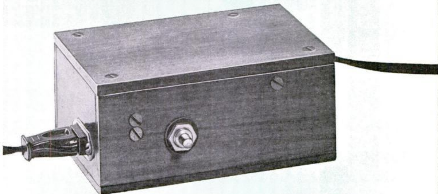
CLOSEUP of the jumping jack. The pictorial diagram of the power supply must be followed carefully. Mount the pushbutton switch in some convenient spot. The plug on the side of the power supply is from separate coil assembly
