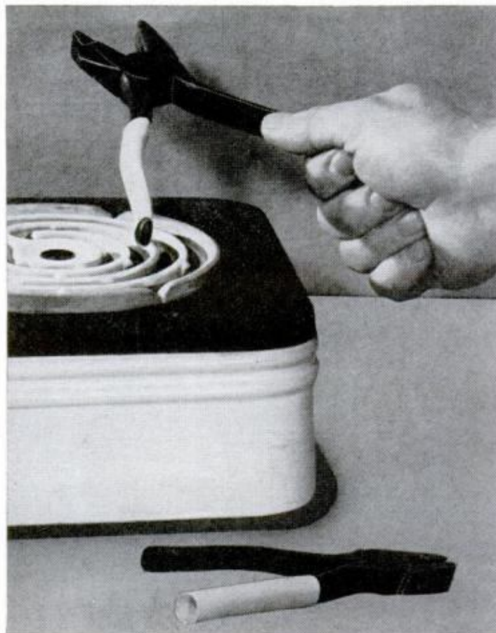
IRRADIATED TUBING is at cold size on lower pair of pliers. Moderate heat makes the plastic contract and form a tight, insulated grip for handle
