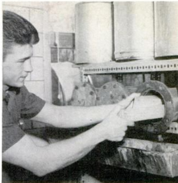
ORDINARY WOOD is put into vacuum tank. With air sucked out, cells soak up liquid plastic sprayed into chamber. Gamma rays solidify the plastic
