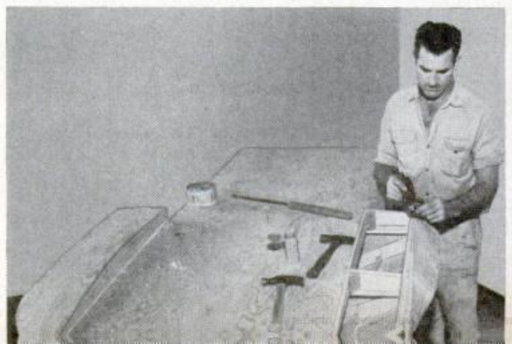
PLANKING for non-trip chine should be bevelled flush with runner so it can be lapped by bottom planking
