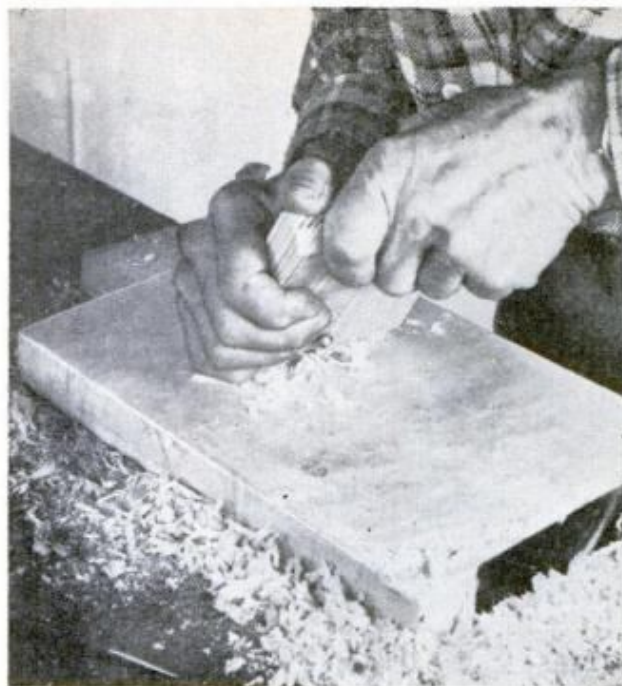
SHARP SCRAPER cuts real shavings. Sliding diagonal stroke gives shearing cut, keeps work flat. Blade above is clamped in kerfed handle, sketched below
