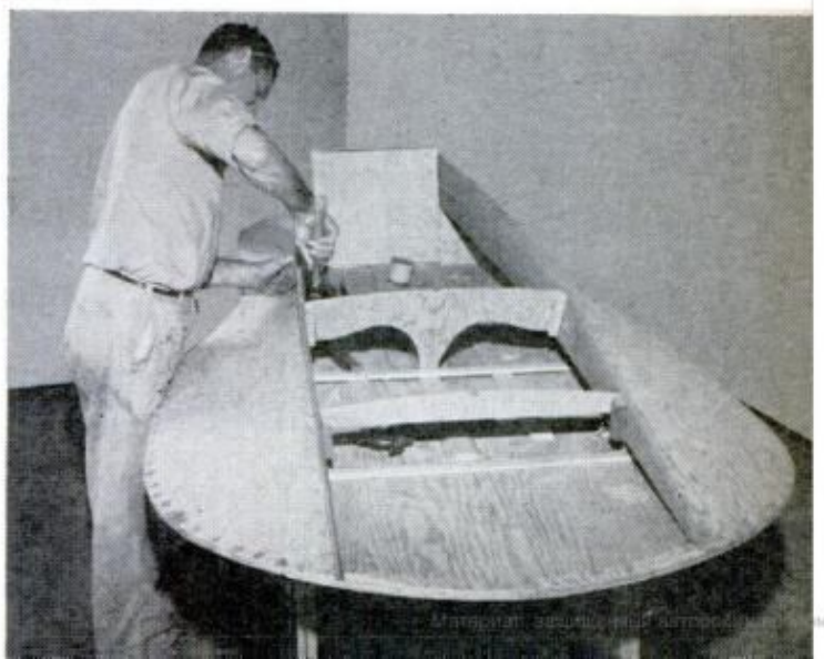
BLOCKING MOUNTED on the inside of the coaming is used to secure dash beam and forward deck beam
