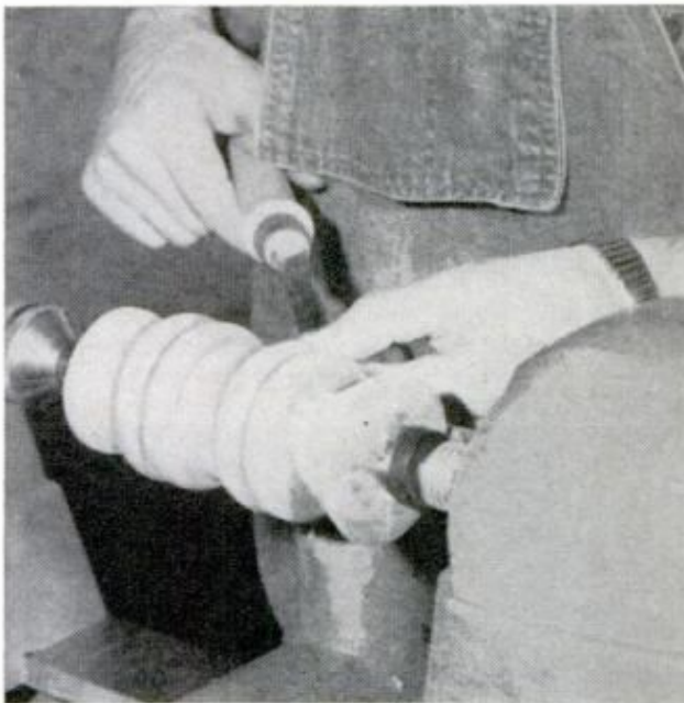
PLASTIC-WOOD composite, though many times harder than untreated wood, can be worked in the usual ways. It can be sawed, drilled, turned and sanded
