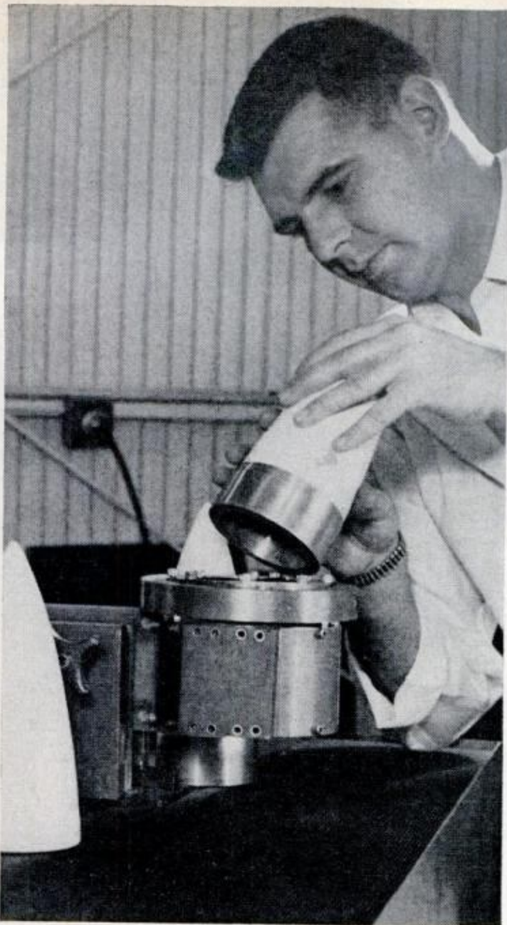
TYPE C lies flat and is used for contouring metal sheet into shape of die above it. Forming works best with materials that are good electrical conductors
