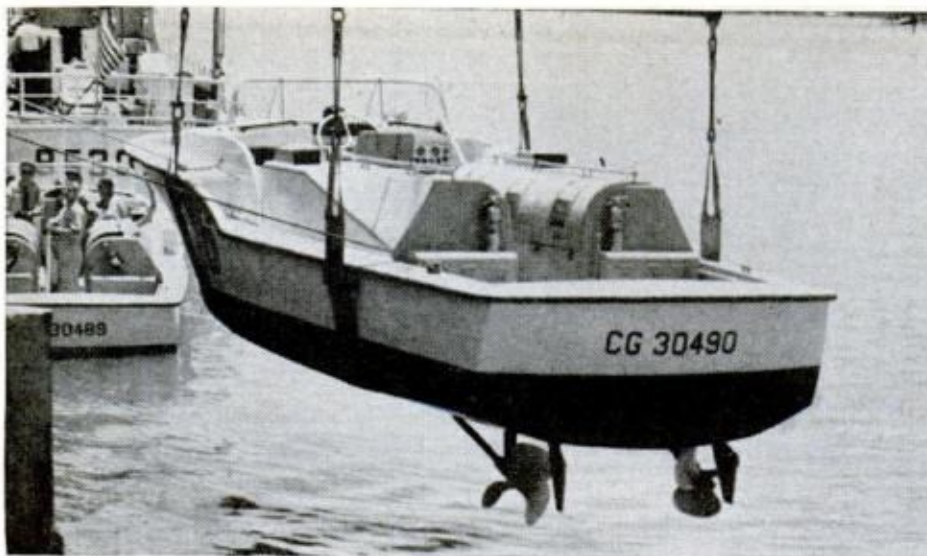
COAST GUARD boat won its class in Miami-Nassau race, required special props that had a deep pitch and were 50 percent wider than usual to utilize the output of two powerful diesel engines
