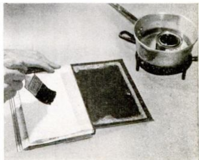
20. GLUE BOARDPAPERS to boards and place completed book in grooving jaws for final 24-hr. pressing
