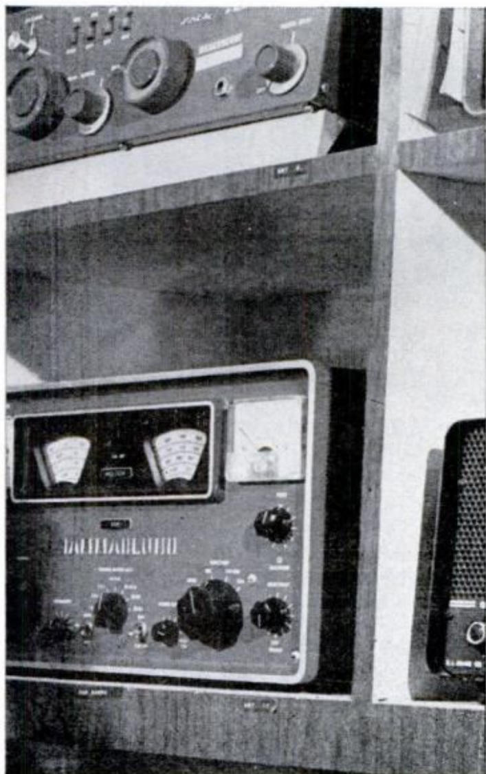
S-METERS MEASURE signal strength. Standard types (top) are easiest to read and large scale makes them most accurate. Current trend is to smaller vertical dial. Avoid the uncalibrated ones (center)
