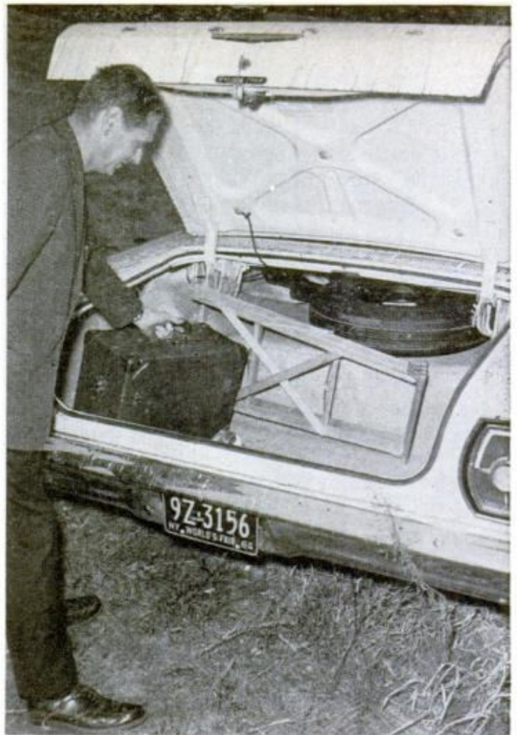
AN EXTRA TWO CUBIC FEET of trunk volume drew praise from 3.5 percent of Ford owners. It's a side benefit from squared-off style. Lift height is reduced
