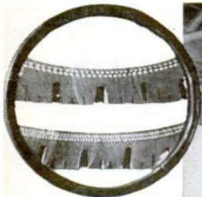
TWO-PLY TIRES USE bigger, stronger cord for similar total strengths as old four-plys. In demonstration photo (right), new cord carries total car weight
