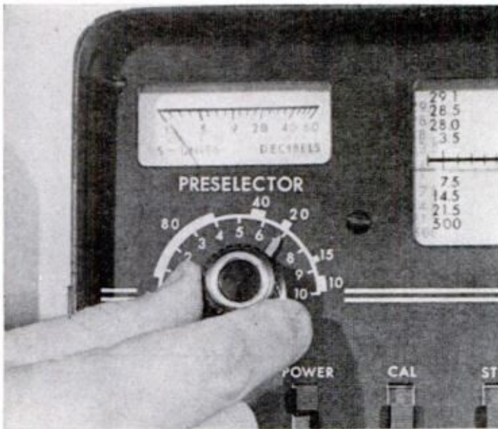
PRESECTOR can really bring in long-range broadcasts. This extra tuned r.f. stage is found in only the very best and most costly shortwave receivers
