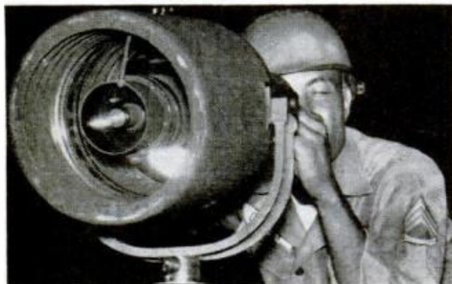
INTENSIFYING the light from moon and stars, a night sight allows soldiers to sight a weapon (top) or view a battlefield (bottom) despite total darkness
