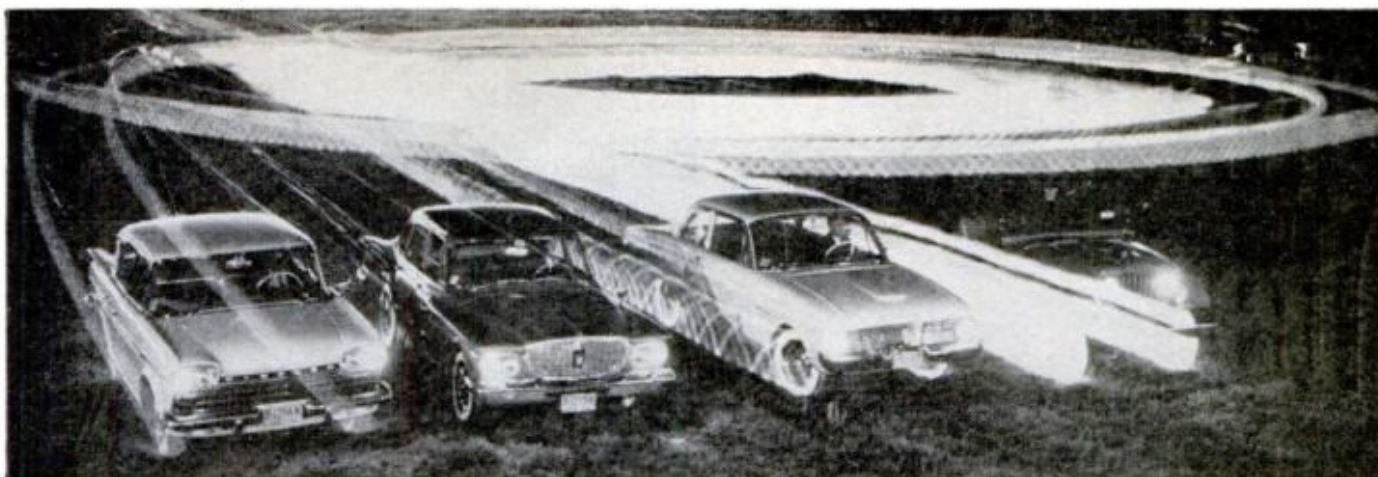
CLEAR, ATTENTION-GETTING polyurethane tires were lighted from inside for promotion shots like this. Material, so tough it needs no cord of any kind, hasn't made the grade. Tires grow until they're too big for the wheel wells
