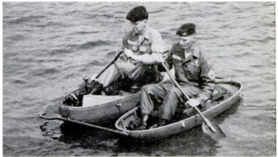
DESIGNED FOR GUERRILLA WARFARE , this two-man boat is primarily used as a load carrying device. The two sides fold together like a suitcase. It is waterproof and can be carried or skidded across the terrain by two men
