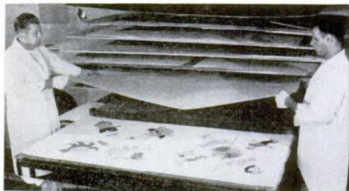
CARTOON DESIGN sheet for table tops at Shawnee is covered with melamine impregnated paper that will become hard, transparent plastic surface in hot press
