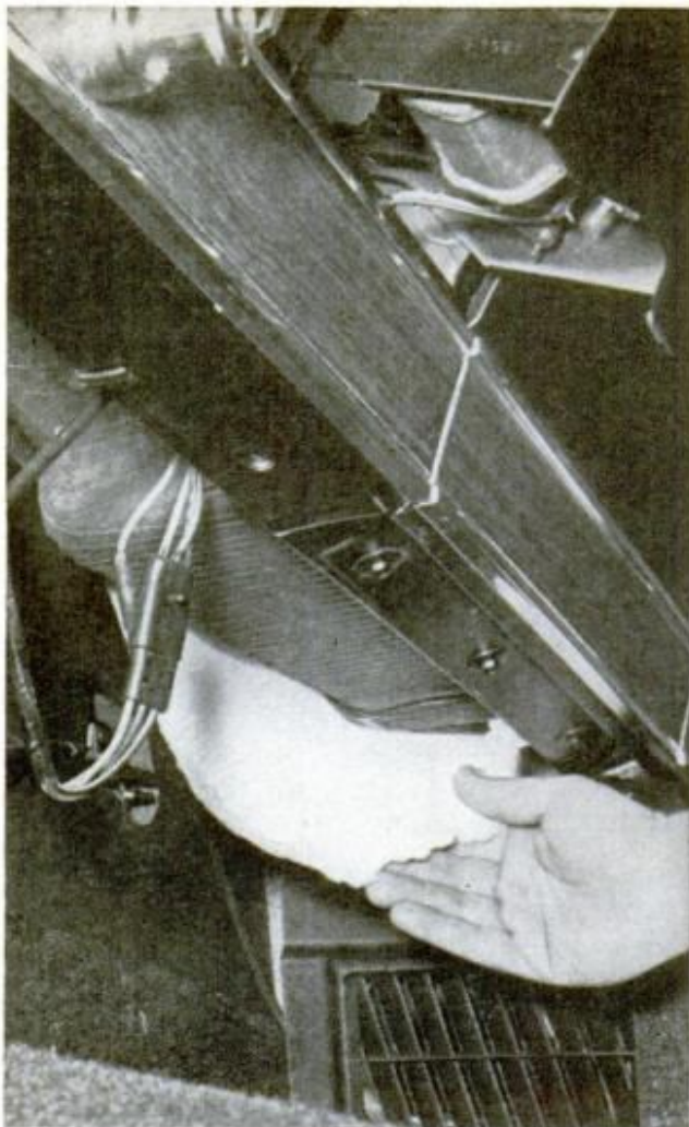
"DO SOMETHING BETTER WITH tangle under the dash," one owner asked. Test LTD also had sound proofing blanket dangling from behind glove box
