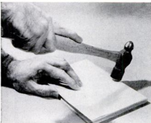
11. AFTER APPLYING flexible glue to spine, tap it into a rounded shape before the adhesive has set
