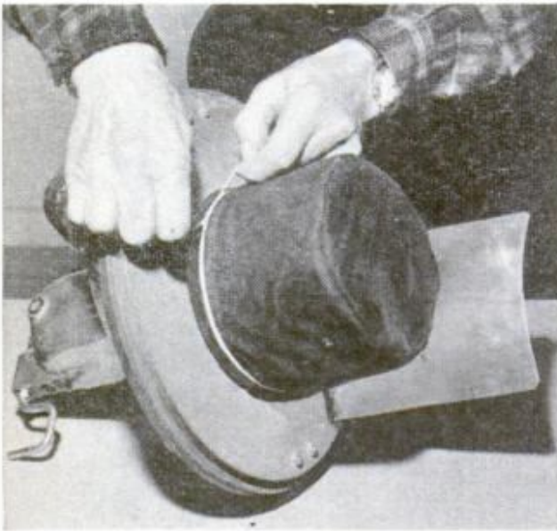
CLOTH BAG that covers blower-intake filter should be of closely woven cotton or other material that will "trap" dust particles. Tie on with double string
