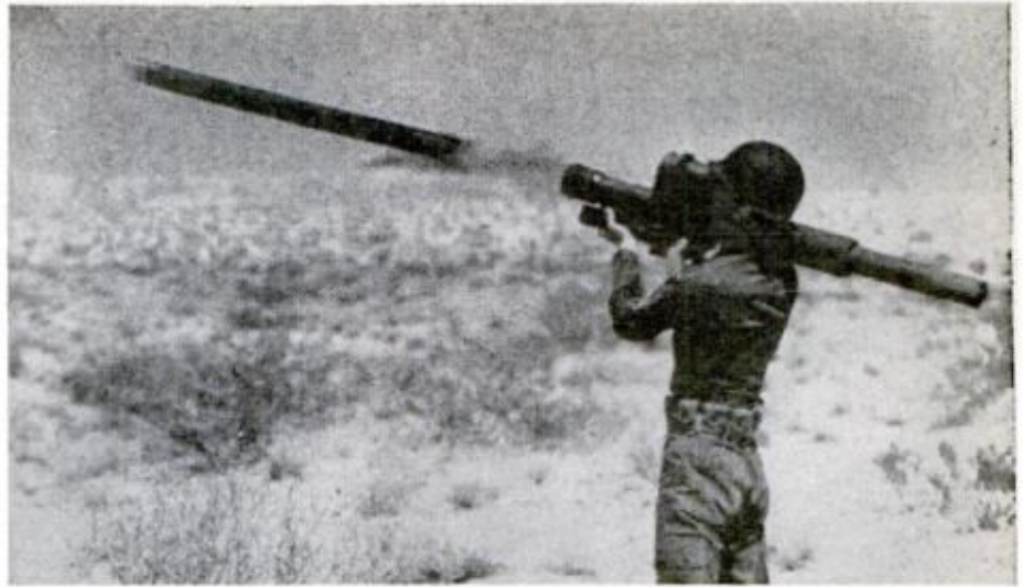
FIRED LIKE A MISSILE , the deadly Redeye missile is attracted by intense heat. When it is aimed and fired at a jet plane, it picks up the plane's exhaust pipe and heads straight for it, exploding a warhead upon contact
