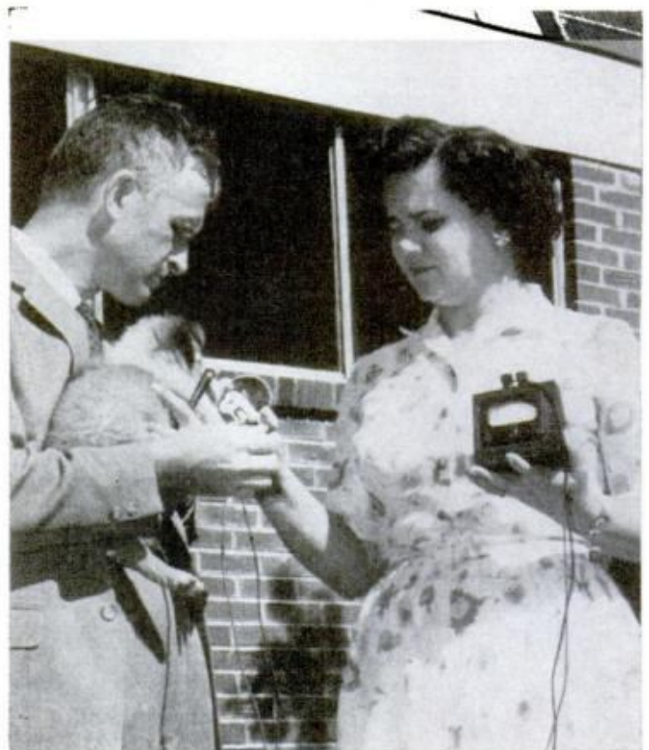
PYRANOMETER is used by the Thomasons to measure intensity of the sunlight. It provides an index to amount of solar energy being taken by system
