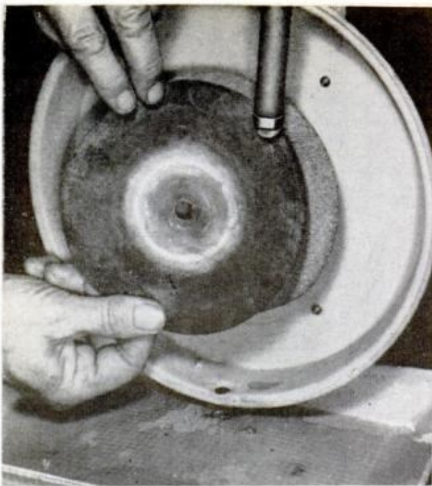
CLOTH-MOUNTED silicon carbide sanding discs in any of several grits may be used, though most work can be handled with only two different grits. A 220-grit disc is used for rough sanding; 440-grit for finishing
