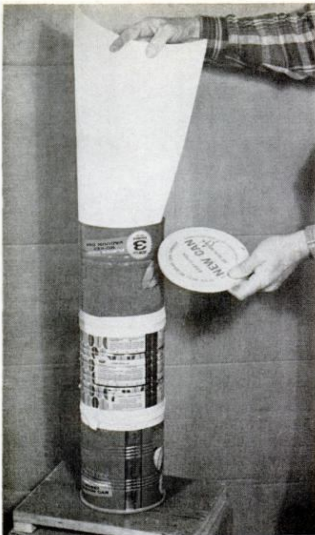
DRY DEVELOPMENT in ammonia fumes gives a ready-to-use copy in minutes. Two ounces of ammonia will last for nearly a full day's processing if care is taken to keep both top and bottom cans tightly sealed
