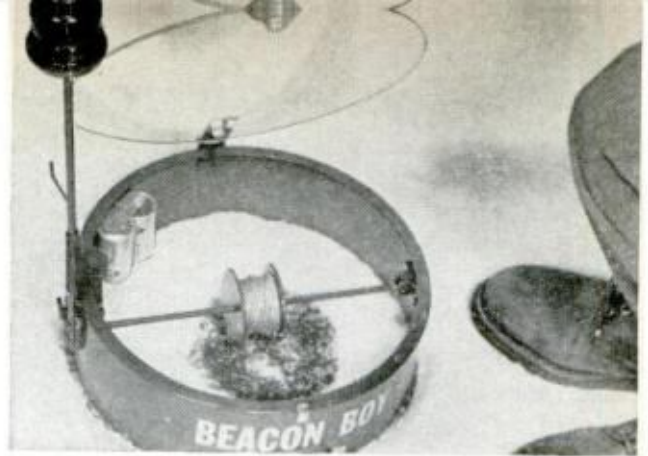
UNIQUE TIPUP employs a battery-operated signal light that is automatically flipped erect and lighted when a fish hits the line and triggers mechanism
