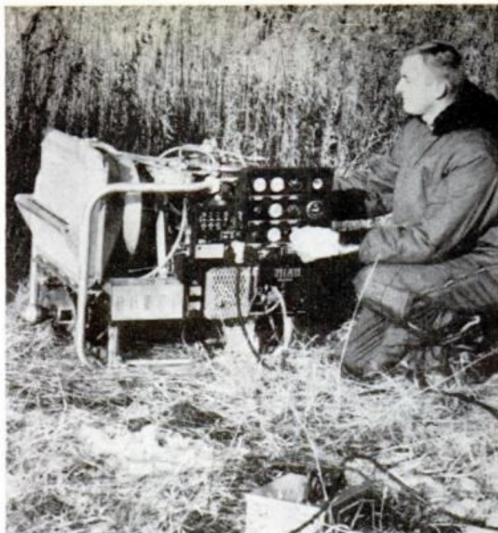
MILITARY VERSION of the Stirling engine satisfied the Army's initial requirements for a soft-spoken power source inaudible from as little as 100 feet
