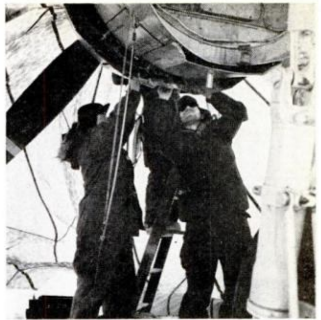
BAREHANDED CREW does minor maintenance on C-47 engine. Without warmed-up parachute tent, hands would stick to super-cold metal parts of plane
