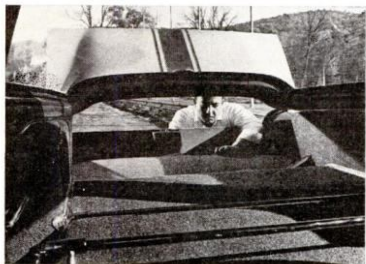
BARRACUDA, LIKE MUSTANG , gives long-load capacity by dropping its rear seat and trunk panel. Bar in foreground restrains load or latches seat upright
