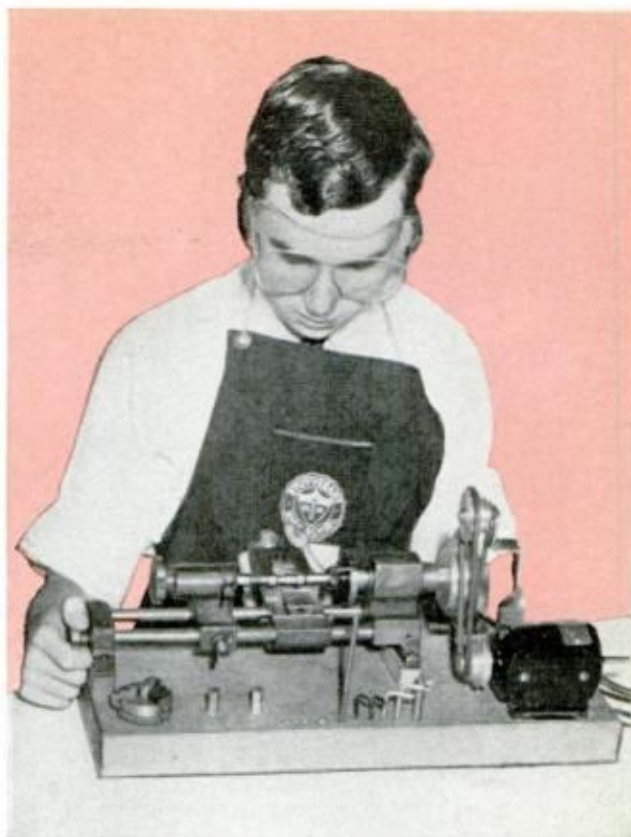
HERE IS ONE of some 300 lathes which have been made by students in learning to operate a metal lathe
