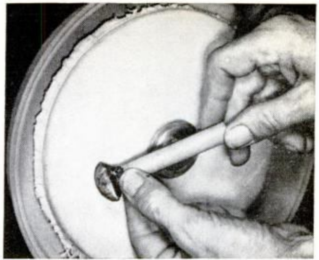
POLISHING WHEEL is made by cementing a sponge-rubber disc to plywood. The assembly is then covered with canvas held in place with chalkline. Charge wheel with a mixture of polishing powder
