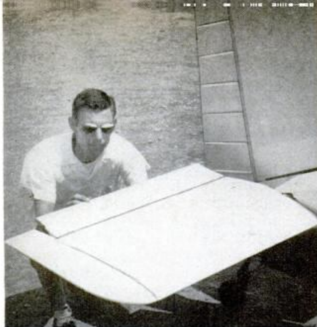
'FLYING TAIL' , designed by Thorp, is all elevator without usual horizontal stabilizer. Bill Warwick was first of 150 T-18 builders to finish his plane
