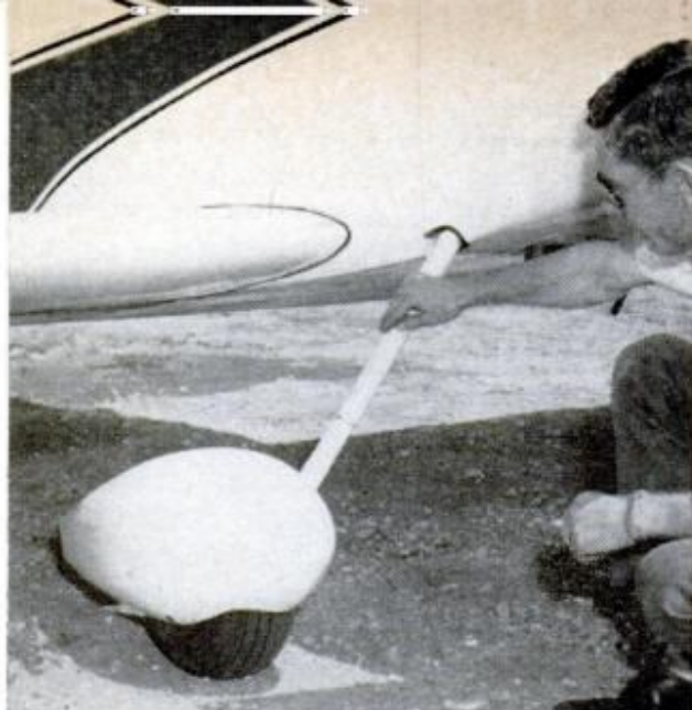
LANDING GEAR , another innovation, is shaped like an "A" and secured to fuselage behind the engine. This part, and others, can be purchased by beginners
