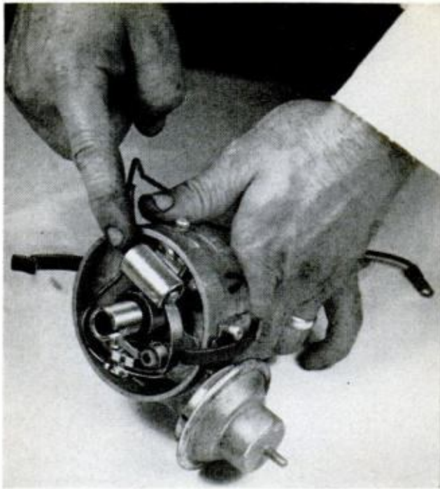
CONDENSER SNUGGLES against rotor shaft. It's a decoy for left-over current when breaker points snap open, prevents arcing which could burn up points
