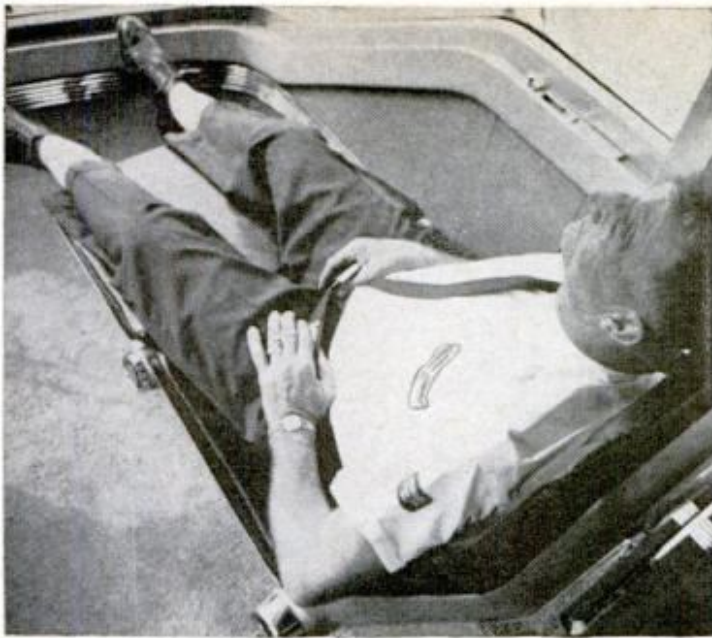
CONTOURED LOUNGE FOR CO-DRIVER proved very comfortable. It was built to recline, but later welded in fixed position because of elusive prototype rattle
