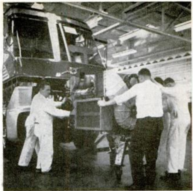
FORD'S TURBINE is virtually two engines in one, producing 45 hp. for running accessories or, with supercharging section triggered, the full 600 hp.
