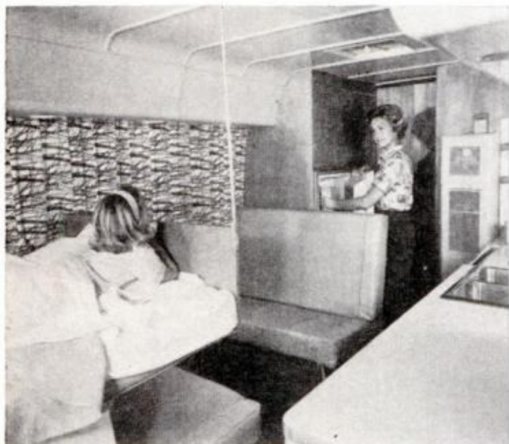
TWO DOUBLE BEDS fold out in ingenious over-under fashion. Interior lights are individually controlled so you can work or read while the kids sleep
