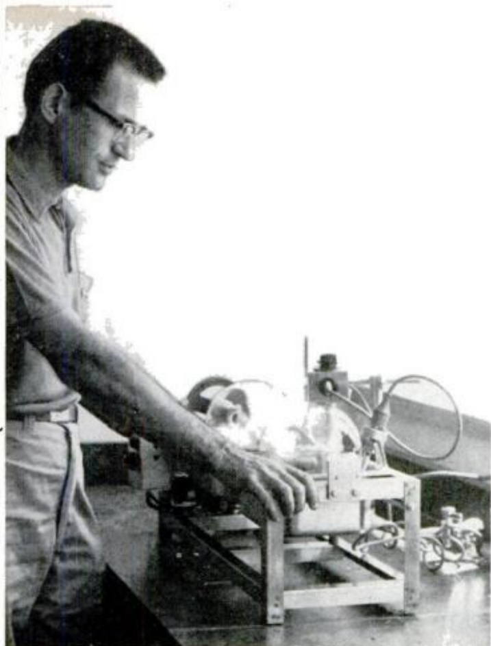
EVAPORATOR is used by bacteriologist John Sieburth to extract moisture from Sargassum weed, which contains an antibiotic and is plentiful in Atlantic
