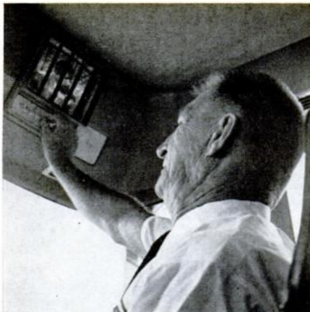
TV SET IN FRONT OF CO-DRIVER has vertical slats so driver's attention isn't distracted. Separate co-driver's air-conditioning control is at the right
