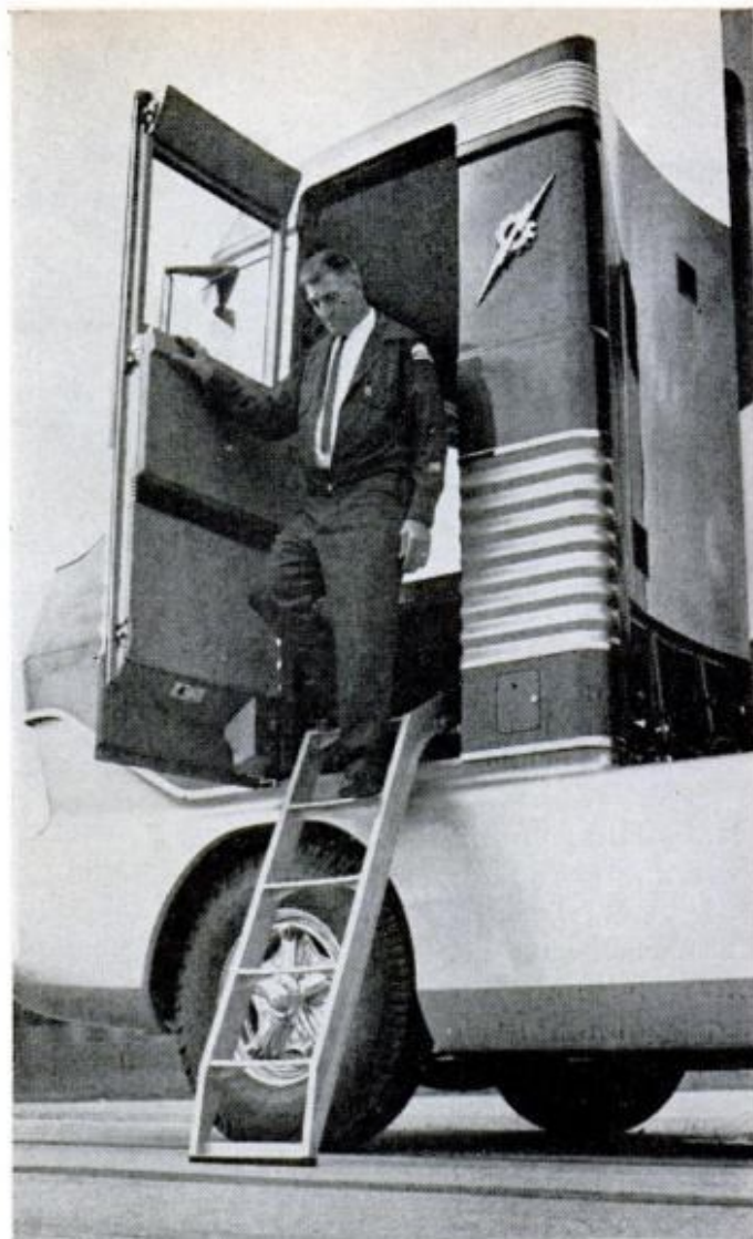
AIR-CYLINDER-OPERATED DOOR opens and electrically powered ladder swings down for easy entry. Cab is slightly pressurized and free of engine fumes
