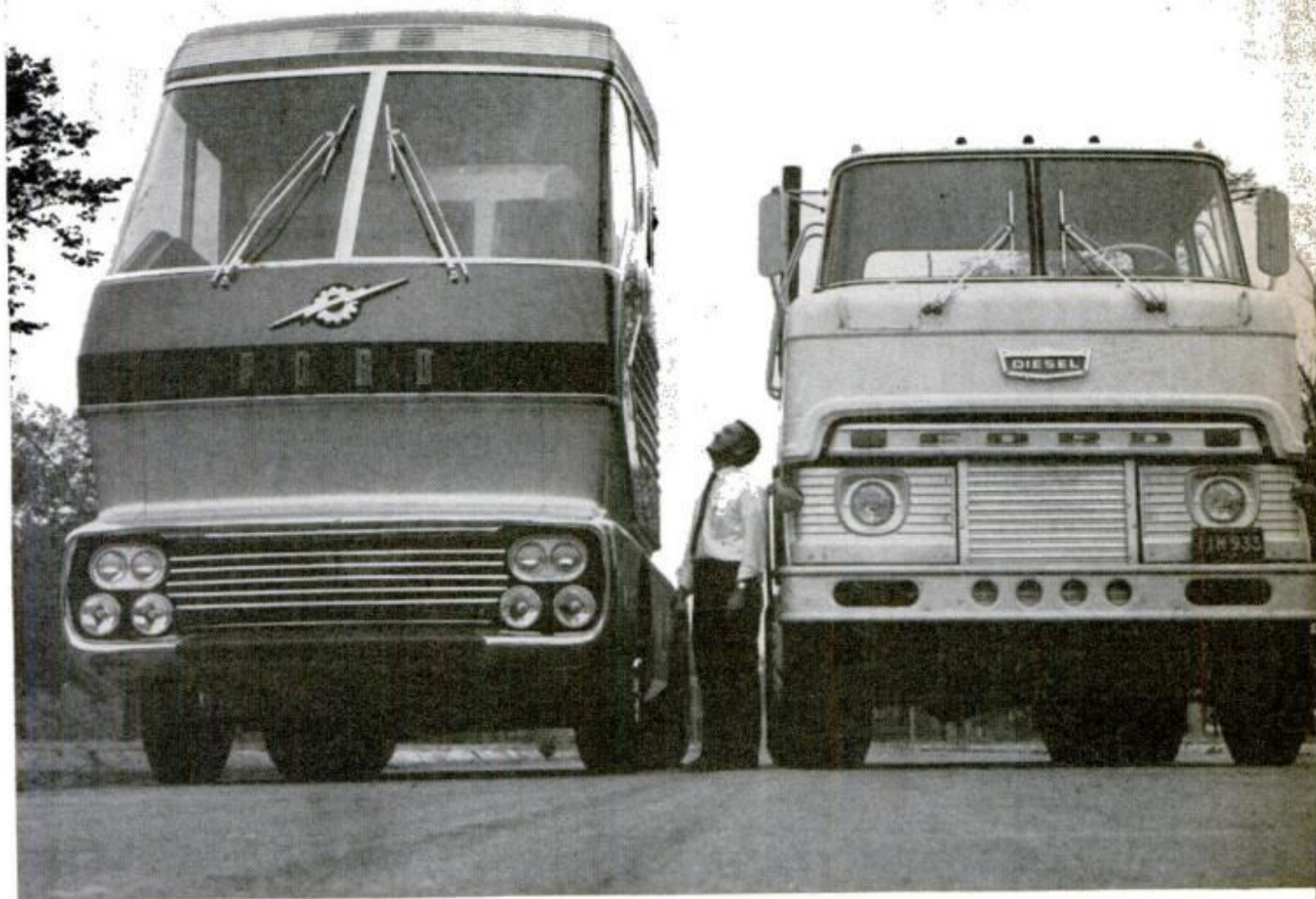
TURBINE TRUCK DWARFS FORD'S BIGGEST DIESEL. Fiberglass cab was built in two sections because of low ceiling. On today's roads, clearances are a problem. In some states, special permit is needed before driving through
