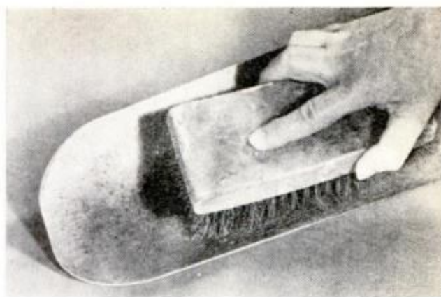
WIRE BRUSH , followed by emery cloth, removes rust and caked-on dirt from spades, trowels and shovels
