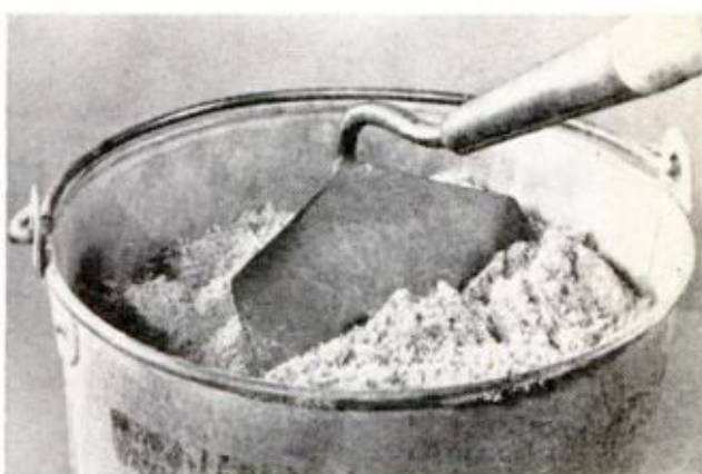
LIGHT RUST AND DIRT comes right off when you work tool in a bucket of sand mixed with machine oil
