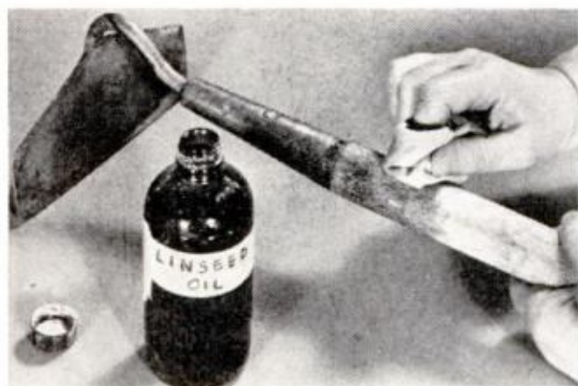
KEEP MOISTURE OUT of handles by sanding any rough spots, and applying several coats of linseed oil
