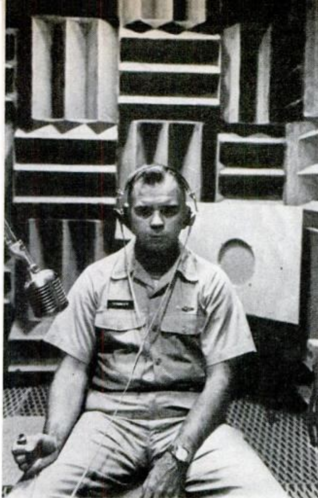
SOUND ROOM , set on springs and heavily baffled, tests hearing level through headset and also through vibrators placed on mastoid bone behind each ear
