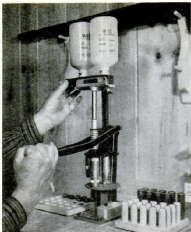
SINGLE STAGE RELOADING PRESS performs the same basic steps as hand loader on previous page, but is much faster. Containers on top hold powder, shot
