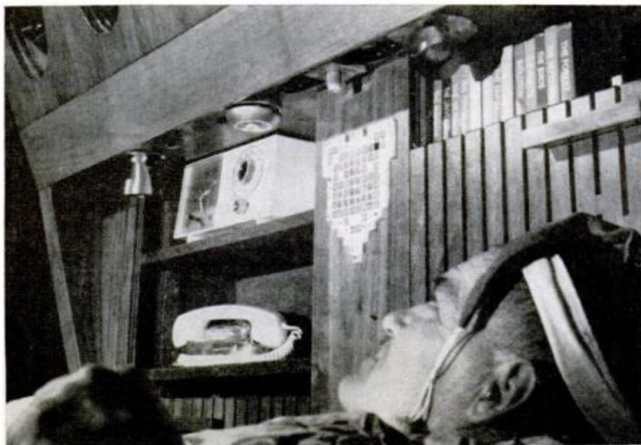
CLOSEUP OF CONSOLE shows controls for television, intercom system, reading lamps, room temperature. Vertical sliding panels are counterweighted for easy closing. Bed is hand-rubbed walnut with shelves and dividers.
