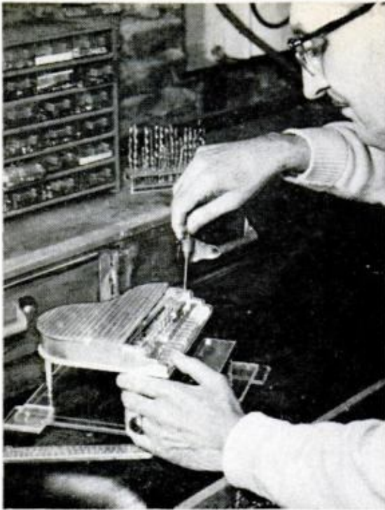
ALUMINUM MOTORCYCLE is miniature of real motorcycle scaled down from advertising photo. Wheels are made from plastic, scored to simulate spokes. Note rear seat, bag
