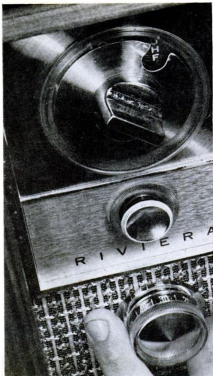
UHF TUNER SHAFT must be carefully positioned to conform to your particular model receiver. Work slowly and follow instructions to the letter
