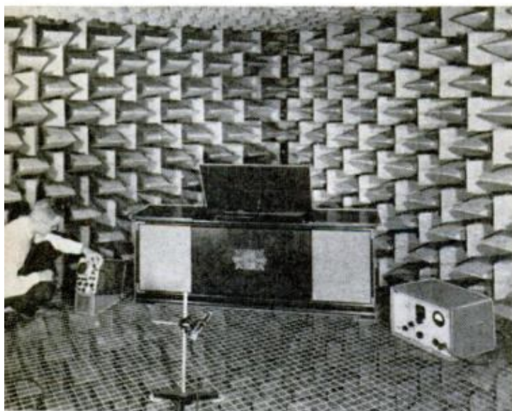
ANECHOIC CHAMBERS facilitate precise control of sound for research on sound measuring devices. This one has 3000 wedges of sound-absorbing material
