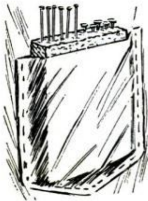
IF YOU FIND that water still enters the space at the top of a screen door despite the regular drip cap, a section of venetian-blind slat mounted over the door will provide a rain canopy to prevent door swelling
