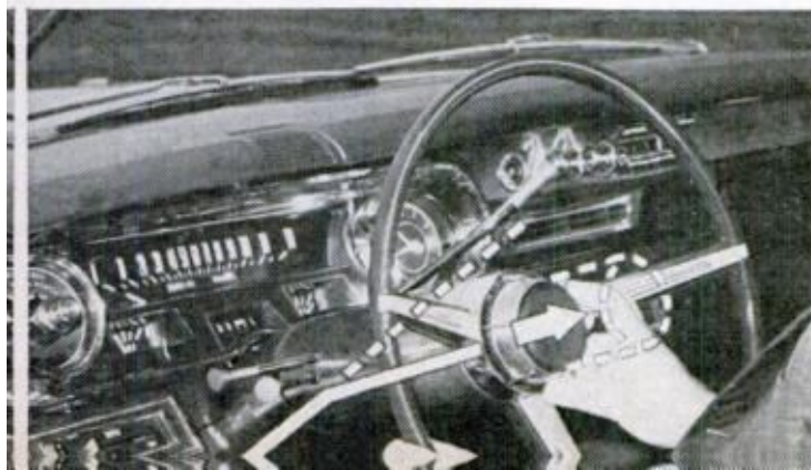
OPTIONAL TELESCOPING steering wheel in Cadillac and Corvair adjusts up to three inches with a twist of a hub ring. Separate lever controls tilt angle
