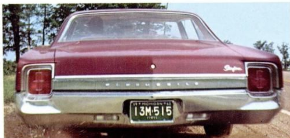
OLDS Starfire may dust off some competition with 10.2-second 0-60 time. It has 425-cu.-in. V8, variable-pitch automatic transmission
