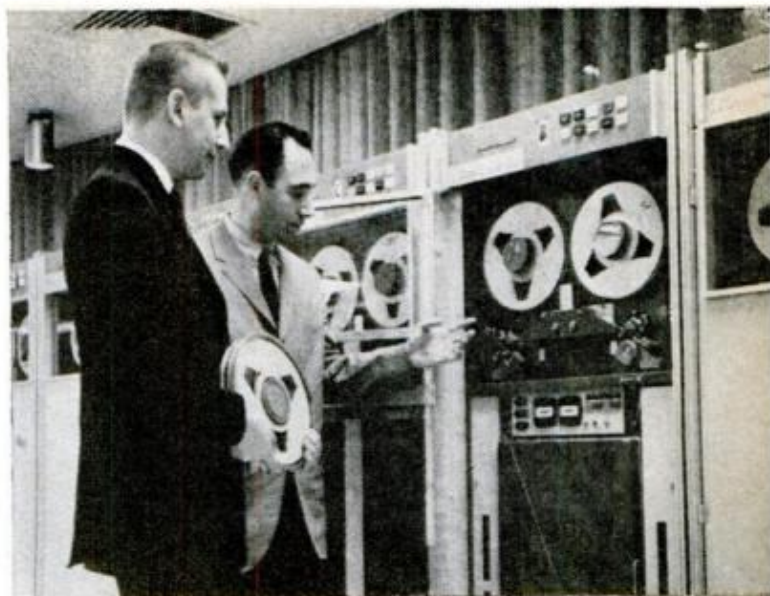
TAPED DATA are stored on reels for quick selection by computer itself. Reproduced below is section of actual flow chart showing typical one-step commands
