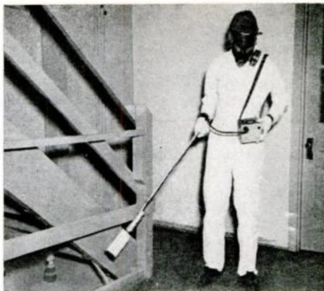
PROTECTIVE clothing and equipment used by AEC inspector (above) are same as the Hot Squad's gear. Man is shown taking reading with a fish-pole meter
