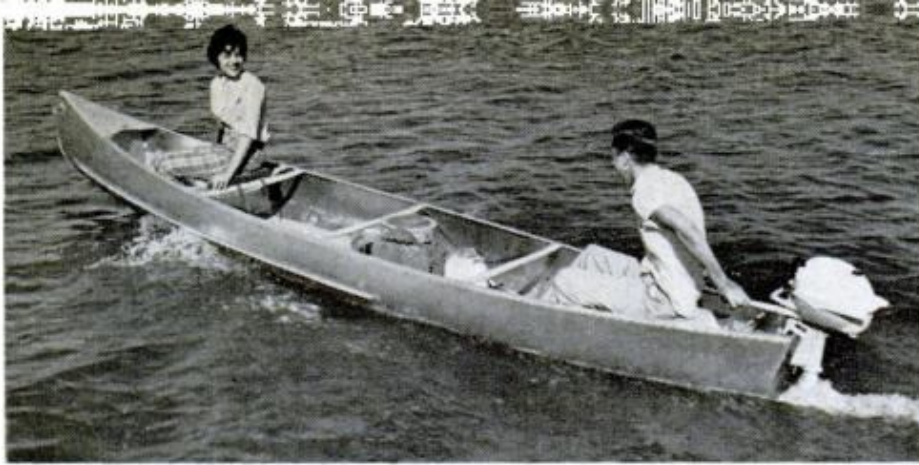
SQUARE ENDER , made of aluminum, is driven here by three-horsepower outboard. However, it will take up to 5\frac{1}{2} horsepower. Note the spray rails just above the waterline of the canoe
