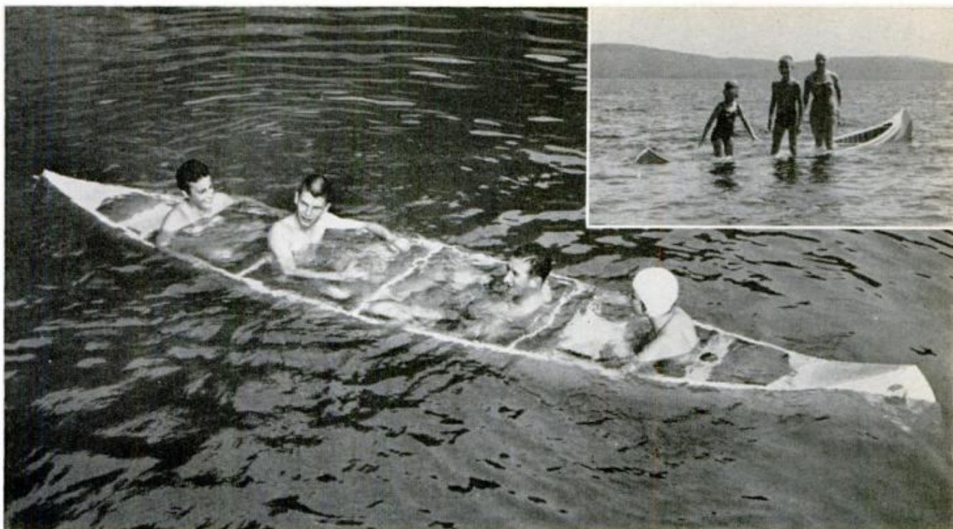
FLOTATION CHAMBERS in most aluminum and some fiberglass canoes will keep a swamped craft afloat, even with passengers aboard. Sponson canoe (inset) with air chamber on each side from bow to stern is almost impossible to tip
