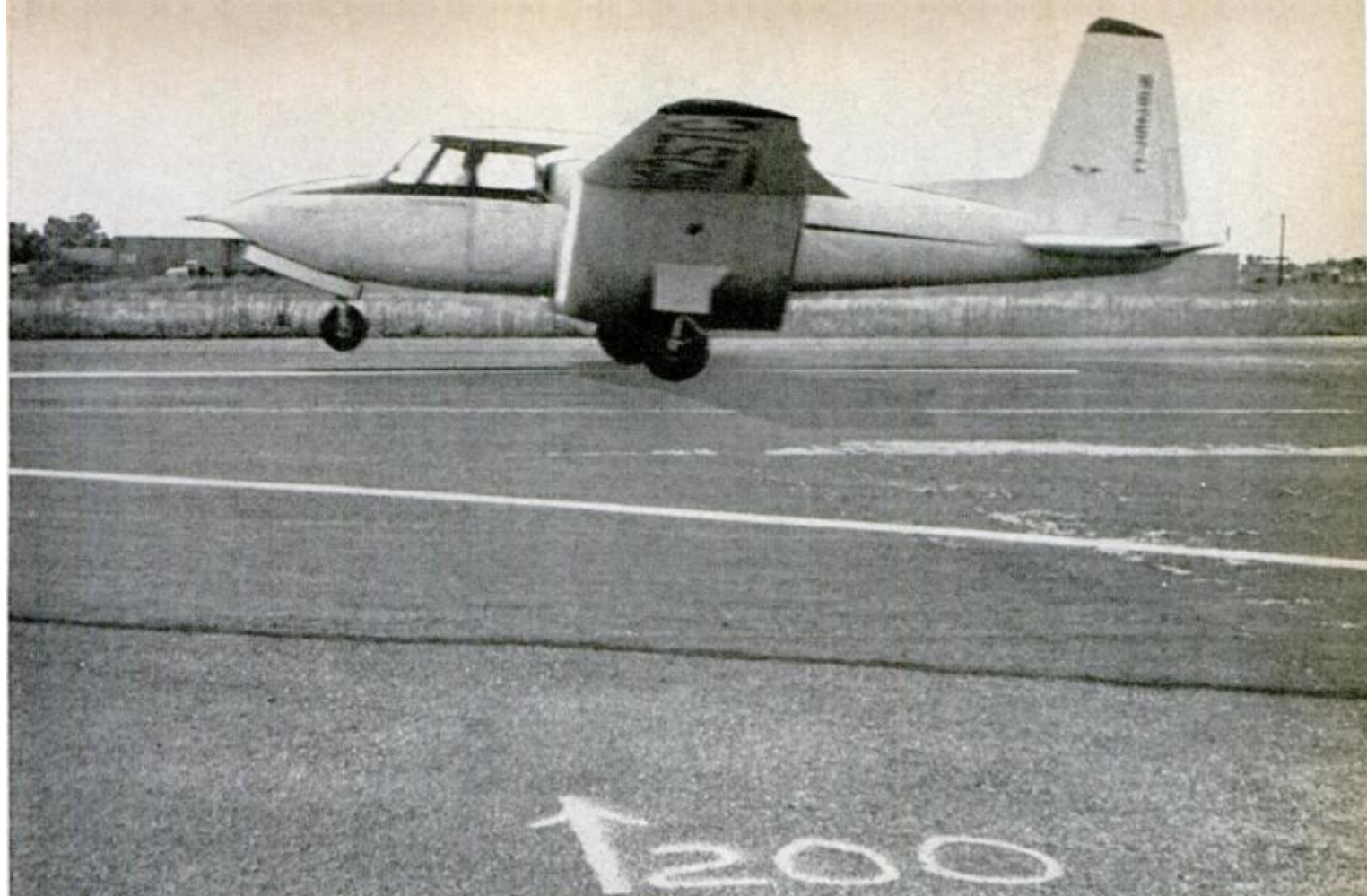
MAJOR ADVANTAGE of channel wing is its ability to take off and land in small areas. Here prototype's nose starts rolling at 200 feet, clears runway within 250 feet. Prop sucking air through channel doubles the lift
