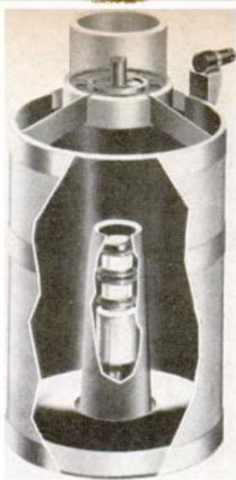
MODEL of the telescopes to be used in mapping project. The TV camera sensitive to ultraviolet light, called a Uvicon, juts up from bottom of instrument
