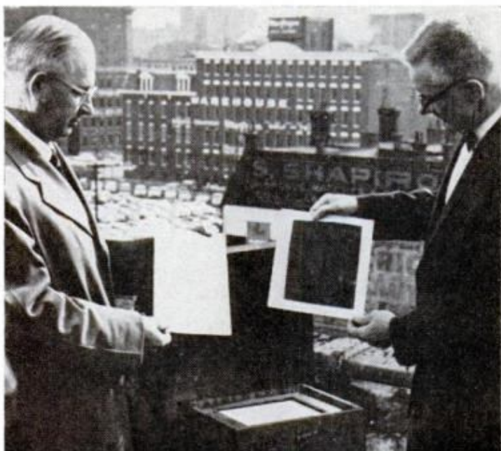
DIRTY PROOF of air pollution is the filter, below right, which was originally white like one at left, until it spent 24 hours in air sampling device (center)
