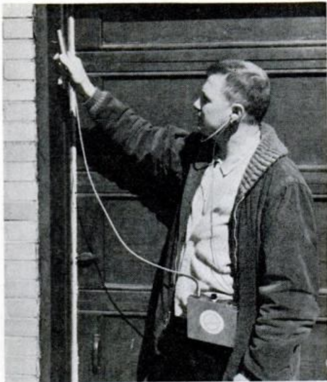
ELECTRONIC DETECTOR helps pinpoint location of nests by picking up sounds within the wood. Type shown is made by Sonitrol Corp., Anderson, Ind.
