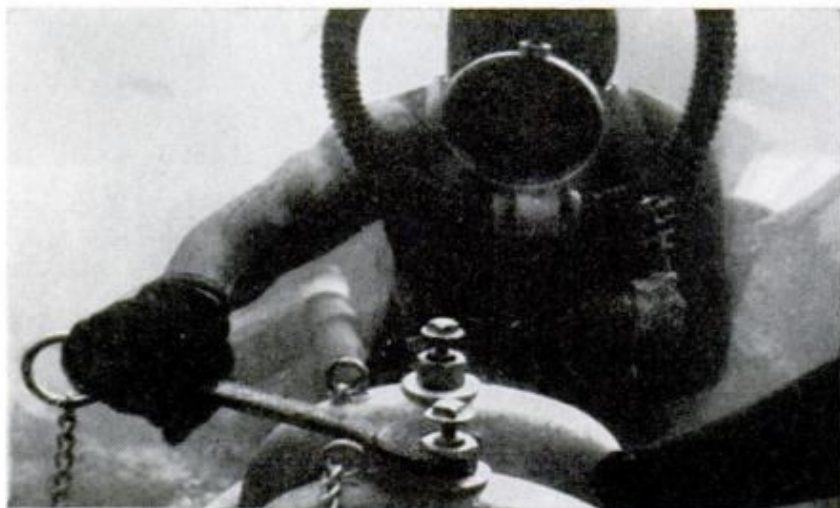
FISH ARE CAUGHT by net or hook and line, and are then placed in the decompression chamber. When the catch is complete, the divers close the tank, securely bolting down the tank's airtight cover plate
