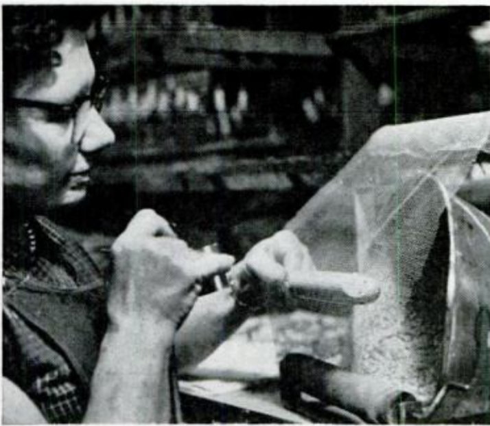
UNIQUE PRODUCTION METHODS are necessary in making lures. The fish-scale effect is created by hand-spraying each lure through a screen of metal mesh
