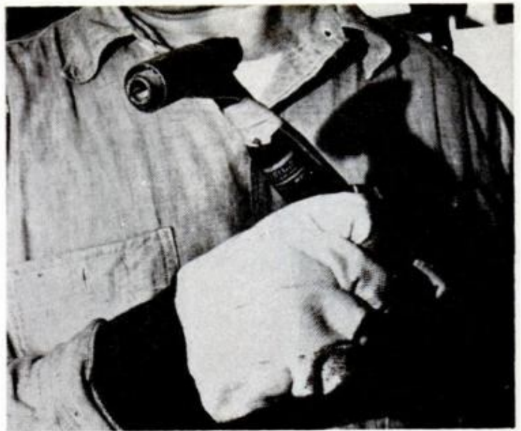
WELDER CAN WORK in the open with this torch. It has dual concentric shields that duct argon gas over the weld, shutting out the contaminating air
