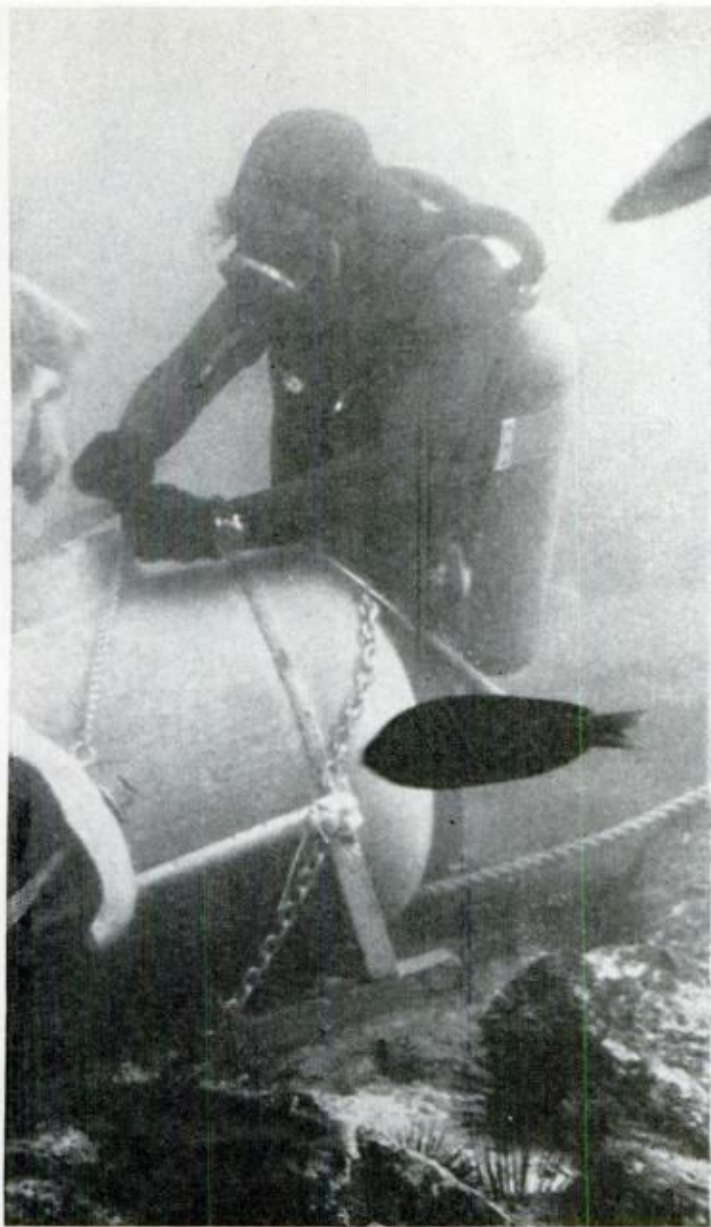
COLLECTED in plastic bags, fish specimens are transferred to the decompression chamber, which is then sealed to maintain the normal deep-sea pressure
