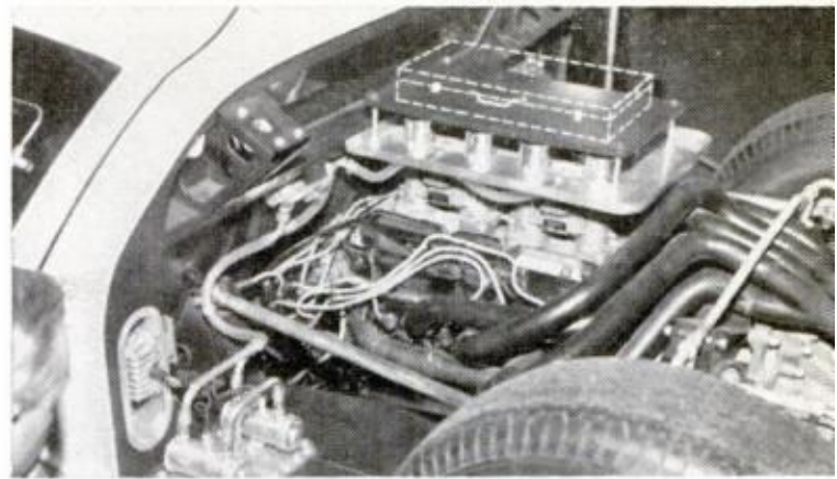
SINGLE, SMALL SUITCASE will rest on an asbestos shelf over the engine to comply with the requirement for "luggage space" in grand touring cars
