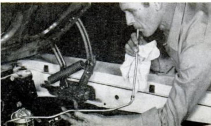
RARE IN MODERN CARS , but pump-to-carb line can clog with dirt. Disconnect the line and blow it out
