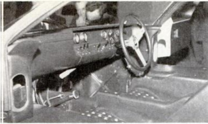
FUEL TANKS , with a 37-gallon capacity, are in the door sills. The brake handle operates horizontally. Air flows to the car's interior through body channels
