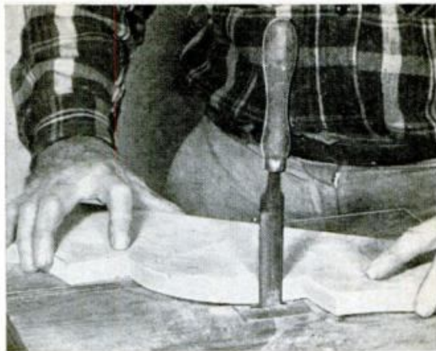
POWER FILING with plain hand files (you don't even have to remove the handle!) saves tedious handwork
