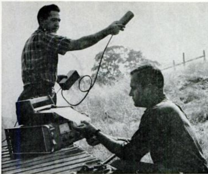
MAGNETIC FIELDS in subsurface rocks change and indicate changes in subsurface stress. Quakes may be predicted by measuring changes with magnetometer
