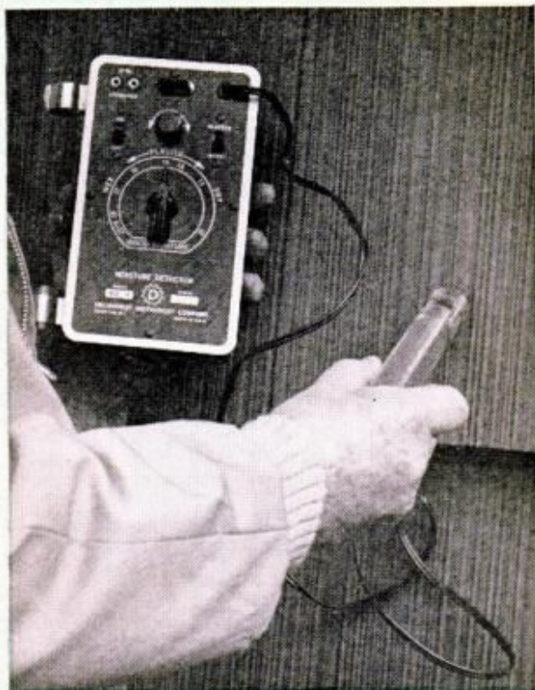
MOISTURE METER set to prescribed percentage tells beforehand if too much moisture is present
