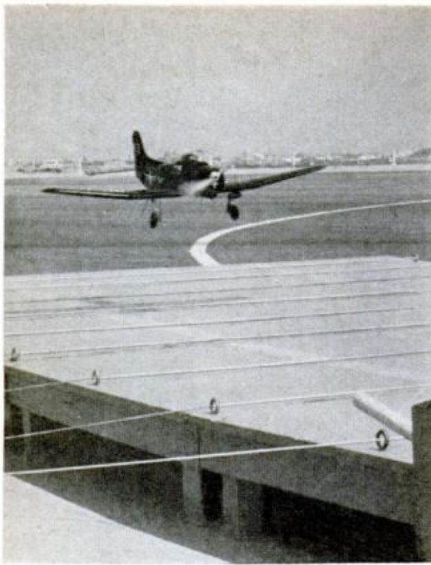
CARRIER MODEL , tailhook down, flies in for arrested landing, just as its big brothers do on an actual aircraft carrier. Arresting wires catch tailhook
