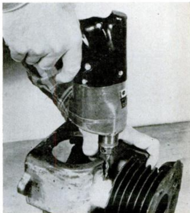
SECOND HOLE goes through lower wall of cylinder on flywheel side, to lubricate connecting rod bearing
