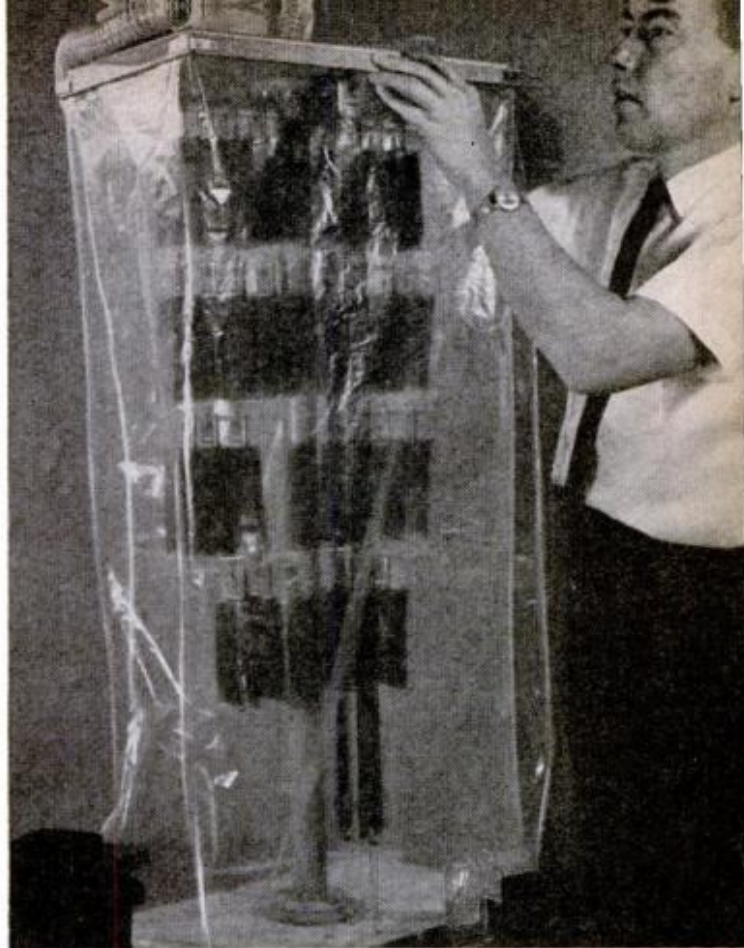
AFTER HANGING the film, the plastic cover is lifted into place and the upper frame is held with nail pins inserted in two holes drilled in long sides of top
