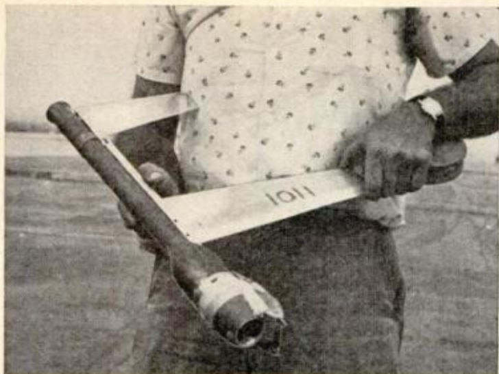
UNIQUE JET has only one wing and elevator. By eliminating wing, maker reduces drag and increases speed. This model got up to 160 m.p.h. in flight
