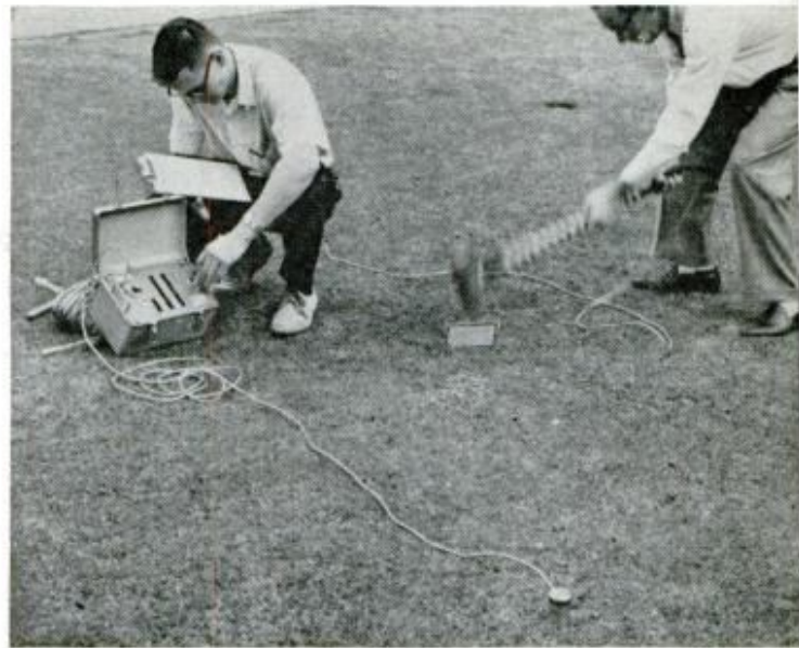
SHOCK WAVES in subsurface soils vary depending on materials. Speed can be measured with geophone which picks up shock waves generated by sledge
