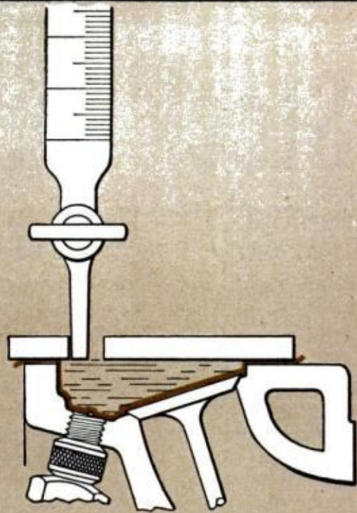
PLASTIC BAG follows every contour of combustion chamber. Water needed to fill from calibrated tube shows its capacity in cubic centimeters
