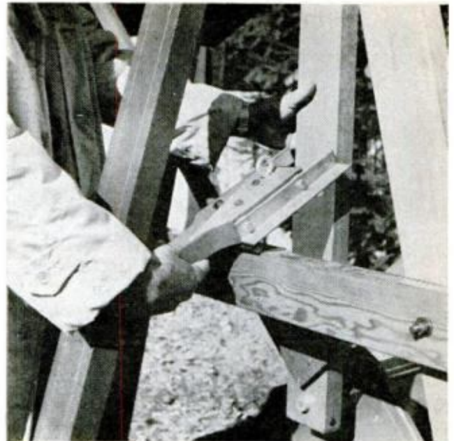
PIVOTED WHEEL LOCKS are provided as a safeguard against use when ferris wheel is unattended by adults
