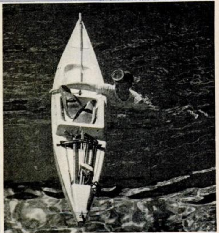
DESIGNED for easy handling in rough surf, Del Wren's diver's float has storage racks for spear guns, a fish well, and ample area for the diver to rest
