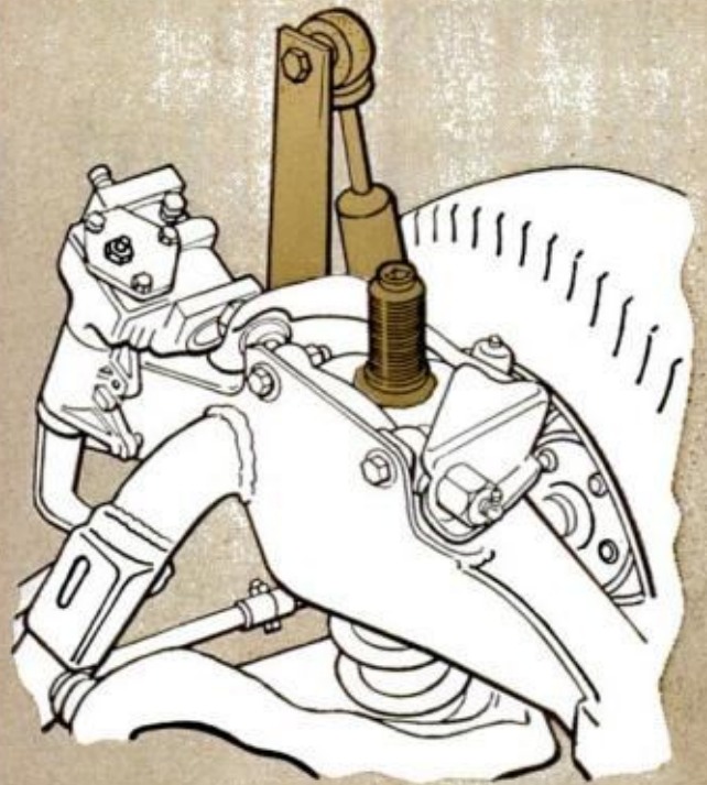
SCREW in front spring pocket bears on upper end of coil via a plate. Turning screw in or out increases or decreases spring rate, tunes chassis
