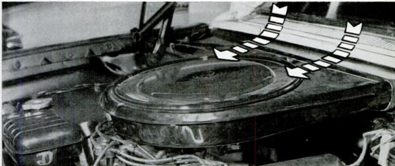
RAM AIR comes down through the ventilation slots but instead of cooling driver it is ducted through firewall into shroud around giant air cleaner. At 160 m.p.h. this air pressure will raise water in a gauge six inches
