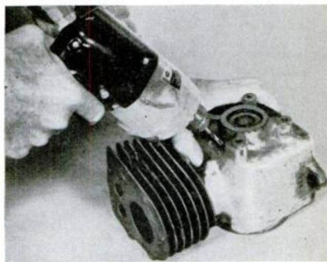
DRILL FIRST OIL HOLE at slight angle through to inner edge of crankshaft bearing opposite flywheel
