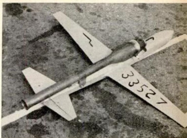
STANDARD JET has full wing and elevator. Jet engine is 21½ inches long and sells at $39.95. Fuselage is metal. Jet takes off without landing gear
