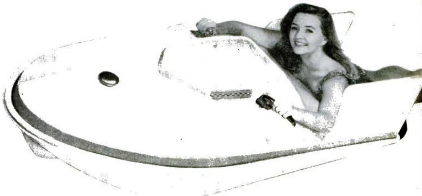
EQUIPPED with a special attachment for underwater observation, the Aqua Jet will haul two divers at speeds up to 25 m.p.h. Made of fiberglass and powered by an inboard engine, it is steered by movements of legs and body
