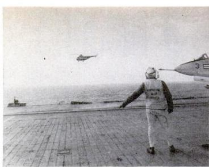
ARM DOWN means "go." Catapult operator (far left) will now lower right hand and push "go" button. Notice 'copter hovering alongside ship in background
