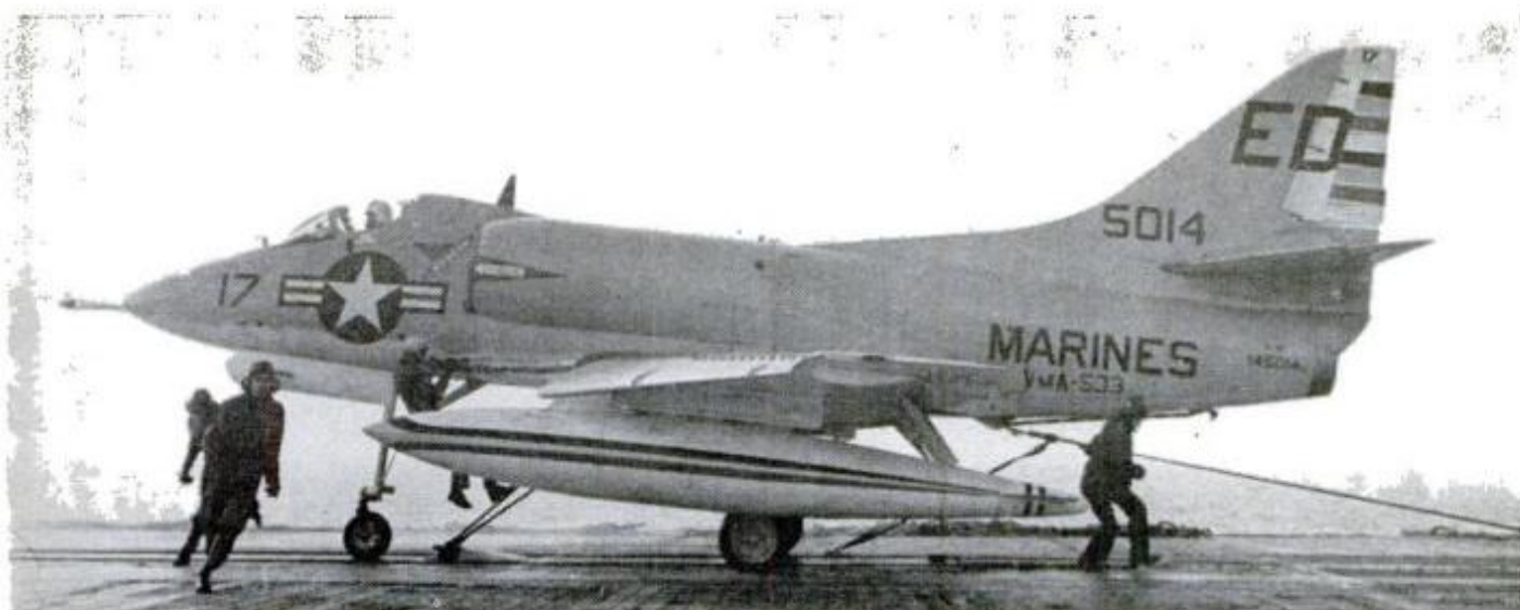
CREW SCRAMBLES from underneath plane just before it blasts off. Front cable attached to shuttle will pull plane down track after tension bar attached to the rear cable snaps. Note man bouncing on front cable to test the tension
