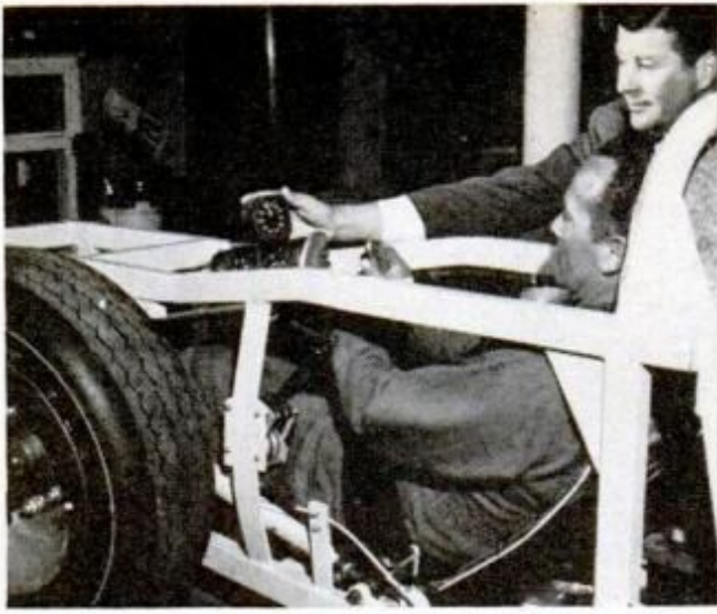
DURING CONSTRUCTION Arfons sits on Wingfoot's cockpit to check the dimensions as well as location of instruments. No details were overlooked
