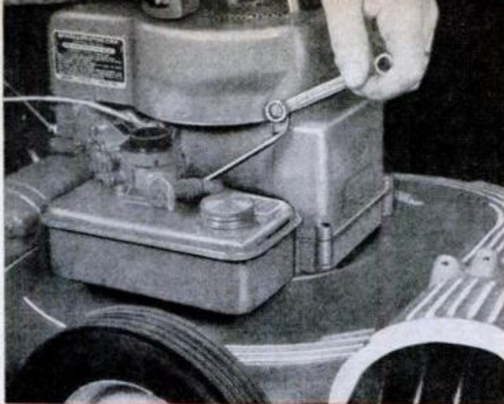
REMOVE BLOWER HOUSING to clean between fins. Most housings are held in place by only three bolts
