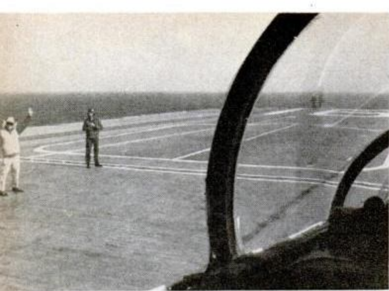
TWO FINGERS UP signals pilot to turn power on full. Author took this picture from back seat of jet just before being catapulted from carrier deck
