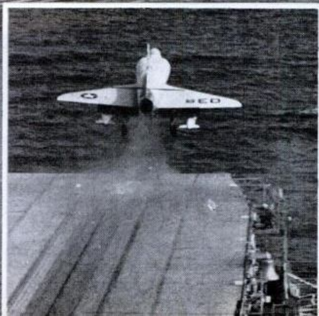
WHOOSH! Jet is literally flung into wind at better than 150 m.p.h. It's a bone-crushing sensation and plane actually slows down slightly after leaving deck
