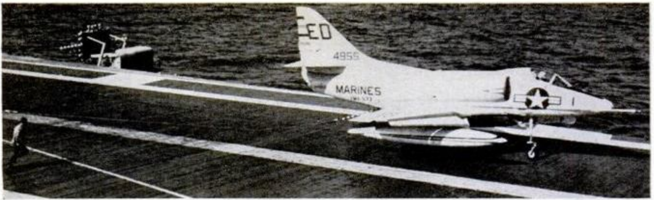
HOOKRUNNER (left), man with most dangerous job in Navy, dashes out to disengage tailhook from cable. If cable snapped before plane stopped, it could tear a leg off. Meatball mirror is shown from the rear at upper left
