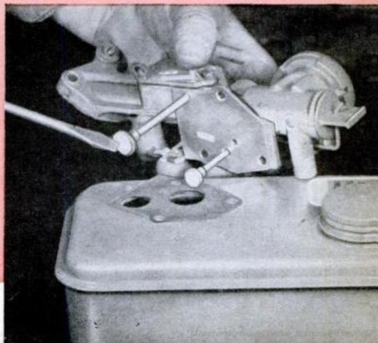
NO FUEL LINE is needed since gas is drawn directly from tank by these pipes, capped with fuel filters
