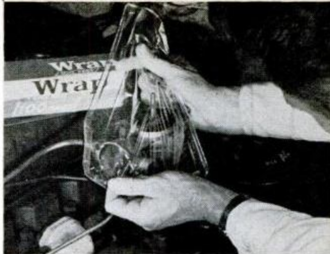
PLASTIC FOOD WRAP is best material to keep water from flooding carb during hosing operations. If water got into carb it would make car hard to start
