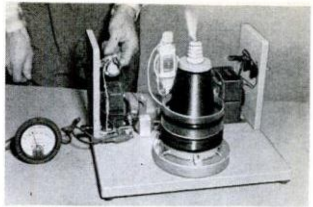
AFTER ASSEMBLY , read plate current by connecting D.C. milliammeter between center tap of filament transformer and ground. Adjust rheostat to 150 ma. maximum for any combination of capacitors and taps
