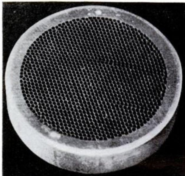
PRECISION WELDING , as in delicate copper grids, is accomplished with such finesse that the process may have many uses in space projects, such as in missiles
