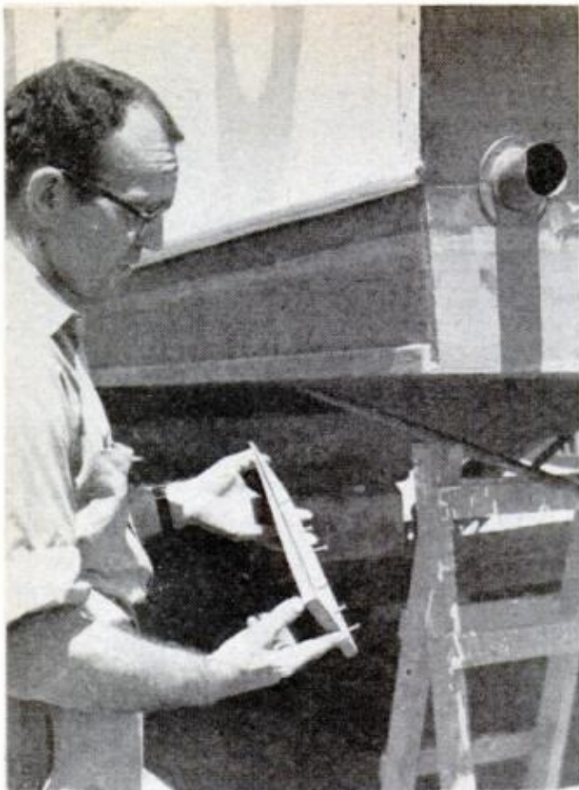
WEDGE INSTALLATION on a wood hull, above, uses screws in addition to epoxy. If covered with fiberglass, fairing strip may be omitted. In drawings below, both wedge and fiberglass have been exaggerated
