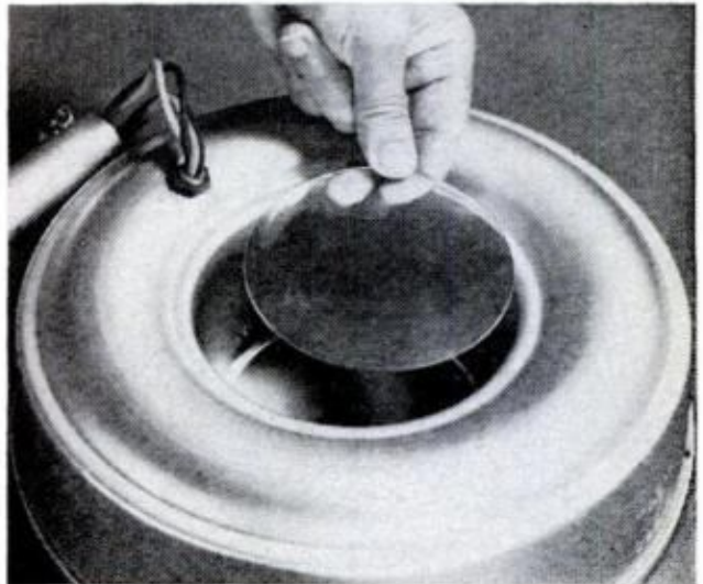
MAGNIFYING LENS is placed on rim of mold opening. If lens is a bit small, bend rim outward with pliers, then secure lens in place with the three clips
