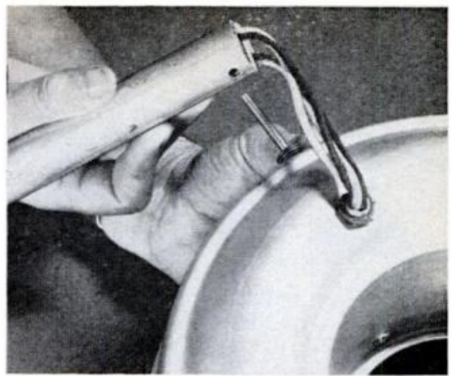
STOVE BOLT , 1½ in. long, is passed through hole in mold, three washers are needed, then bolt is inserted in hole in tubing and secured with wing nut
