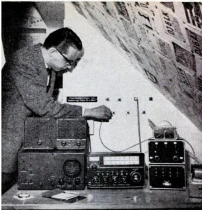
BY PLUGGING IN a wire, one of the nine remote-controlled antennas is selected. Each one is set for maximum reception on a particular radio frequency
