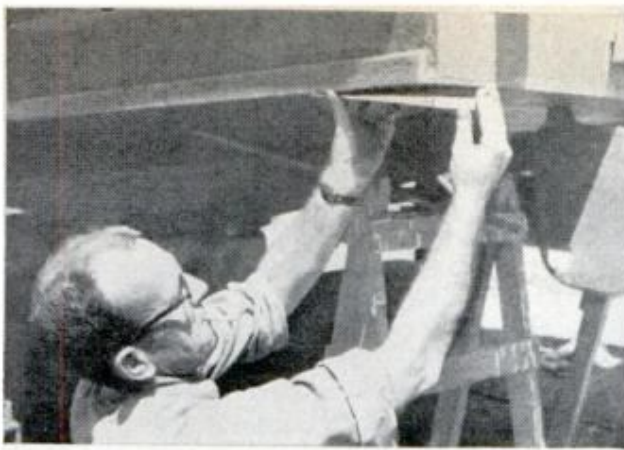
OUTER PIECES should be faired to match the angle of the sides and transom to avoid creating turbulence
