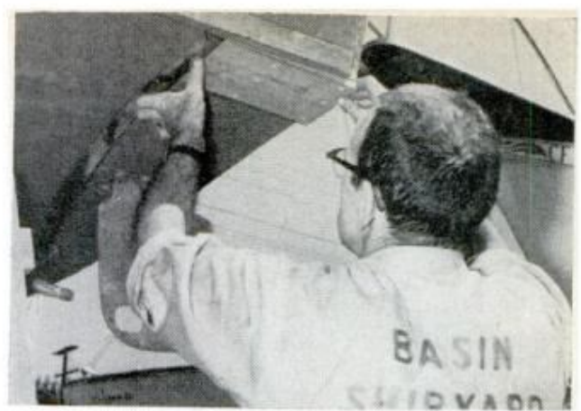
METAL FAIRING STRIP mounted along leading edge of wedge would be omitted if plan to add fiberglass
