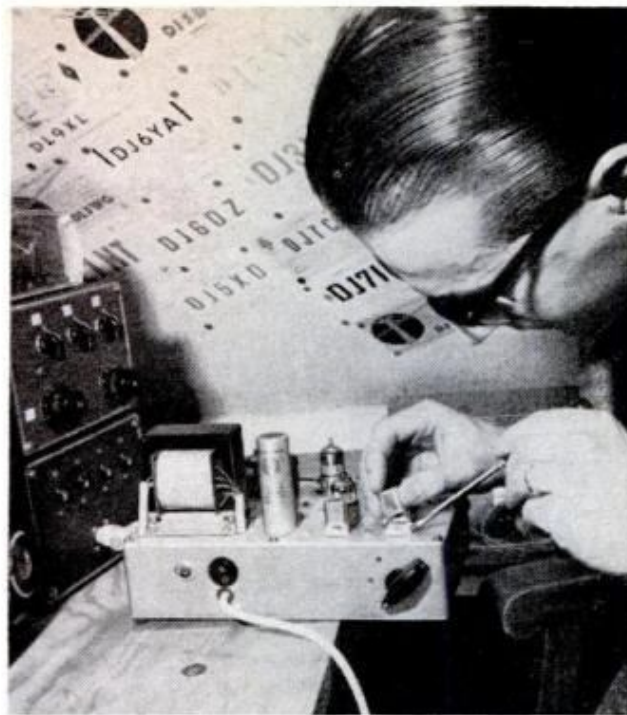
PLUGGING IN a finely tuned crystal—the heart of the system—Oslender can grab hold of a weak satellite signal and hang onto it without any drifting
