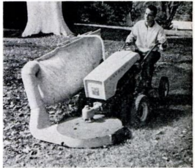
LEAF-AWAY cleans 30" swath, mulches and bags leaves and lawn litter . . . one of eight lawn-care tools.
