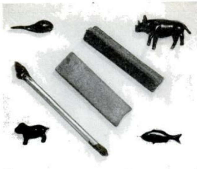
FIRST TOOLS were modest. They included metal rod with sapphire and ruby tips, pocket whetstone and small sand cloth. First carvings are also shown
