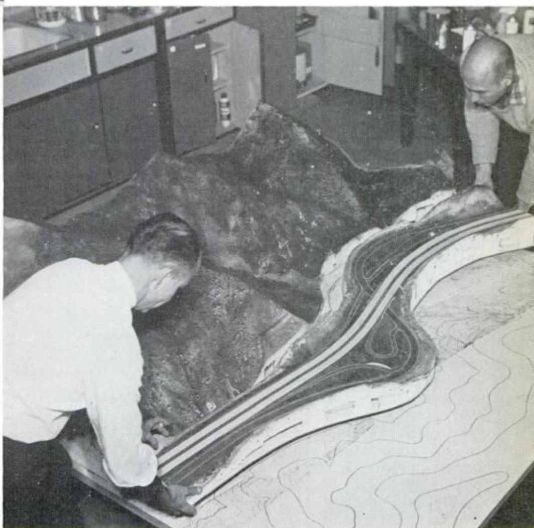
CUT TO THE CONTOURS of a topographical map, layers of plastic foam are built up, then sanded off to reproduce California's hills in detail
