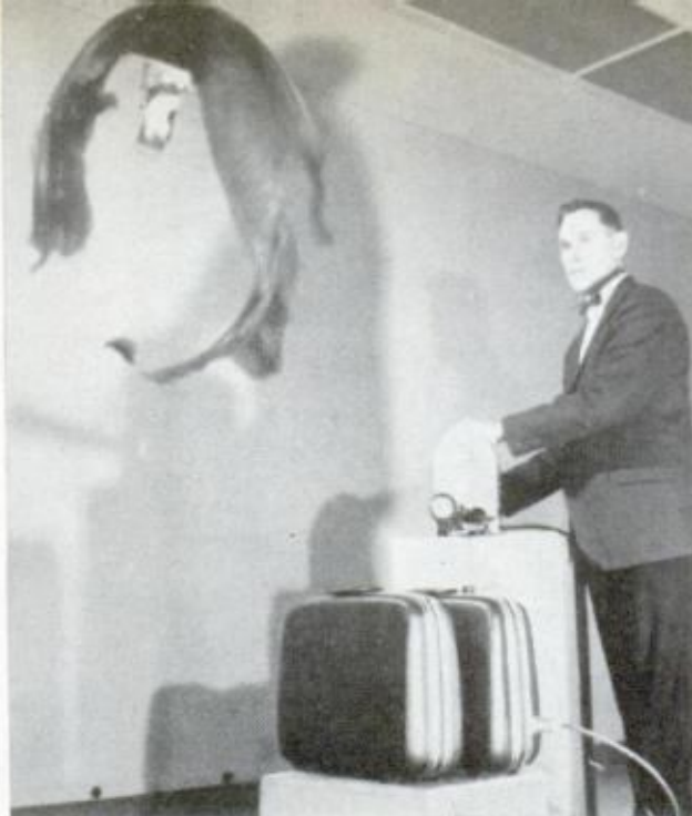
BURNING THROUGH a sheet of stainless steel, the beam of a laser developed by Raytheon Co. bursts a balloon 10 feet beyond. Dot of light in balloon is laser light, captured on film in its duration of 1/2000 th of a second
