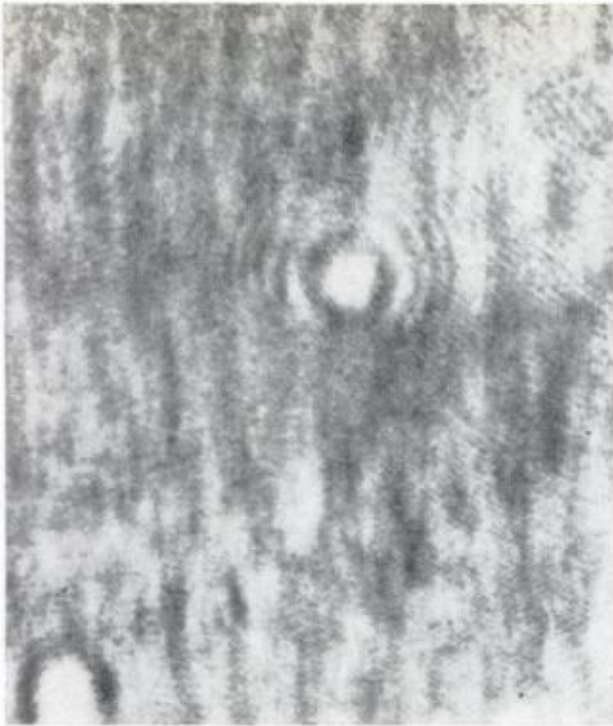
LENSELESS PHOTOGRAPHY: Helium-neon laser light beamed at an original snapshot of little girl resulted in blurred negative, left. Laser beam trained on the negative in a lensless projector produced the clear image at right
