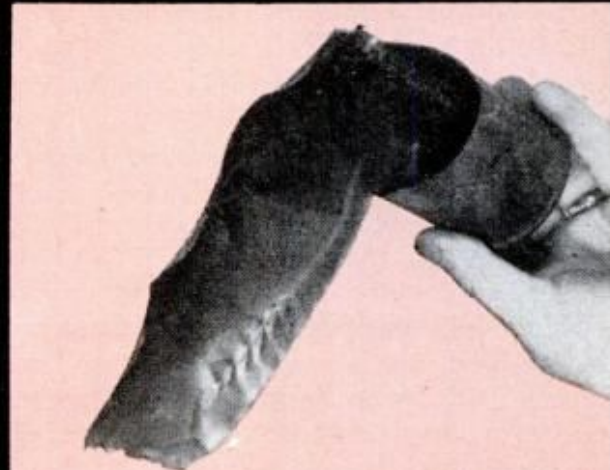
EXPLOSIVE expansion forces unpeeled this can to produce sharp-edged metal projections
