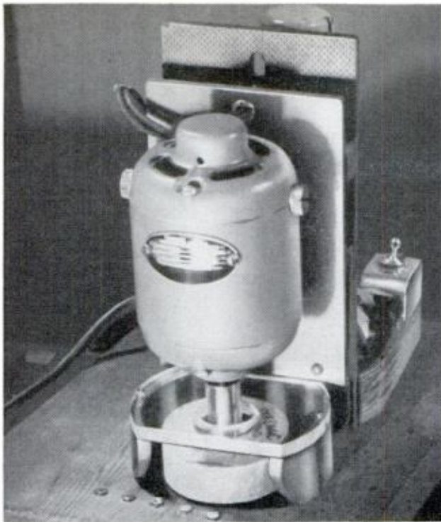
DRESSING BOLTS to uniform length is easy with tilt panel adjusted forward. Bolts are inserted through holes in a board, their heads underneath
