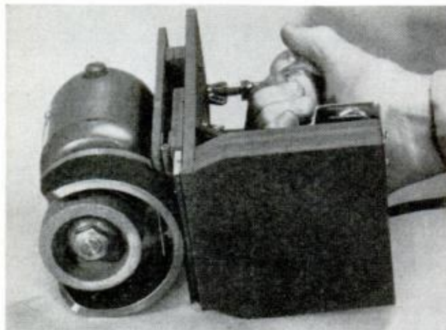
WORM'S-EYE VIEW of grinder shows how No. 6 cup wheel fits within guard. Its face is higher than the base edge of the guard, which is flush with hardboard
