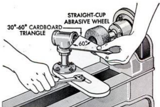
TRIANGULAR TEMPLATE speeds adjustment of jig for grinding 30-degree bevel as in title photo at left
