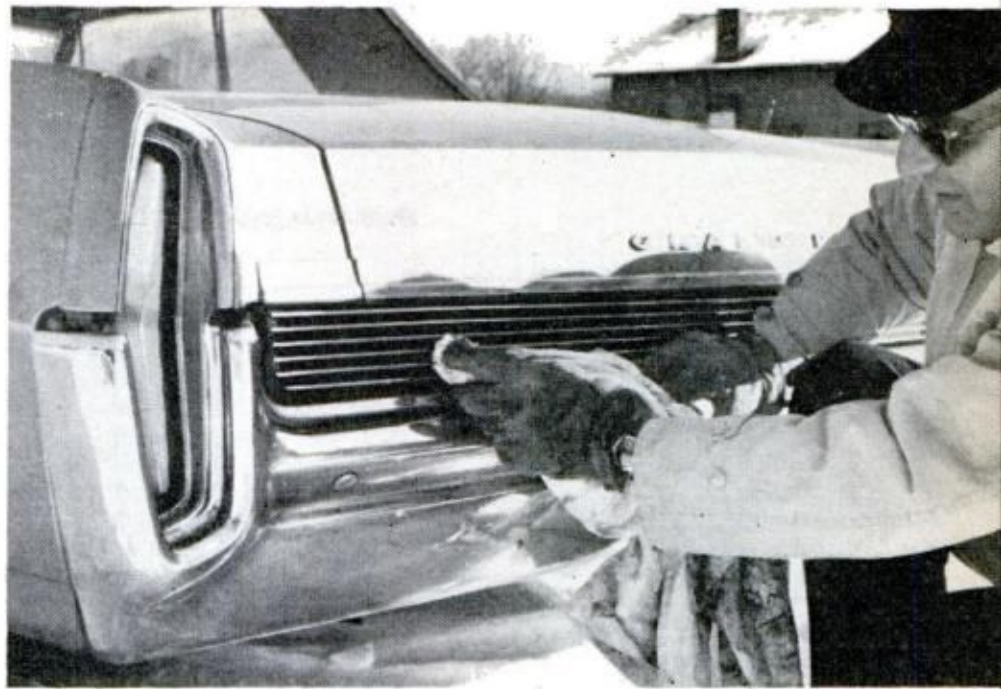
TAILLIGHTS ARE HIDDEN behind closely spaced chrome bars—a slick styling touch which makes lenses hard to clean, however. System, limited to Grand Prix models, has huge back-up lamps protected by massive bumper
