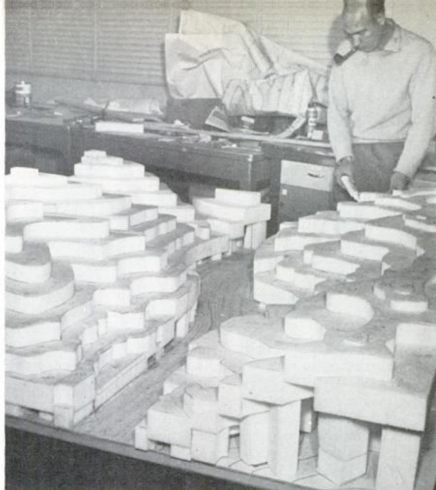
CUT TO THE CONTOURS of a topographical map, layers of plastic foam are built up, then sanded off to reproduce California's hills in detail
