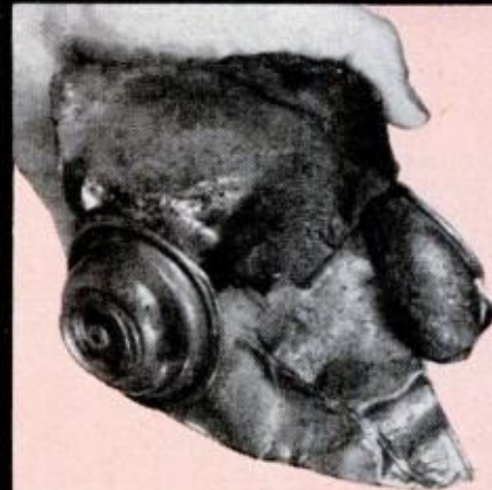
BOMB BURST pressures built up inside by heat, tore this can into blossom of knife-like petals
