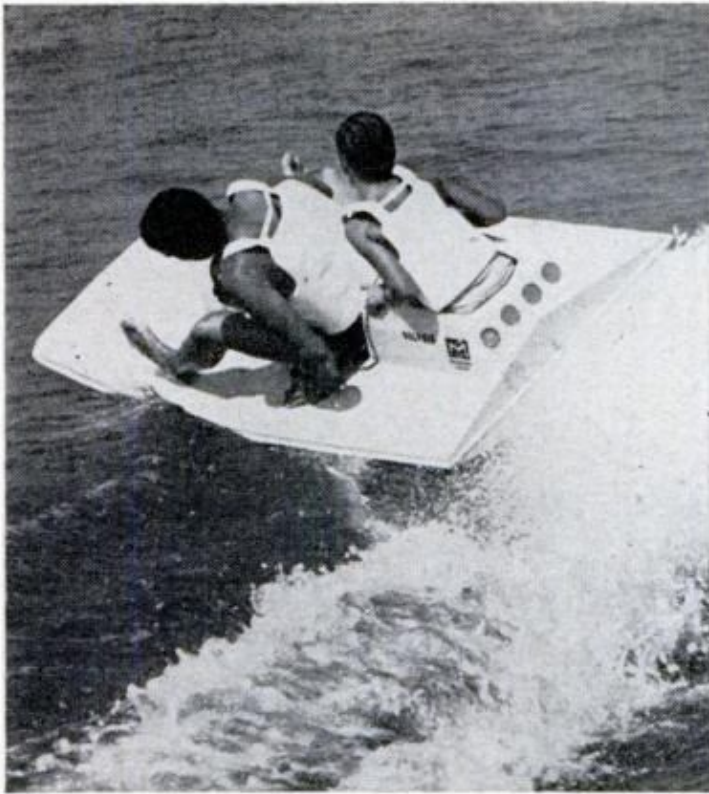
TWO-SEATER KART designed by Dolphin mounts passenger on an elevated piggyback seat behind driver. It's powered by a front-mounted McCulloch inboard
