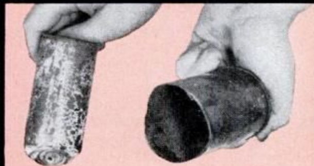
BLOWN OUT bottoms of heated aerosol containers show how they can become rockets
