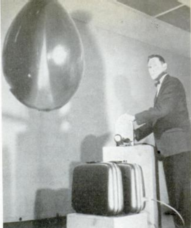
BURNING THROUGH a sheet of stainless steel, the beam of a laser developed by Raytheon Co. bursts a balloon 10 feet beyond. Dot of light in balloon is laser light, captured on film in its duration of 1/2000 th of a second
