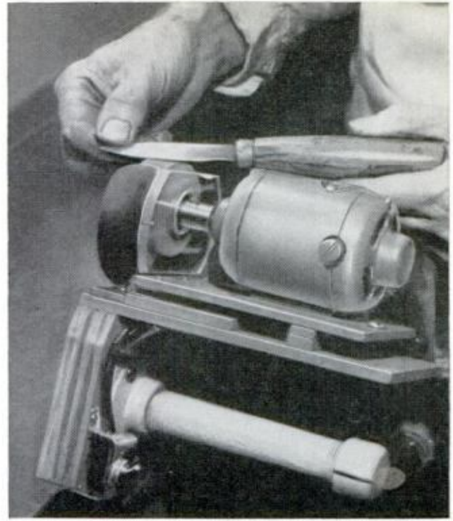
LAI D ON ITS SIDE with a corner of the base clamped in a vise, unit becomes a horizontal tool grinder which puts a quick sharp edge on a knife or chisel
