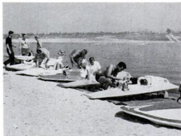
LAST-MINUTE TUNING continues right up to race time. Note the high-mounted outboard on HK-43, second from left. It's McCulloch's Hydro-Mac racing model
