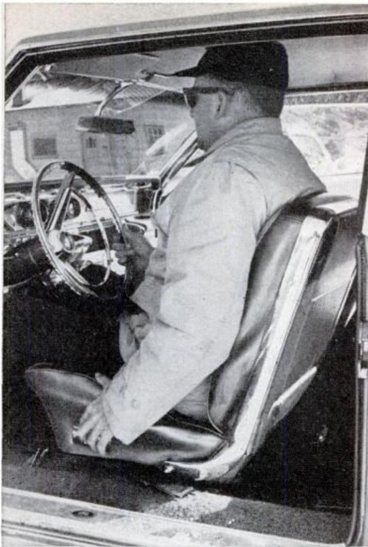
A HAPPY FEATURE OF THE POWER SEAT on the test Pontiac: Besides gliding fore and aft to adjust for leg length, it tilts around a pivot point at the rear for an almost limitless range between sitting upright and near-reclining
