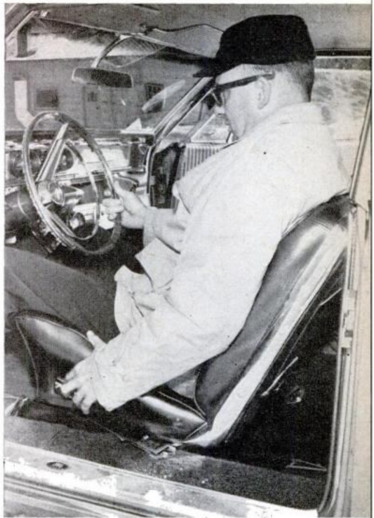
A HAPPY FEATURE OF THE POWER SEAT on the test Pontiac: Besides gliding fore and aft to adjust for leg length, it tilts around a pivot point at the rear for an almost limitless range between sitting upright and near-reclining
