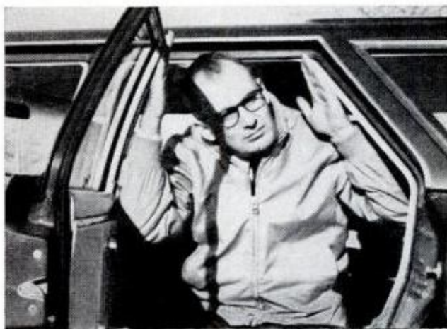
RAKISH C-PILLAR ANGLE and curved door reduce entry-exit area. Some cases of poor door fit, with rattles and squeaks, sparked complaints by owners
