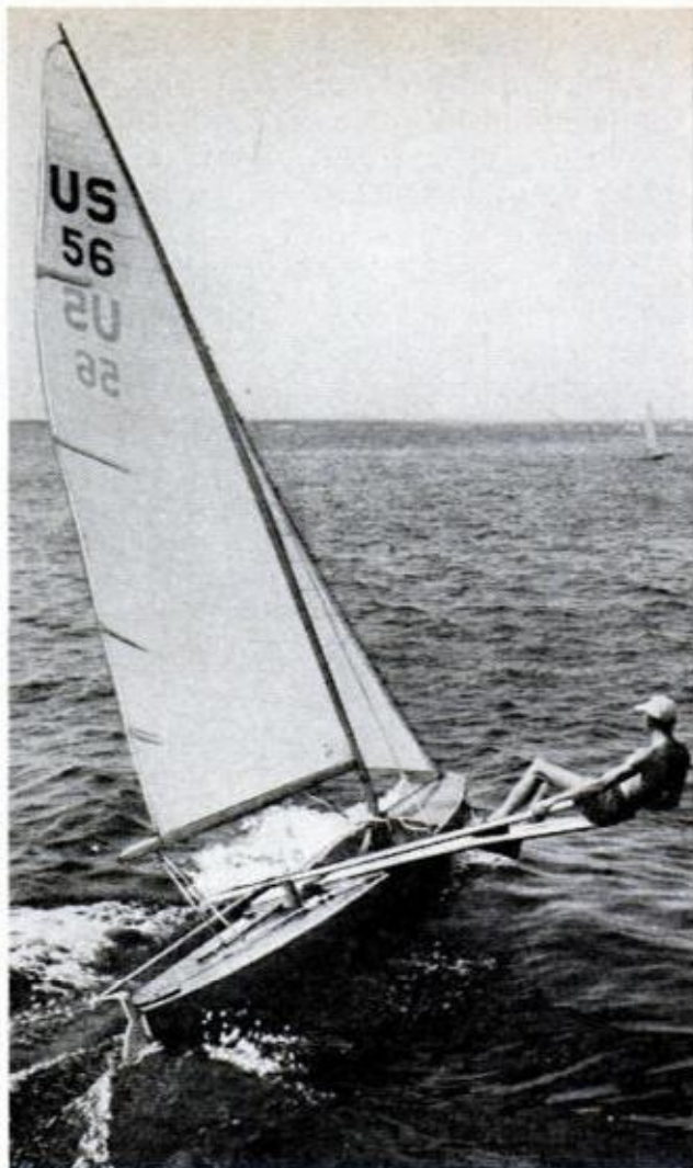
HIKING BOARD , still used in the International Decked Sailing Canoe class, has generally been replaced by trapeze. Note the "hiking stick" tiller extension
