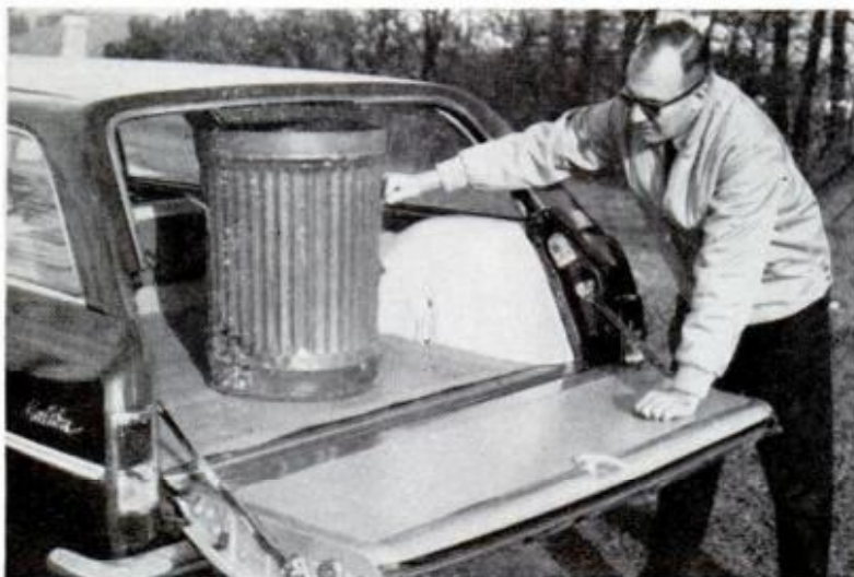
THE STATION WAGON'S REAR OPENING takes loads to 28½ inches high. The tailgate is less than 20½ inches from the ground. About 10 percent of the owners surveyed chose station wagon
