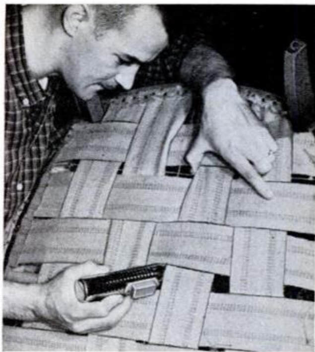
LIGHT UP spring assembly with flashlight to examine it. If OK, start applying the steel webbing
