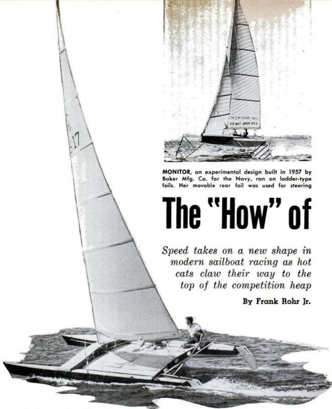
SEALION , a 25-ft. featherweight, weighs only 632 lbs. Her slim fibreglassed hulls are planked with strips of polyurethane foam
