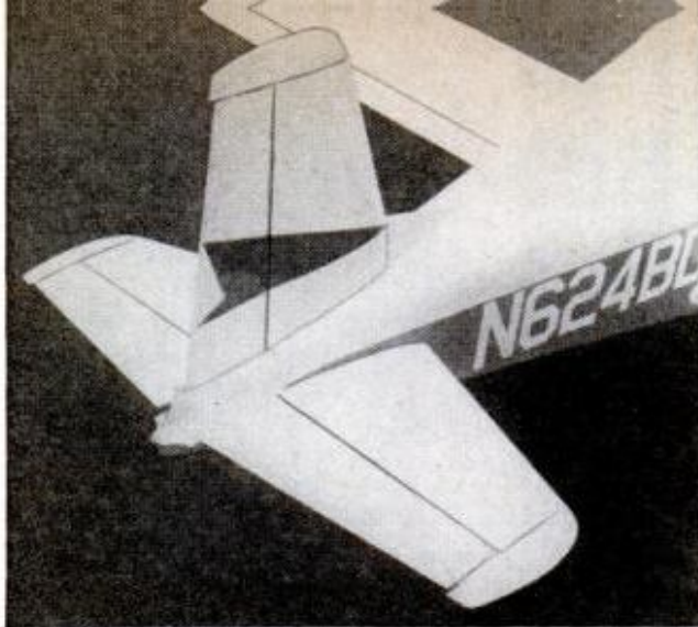
INTERCHANGEABLE PARTS are most unique feature of BD-1. Note symmetry of tail assembly; fins, tips and control surfaces can be used in any position
