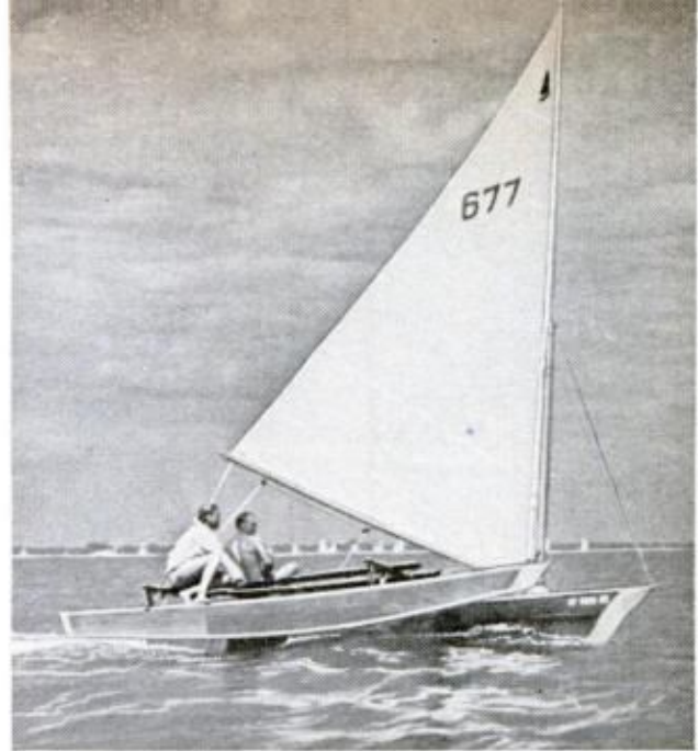
MALIBU OUTRIGGER , an up-to-date version of the old Polynesian sailing craft, features two hulls of different sizes with mast stepped in larger one
