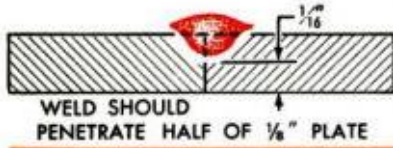
GOOD BUTT WELD with tight fit-up. Underside of bad gap-fit-up weld (below) shows burn-through gobs
