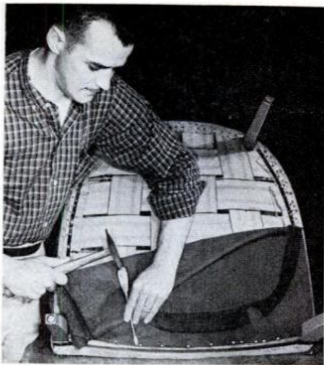
SET CHAIR upside down on table or bench and remove dust cover. This can be reused if undamaged
