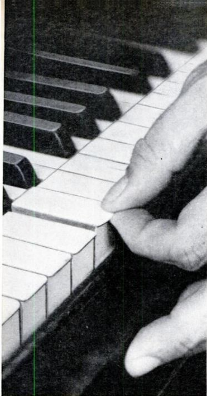
TESTING HAMMERS for "lateral motion" which will cause poor action and a distorted tone, move hammers forward and work them gently from side to side
