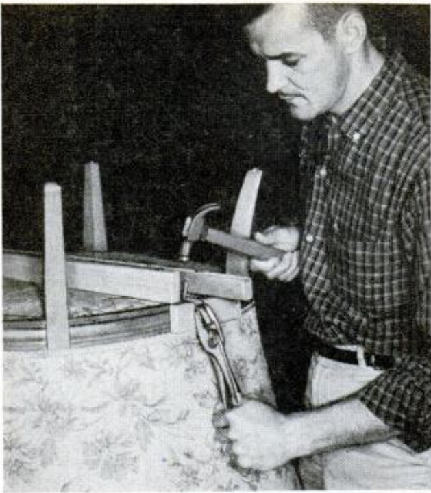
PLIERS or webbing stretcher pulls webbing taut at rear rail after nailing webbing to opposite rail
