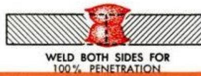
GOOD BUTT WELD with tight fit-up. Underside of bad gap-fit-up weld (below) shows burn-through gobs
