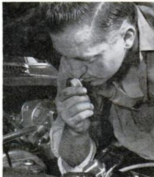
3. WHILE DISCONNECTED , manifold hose can clue you to internal leaks in power-assist unit. If hose has vacuum check valve at end (as in Fig. 1) remove it and twirl screwdriver inside to see if hose is coated with brake fluid. Valve itself can be cause of poor vacuum: check it by blowing through both sides as at right
