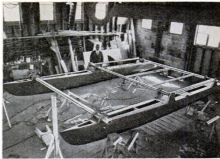
LINKED BY THREE transverse aluminum tubes, Beverly's twin 25-ft. fiberglass hulls are mounted far enough apart to give the boat a whopping 12-ft. 6-in. beam
