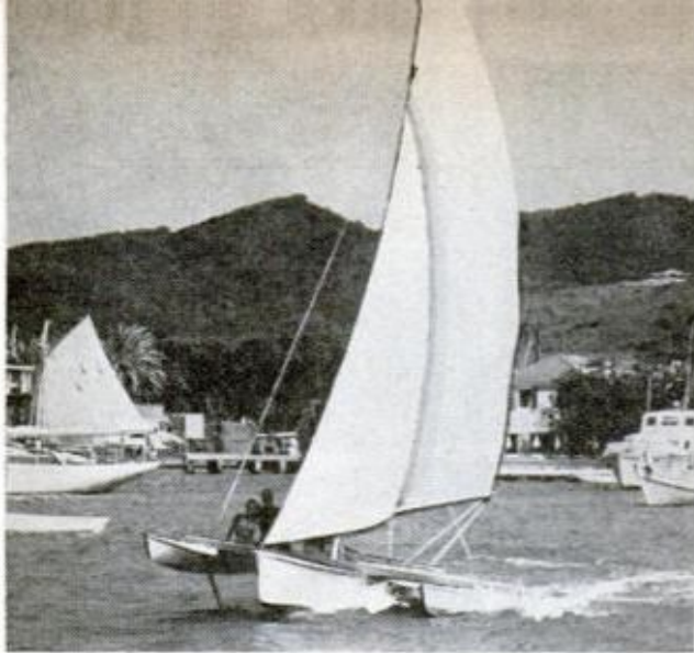
24-FT. TRIMARAN has stabilizing foils on the outrigger hulls, tops 20 knots with 275-sq.-ft. of sail. It's owned by Dick Newick of the U.S. Virgin Islands
