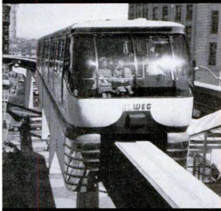
SAFEGE suspended-type monorail (below, left-hand page) is AMF's high-speed system; box rail is 6 by 6-foot hollow steel or concrete beam. Alweg (above) has its supported system in Seattle; tires run on a 3 by 5-foot concrete beam.
