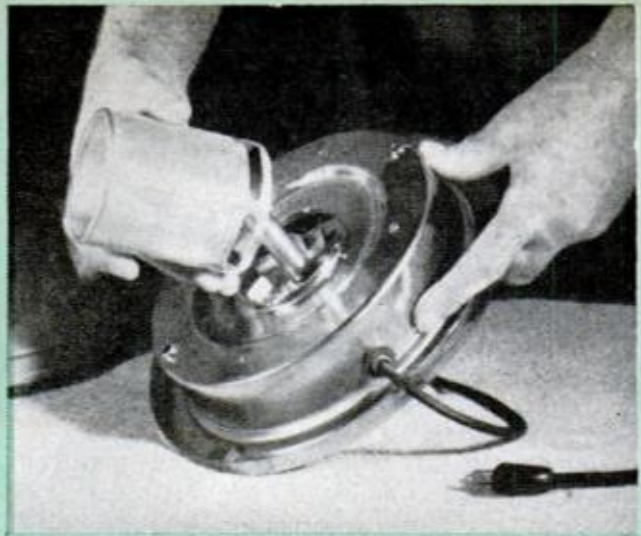
MAINTENANCE involves removal of the perforated screen for cleaning. Screen serves as filter to protect unit from foreign matter present in water
