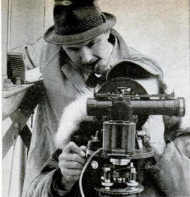
SURVEYOR'S THEODOLITE is set at predetermined angle and technician with mike tells pilot which way to fly to keep plane lined up in its crosshairs
