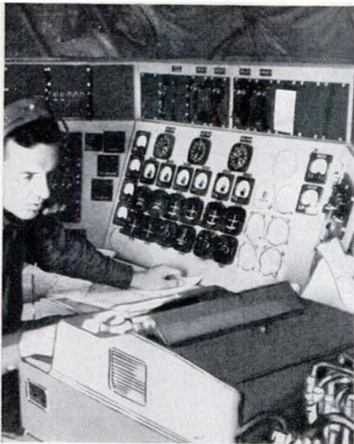
RECORDING EQUIPMENT (foreground) keeps record of inspection flight made by author. Technician mans panel which receives signals from ground stations
