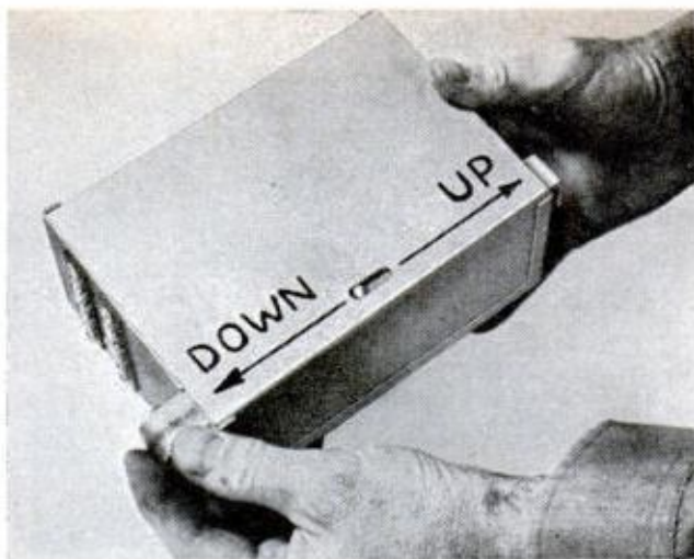
CONTROL BOX is modified Minibox. Ordinary toggle switch reverses motor connections, is flicked by sliding bar with hole to take bat handle. Switch is mounted on ledge as shown at left and in alteration sketch, next page
