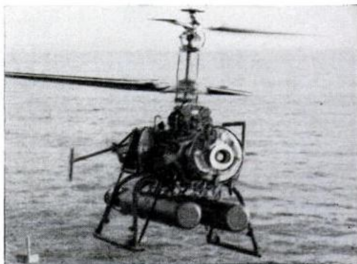
NEWEST ADDITION to ASW team is DASH, drone anti-submarine helicopter. Stationed on destroyers, it can be sent winging to undersea targets by carrier CIC
