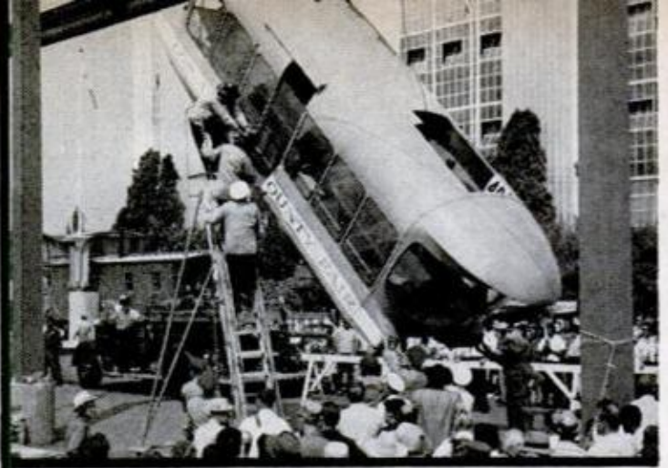
IT CAN HAPPEN—as it did at Los Angeles County Fair when a bolt snapped. However, suspension system isn't type used on fast mass-transit train
