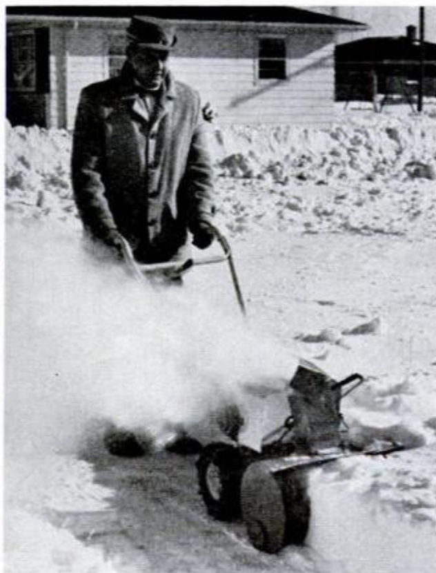
SNOW REMOVAL is easy with the right size blower working at perfect efficiency. With chute at the proper angle, snow is blown across cleared area
