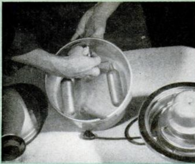
ATOMIZING HUMIDIFIER has three basic parts—from left to right: cover, float pan, and motor. Before installation, see float assembly is properly adjusted
