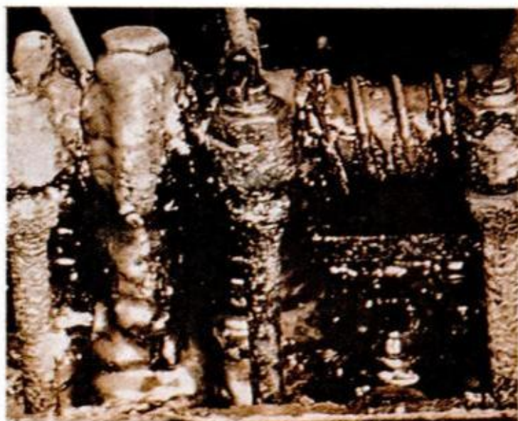
ANOTHER MS OIL went through the same test sequence as the engine at left but a look at the sludge generated told engineers the oil was not qualified MS
