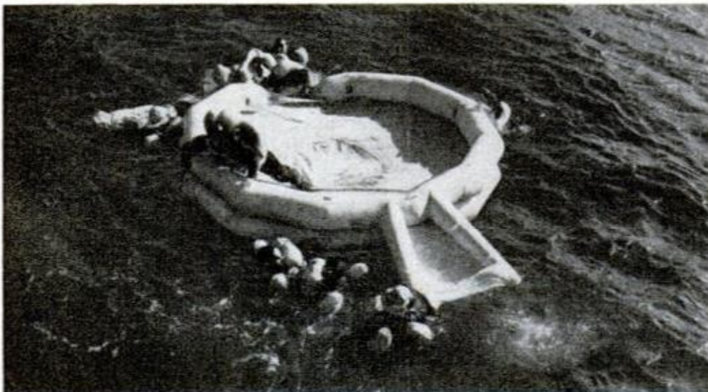
20-MAN RAFT crew struggles to get on board. Boarding stations project from opposite sides of raft. Survival kit and canopy are in center of raft. Double rim, inflated simultaneously, can be protected from double blowout by equalizer clamp
