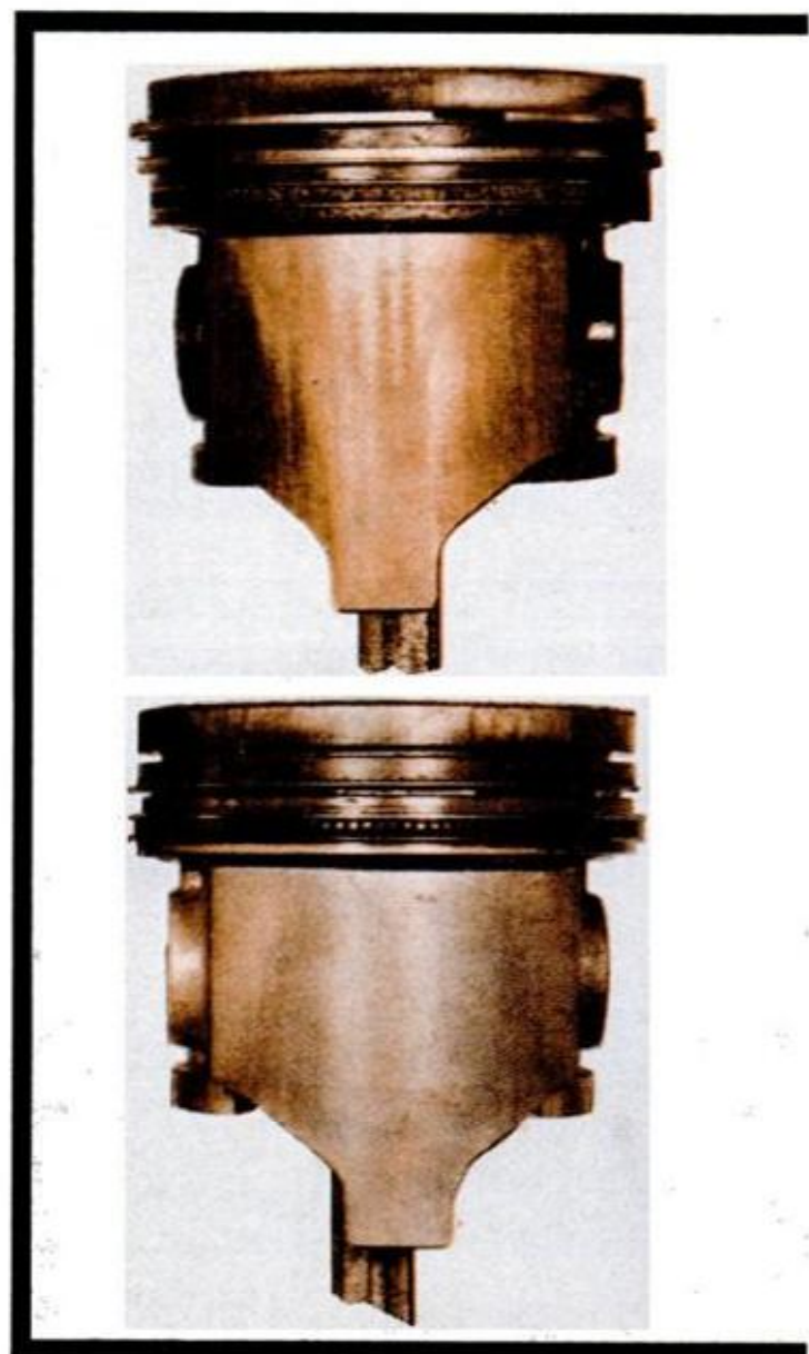
PISTON VARNISH on the top piston shown below was result of running sequence test with inadequate MS
