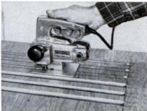
AIR SLOTS in top of cover can be cut on table saw with ganged blades—or by running saber saw between \frac{1}{2} -in. holes, above
