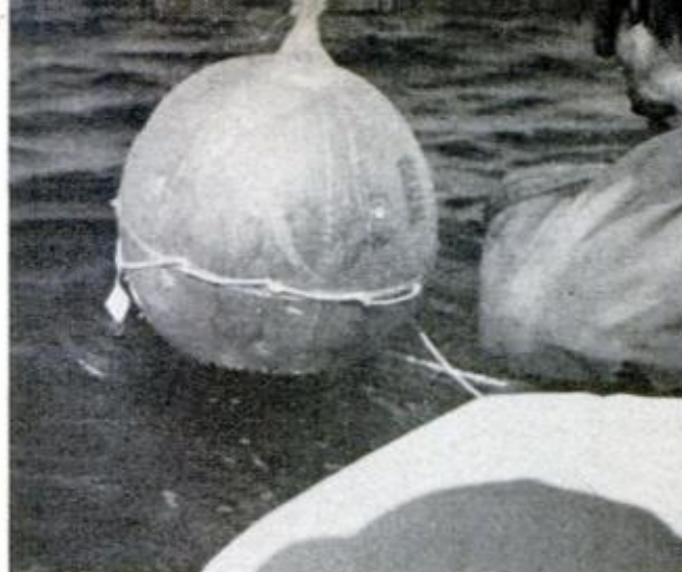
SOLAR STILL distills sea water. Sea water is poured in top and it filters through to bottom as drinking water. Student (right) was relieving his nausea
