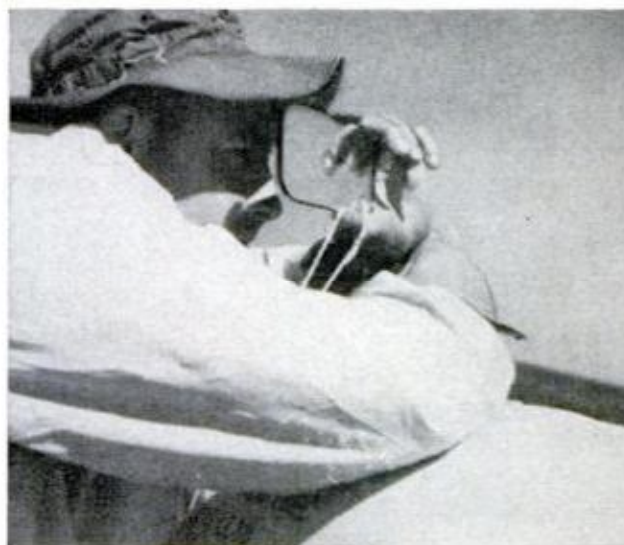
SIGNAL MIRROR is tested by student aboard 20-man raft. Sun's reflection can be aimed through center hole, and messages directed where you want them
