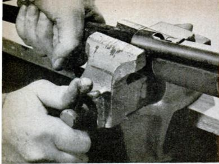
TINY CRACKS IN THE BARREL of the Krag are not easily detected. Coat barrel with oil and wipe dry. Squeeze barrel in vise; emerging oil will locate cracks
