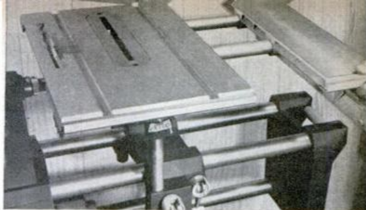
BEFORE THE MARK VII you could not attach the table extension directly to the saw table. Now you get 24 in. rip cut on main table with blade in edge slot
