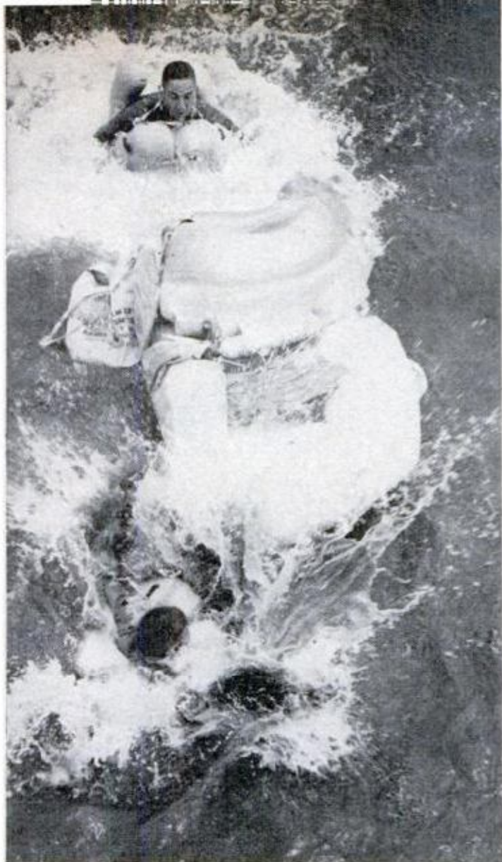
DURING INFLATION rafts look like this as they unfold. Inflation cord is pulled, then raft is thrown overboard and survivors jump in after it immediately
