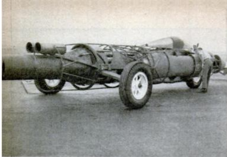
J-47 ENGINE mounted on test chassis of the Spirit of America . It's rated at 5200 pounds static thrust, which can be increased to 5900 pounds with water injection, and 7600 pounds with an afterburner
