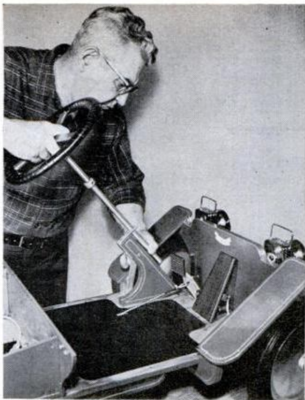
STEERING COLUMN is held in position by wooden support (plywood) and metal brace to frame. Metal angle screwed to top of support serves as a bearing
