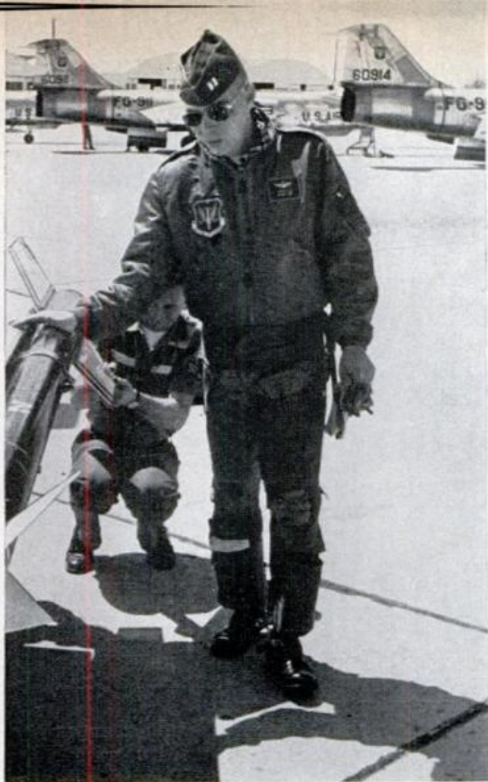
SIDEWINDER MISSILE is examined by Tofferi during preflight inspection. Red, transparent nose on missile covers heat-seeking device which homes in on engine exhaust of other aircraft in air-to-air combat missions
