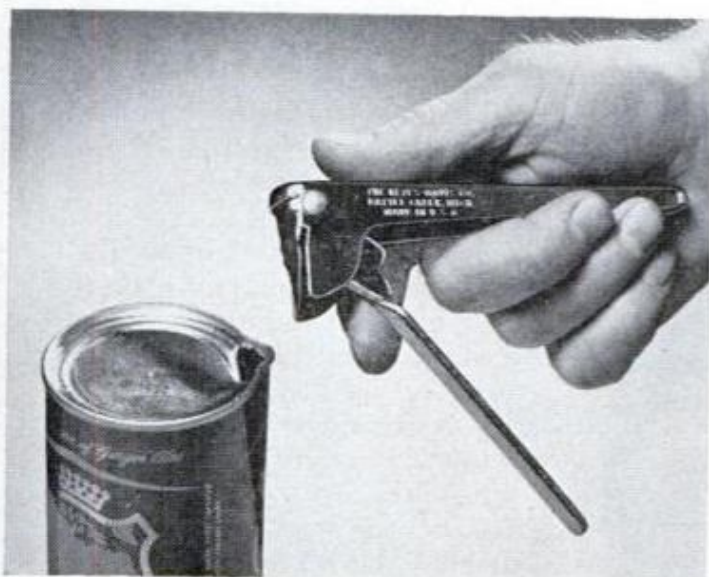
CAN OPENER makes a pouring spout as it opens any size can. Hold chrome-plated opener in hand, push down on knife button, squeeze lever to form spout. Can becomes dripless pitcher. By Keyes-Davis Co., Battle Creek, Mich.
