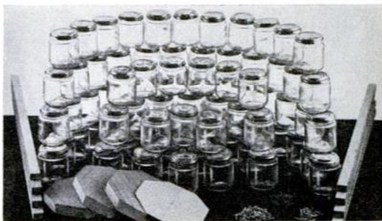
EASILY OBTAINED odds-and-ends, including 80 baby-food jars, are all you need to make a convenient small-parts storage rack
