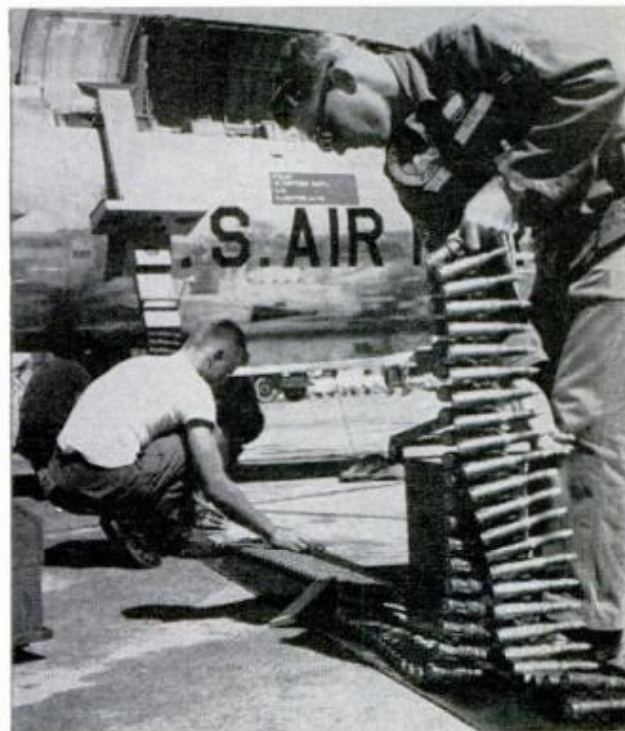
GATLING GUN , as pilots call the six-barrel cannon, is loaded with 20-mm. shells by armament crew. Gun's six barrels rotate, giving it rate of fire of 6000 rounds per minute. Each shell is explosive
