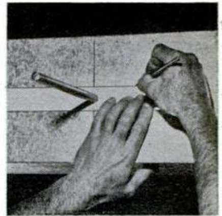
5. SLIDE template over shaft and carefully scribe around outline
