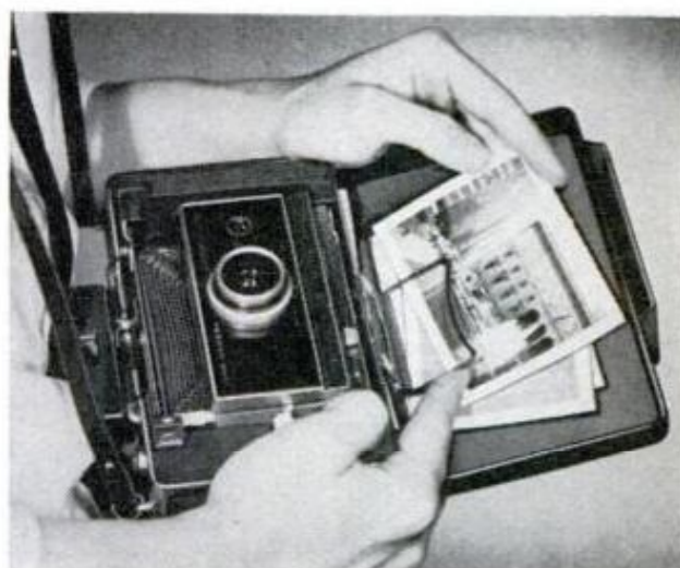
FRONT CASING of Polaroid 100 has a clip for holding prints during shooting session. Photographer must still dispose of messy negatives as before
