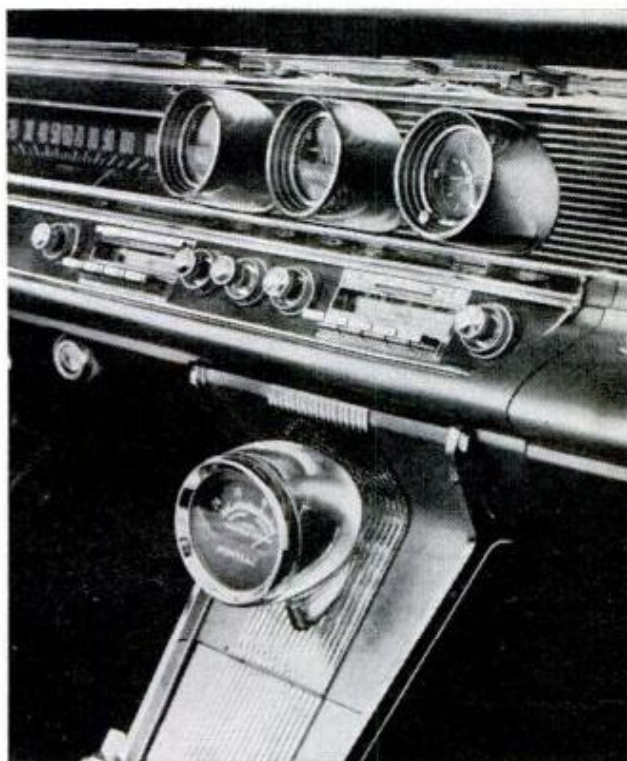
A NEW SLANT ON PONTIACS' instrument housings points dial faces slightly to the left so the driver can see and read them more easily. Tach is in console
