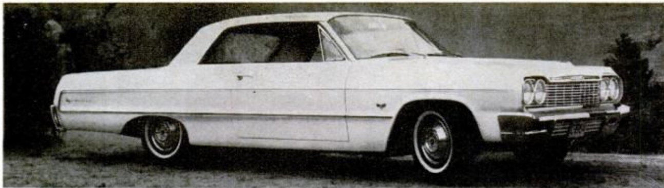
ALL-NEW SHEET METAL FOR THE CHEVROLET'S basically unchanged body and 119-inch-wheelbase frame give a new yet familiar look to the car for 1964. Mechanical changes are minor but even Biscayne now has a hot V8 option
