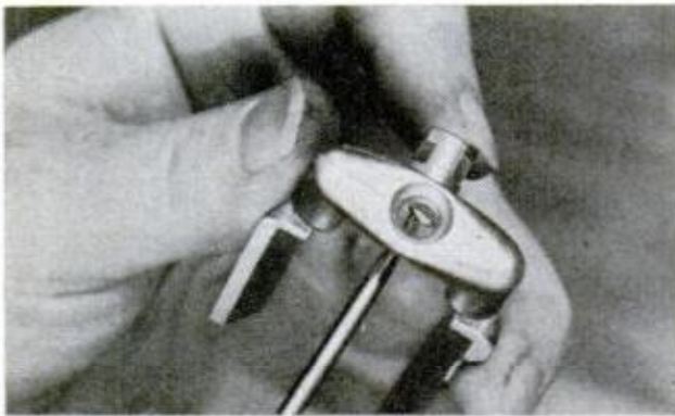
BRASS SLIDE that rides in yoke at outer end of carrier arm is fastened to rasp frame with small screw
