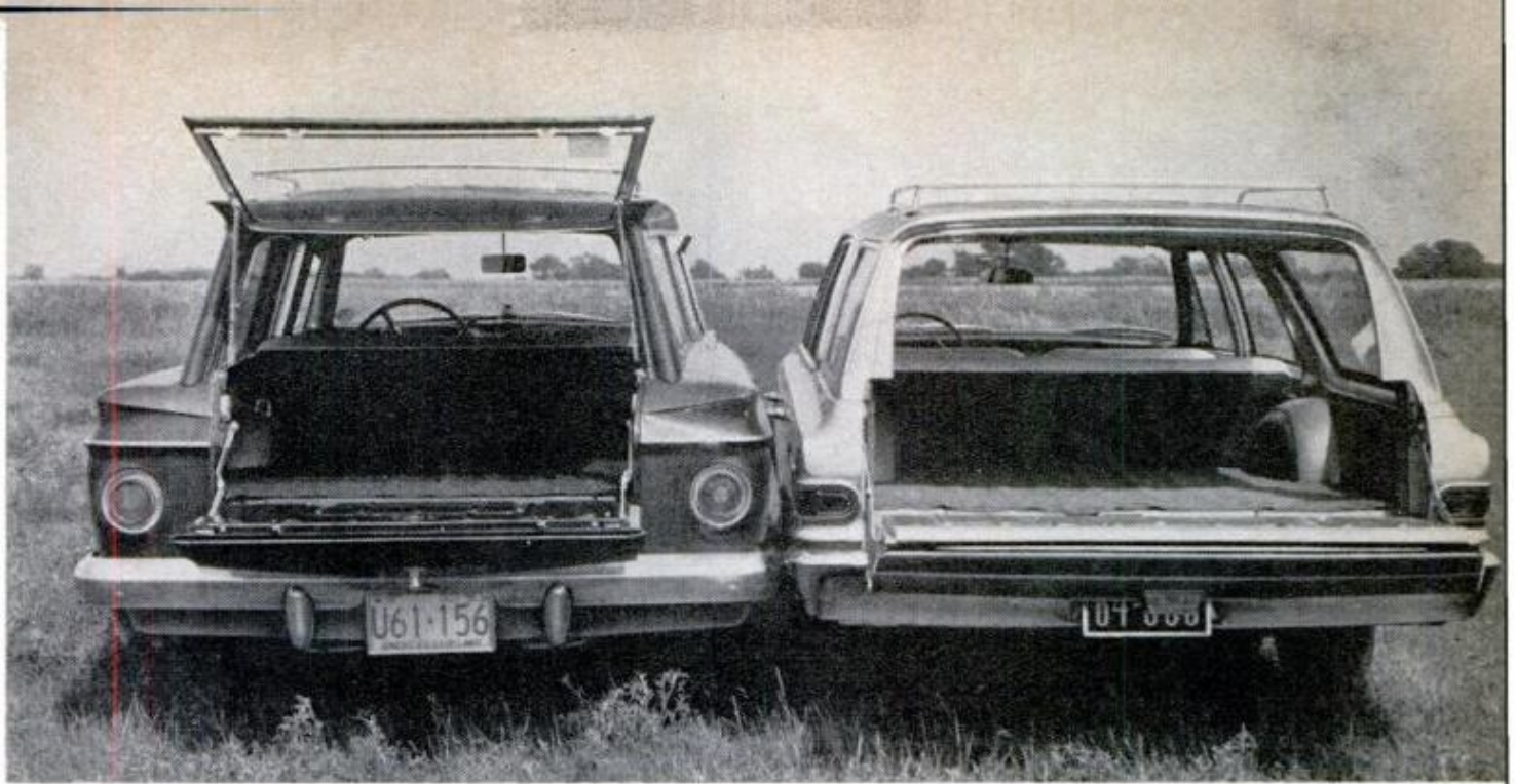
DESIGN PROGRESS IS SOMETIMES GRADUAL , sometimes startling. This comparison of the 1963 (left) and 1964 Rambler American wagons shows increase across rear seat of from 42 to 57 inches—and more loading area
