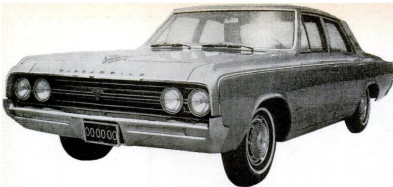
ONE OF THE FOUR GENERAL MOTORS PARTNERS in a joint new body-and-frame venture, the Olds F-85, now has its own 330-cubic-inch V8 engine and shares Buick Special's 225-cubic-inch V6. Wheel diameter is up an inch to 14
