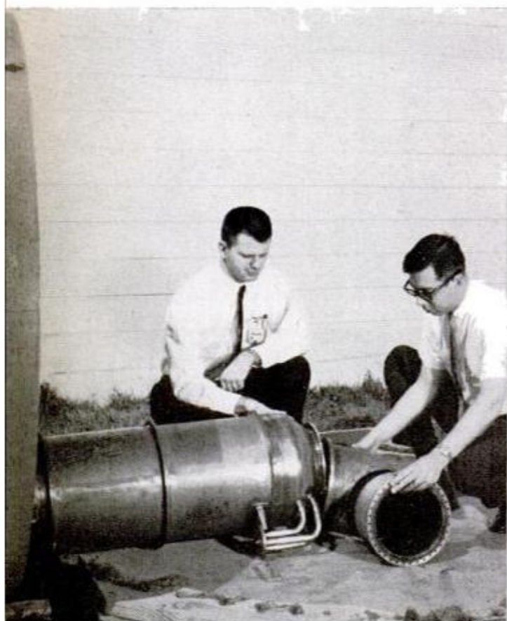
FAULTY EXHAUST DUCT of a rocket arrives at the morgue, and is carefully unpacked by "Doc" Rollin Wagner (right), head of the small group of "space coroners," and one of his assistants, Robert Manzell
