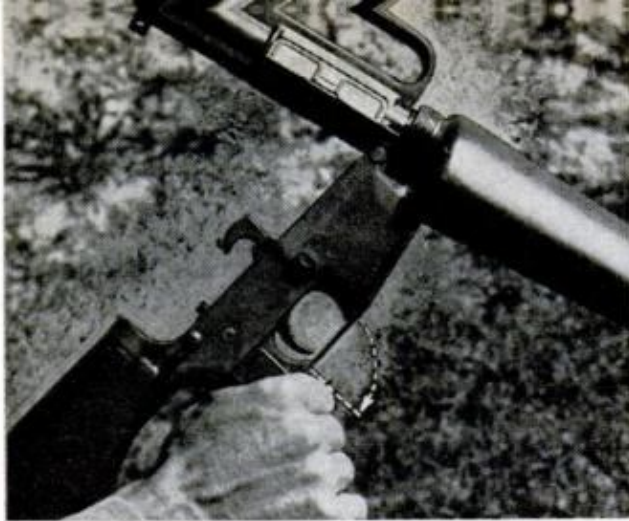
UNIQUE HINGED TRIGGER GUARD on the AR-15 can open to allow rifleman to shoot while wearing gloves
