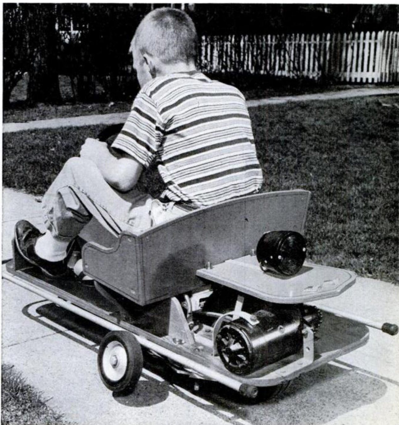
ROLLER-CHAIN assures positive drive from motor to ground wheel. Slack in chain should not exceed \frac{1}{2} in. Note position of the ground and power straps
