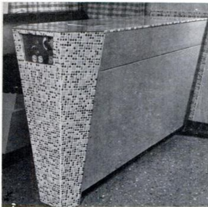
DINER COUNTER , made by engineer John Lenz for his home, is a combination table-dishwasher-disposal unit. Sides come off easily for servicing
