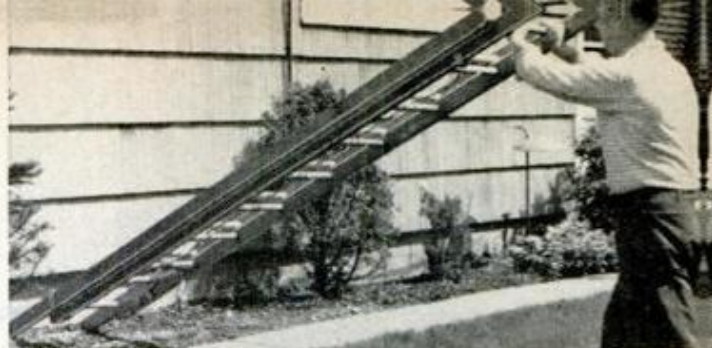
2. Raise ladder until end is head-high, grasp top rung as shown and "walk hands" toward the building
