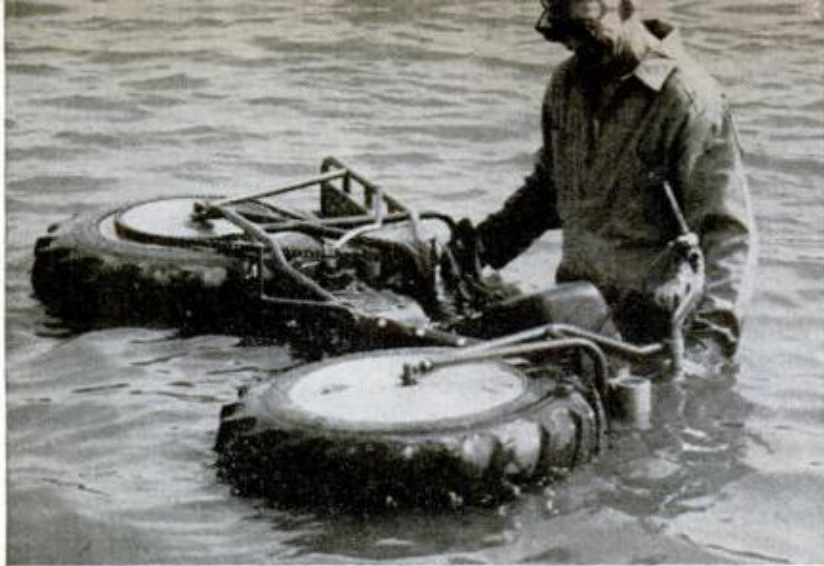
CYCLE WHEELS are actually airtight drums, enabling vehicle to be floated in deep water. Fitted with outrigger pontoons, it maneuvers like a boat with driver on the seat
