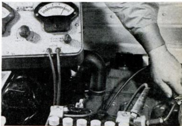
BATTERY CHECK using hydrometer is made by drawing a small amount of electrolyte out of each cell
