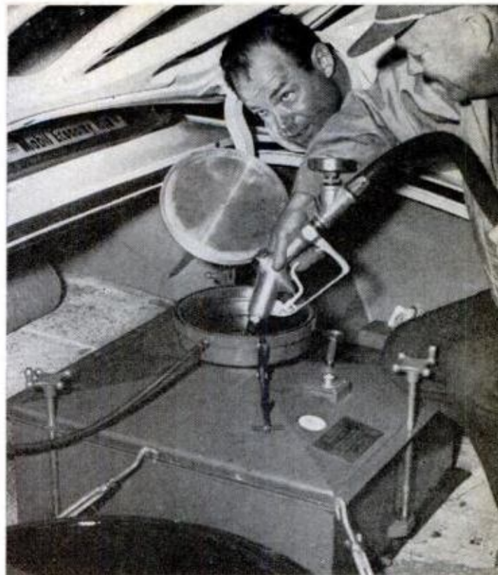
GASOLINE is metered into special Mobil Run tank by a U.S.A.C. official at two daily fuel stops. Gas is measured in 1/50th gallon increments at topoffs
