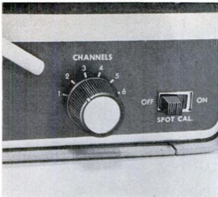
GOOD VS BAD. Selector switch that crystal-controls both transmitter and receiver (above left) is easy to use and absolutely accurate. Continuous tuning dial (right) on superregenerative sets only approximates channel settings.
