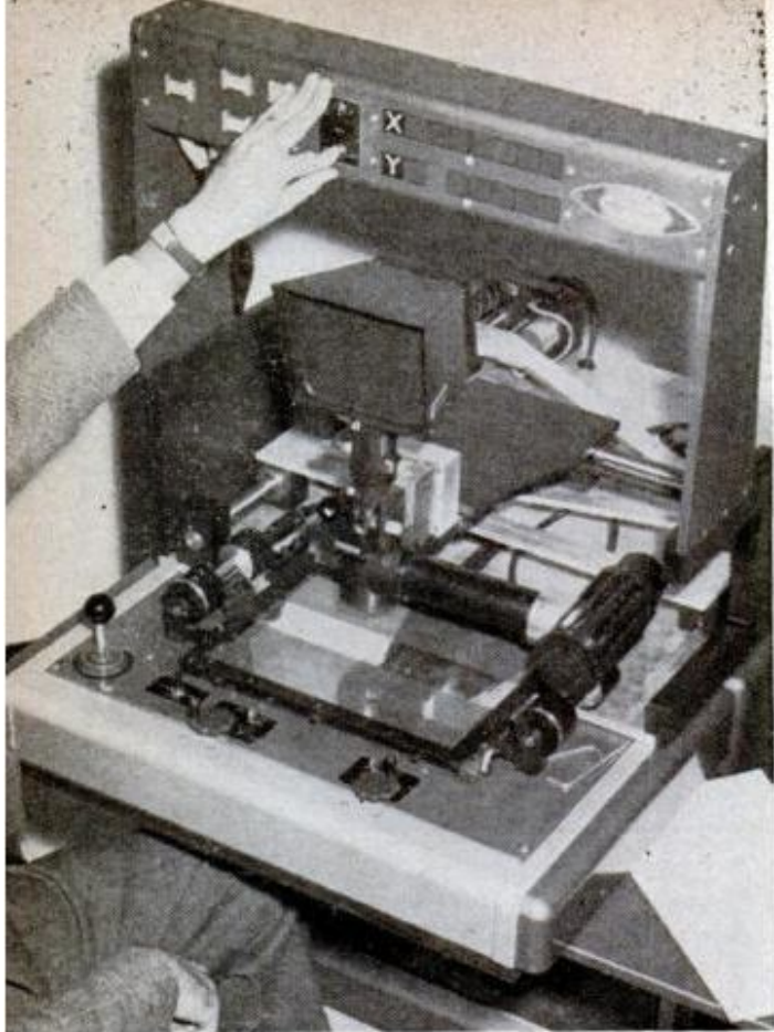
READOUT MACHINE aids investigators. Tape is smoothed out under glass, tracings are magnified on screen, and computer measures each minute marking
