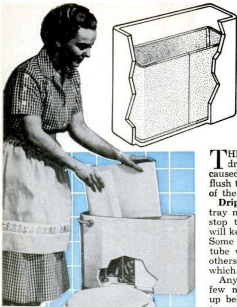
STYROFOAM lining, called Jayelite, prevents tank walls from cooling and thus stops condensation
