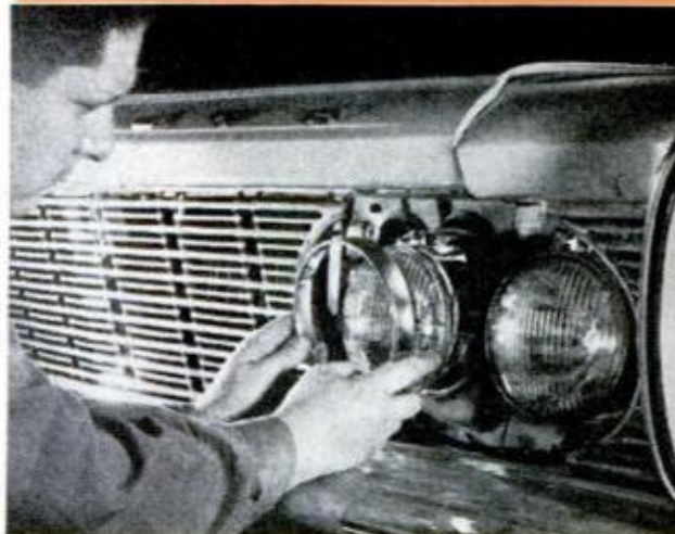
ALMOST AS SIMPLE as replacing a household bulb: Remove panel (page 157), then retaining ring (above)
