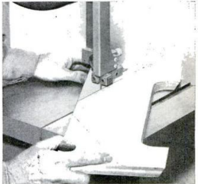
FOOT OF SLIDE FRAME is bandsawed from plywood; table was tilted for 60-deg. bevel at base. Dowel-supported cover (below) permits use in lighted room
