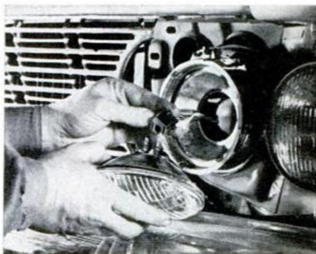
SEALED BEAM UNIT pulls out, towing its wire after. Unplug the connector from prongs. If you don't touch aiming screws, new lamp won't need adjustment
