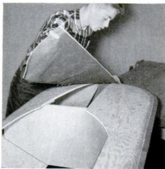
COVERING GAP between the right and left pairs of panels is the last step before finishing the hull. Allow 2 in. extra at cockpit and fold it underneath
