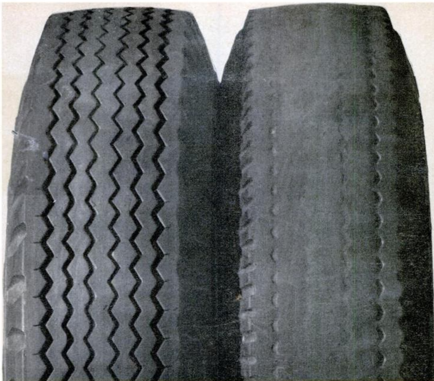
Super Hi-Miler (at left) vs. comparably priced truck tire (at right) after typical accelerated, high-speed, overloaded, 50,000-mile test on same equipment, over same roads, with same driver.
