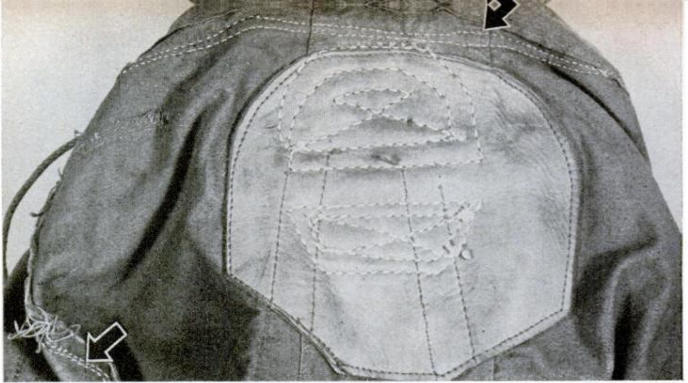
INSIDE SEAMS should be overlapped and double-stitched (arrows). Strap connections should be leather reinforced, and wear areas all multiple-stitched
