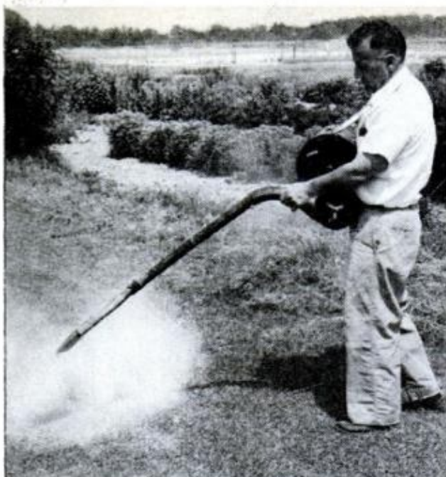
CRANK DUSTER comes in wide variety of sizes, from small hand-held model to this large heavy-duty type
