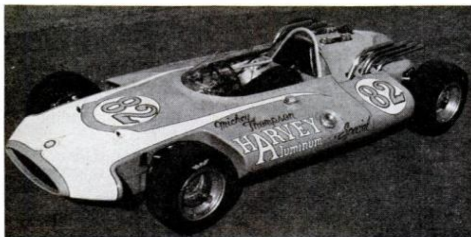
HARVEY ALUMINUM special at left, by Mickey Thompson and powered by an aluminum Chevrolet V8 of 350 horsepower will weigh 1050 lbs. dry, 36 percent less than the average Watson or Kurtis-built Offy-engined car. Sketch, top, shows the major parts
