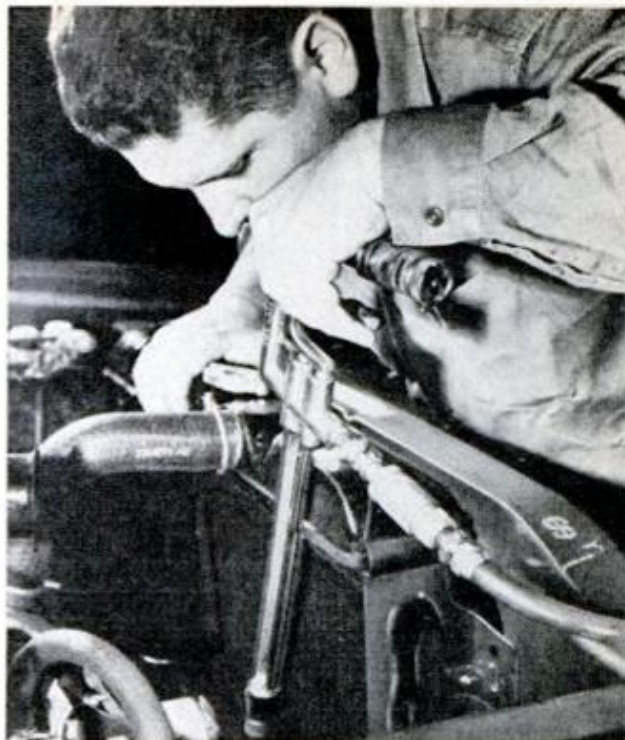
STREAM OF AIR directed through the radiator from the rear face will blow bugs, debris and dust out of the core. Loosen large bugs with a soft brush
