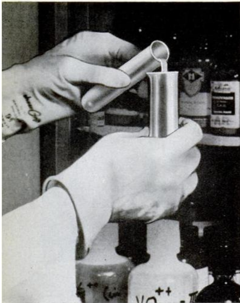
WHERE POISONING is suspected, a specimen of the victim's hair or nails is placed in a reactor. The poison is then isolated by radiochemical separation
