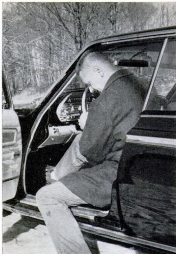
STEEPLY SLOPED windshield corner post combines with forward location of center post on four-door to make for head-bumping, according to some owners
