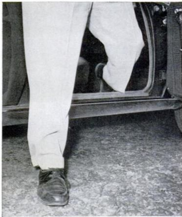
TEMPEST'S FLOOR , like so many others, is recessed to provide adequate interior height combined with the fashionably low roofline buyers seem to want
