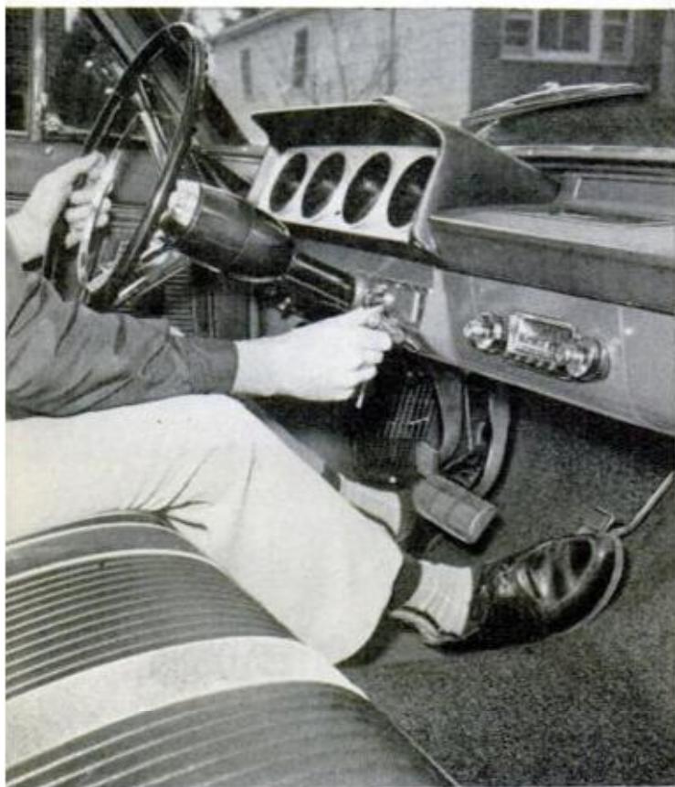
TRANSMISSION RANGE SELECTOR down on the dash led the list of owners' complaints about the interior. With transmission in rear, front foot room is good
