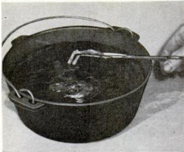
7. PLUNGE the zinc-coated part into cold water immediately after withdrawing it from the zinc bath
