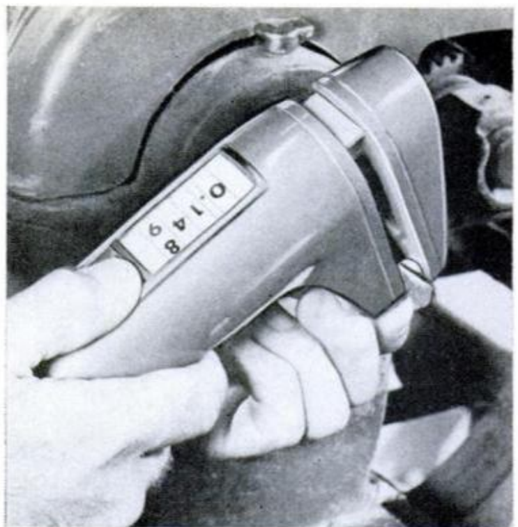
ELECTRIC MICROMETER uses tiny battery-powered motor to move anvil in and out, stalls at just the right pressure. Dial counter is spun by same drive system
