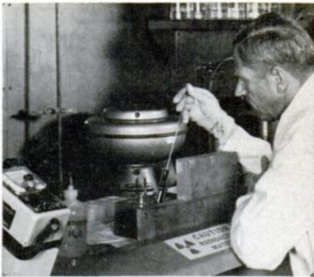
A SMEAR from the hand of a suspected gunman is prepared for NAA analysis; this may soon replace the paraffin method for detecting gunpowder residues
