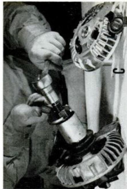
ALTERNATOR REPAIRS in chart include: (A) Replacing brushes—a lot easier than same job on a generator; they spring out when unscrewed from their sockets (arrows). Numbers are to show this is a six-rectifier alternator. (B) Replacing stator—just pry from case; (C) Replacing rotor—use pulley tool. In each photo, new parts are ready nearby
