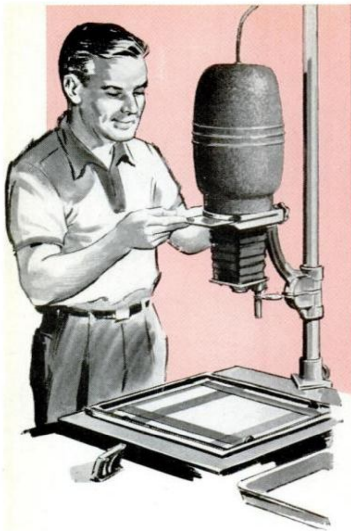
BLACK-AND-WHITE NEGATIVES of extreme contrast are made by simple process of projecting or printing color transparencies directly on high-contrast film
