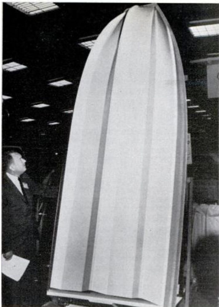
MODIFIED CAT HULL of this 12-ft. fiberglass fisherman has three longitudinal runners for more stable ride, weighs 110 lbs. Selling for under $200, it's made by Molded Fiber Glass Boat Co., Union City, Pa.
