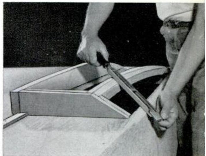
SPONSON FRAMING will require a considerable amount of fairing. To save time, you might cut this bevel oversize with a saw, then finish it with rasp
