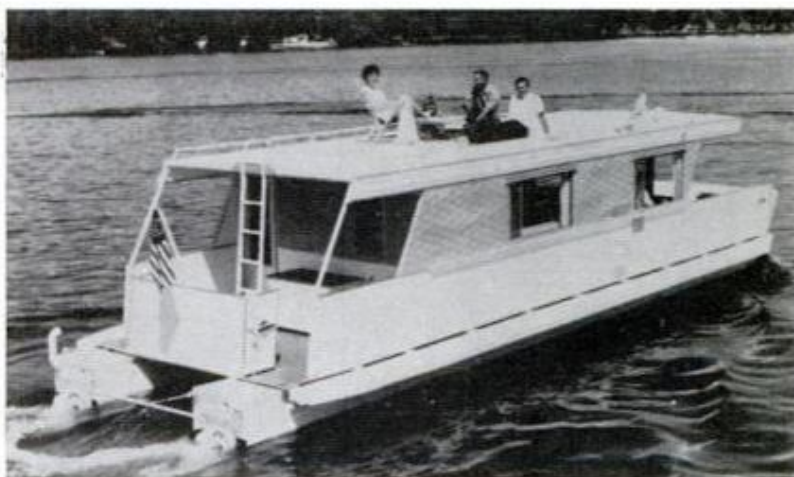
42-FOOT HOUSEBOAT powered by twin stern drives mounted in pontoons is equipped with gas refrigerator, hot-and-cold pressure water system. Without stern drives, it's priced at $8900 f.o.b. Carri-Craft factory in Berlin, Wis.
