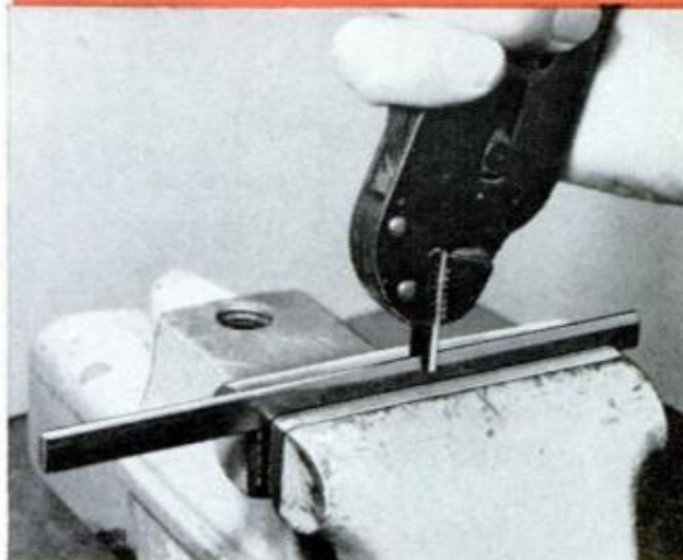
CUSTOM-MADE CUTTER makes fast work of wooden gears. Before filing teeth (sketch), bevel bar with file, and finish shaping with scraper made of tool steel
