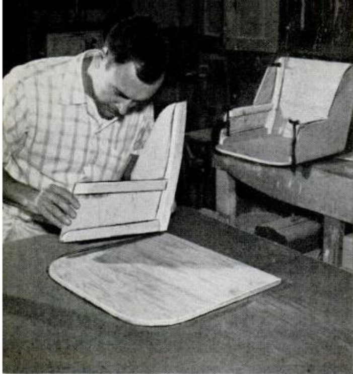
BUCKET SEATS are framed with light battens obtained by cutting 1 x 2 stock in half on a circular saw
