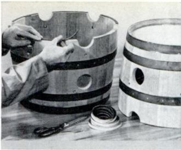
WEATHERSTRIP lower half of keg with adhesive-backed felt strip. Notch felt to obtain easy fit on curve
