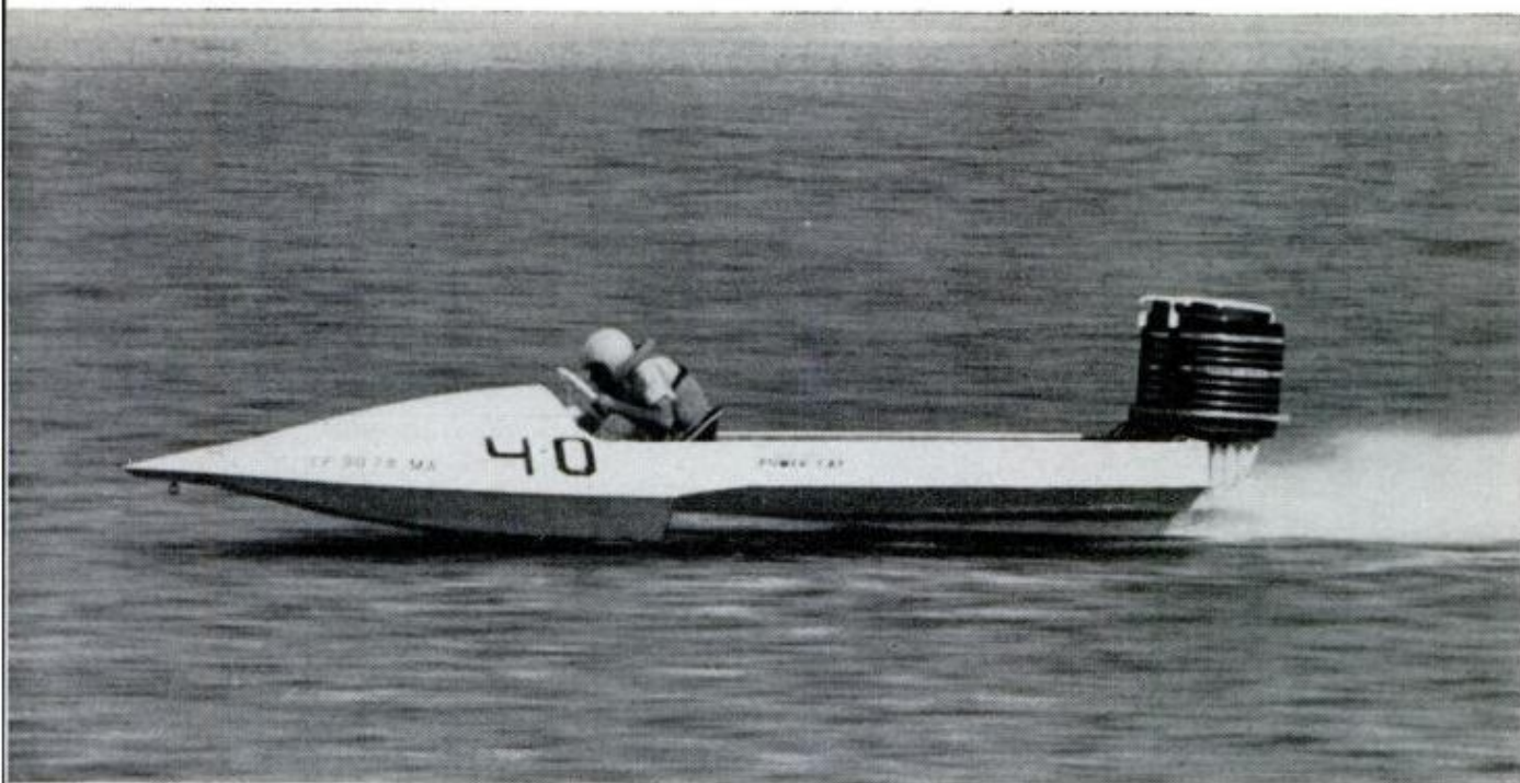
BARELY TOUCHING THE WATER , a dragster driven by two 100-horsepower outboards tries for speed record
