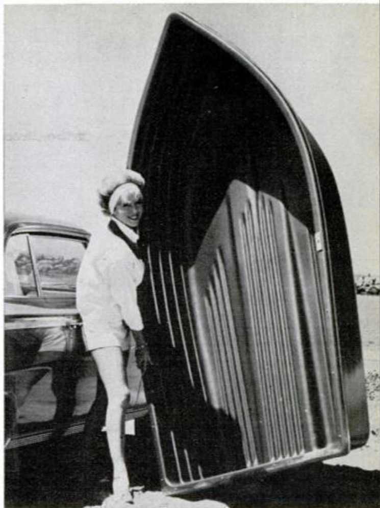
ULTRA-LIGHT 8-ft. all-plastic car-topper weighs 45 lbs., can carry over 500 lbs. Craft accommodates outboards up to 5½ hp. or special sail kit. Columbia Plastics Corp., Los Angeles, Calif., makes it
