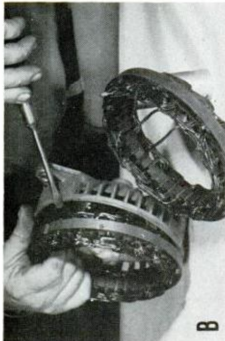
ALTERNATOR REPAIRS in chart include: (A) Replacing brushes—a lot easier than same job on a generator; they spring out when unscrewed from their sockets (arrows). Numbers are to show this is a six-rectifier alternator. (B) Replacing stator—just pry from case; (C) Replacing rotor—use pulley tool. In each photo, new parts are ready nearby
