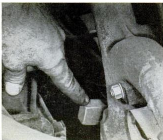
TURN COUNTERWEIGHT by hand to see whether manifold heat control valve is operating properly. It should pivot back and forth without resistance
