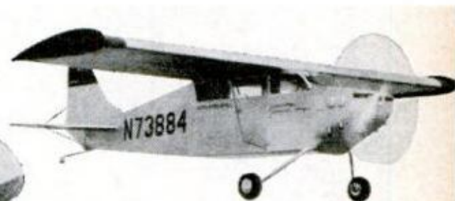
RUNNERUP was another cabin plane, Lacey M-10 , which has unique wing that doesn't fold but pivots to lay lengthwise. Cost: $1500
