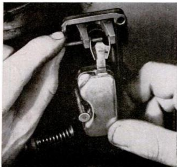
INSIDE THE CARBURETOR BOWL is a float assembly consisting of float (being disconnected at left) with a needle valve and seat beneath. In reassembling, check height with a float-adjustment tool, as at right
