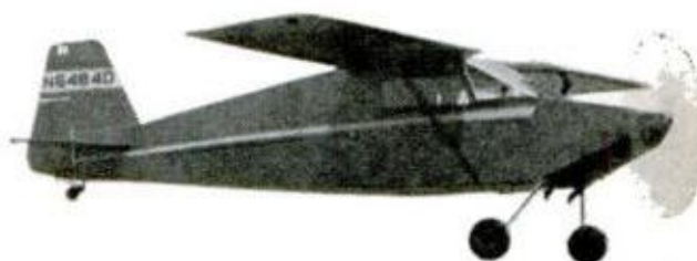
THIRD PLACE went to two-place cabin plane, Eaves Cougar I . It cruises at 125 m.p.h. and has range of 500 miles. It also cost $1250
