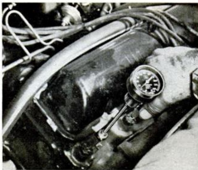
ENGINE COMPRESSION TEST determines if a burned valve is causing rough idle, but won't necessarily tell you if trouble is caused by a sticking valve
