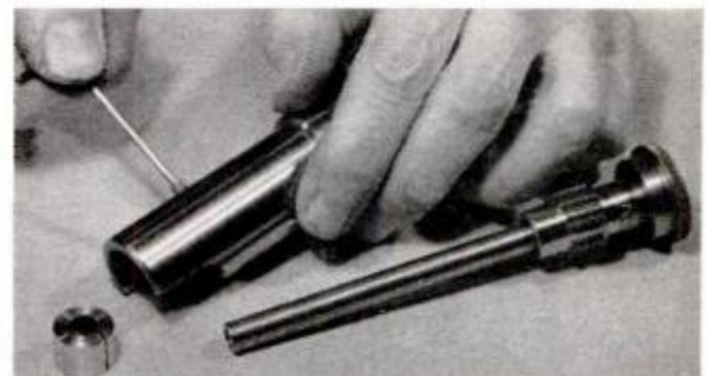
2. SPLIT BRONZE BEARINGS are held in recesses by setscrews, which also adjust clearance. Gear shaft (lying alongside body) is inserted through them
