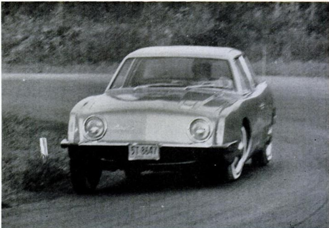
ON THE RAGGED EDGE of controllability at 50-55 mph in hard right bend, Avanti ploughs with overweight front-end causing an understeering problem
