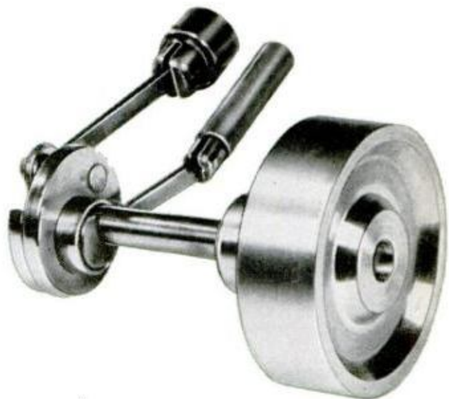
CRANKSHAFT ASSEMBLY , detached from engine block, shows how connecting rods link pistons to crankplate. Both plate and eccentric are soldered to flywheel shaft
