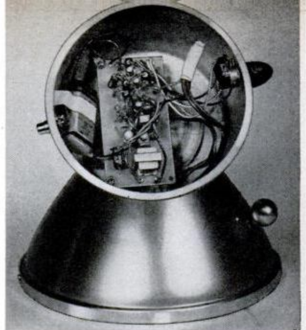
VIEW FROM BENEATH amplifier shows location of parts in the lamp base housing
