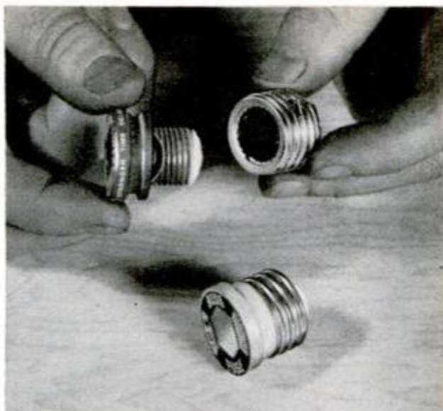
TAMPER-FREE FUSE (held in right hand) has smaller-diameter base that requires special adapter to fit standard socket for Edison-base fuse (foreground). Spur on adapter locks it permanently into socket
