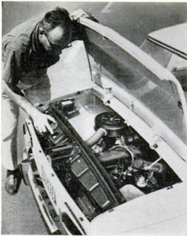
FAN on R8 engine, left, draws air down through slots in rear deck lid, then forward through sealed cooling radiator and thence to a final exit below car
