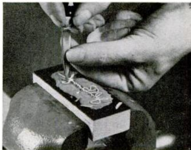
3. FOR SIGNATURE stamp, cement pattern face down on linoleum block and cut away background
