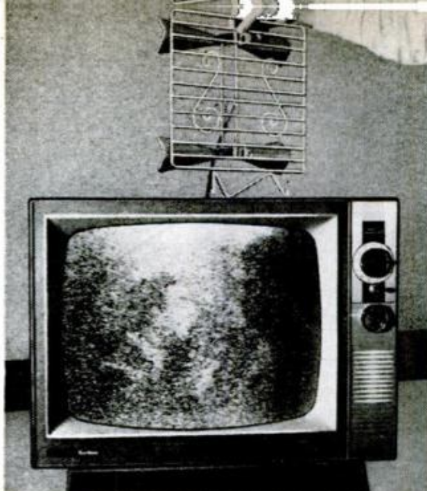
INDOOR ANTENNAS for UHF give poor pictures in fringe areas. Weak signals need outdoor antenna
