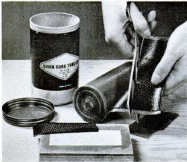
7. CUT GUM RUBBER to approximate size of stamp, and place two layers over the talc-polyester matrix
