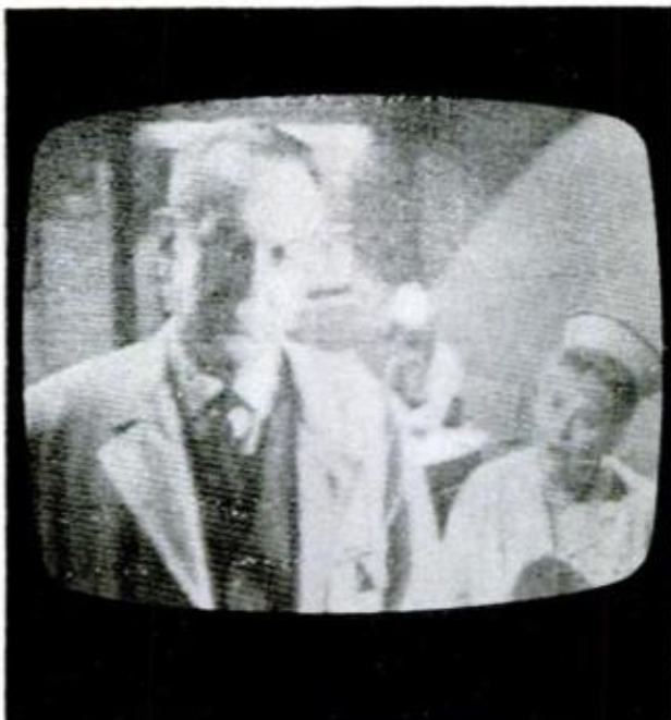
UHF PICTURE , taken about same time as VHF picture at left, picks up hardly any interference, yet both sets were equidistant from station and interference
