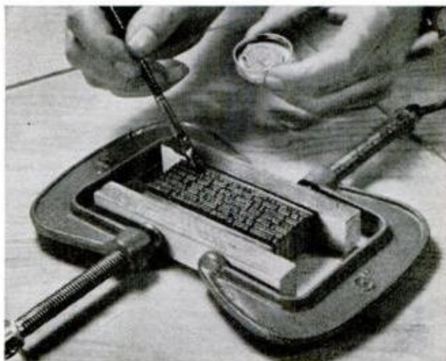
2. CLAMP TYPE SLUGS between \frac{7}{8} -in.-high wooden bearer strips and paint them with a parting agent
