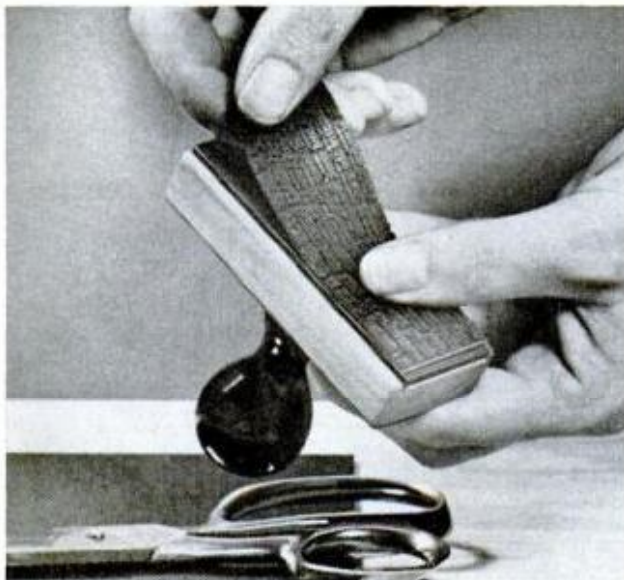
9. MOUNT CURED DIE on block over 1/8-in. sponge-rubber cushion, using a thin-bodied rubber adhesive
