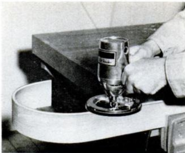
ROUNDING OVER edges of slats and runners is quickly done with a router-shaper, or with sanding block
