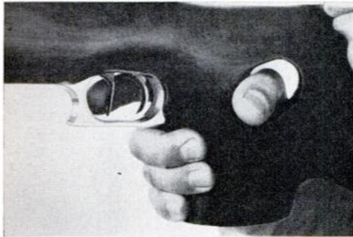
RIGHT-HAND POSITION on free rifle shows "saw-handle" pistol grip and double set triggers. Natural fit aids right hand's single task — squeezing trigger
