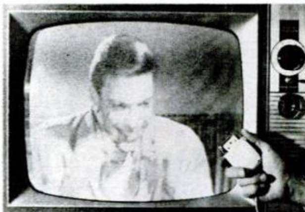
OUTSIDE ANTENNA produces excellent UHF picture. Even electric razor does not distort it, as it would VHF
