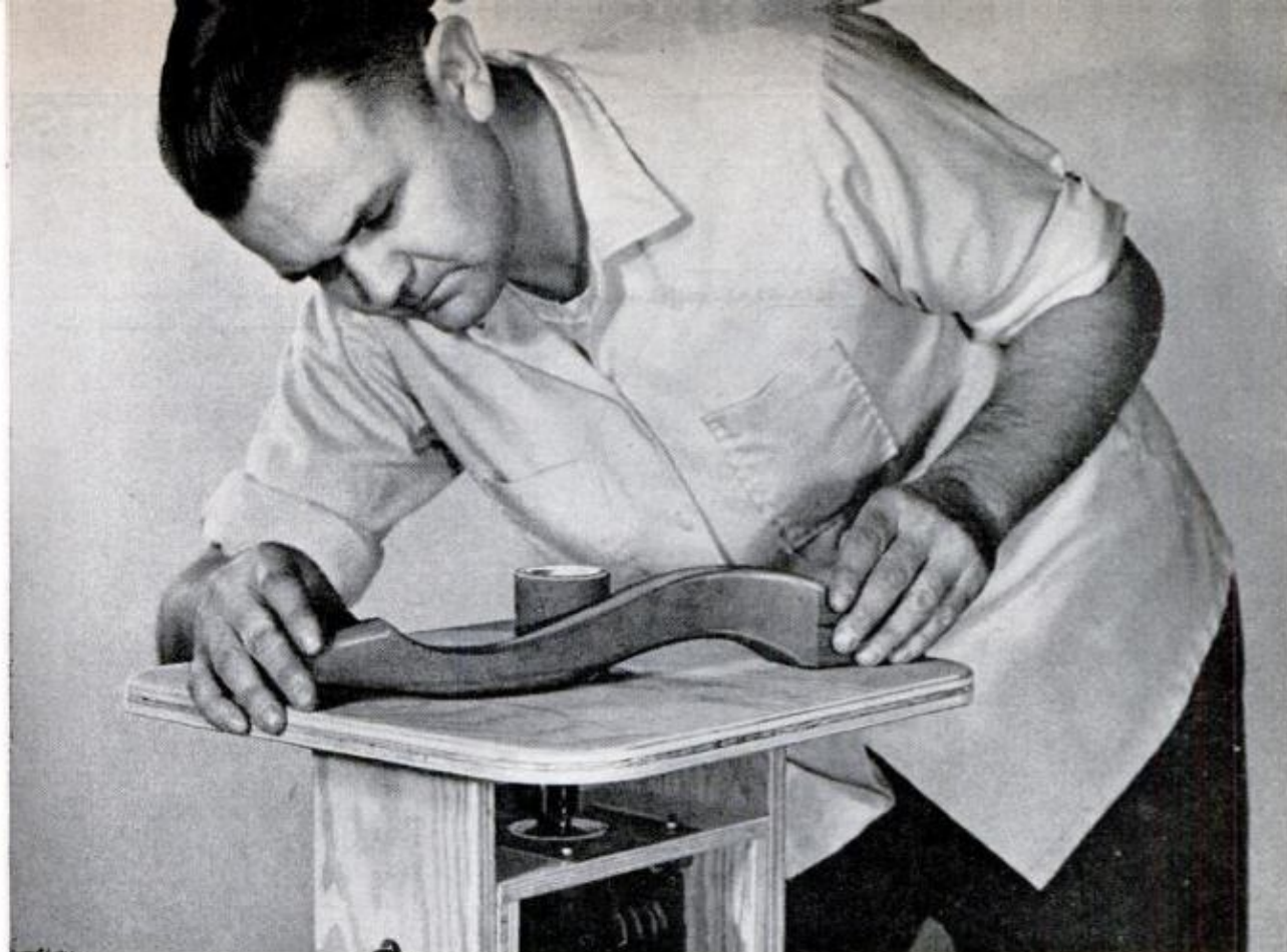
FAST SANDING of such difficult work as a bandsawed cabriole leg. Table can be raised or lowered easily
