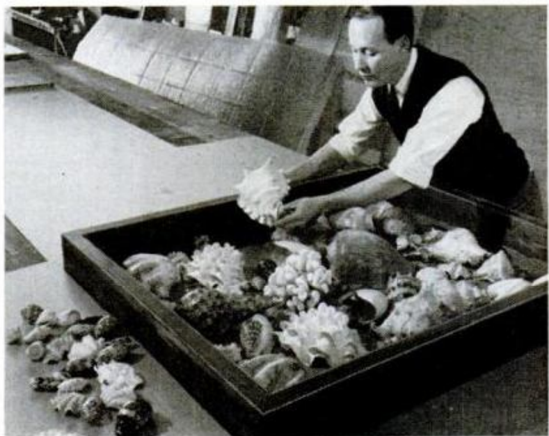
UNLIKE PANELS , such wall decorations use only one plastic sheet. Shells arranged on wet sheet become fused permanently when dry
