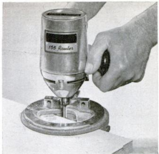
ROUTER JIG in use. Care must be taken to set it so that edge of laminate will be trimmed flush, no more
