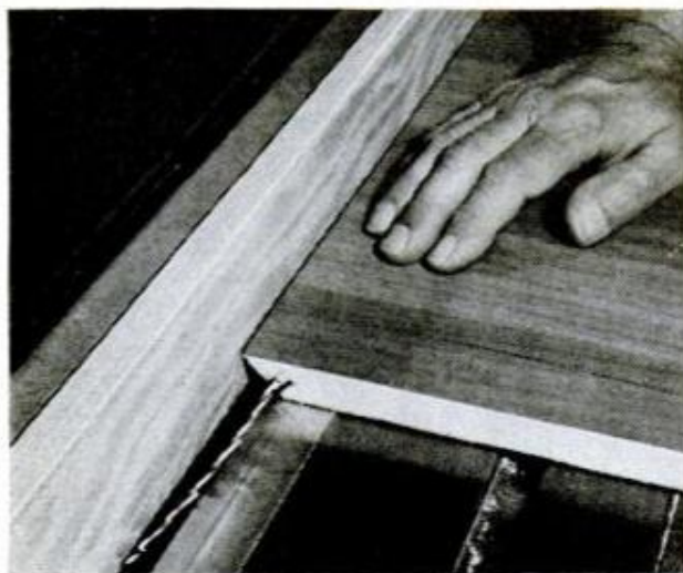
5. ASSEMBLY OF CABINET with one miter joint clamped and a second being assembled. Note especially the spline in, unassembled miter and spacing of the four pairs of triangular clamping blocks
