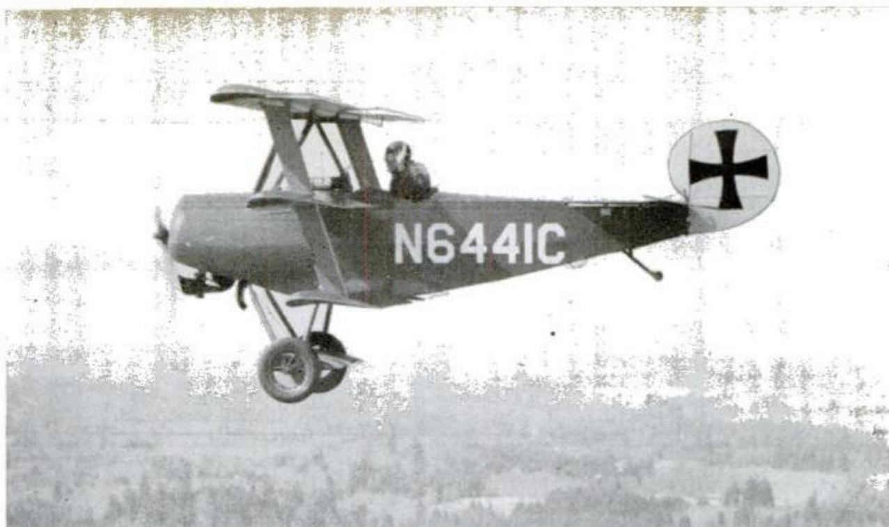
PINT-SIZE REPLICA of German Fokker Triplane was scaled down to \frac{3}{4} -size, fitted with new 65-hp. engine
