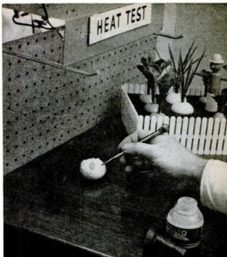
SHOCK CHECKING phonograph chassis (upper left) and heat testing toy vegetable (upper right) with temperature-indicating paints—two of the tests which supplemented an expert judging of the PM toys' play value
