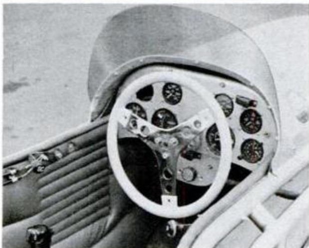
STEERING combines wheel and "dead man" control that shuts off everything if pilot relaxes grip
