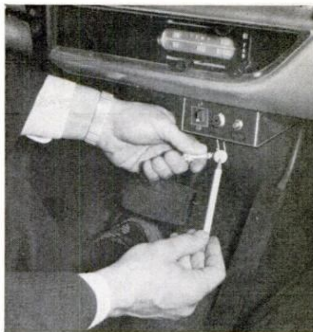
INTERIOR THERMOSTAT is held behind the dash-panel unit in free air out of airstream of the car heater
