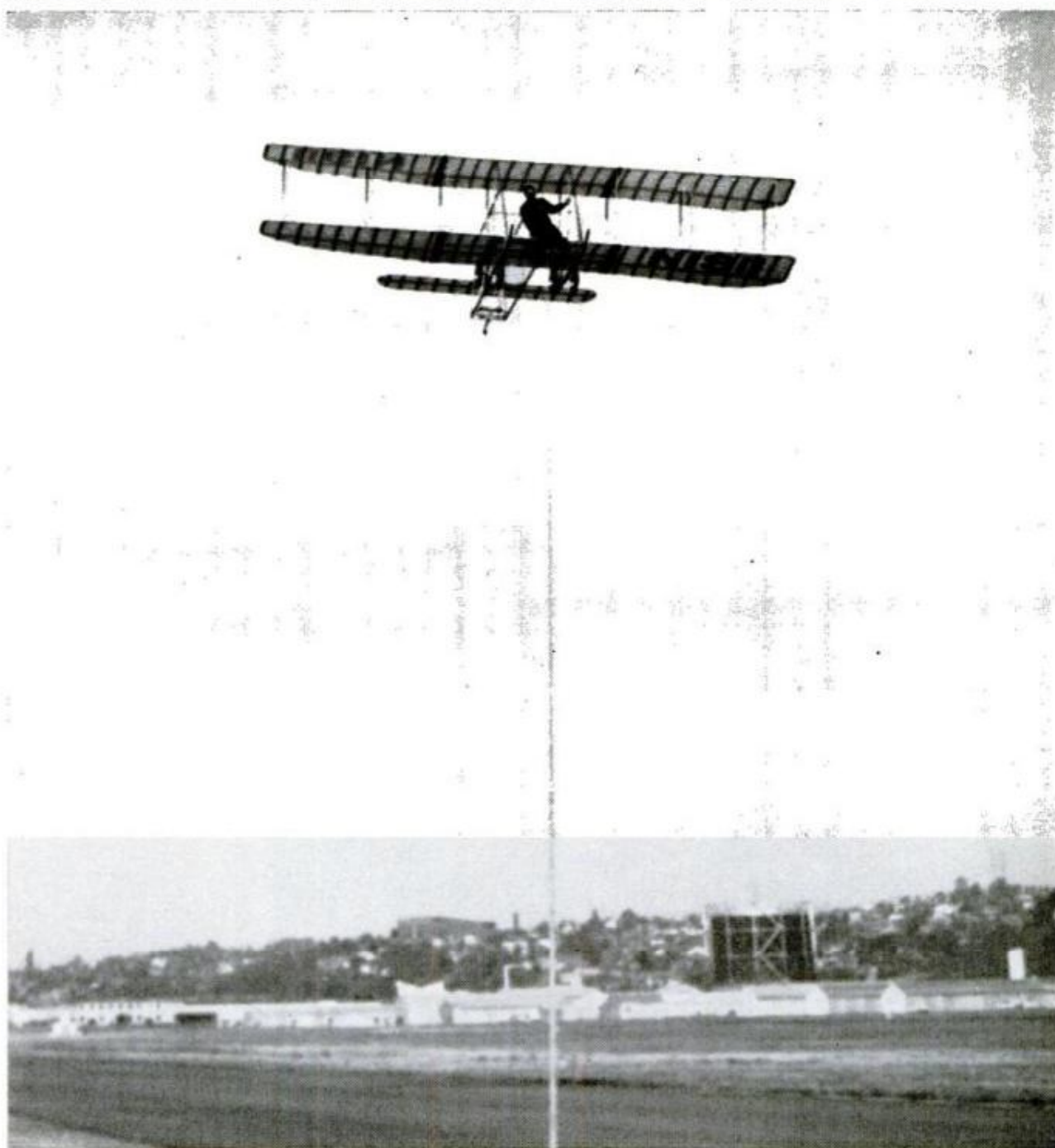
WRIGHT REPLICA was built new by Bowers. Original was first plane to cross United States. Below Bowers flight tests it, without engine, by tow rope hitched to car. Glider flights prove craft's airworthiness
