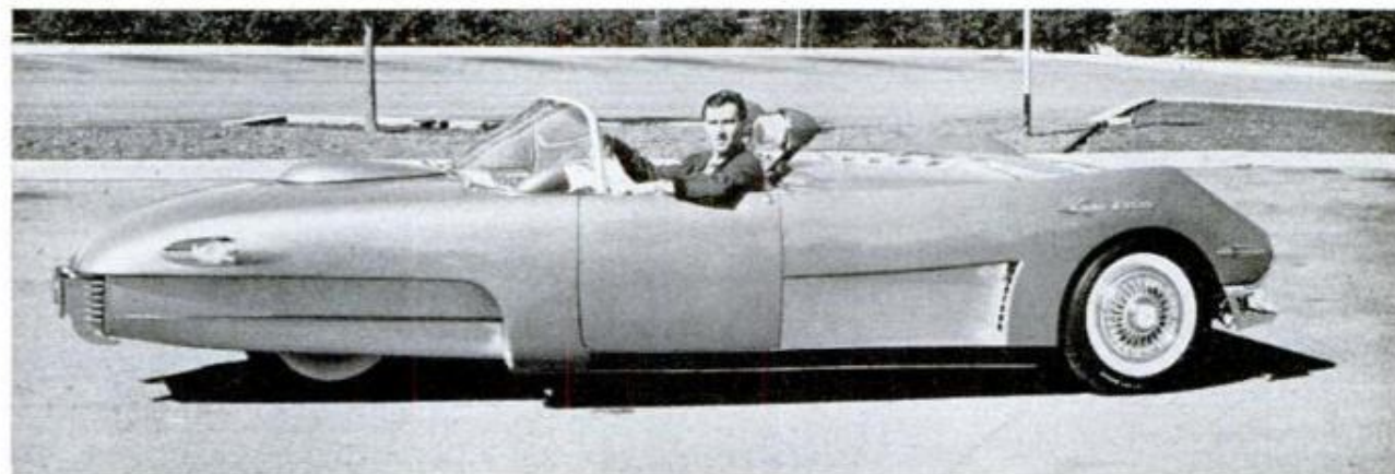
TRIANGULAR SHAPE of the Vortex emphasizes builder's use of full-width taillights which are encircled by the rear bumper. Door locks are electrically-operated by the driver. Windshield frame incorporates a roll bar
