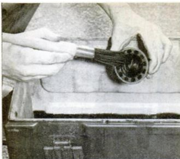
8. AS FIRST STEP in making installation remove the breather cap, clean in solvent thoroughly and re-coil
