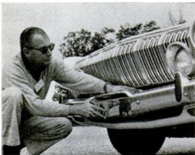
DODGE'S whale-toothed grille swallows human hand in search of a relatively inaccessible hood latch
