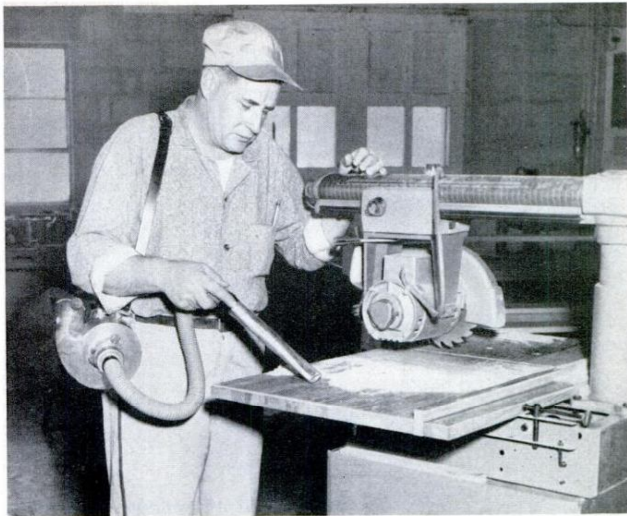
CARRIED WITH EASE, this little vacuum cleaner quickly removes all traces of sawdust from woodworking tools
