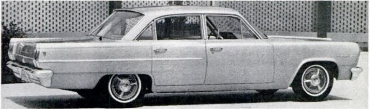
OLDS F-85 (above) has same inner body-frame structure and greenhouse as '62 model, but fenders, doors, panels are new. Instrument cluster for Chevy II NovaSS (below) has temperature, oil pressure, amp gauges
