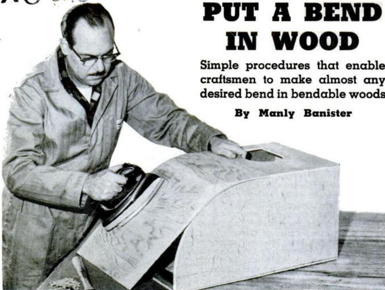
1. APPLYING HEAT with electric iron will cause \frac{1}{4} -in. plywood to take a moderate bend. Fasten as you go
