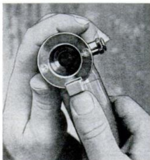
ROTOR ARM should lift out easily for occasional cleaning. Main rotor here is on direct drive. If machine has second rotor (page 131), top rotor is usually operated by water pressure only
