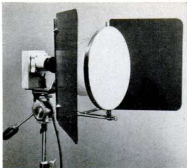
READY FOR USE , swinging vanes control background lighting and diffuser softens too brilliant light
