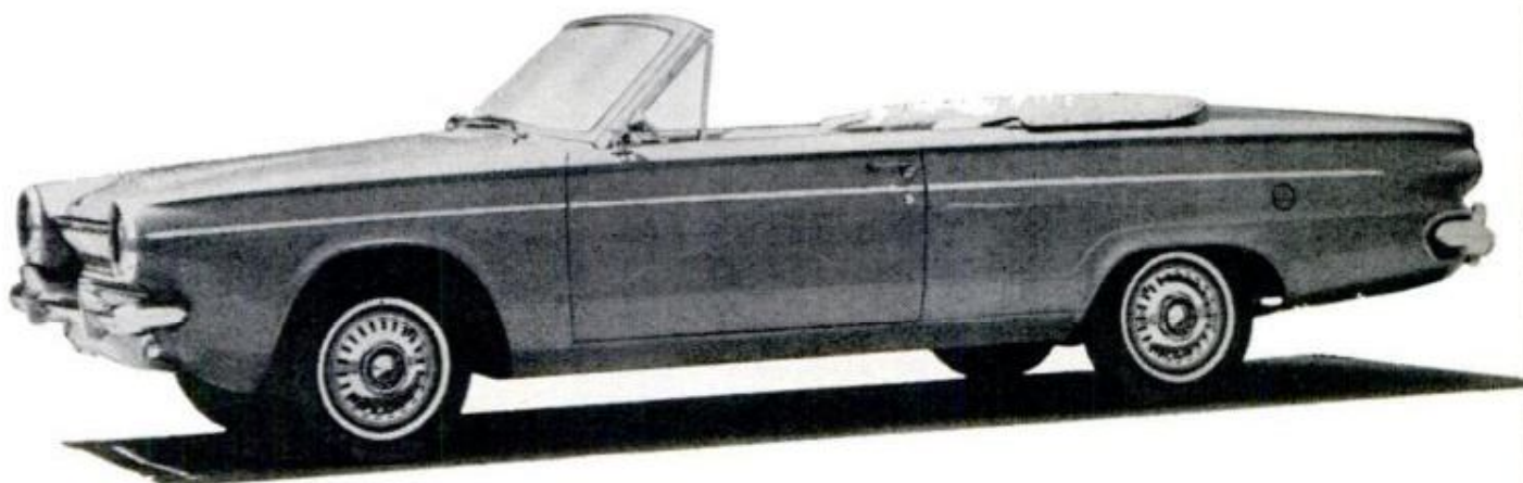
CONVERTIBLES are available for the first time on all Chrysler Corporation compacts. Above is Dart's on 111-inch wheelbase with choice of manual or automatic top. Front seat may be either three-place bench or buckets
