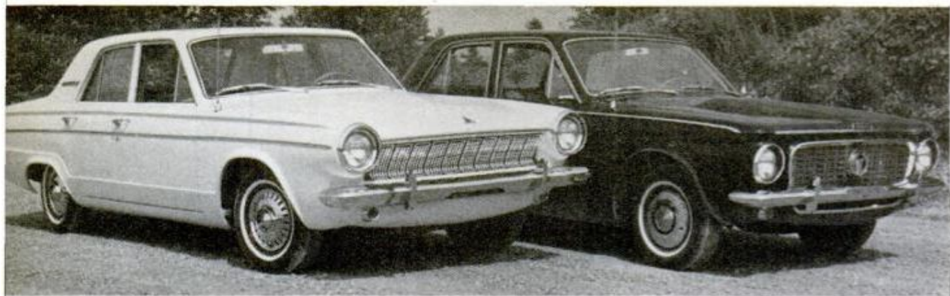
DODGE DART and Valiant looked alike, were sized alike in 1962. For '63 (above) they share slant Six engines, windshield, suspensions and drivelines but have different bodies. Valiant's wheelbase is 106, Dart's 111 inches
