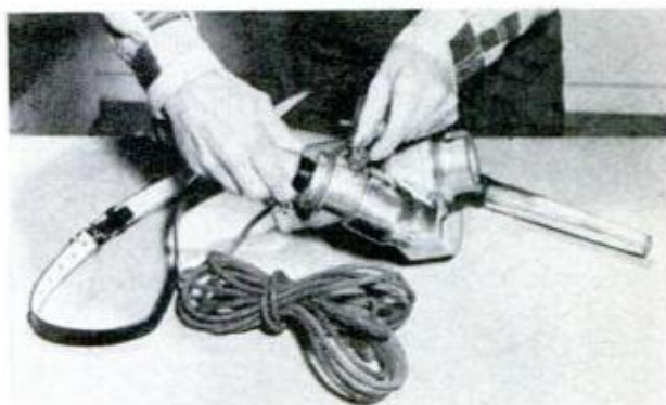
QUICK CONNECTION of the hose to outlet port of the unit before using it as blower to clean out crevices
