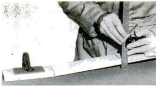
6. METHOD OF MEASURING spacing of kerfs. Raise stock until kerf at left closes. Then measure as shown
