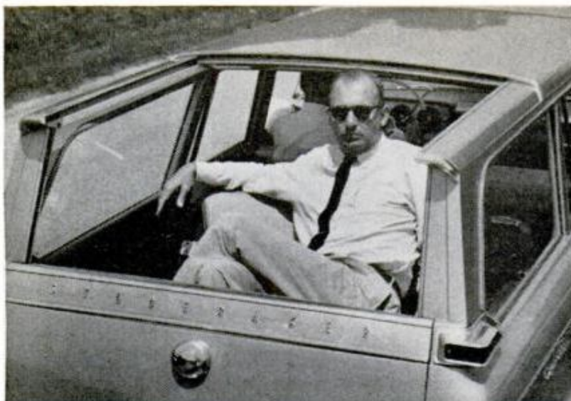
LARK'S ingenious sliding roof is standard on all station wagons; they call it Wagonaire. Panel slides rearward to meet back glass
