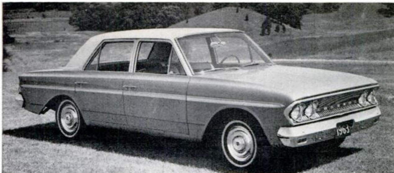
RAMBLERS have completely new unit bodies for '63. Shown above is Classic four-door. Although wheelbase has been upped from 108 to 112, over-all length has been reduced by over an inch. Windows are curved
