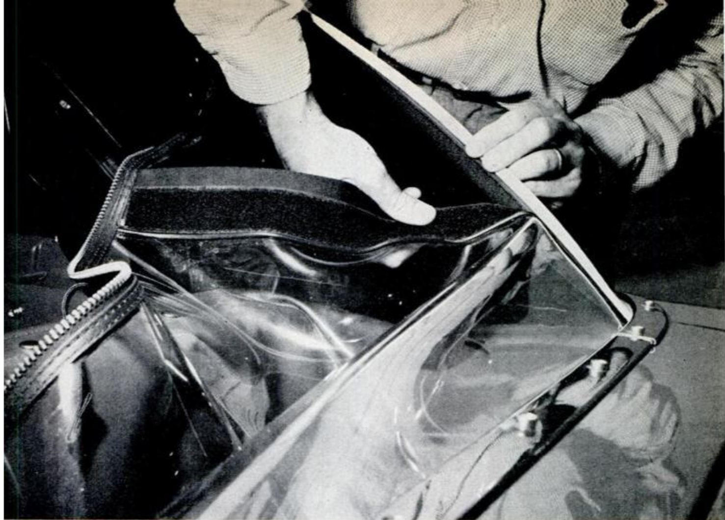
REAR WINDOW is sealed at the sides by merely pressing together the novel strips of nylon "cockleburrs"
