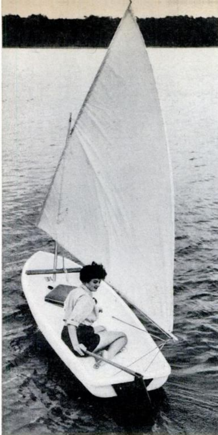
SAILBOAT has foamed hull, polyethylene sail, is 11 feet long, weighs 50 pounds but supports 500 pounds
