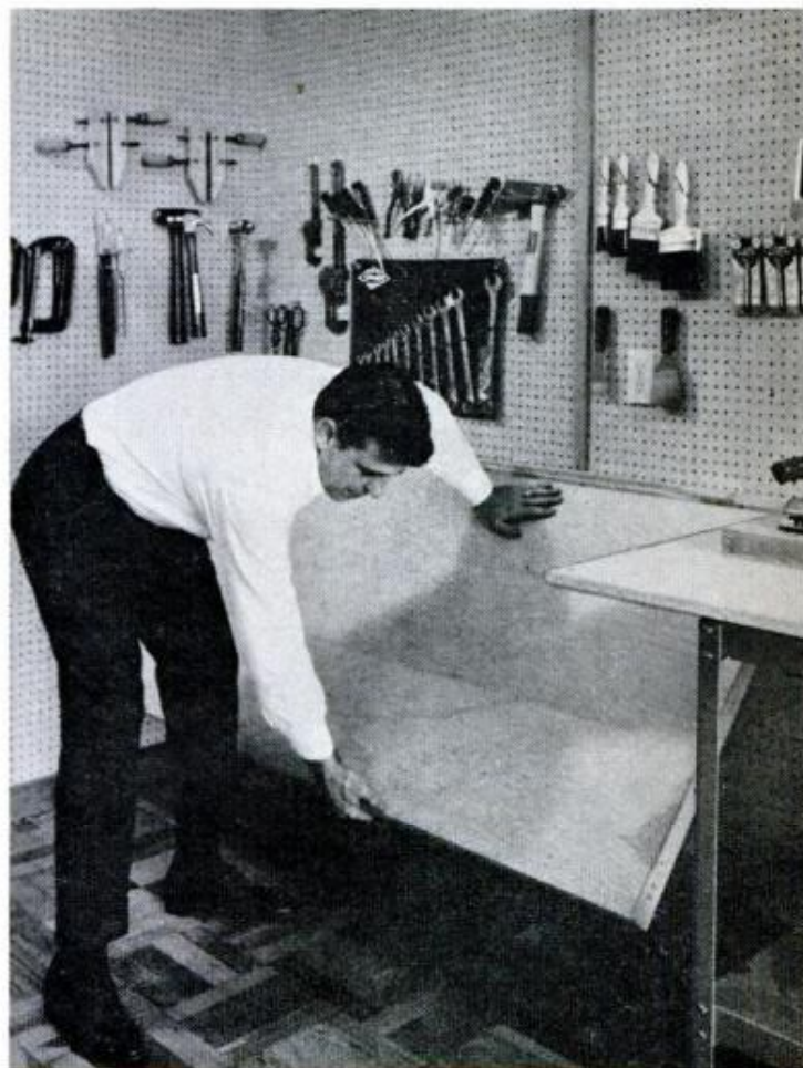
Workshop features a sturdy, folding bench on each side of radial-arm saw
