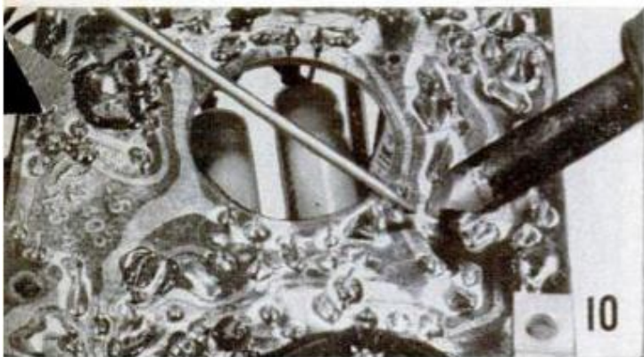
MOST KIT BUILDERS don't apply enough heat to printed circuit board connections. Make sure solder flows
