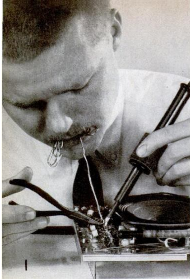
THIRD HAND? You can actually hold solder between your teeth while hands are busy. Use pliers or clips on component wires to draw off damaging heat
