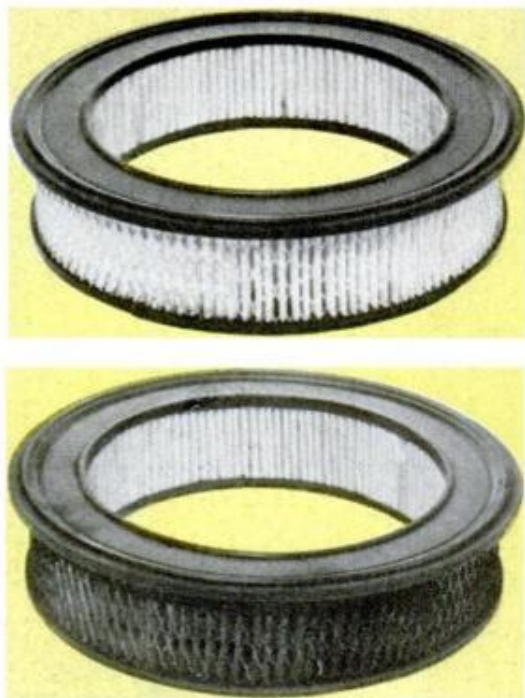
6. YOU CAN tell by this comparison photo which is the clean air filter. A semiclogged filter wastes gas
