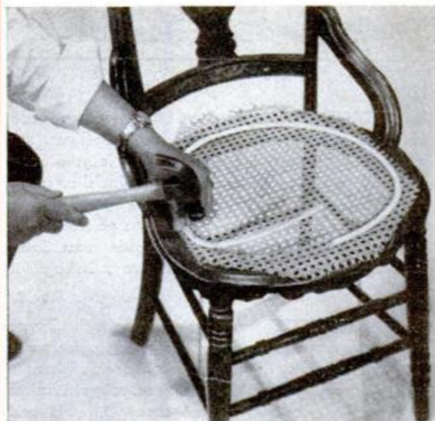
1. PLASTIC-COVERED electrical cord serves as a binder under clamping pads. Cord is tacked in place
