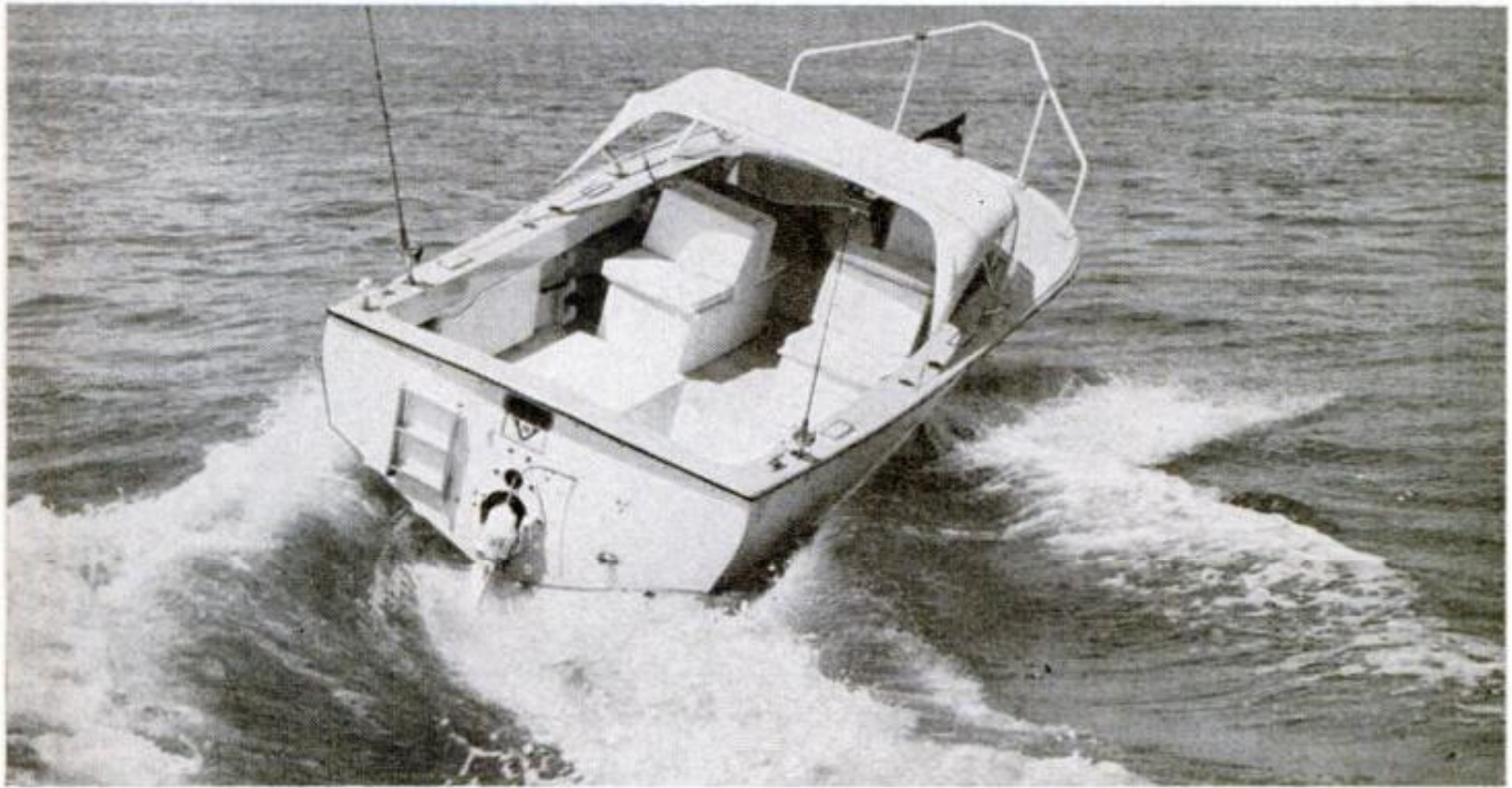
JIM WYNNE , Volvo outdrive designer, with his 17-foot sports runabout. Powered with a 100-horsepower Volvo unit, it hit 45 m.p.h.; won the 1961 Orange Bowl Endurance Race
