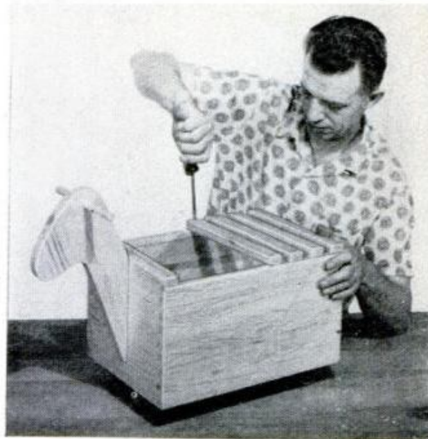
SLATS which form the seat, or saddle, of the horse cart are spaced and attached with screws and glue
