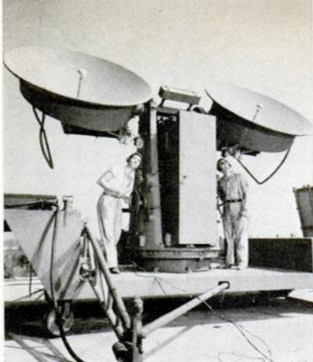
OLD Radar equipment was calibrated by tracking .22 rifle bullet fired over the surf
