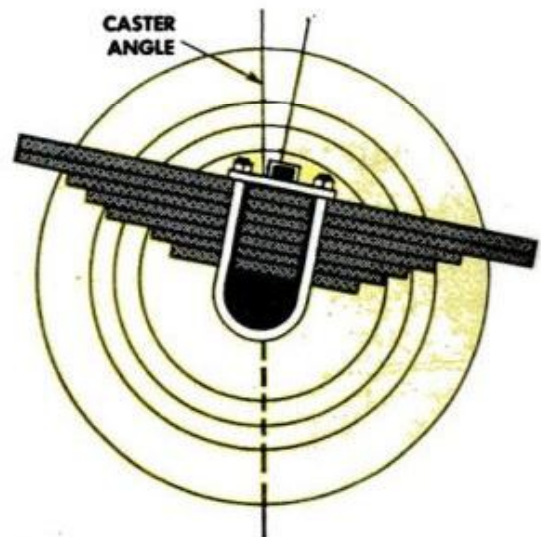
EXCESSIVE CASTER shown diagrammatically. Too much tilt of axle causes the tire tread to wear unevenly
