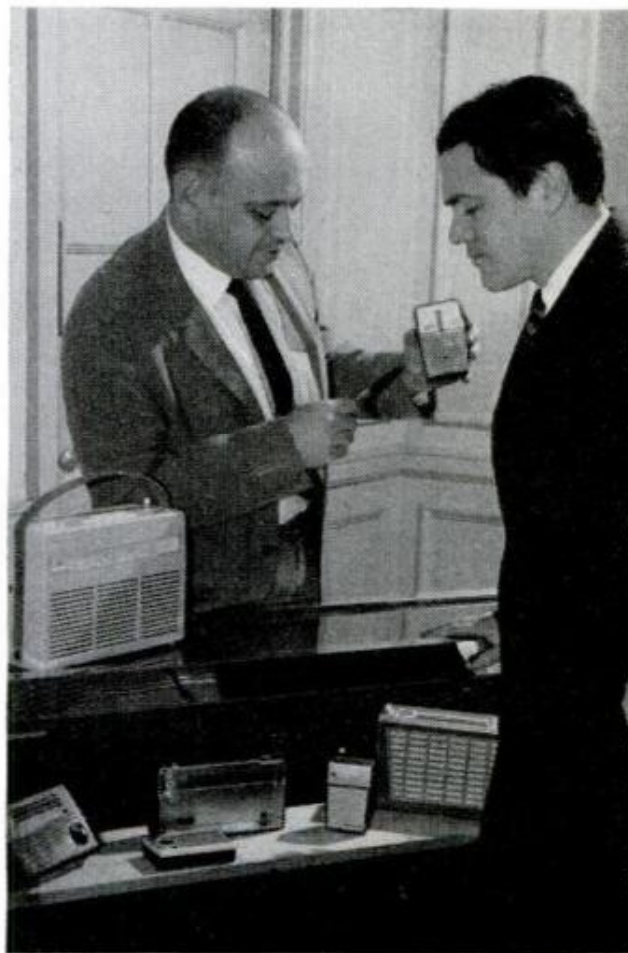
SOUND MAY INCREASE or decrease when set is grasped with hand. Raising set away from counter should not cause any additional alteration in volume or sensitivity, however
