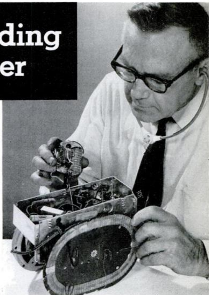
USED WITH HEADPHONES as a tracer, you actually hear the broadcast in the circuits if they are working
