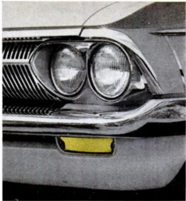
EVERYBODY'S DOING IT on the '63 models; all front turn signals will be amber for greater visibility
