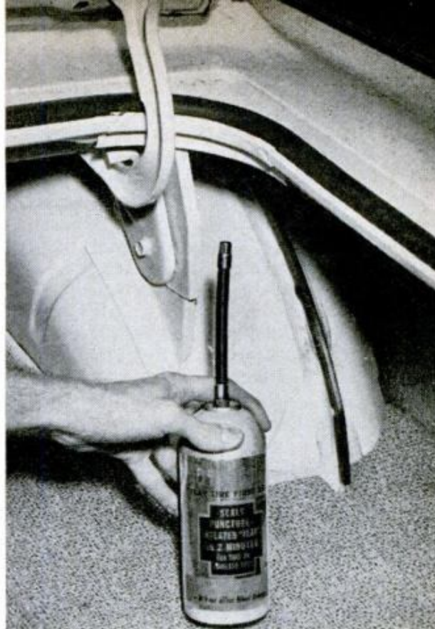
BEGINNING OF THE END for the spare tire; you may see the emergency pressure-can inflator on one model
