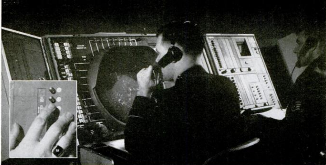
2 When blip can't be identified, scramble button is pushed (inset), alerting pilots. Planes are actually flown by this weapons team consisting of Canadian intercept director (left) and American technician
