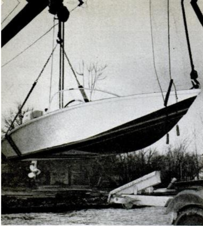
ON THE HOIST , PM-38 displays the planing hull lines which make possible high speeds with small motor
