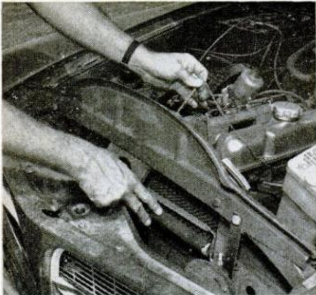
NEAT ITEM for Scandanavian (or Midwestern) winters is the roller blind that shuts off radiator with the simple pull of a chain from the driver's seat
