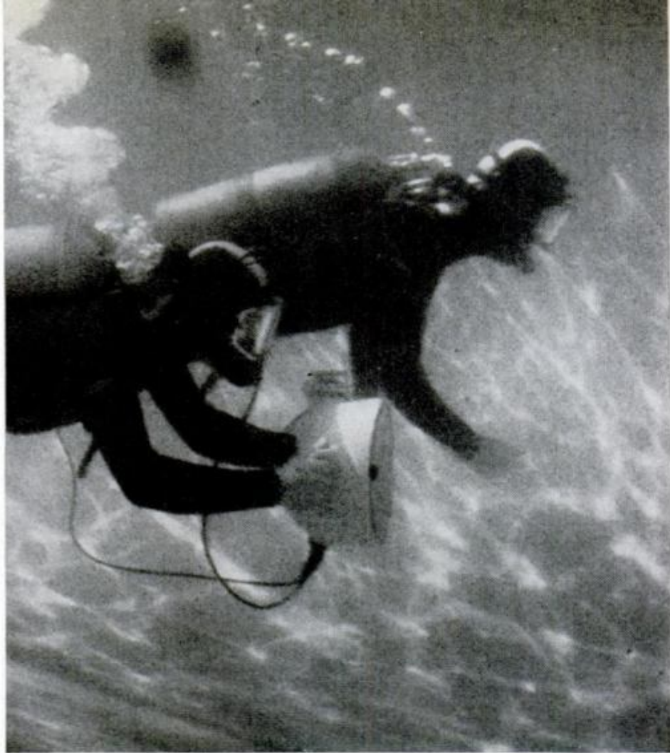
DIVER-HELD SONAR senses objects up to 120 yards away. Self-contained unit has two sets of earphones for two divers; three-position switch for range settings; is pressure resistant to 200-foot depths
