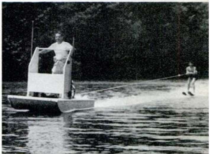
SCOW HULL is very fast when planing. With a 15-hp. motor, you can even use it for water skiing
