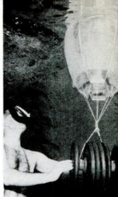
HIGHLY MANEUVERABLE diving plane (left, above) lets a towed diver "fly" through water behind a boat. Flexible planes are controlled by an aircraft-type joystick. Simple lifting "balloon" (right, above) is a strong plastic bag which is tied onto a find, then inflated from diver's air supply or from a separate tank. Easier to use than makeshift oil-drum floats, the bags come in sizes to lift weights from 100 to 1000 pounds
