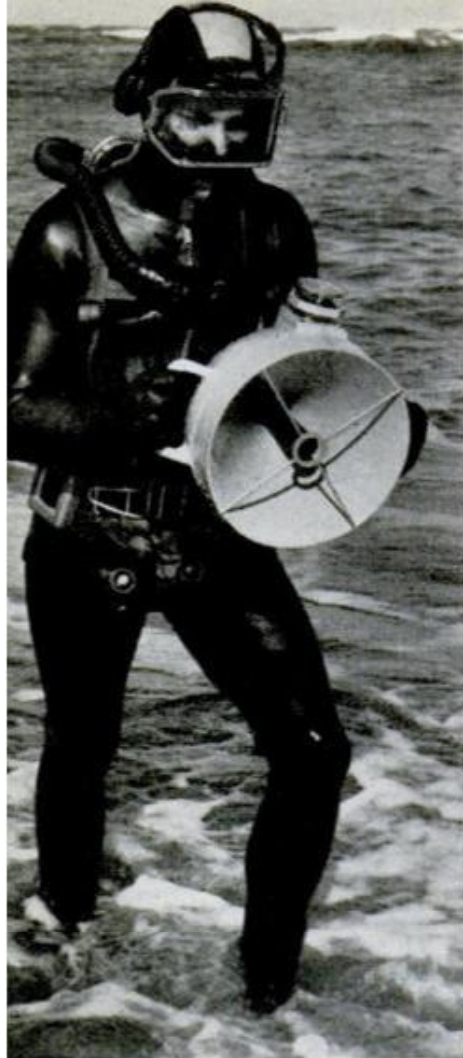
DIVER-HELD SONAR senses objects up to 120 yards away. Self-contained unit has two sets of earphones for two divers; three-position switch for range settings; is pressure resistant to 200-foot depths
