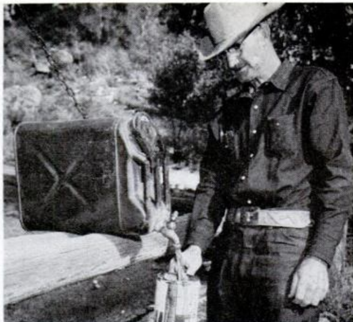
ORDINARY FAUCET , welded onto jerry can, saves pouring and keeps fresh drinking water "on tap" in camp
