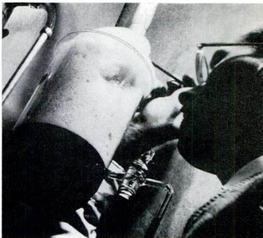
FOAM FRACTIONATION , a means of ridding water of detergent waste, is explored in Esso laboratory. Air is introduced in tubes, left, and rising bubbles carry chemical waste to top, as at right. Foam is then drawn off
