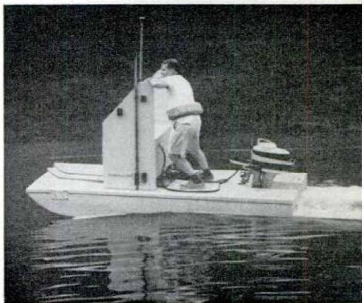
BALLAST STEERING adds new excitement to just plain boat riding. Manual steering is used at slow speeds
