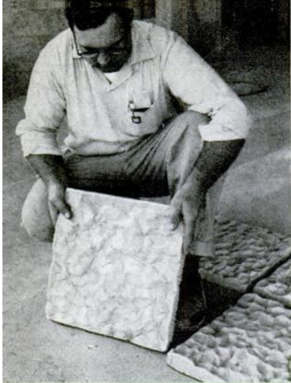
CASTINGS made in this fashion can be used as flagstones or, with a little ingenuity and imagination, they can be used as pattern insets in a retaining wall of blocks or other masonry
