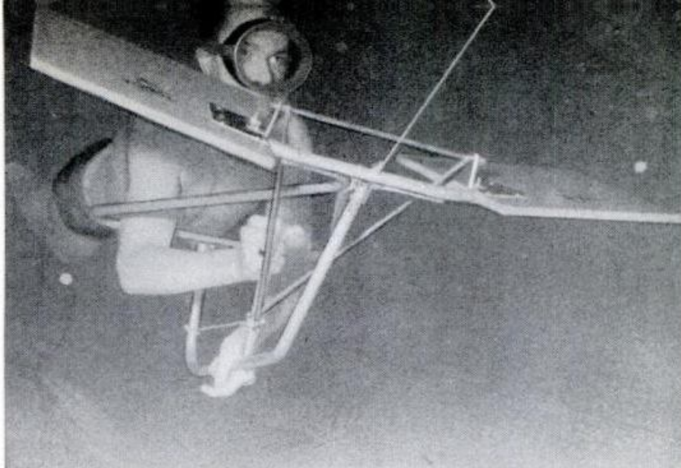
HIGHLY MANEUVERABLE diving plane (left, above) lets a towed diver "fly" through water behind a boat. Flexible planes are controlled by an aircraft-type joystick. Simple lifting "balloon" (right, above) is a strong plastic bag which is tied onto a find, then inflated from diver's air supply or from a separate tank. Easier to use than makeshift oil-drum floats, the bags come in sizes to lift weights from 100 to 1000 pounds
