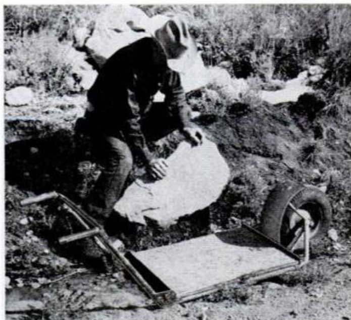
LOW-DOWN wheelbarrow simplifies handling heavy rocks; ground-level bed eliminates lifting and carrying
