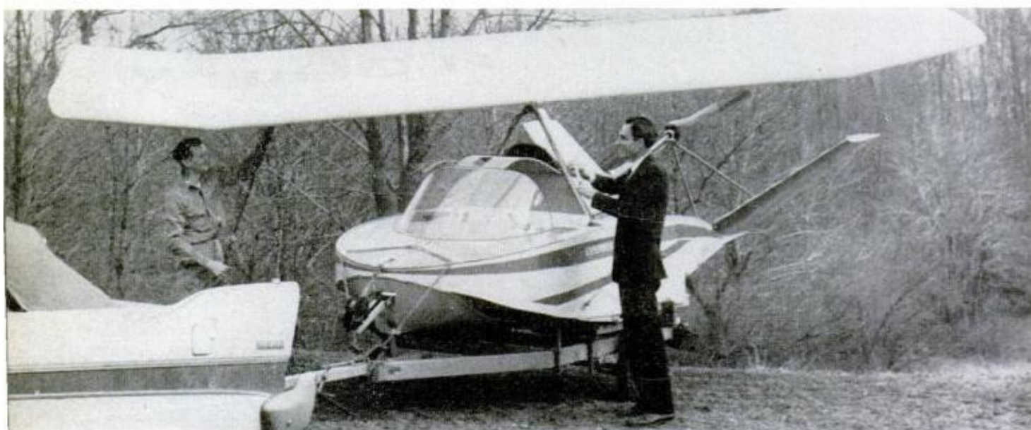
2. AT WATERWAY , wing is easily set in place and secured with wire cables. It will now tilt or dip
