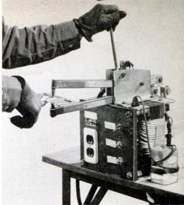
SWITCHES AND TAPS on insulating panel should be labeled for easy identification and to prevent error
