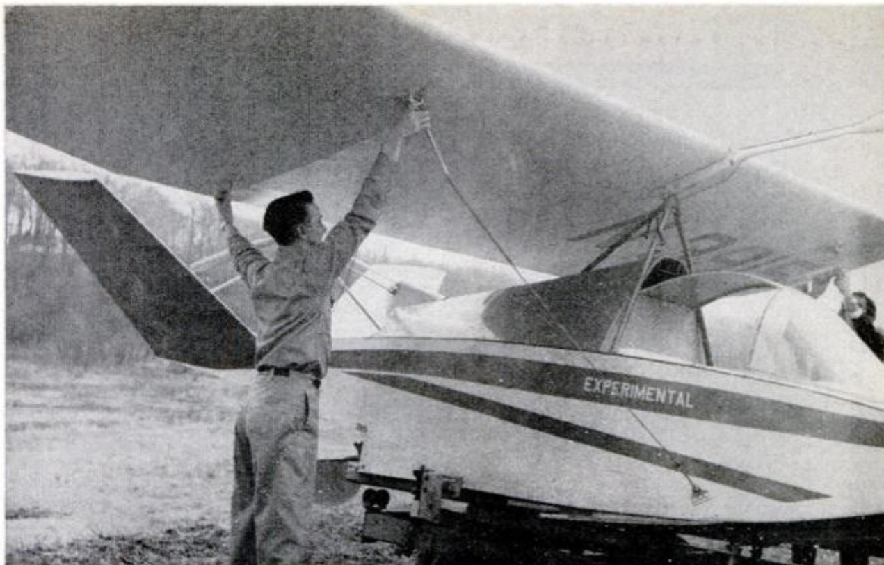
WIRE CABLES hold the wing in place for flight. The wing is anchored at the center post behind the cockpit. In production models, the builders plan to eliminate the cables, and control the wing entirely from the post
