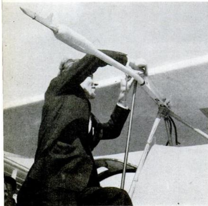
PITOT TUBE , located on wing directly above cockpit, is standard equipment on aircraft. Its air intake is translated into air speed which is shown on air-speed indicator in cockpit
