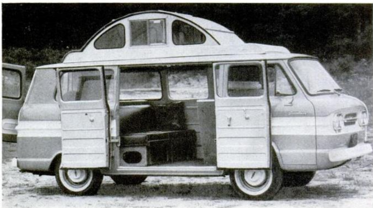
TRAVEL TOP RAISES in a jiffy to over six feet of stand-up space. Sliding windows in dome have screens
