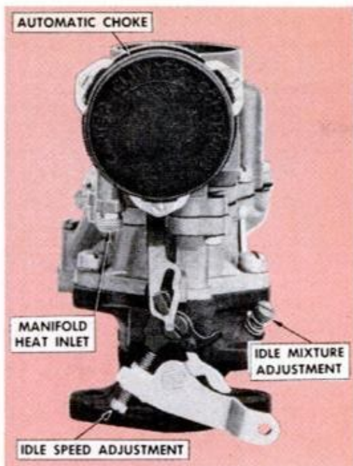
SINGLE-BARREL CARB , above, is standard on 4s and 6s. Right, if used regularly, carb detergents will dissolve gum deposits
