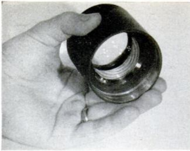
METROGON LENS has good correction for flatness of field over large angle, and is perfect for projector
