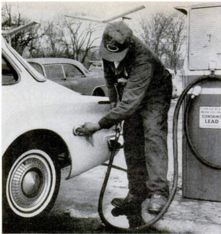
VALIANT'S HORIZONTAL FILLER neck has been regurgitating fuel on fenders for 2½ years now, to the tune of owner protests
