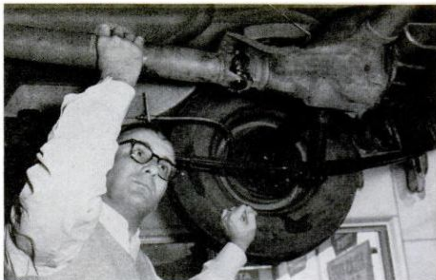
COUNTING DRIVE-SHAFT TURNS per revolution of wheel to check rear axle ratio might well be standard procedure for owners getting unaccountably low fuel mileage or poor performance. Valiant had proper 3.23:1 gearing
