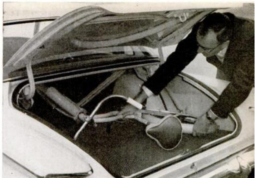
VALIANT'S TRUNK swallowed bike with 20-inch wheels, thanks to its high forward end, plus spare tire buried under floor
