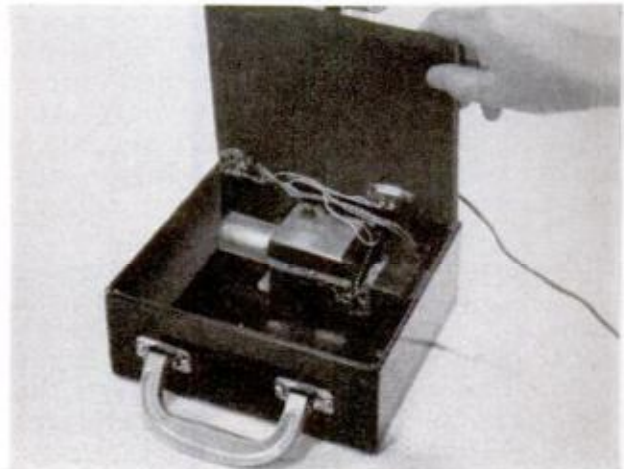
ALL PARTS of enlarger, including lamphouse, pack into carrying case, or box, as in photo above. Below, you see electrical parts which remain in box in use
