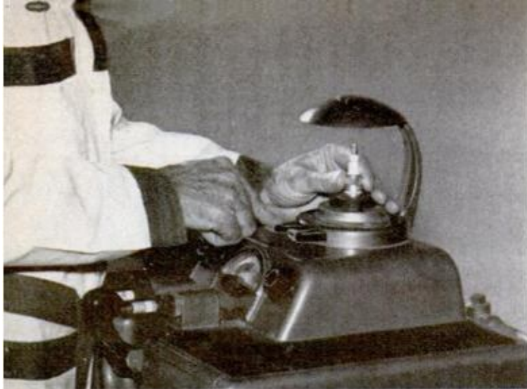
8. MECHANICS CLEAN plugs by sandblasting on a machine like that pictured. Unit does thorough job
