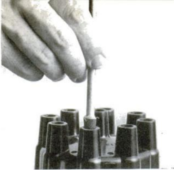
11. CLEAN DISTRIBUTOR towers with a brush made for the purpose or with sandpaper on dowel
