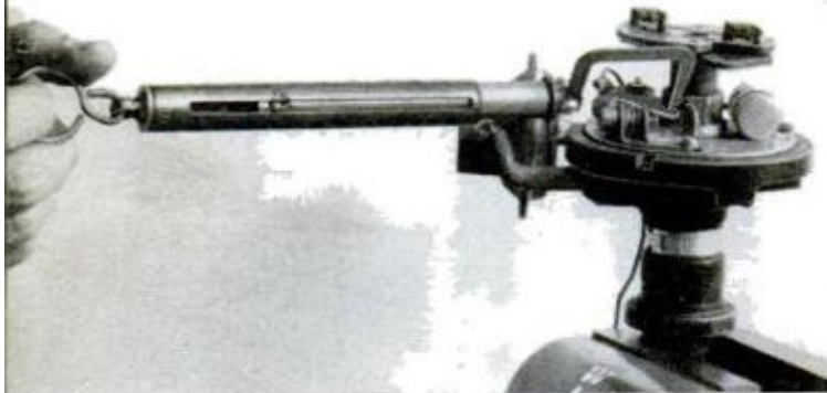
13. CORRECT POINT TENSION is necessary to prevent point bounce. Tension scale gives accurate check
