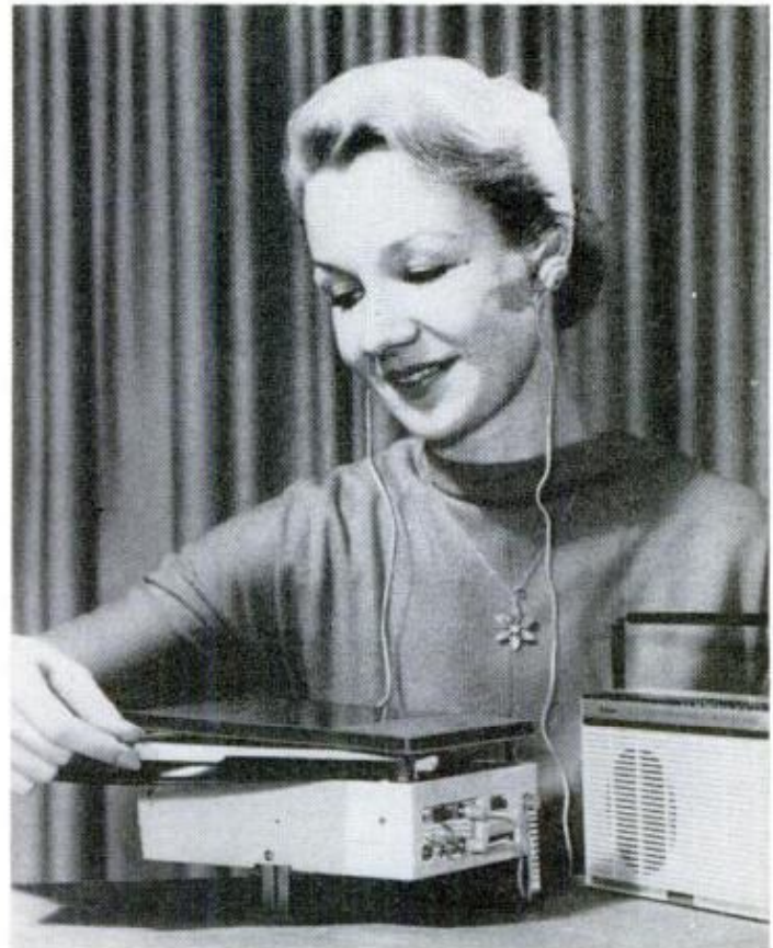
TRANSISTORIZED STEREO PHONO and AM-shortwave radio plays through speaker or stereo earphones; runs on flashlight batteries. Portable unit costs $79.95 from the Hoffman Electronics Corp., 3761 S. Hill St., Los Angeles 7
