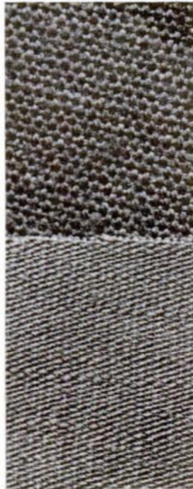
SHELL FABRIC needs high thread count; lower sample is best
