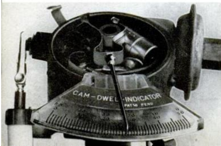
14. INEXPENSIVE CAM-DWELL indicator of mechanical type permits cam adjustment in car or at the bench
