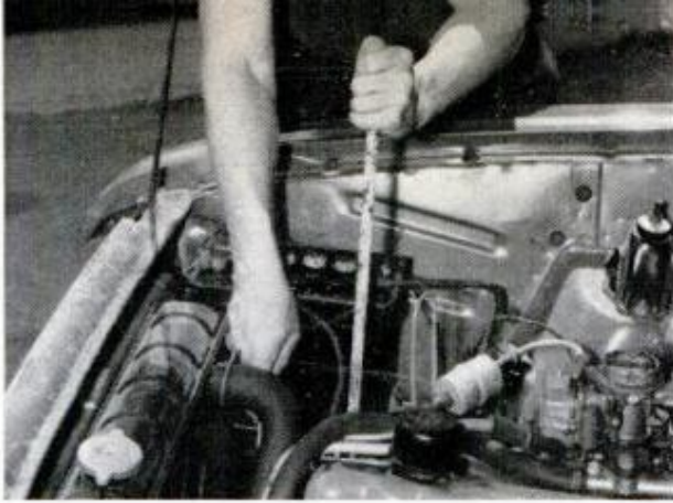
13. WHEN TIGHTENING fan belt you may need a pry bar to hold generator while you tighten the bolt
