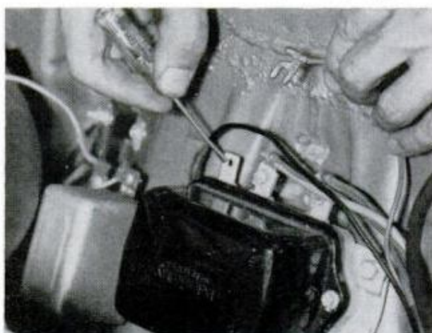
10. CLEAN ELECTRICAL CONNECTIONS are critical in wiring. Take time to do a thorough job of cleaning
