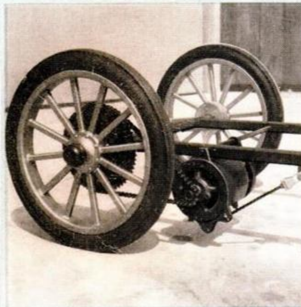
2. CHAIN DRIVE transmits power from the motor to the large sprocket mounted inside the right rear wheel
