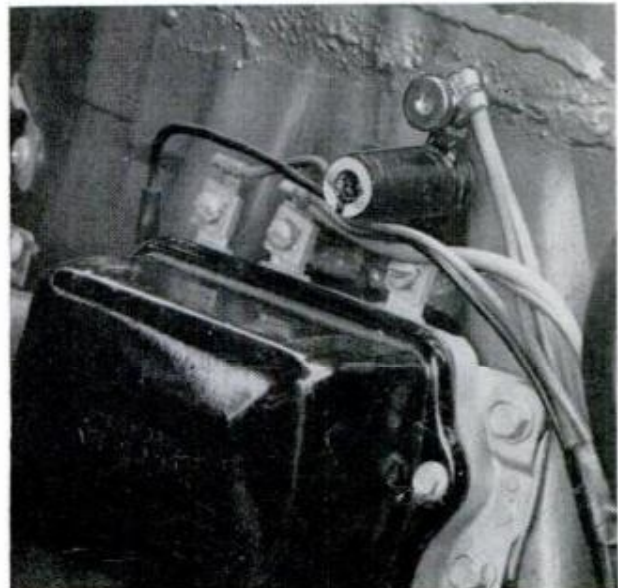
6. RESISTOR of 1/4-ohm capacity assures correct regulator adjustment when used with test equipment
