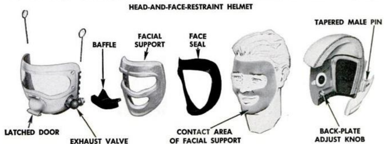
FACE MASK, shaped by making a plaster cast impression of the pilot's face, provides a sealed compartment
