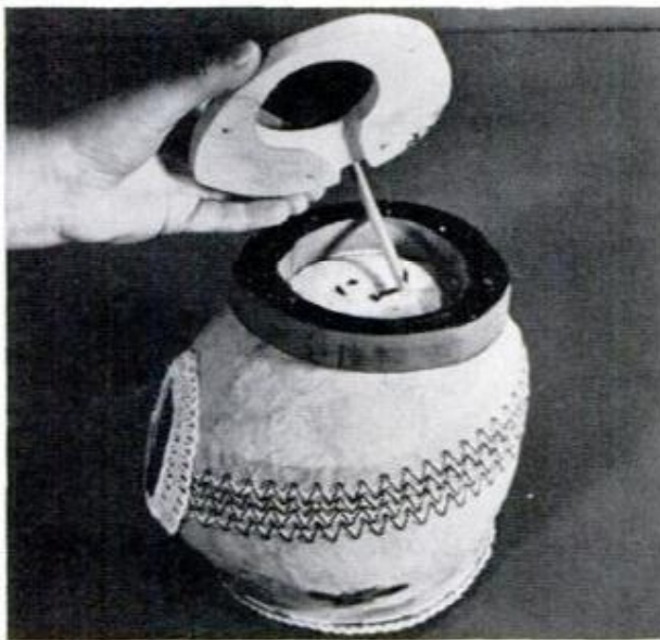
DOWEL CRANK has a hole drilled in one end to hold the bent end of the wire axle which turns the disk
