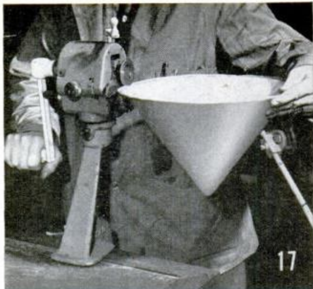
STANDARD ROTARY MACHINE is regular equipment in most sheet-metal shops. Here an edge is wired
