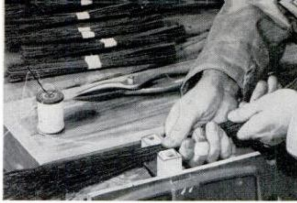
BROOM STRAWS are bundled in jig, then taped and sewed. Keep bundles as nearly uniform as possible
