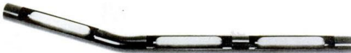
SILENCING SYSTEM installed on T-Bird (top) has no conventional mufflers. Cutaway above shows resonators
