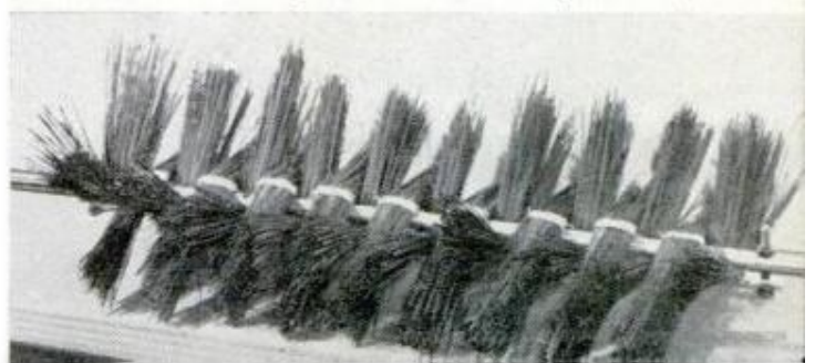
ONLY WHEELS and wheel plates of original mower are used, as pictured at the left. Below, partially assembled brush with all bundles in place ready for placing the second angle which forms complete hub
