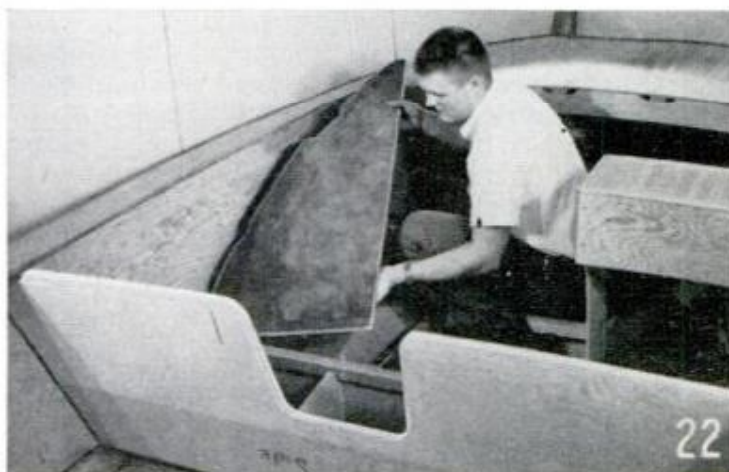
FORWARD FLOORBOARD panels must be cut to follow the curve of the hull but shouldn't come in contact with the planking
