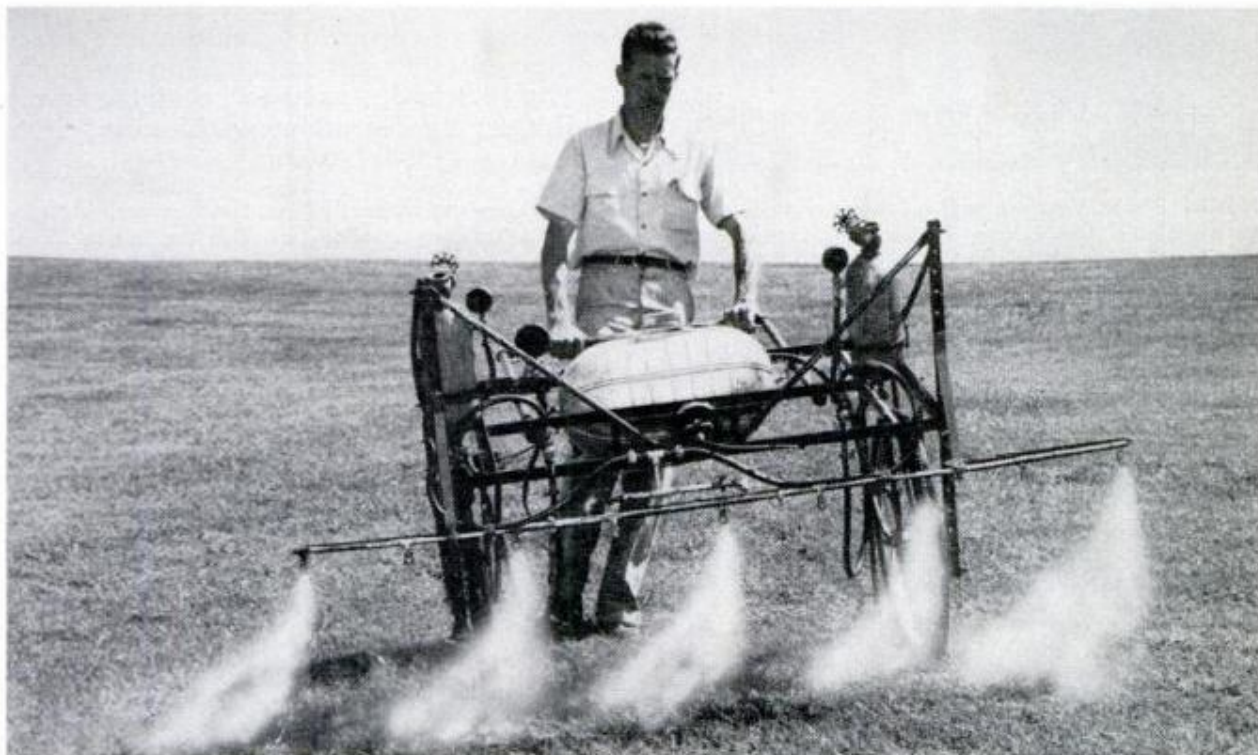
FIELD TRIALS also include use of experimental spraying equipment such as this vehicle. Air tank forces spray
