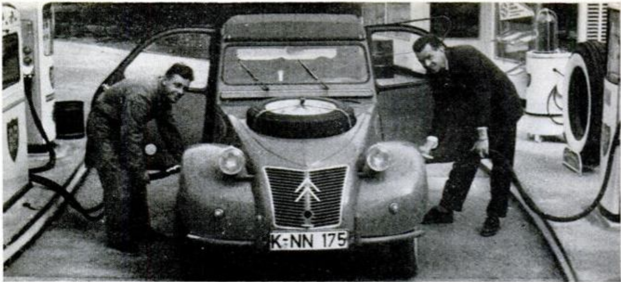
DOUBLE-THINK is needed when refueling twin-engined Sahara as each engine has its own under-seat tank
