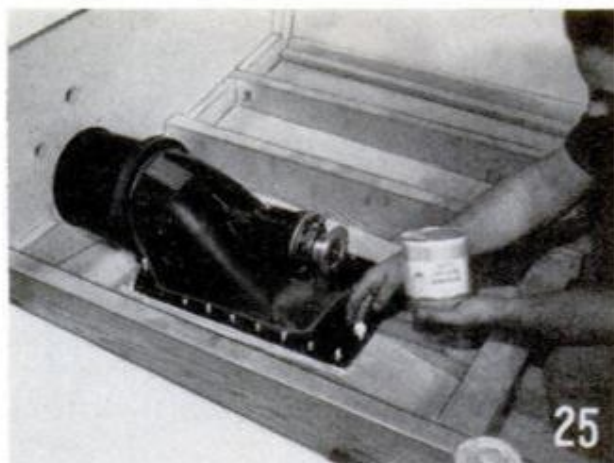
BEDDING COMPOUND must be used when installing the jet unit and at all other through-hull fastenings
