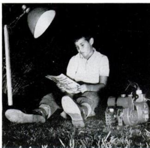
CAMP LIGHT is powered handily by 200-watt plant. In use, it would be stashed in woods out of hearing
