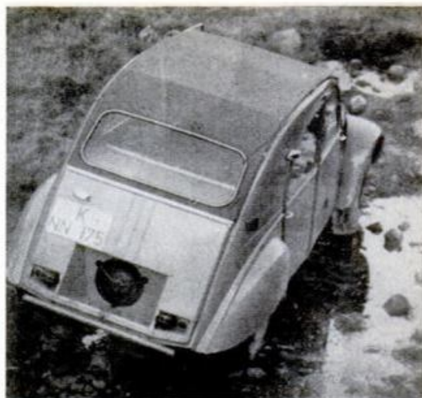
SECOND ENGINE drives the car's rear wheels and "breathes" cooling air through port in the trunk door
