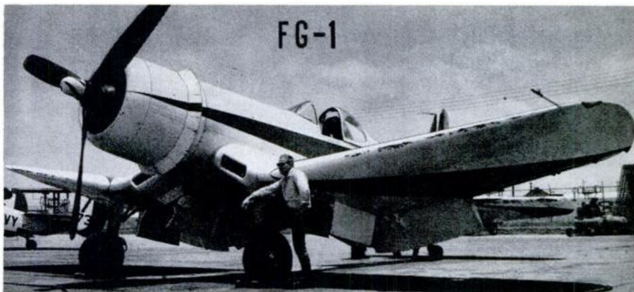
GOODYEAR FG-1 "CORSAIR" (same as Marine's F4U, but without the folding wings) is private "runabout"
