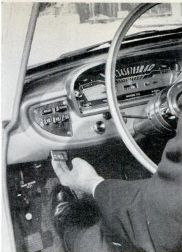
SLIDING PULL-TAB is used for PARK while other automatic transmission controls utilize push buttons
