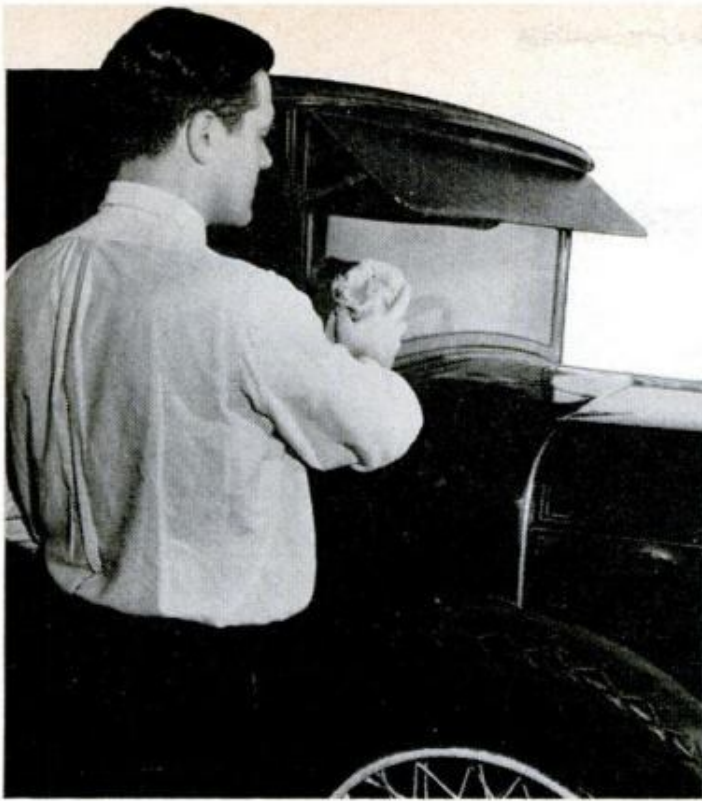
WHEN A SUN VISOR was really a visor, as on this 1928 Franklin, it was outside the car body, and helped keep snow off in winter as well as blocking glare. Most cars of the '60s could use a similar device
