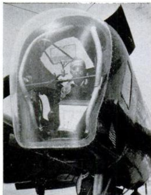
P-38 NOSE, that once held cannon, machine guns, now carries aerial camera
