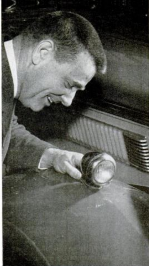
FENDER LAMPS like this on 1936 Horch (German) were almost universal in 1930s. They'd be great on today's cars as ultra-visible directionals as well as for parking
