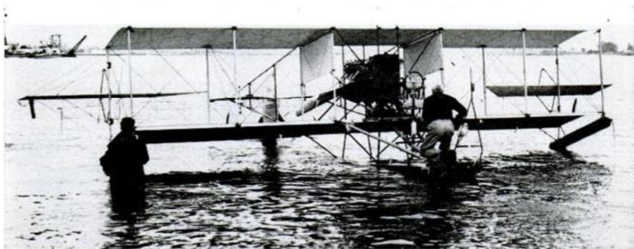
CURTISS BIPLANE , rebuilt from original plans, takes to the air where prototype flew some 50 years before A-1 REPLICA weighs 1500 pounds fully loaded. Powered by 1913 engine, it got up to speed of 60 m.p.h.
