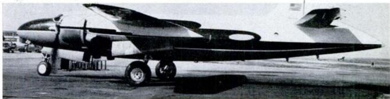
MARTIN B-26 "MARAUDER," medium bomber, was converted by commercial firm into an executive plane
