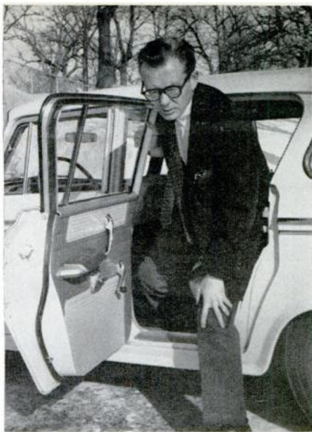
UPPER REAR CORNER of Rambler's back-door window frames has been rounded off from '61's sharp points
