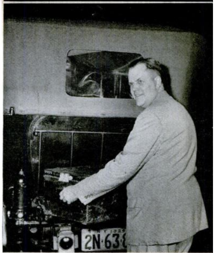
MANY MOTORISTS today could use a real trunk rack like the one on this 1915 Belgian Minerva. The vertical cylinder at lower left of picture is a shock absorber that operated by compressing trapped air
