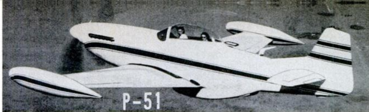
NORTH AMERICAN P-51 "MUSTANG," famed long-range fighter is converted into a tandem-seat executive
