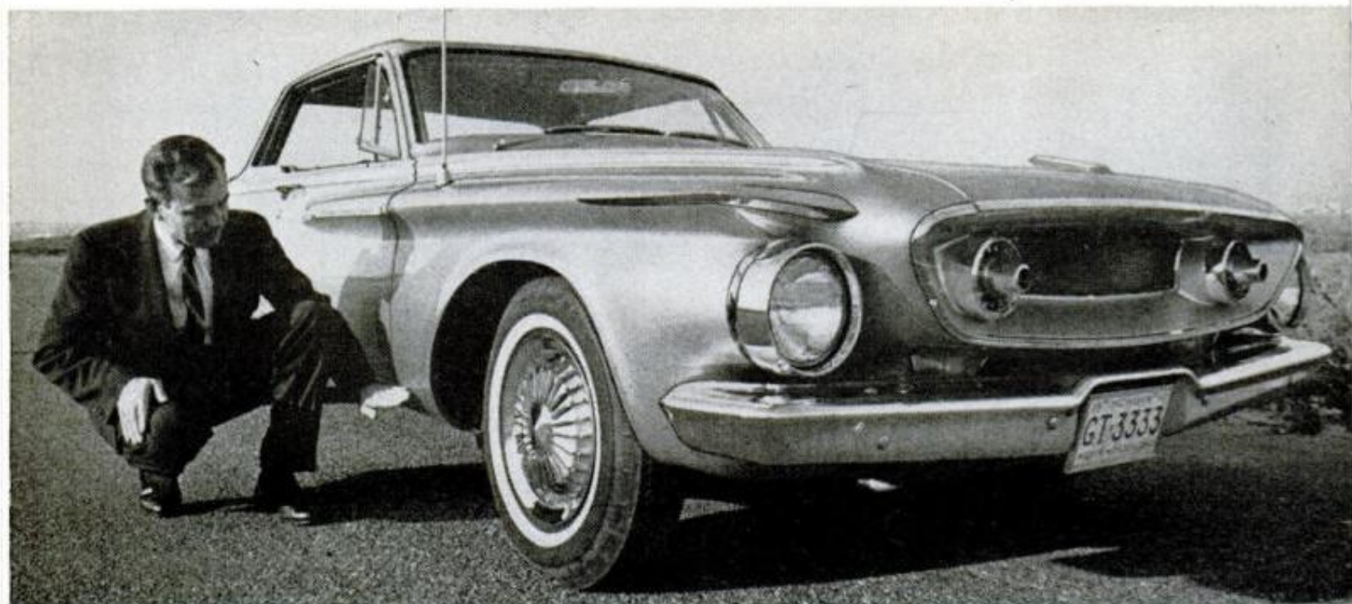
FEELING 200-DEGREE-temperature exhaust, which comes out under front wheel wells on prototype models
