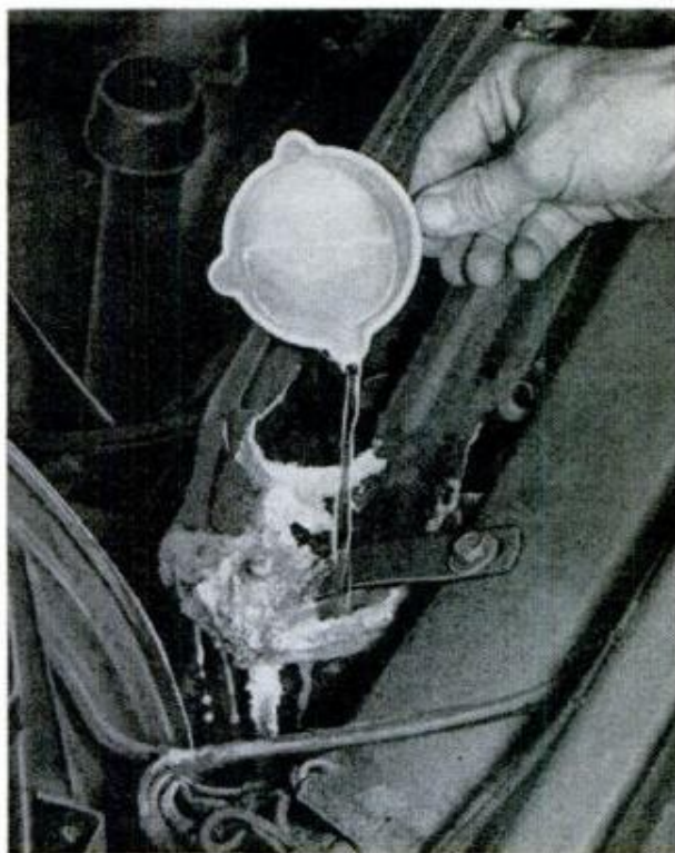
9. SODA-WATER SOLUTION poured or swabbed over corroded battery and rack removes the coating. Use about one teaspoonful of soda in a pint of water. After cleaning, coat parts with petroleum jelly
