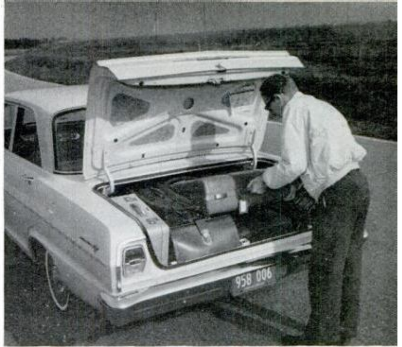
LOW RIM makes loading of the trunk easy, but full use of the space is hampered by a flat-mounted spare
