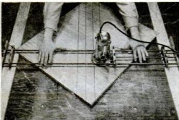
8. NOTCHED GUIDE STRIPS are used to hold work for diagonal spaced cuts. Slide supports ride guides
