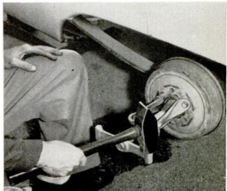
10. SPECIAL PULLER of this type assures easy removal of parts without damage to rear axle or differential
