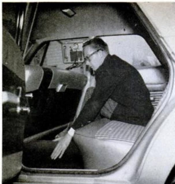
LOWER TUNNEL shows real efforts to cut it down in '62; owners' beefs are fewer than on '60 Plymouth
