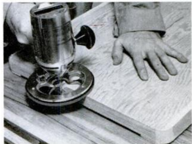
ALL SHARP EDGES of the belt-massager platform should be rounded to avoid slivers, and then sanded
