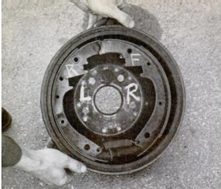
5. CHALK-MARK all parts of each brake unit as they are removed and replaced to keep them in sequence
