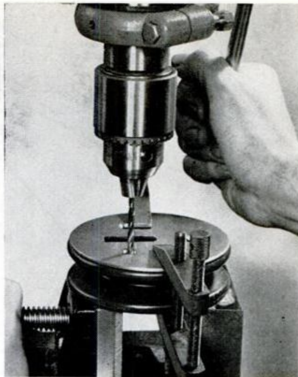
WITH SLOT ALIGNED with pulley keyway, crankplate is clamped to pulley and holes are drilled through
