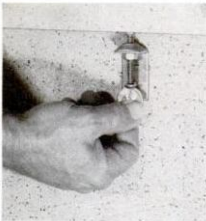
SWIVEL CASTERS , two with brakes, are attached to leg cabinets as in photo at left and center detail. Right-hand detail shows how levelers are attached to leg cabinets. Four identical levelers are needed
