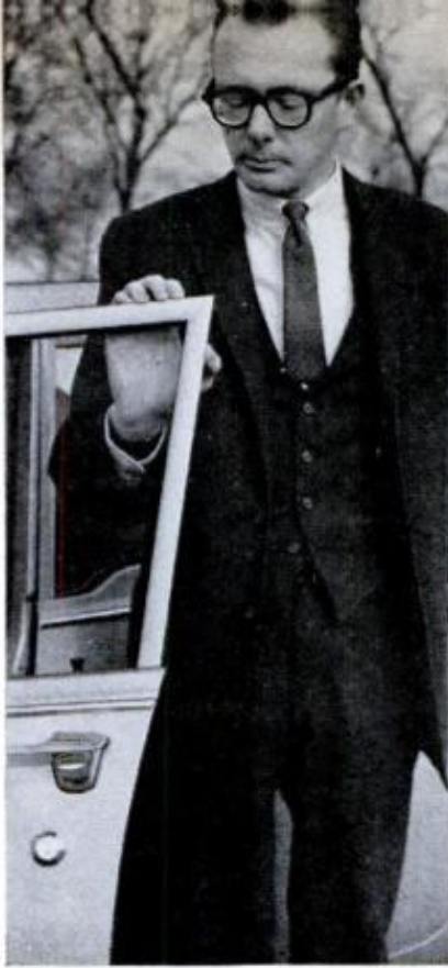
DOOR FRAME CORNERS can scratch, snag clothes, some owners said. Right, rear door has full exit room but sill is high
