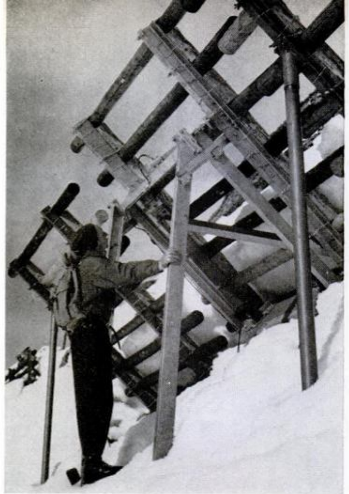
SNOW FENCE , an experimental avalanche retainer, is one of variety tested at Weissfluhjoch, Switzerland
