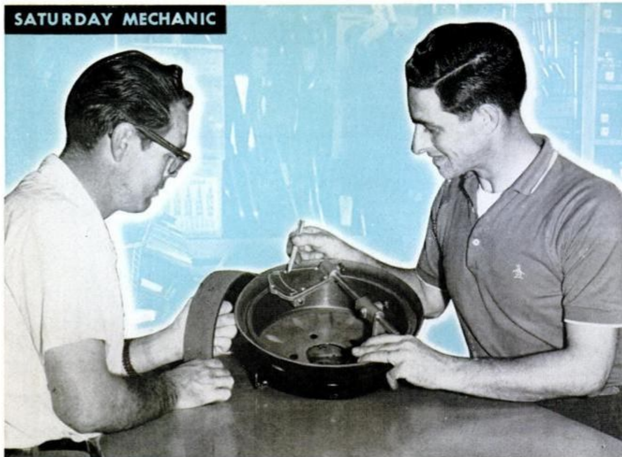
1. BRAKE DRUMS that may be defective should be checked by your parts dealer with a brake micrometer
