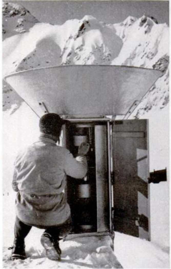
MEN OF WEISSFLUHJOCH measure snow pressure and density on instruments spaced around three miles of mountainside. Right, avalanche researcher monitors precipitation meter; it registers snowfall electronically
