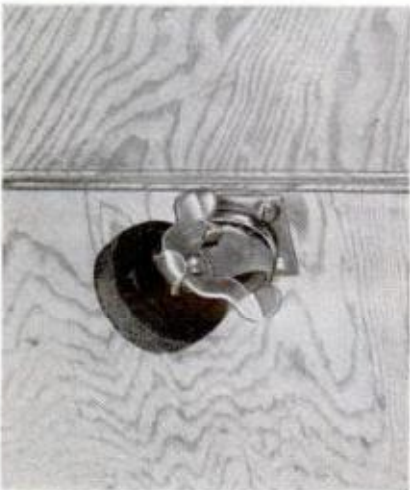
SWIVEL CASTERS , two with brakes, are attached to leg cabinets as in photo at left and center detail. Right-hand detail shows how levelers are attached to leg cabinets. Four identical levelers are needed
