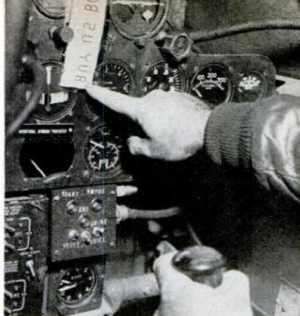
JOB "STRIP," mounted vertically in lead-plane cockpit, corresponds to pattern flown by formation
