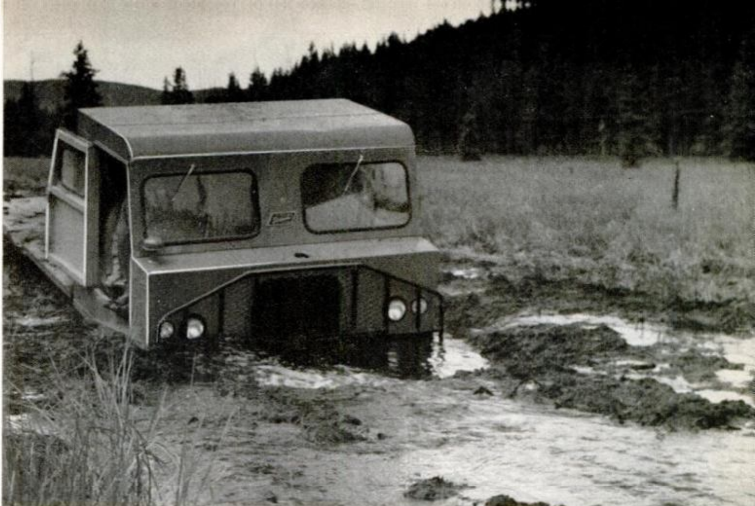
MUSKEG BUGGY sloshes its way through shallow area of muskeg. Normal vehicles would disappear in muck
