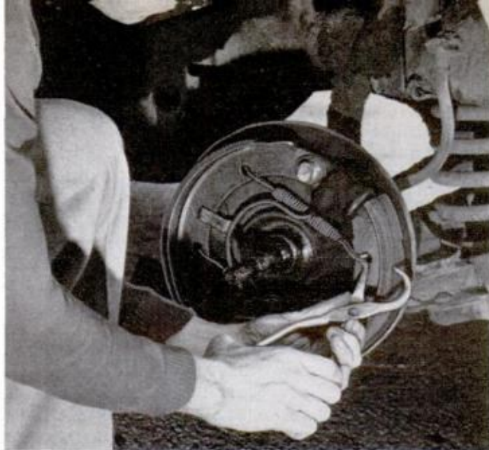
6. SPECIAL BRAKE TOOLS , made for the purpose, will save a lot of time when removing or installing shoes
