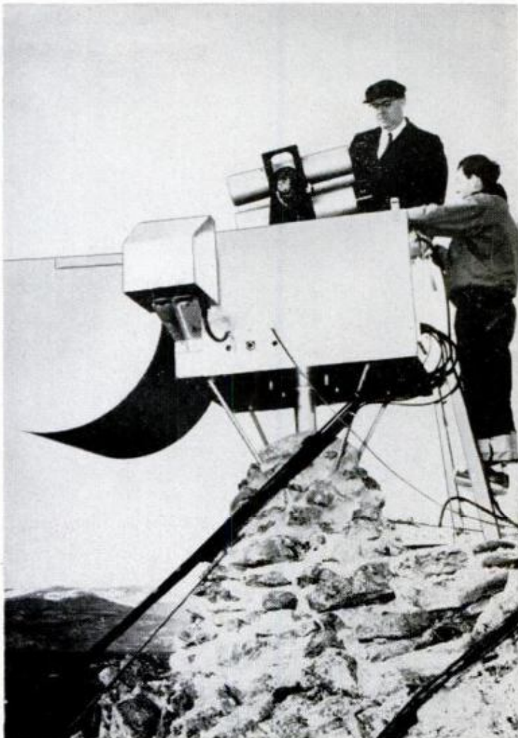
JET PILOTS climb treadmills 14,000 feet up at Mt. Evans, Col., to build tolerance for high-altitude work. Photometer, right, measures sky glow, a phenomenon of outer atmosphere, from Fritz Peak, Colorado
