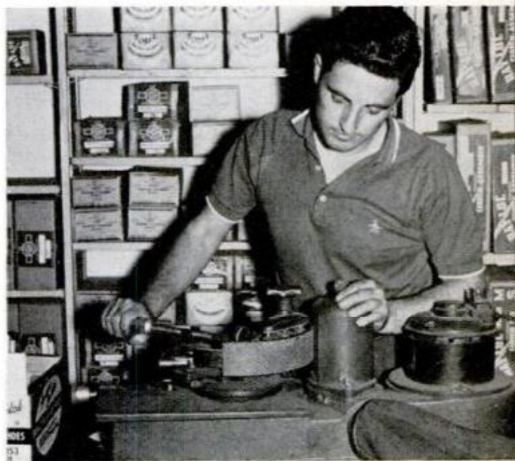
4. BRAKE-SHOE LININGS are arced to concentricity with drums on a machine designed for the purpose
