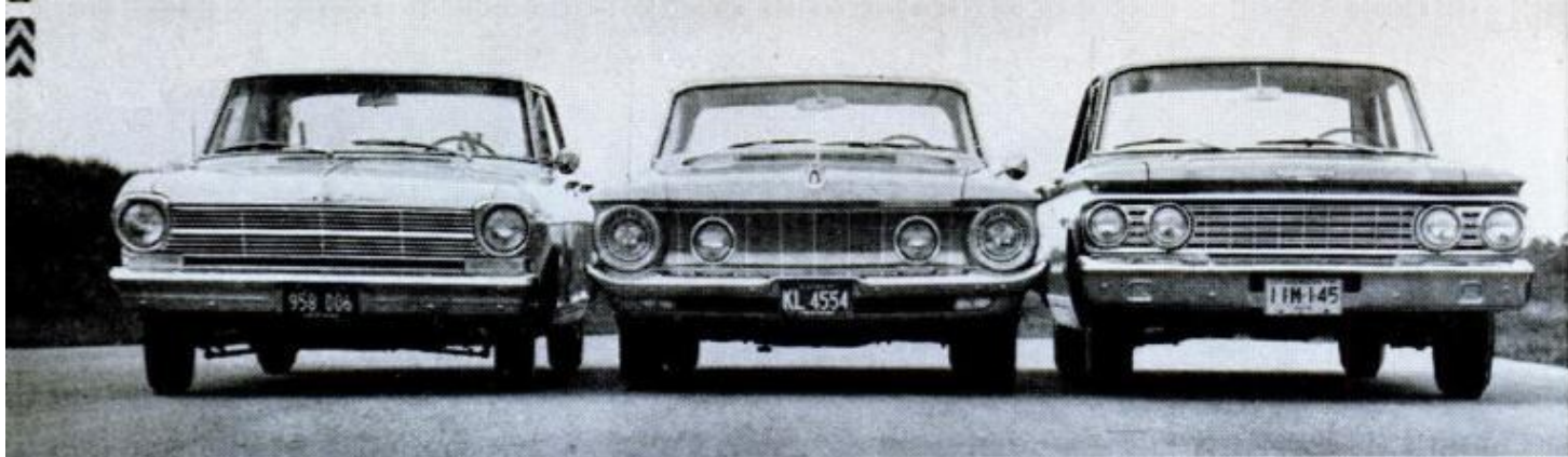
PLYMOUTH'S SLOPING HOOD stands out when parked between high, boxy Fairlane, right, and compromise angled, shorter hood of Chevy II. Ground clearance is about equal but for 5½-inch height of Chevy II's tie rods
