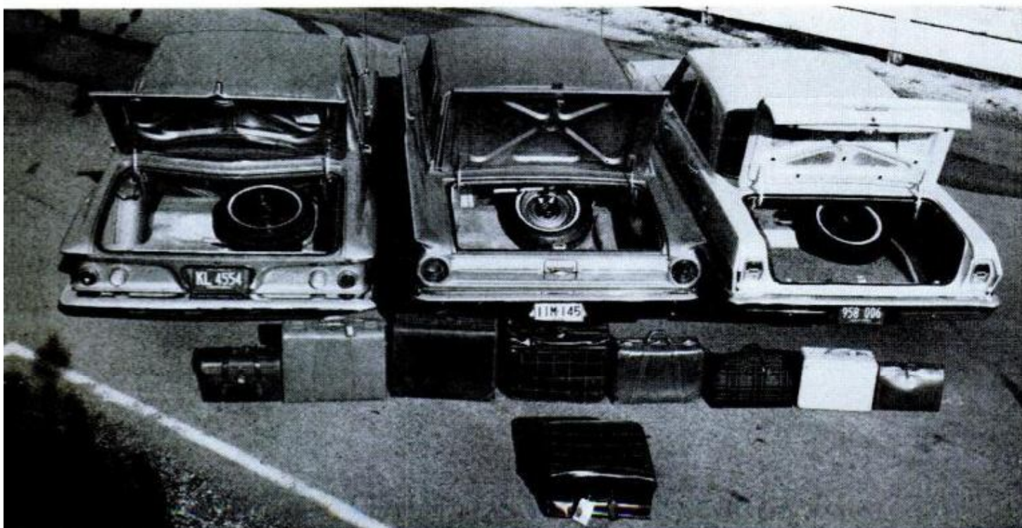
ALL OF THE BAGS SHOWN above were packed into the trunks of both the Plymouth, left, and the Fairlane, center. Chevy II's trunk, right, held all the baggage except the large suitcase shown in the foreground
