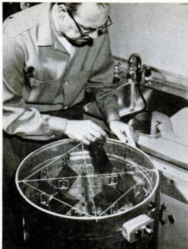
1. DRYER handles twenty-four 4 x 5 cut-film negatives or several film strips on upper, lower hangers
