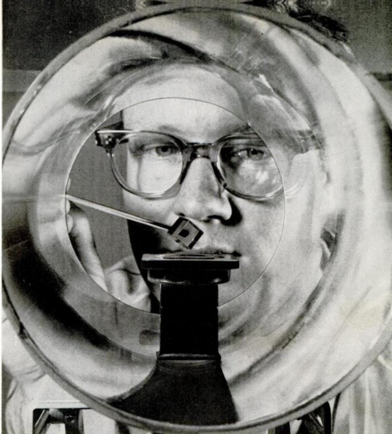
LASER research: A synthetic ruby crystal is tried in a wave guide component to add power to fantastic beam
