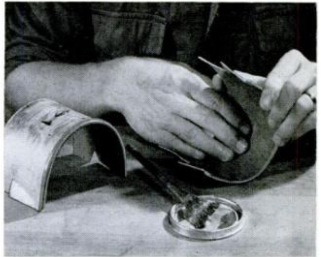
CORNER AND SIDE-POCKET LINERS are made from No. 2½ tin cans lined with a flexible countertop material
