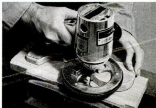
SIDE MEMBERS of rowing seat are jigsawed to shape (above), then shaped (below) to relieve all sharp edges. All four side members extend below rails to keep seat from coming off the track as it rolls
