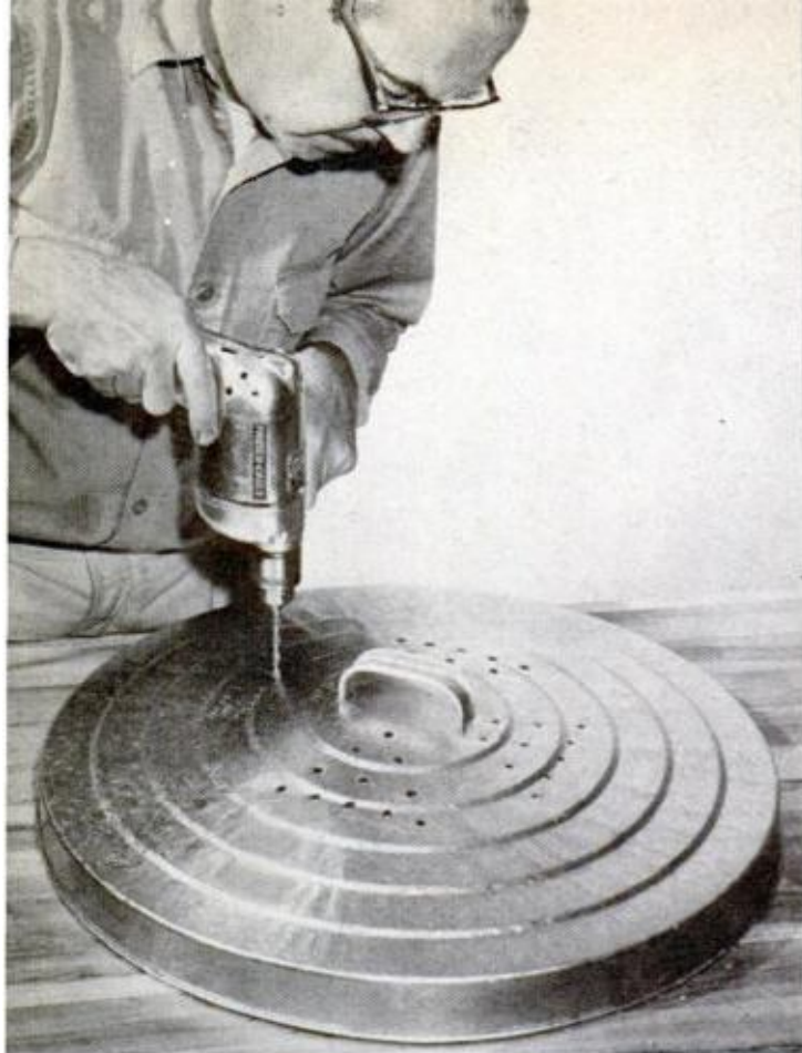
6. HOLES IN a V-shaped pattern are drilled through can cover. Deburr with reamer to prevent hand injury
