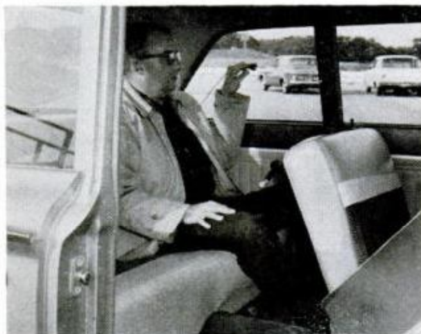
REAR SEAT RAISED well above floor in Fairlane makes seating comfortable. Tunnel is relatively low
