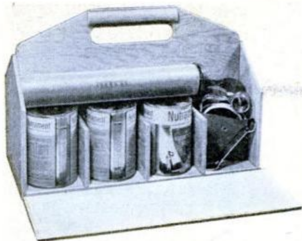
ATTACH HANDLES to the center panel, above, before assembling the kit. The inside of the box, below, should be finished before adding the sides and lids
