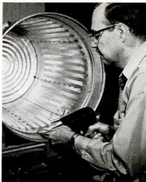
11. HEATING TAPE , above, is plugged into wafer-type outlet. Right, solder spots being sweated onto can
