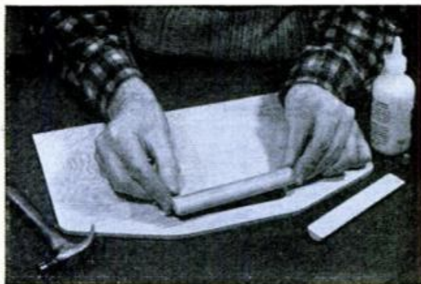
ATTACH HANDLES to the center panel, above, before assembling the kit. The inside of the box, below, should be finished before adding the sides and lids
