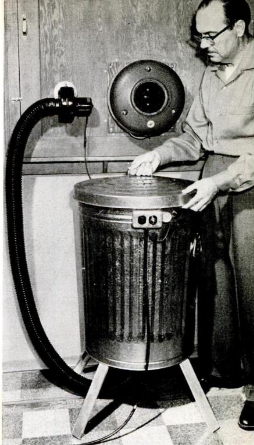
5. AIR OUTLET , above, left, is soldered into hole in bottom of can. Above, right, the finished film dryer
