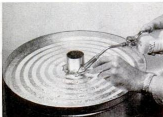
8. AIR OUTLET , Fig. 5, is soldered into hole cut in bottom of can. Outlet is covered with 1/16-in. felt
