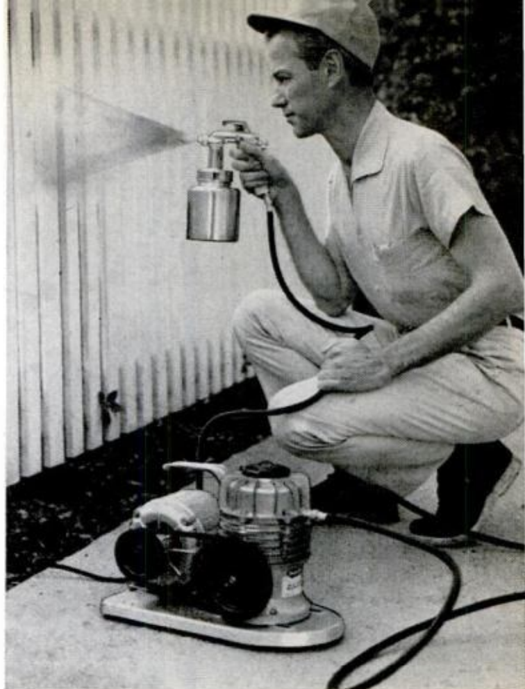
6. EVER BRUSH-PAINT a picket fence? Then you can appreciate the speed and ease with which a spray unit gets the job done—on both sides of fence, too
