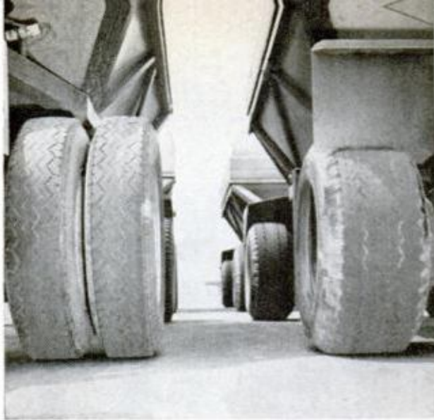
WIDER, EXTRA-STRONG supertires, right, replace conventional duals as shown on cement-hauling truck
