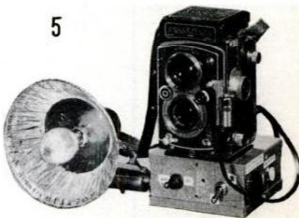
SOLENOID IS BEING USED when box is mounted on the base of an old model Rolleflex. If additional side lights are desired, they may be connected through box
