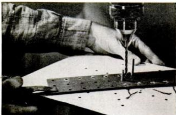
PERFORATED HARDBOARD template must be clamped so it cannot shift while each set of holes is drilled
