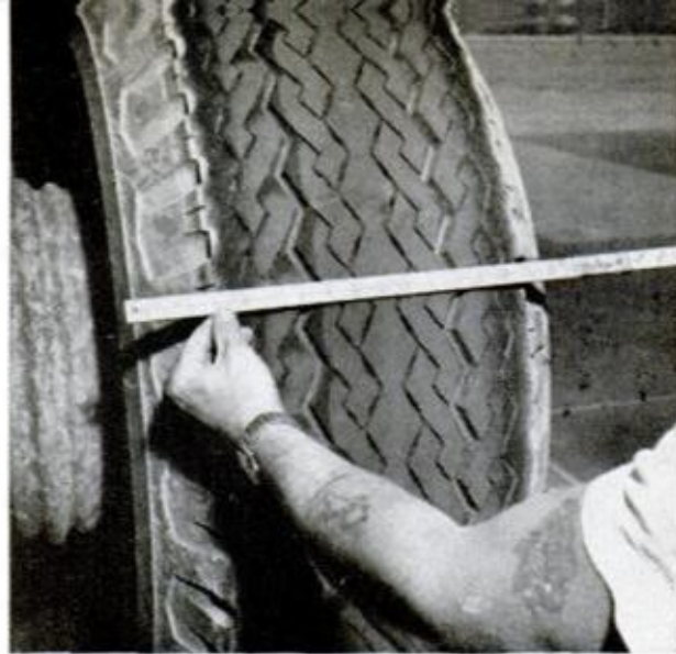
"SUPER" PUTS 12 inches of tread on the road as compared to only 15 inches for two tires it replaces
