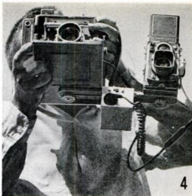
IF YOU WISH to take color and black-and-white shots simultaneously, you can mount a second camera on a bar connected to the first and attach box between
