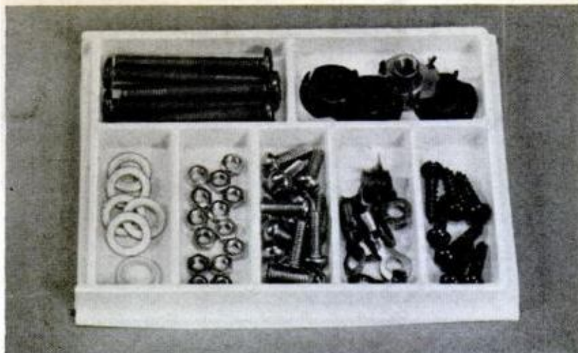
4. SMALL-PARTS TRAYS can be duplicated in vacuum-formed plastic. Or you can assemble a small tray from thin stock and use it as a pattern for forming any number of duplicate plastic trays
