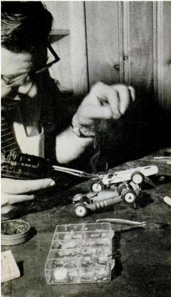
PLASTIC BODY and wheels are taken from kit, axles are specially made. Guide pin projects down, front
