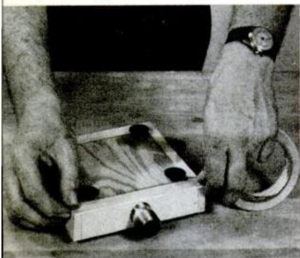
5. BOTTOM of vacuum box is plywood. It must fit tightly to prevent air leaks. Corners of box are made airtight with tape
