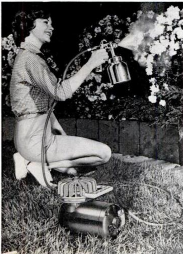
5. NEARLY ALL TYPES of sprayers can be used for spraying insecticides effectively. Gun is adjusted to give fine-mist spray pattern for full, uniform coverage
