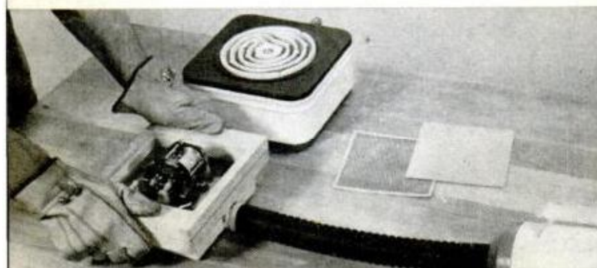
2. PLASTIC SHEET , above, is heated on both sides over electric plate to bring it to right degree of plasticity for forming. Then holder and sheet are placed over pattern on vacuum box. Air pressure, below, forces plastic into contact with pattern
