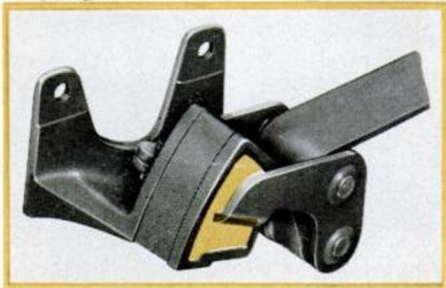
METEOR'S "Cushion Link" rear suspension recesses with horizontal bump thrust absorbed by arm embedded in rubber attached to swing shackle
