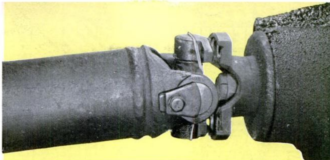
8. OPEN UNIVERSAL JOINTS on drive shaft need lubricating at 25,000 miles, or less. Before you loosen nuts have rubber bands at hand to hold parts in place. It's a good idea to have instruction sheet for your car
