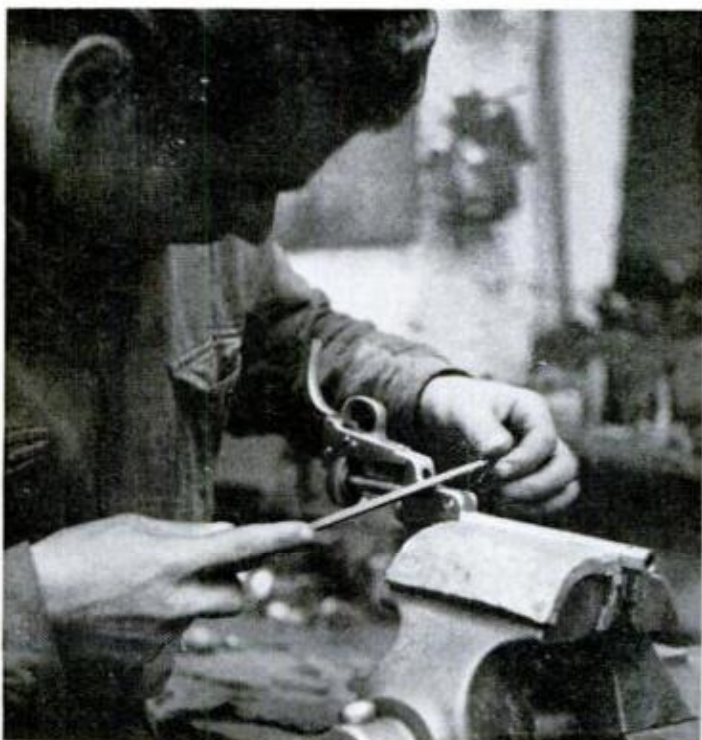
ITALIAN GUNSMITH files revolver frame. Forgett went to Europe to make replicas because of high labor costs in U.S.
