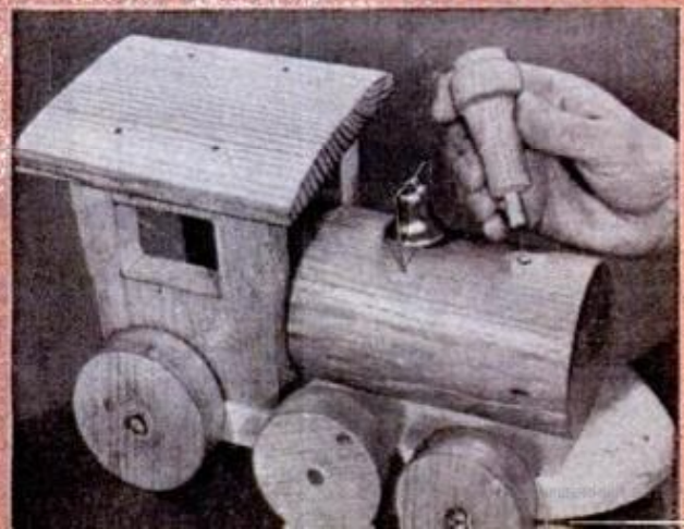
6. SMOKESTACK is turned to a diameter of 1\frac{1}{2} in. and pegged into the boiler ahead of the small bell
