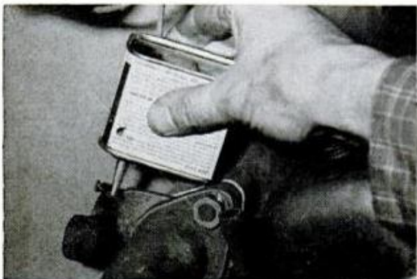
6. HEAT VALVE on exhaust manifold is another lube point that is easily overlooked. It should get regular attention. Use special oil to withstand heat
