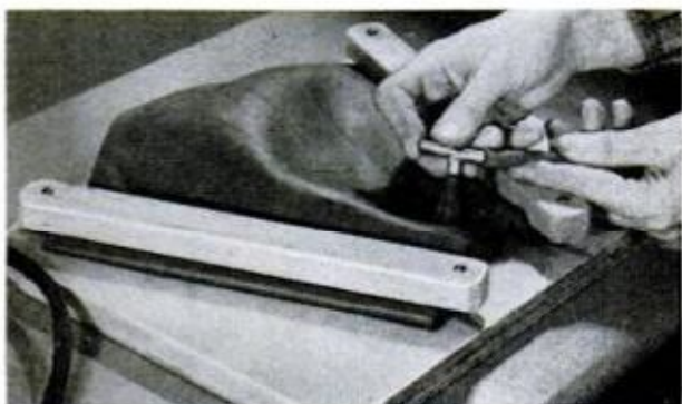
10. TEE CONNECTOR on the rubber air chamber is made from a valve cap and a piece of copper tubing. Syringe tubing connects the chamber to the bellows
