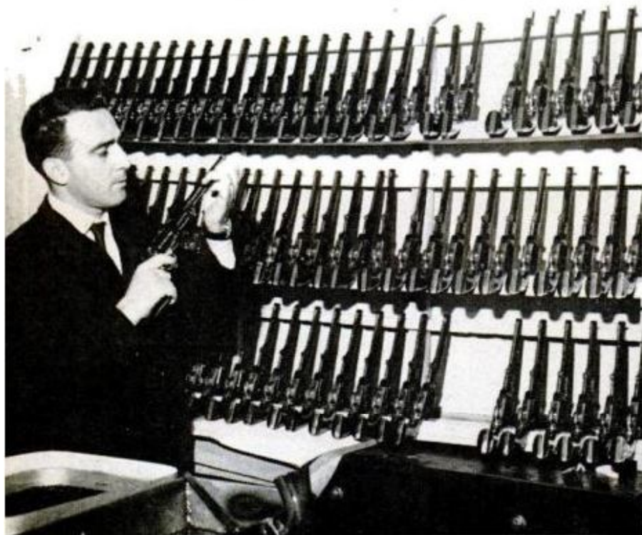
FINAL INSPECTION of pistols is made by Forgett's Italian agent. Guns are then dipped in tub of grease (left) to prevent rust
