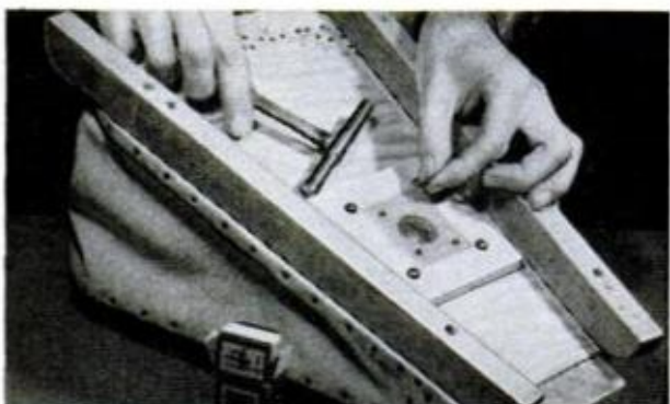
9. WIRE SCREEN over the inlet valve opening will catch small objects which might otherwise be sucked up through the valve and into the bellows chamber
