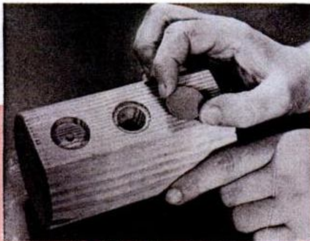
3. SOUNDING BOARD about the weight of a postcard is glued flush with surface over sound chamber
