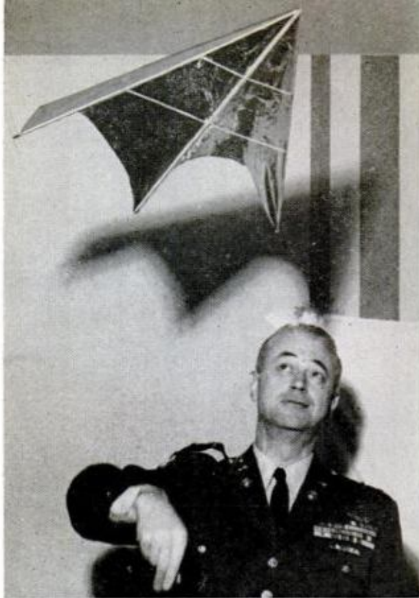
MODEL GLIDER , left, and full-scale craft, below, show arrow-head shape of Flex Wing design
