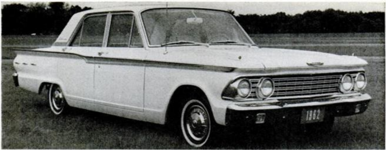
SOLID, SENSIBLE and conventional lines with typical Thunderbird roof profile mark Fairlane 500 for as one of the Ford family. The wheels are 13-inches, tires 6.50, and brake drums are 10 inches in diameter
