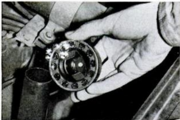
5. BREATHER CAPS get too little attention. They're really filters and should be serviced regularly. It takes a thorough cleaning to remove dust and sludge
