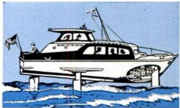
PROPOSED TURBINE-POWERED hydrofoil cruiser, with turbine mounted in bow, will top 45 miles an hour
