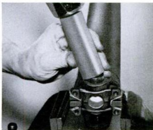
9. DRIVE UNIVERSAL JOINT apart with a short length of pipe. Take it easy with the hammer as otherwise you may damage parts. Note position of rubber bands that hold the bearing cages in place
