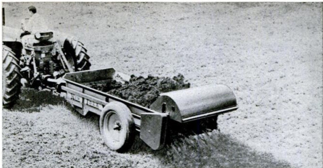
FLAIL-TYPE MANURE SPREADER discharges load low where wind can't carry it. Free-swinging flails mounted on a single rotating shaft shred the manure and spread it in a uniform band 80 to 90 inches wide
