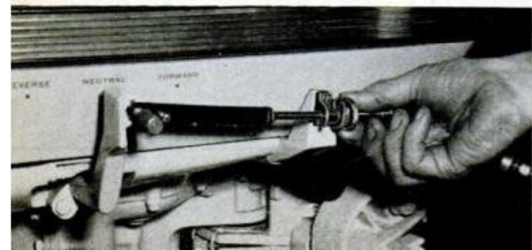
3. KNURLED NUT on shift cable end fitting permits installer to adjust it to exact length required
