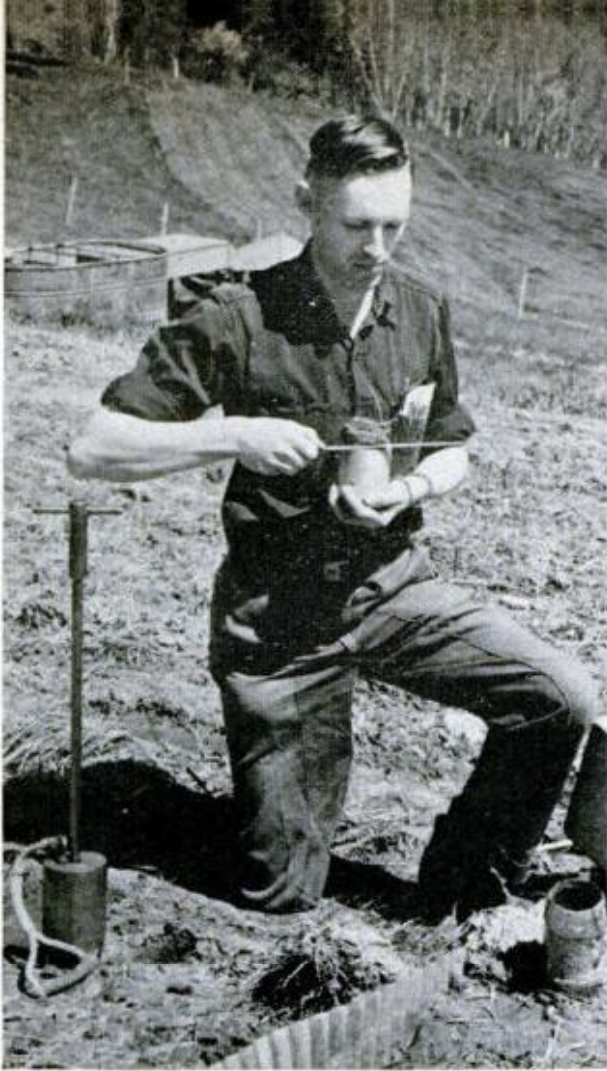
BULK DENSITY samples show the difference in compaction between methods of small-grain seedbed preparation. Below, metal frame is fitted around an exposed soil profile face preparatory to its removal
