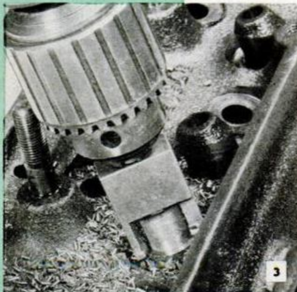
OIL LOSS through valve guides is graphically shown in the diagram above. Note variation in pressures. Below, left, on some cars it is necessary to machine valve guides. Right, installing O-ring on stem
