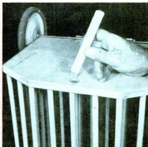
WHEELS, above, are held on axles with washers and cotter pins. Below, short length of dowel provides foot on which cart stands vertically
