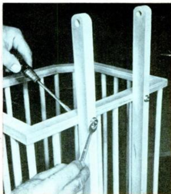
HARDWOOD HANDLE BARS are bolted to top frame but lower ends are held with screws
