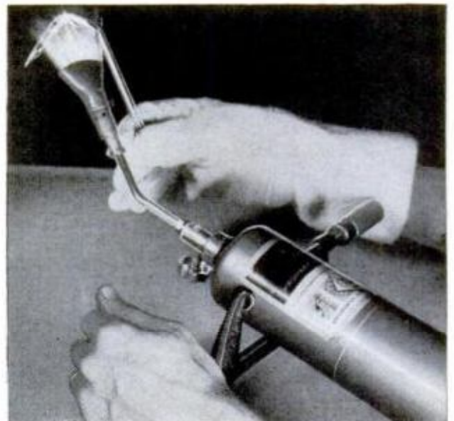
18. LABORATORY GLASS TUBING can be bent into almost any desired shape if you heat it slowly with spreader flame tip. Protect hands! That glass is hot!
