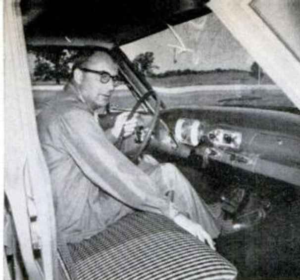
FRONT-MOUNTED engine-transmission requires a moderate tunnel in front compartment, but legroom's good
