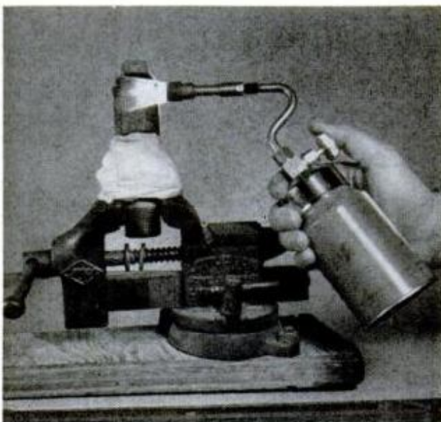
17. REMOVE A STUBBORN pipe fitting by heating with torch, using the flame spreader, Fig. 11. Heat expands fitting to the point where it will let go easily
