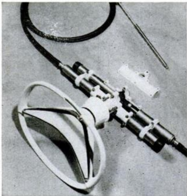
16. SUPER RIDE GUIDE steerer, above, is designed for large motors. Double gear racks actuated by a common pinion, and port and starb'd cables provide easy operating, backlash-free closed-circuit system. Below, neat routing and attachment of remote-control cables to motor make for trouble-free service
