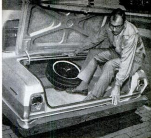
CHEVY II's 13-inch spare sits forward in 13.3-cubic-foot trunk, leaving usable space unobstructed
