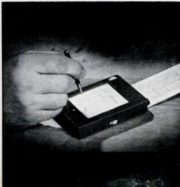
JOTTING NOTES AT NIGHT —when a name or appointment is suddenly remembered—is easily done on an illuminated memo pad. Light glows through translucent plastic under paper. Another light in side of case is flashlight. Bedside Secretary is sold for $4.95 by Hollis Co., Dept. BS-1133 Broadway, New York 10
