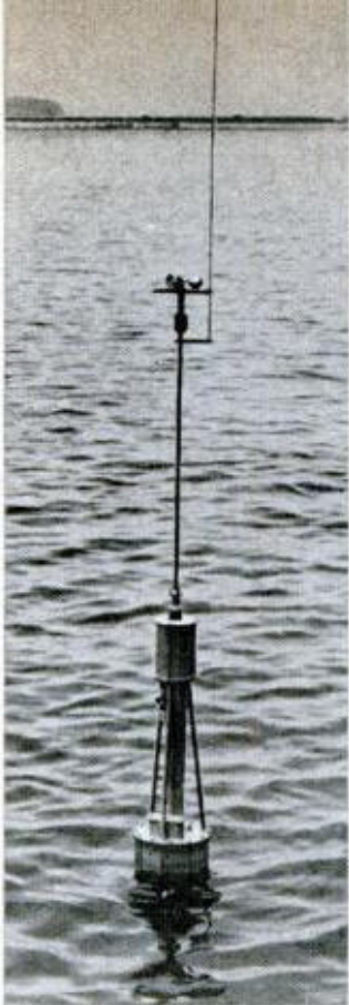
EXPENDABLE , buoy is dropped in path of potential hurricane. Boat sends coded weather report six times daily
