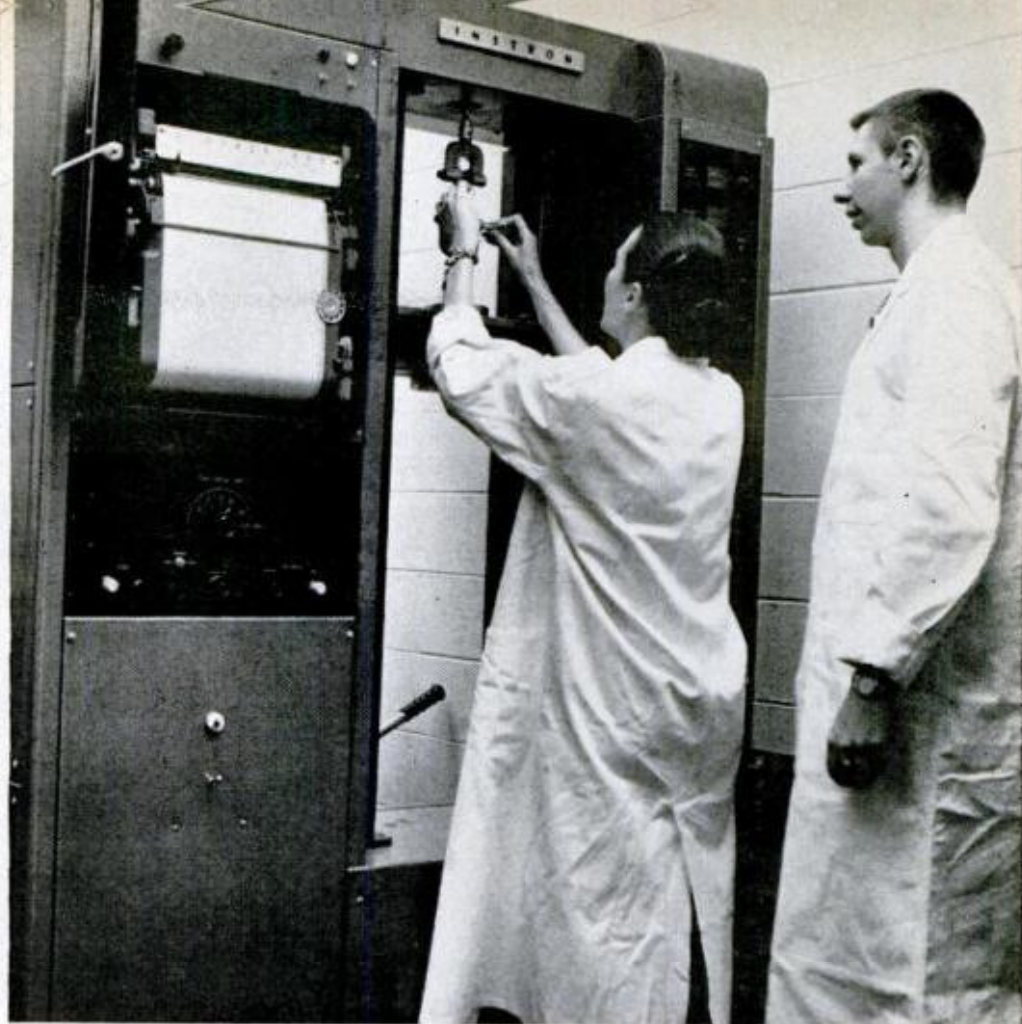
DR. MILLER and an assistant set up for a test of the breaking strength of winding fibers. Test, on the "Instron," will show the relative strength of fibers taken from both old and new baseballs
