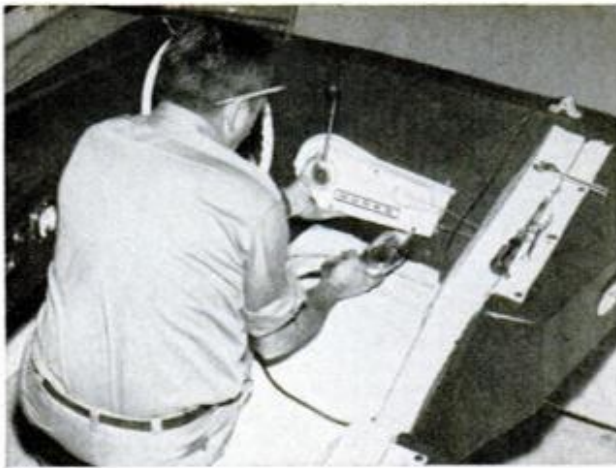
8. THROTTLE-SHIFT unit must be positioned parallel with cables, with adequate clearance for lever
