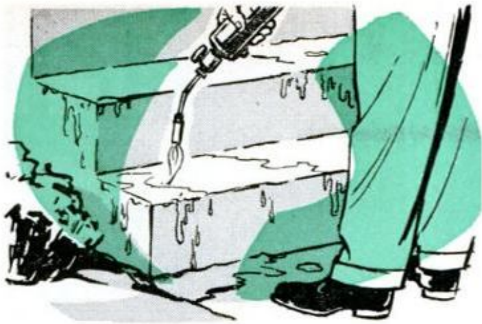
9. THAW dangerous ice patches, above, in seconds. Right, a torch kit made up with igniter, two torch tips and soldering tip is useful in any household
