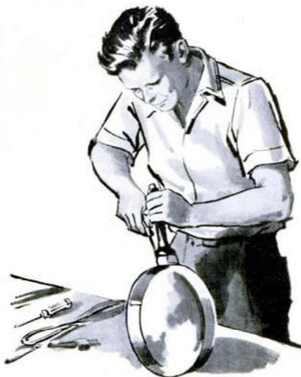
3. YOU'LL NEED a Phillips screwdriver to remove screws in most fry-pan handles. Be especially careful
