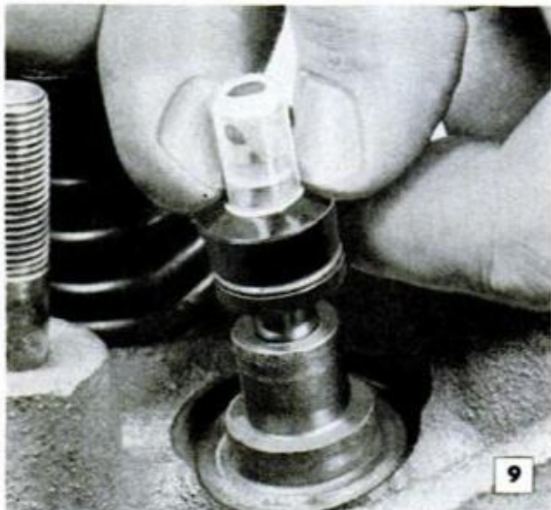
PLASTIC CAP is removed after seal has been pushed down over it and seated. Note retainer on the seal
