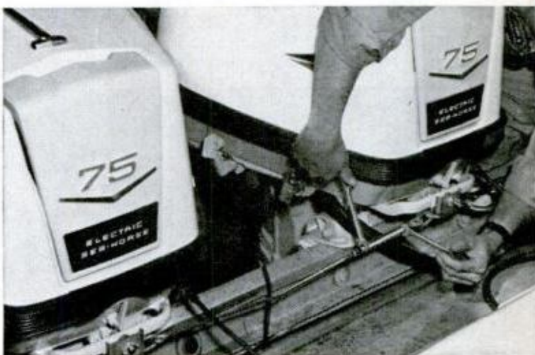
5. TIE BAR linking twins together, is set to toe out motors slightly to minimize torque on steering
