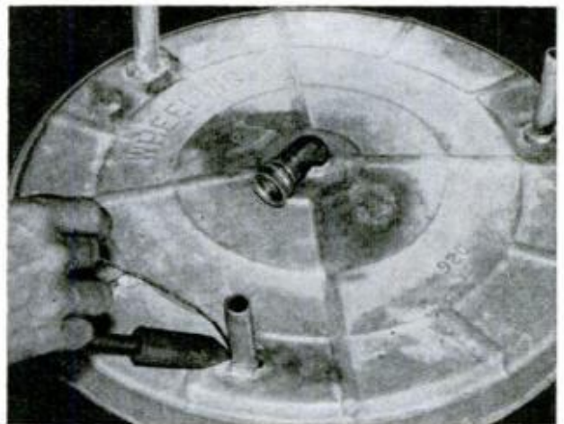
COPPER-TUBE LEGS are soldered to bottom of washer
