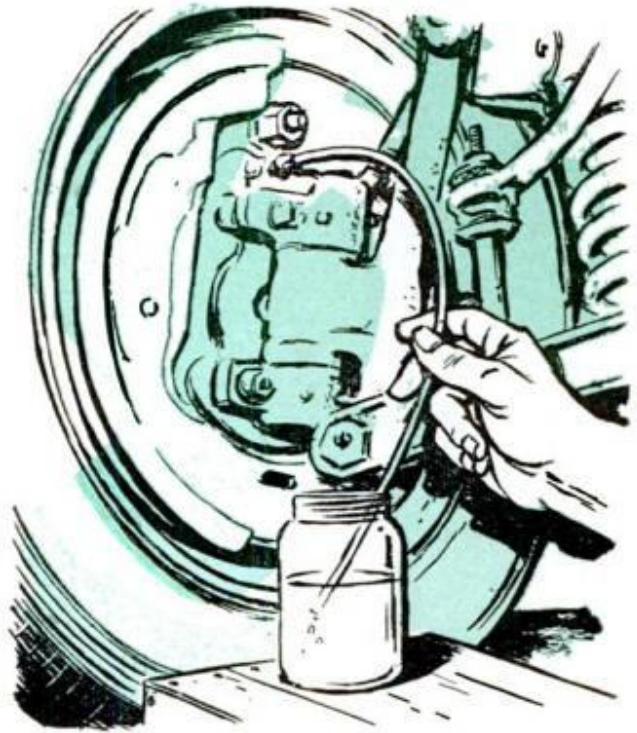
AUTOMATIC REFILLER saves time, eliminates possibility of emptying the master cylinder while bleeding
