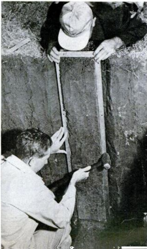
BULK DENSITY samples show the difference in compaction between methods of small-grain seedbed preparation. Below, metal frame is fitted around an exposed soil profile face preparatory to its removal
