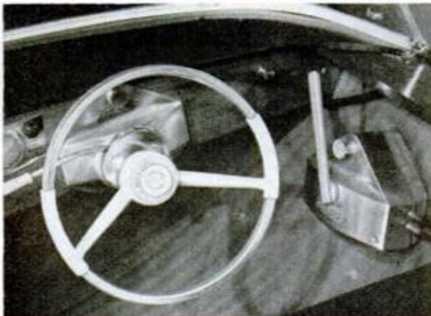
9. MOVING PARTS of husky control unit shown above are made of nylon, which requires no lubrication
