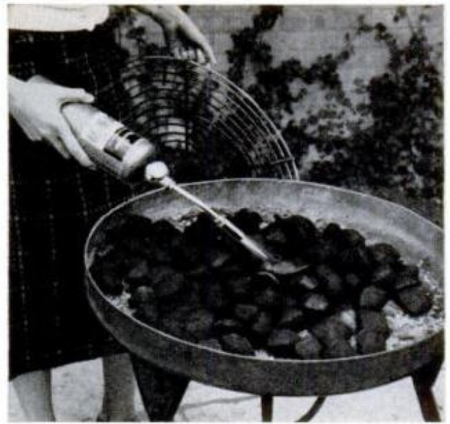
14. IF YOU HAVE trouble lighting charcoal briquettes, try your propane torch. You'll find it the fastest "match" you ever used. No paper or kindling is needed
