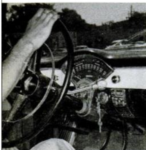
7 VIBRATIONS IN SHIFT LEVER may only mean loose linkage—or transmission's death rattle
