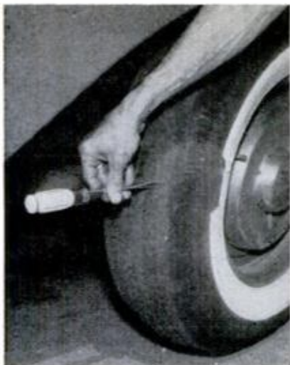
4 SCREWDRIER TEST gives idea of tread depth. Close look may reveal regrooving job
