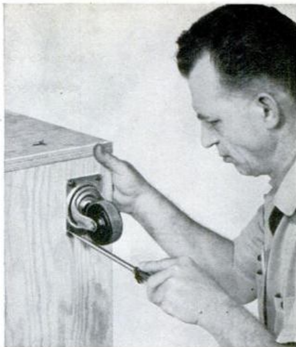
TOOLBOX rolls easily on rubber-tired swiveling casters. Caster plates are attached to bottom with screws
