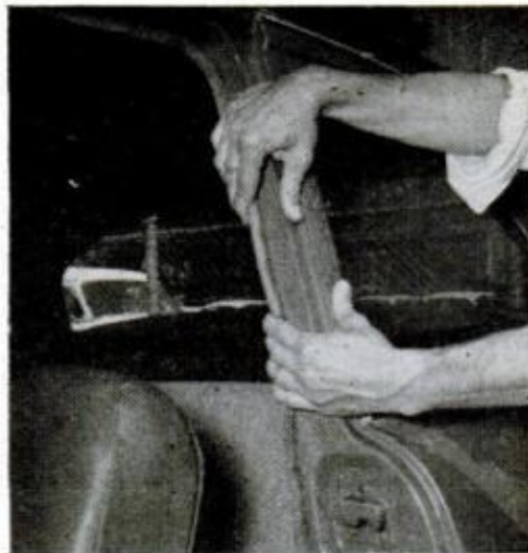
3 REPAINTING BATTERED BODY may leave paint flecks on sills, seats and weather stripping
