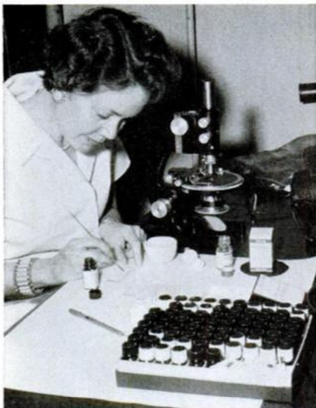
MICROSCOPIC TESTS of drug tablets help identify filler material used to bind actual drug ingredients
