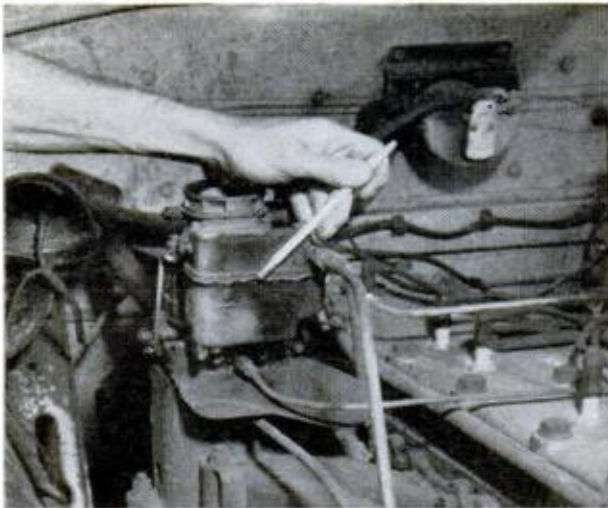
13 LEAKY CARBURETOR GASKETS allow fuel to wash down and leave "varnish" deposits on float bowl—bespeak lack of basic maintenance
