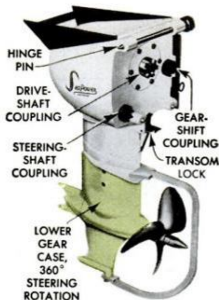
2. SEA POWER drive unit is secured to transom by means of hinge pin and locking lever. Entire lower gear case rotates, permitting 360-deg. steering
