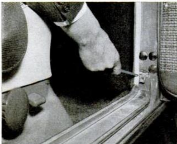
DOOR TRIPS LATCH (when closed) which works through cable to lock front seat-back upright for safety. Handwheel, at left, adjusts seat-back rake
