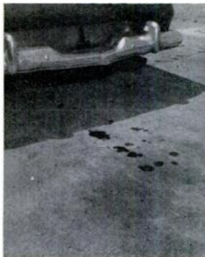
5 TELLTALE OIL DRIP? It may be just a bad pan gasket or a main bearing may be gone
