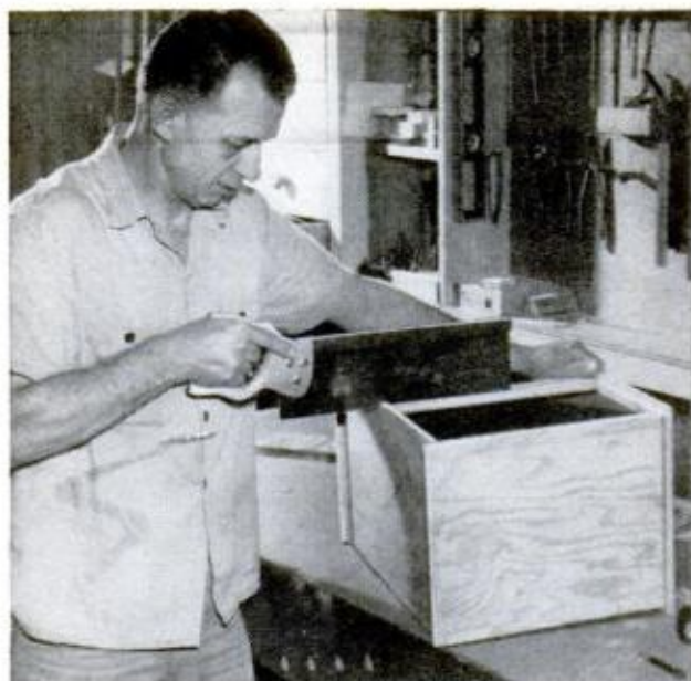
DRAWER BACK is notched to permit grooved slide to engage guide strip. Notch is same size as groove
