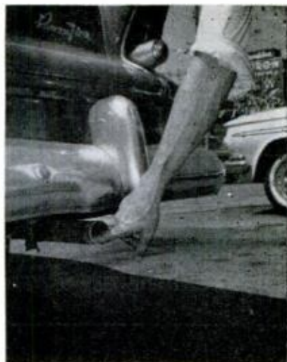
6 WHAT'S UP THE PIPE? If carbon deposits are oily, it may mean engine is an oil pumper
