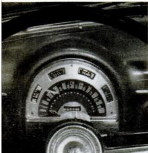
1 OIL PRESSURE DIVES as water temperature hits normal, look for bad oil pump or rings
