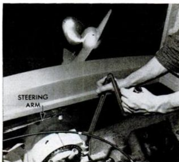
4. DRIVE UNIT of Mercruiser can be hand cranked 180-deg. into raised position for easy prop changing. OMC (Outboard Marine Corp.) unit may be tilted up like outboard, except that it is power operated
