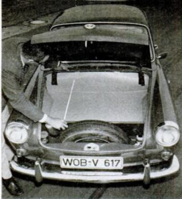
FRONT TRUNK of VW 1500 measures 27 inches long by 41 inches wide at the rear, is 11 inches deep at rear. Cowl air intake can be seen at upper edge of trunk
