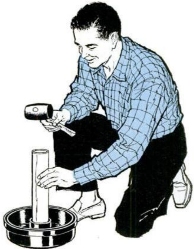
4. MAILING TUBE makes a good driver for removing and replacing oil seals in brake drums. Tap lightly
