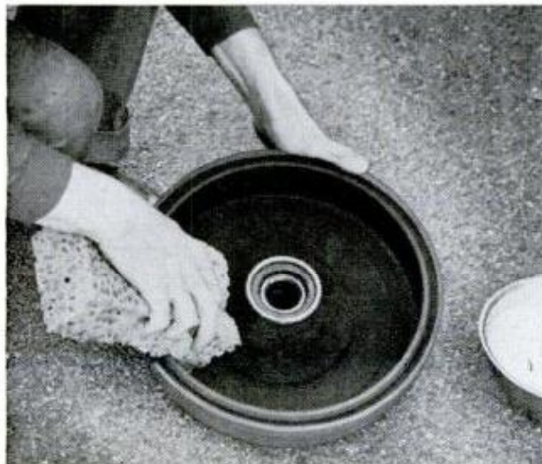
5. CLEAN BRAKE DRUM with detergent and hot water or with a solvent. Make sure it is thoroughly cleaned
