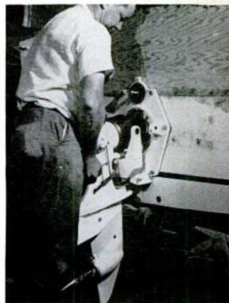
9. BELL HOUSING , left, is bolted to inside of transom, after which engine is lowered into cockpit and bolted to bell housing, center. Right, drive unit is fitted to shaft and locked in place with pins, completing installation except for connecting remote controls, fuel lines, electrical and cooling systems
