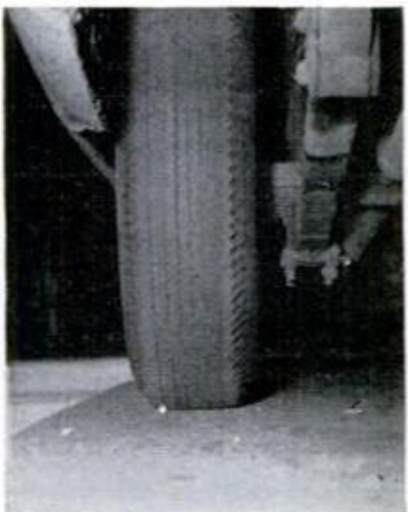
10 WHEELS OUT OF BALANCE or out of line show up in uneven tread wear, bald spots
