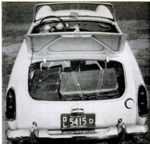
LUGGAGE COMPARTMENT has 11½ cubic feet, is moderately capacious by two-seater sports car standards
