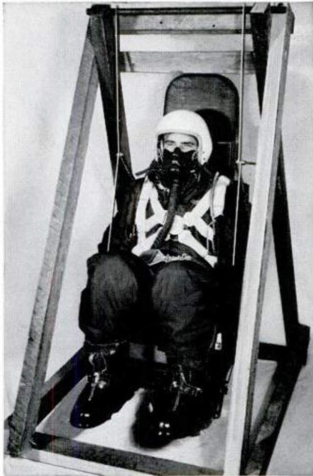
SWING CHAIR works just like baby's, but is used to determine the exact center of gravity of the body
