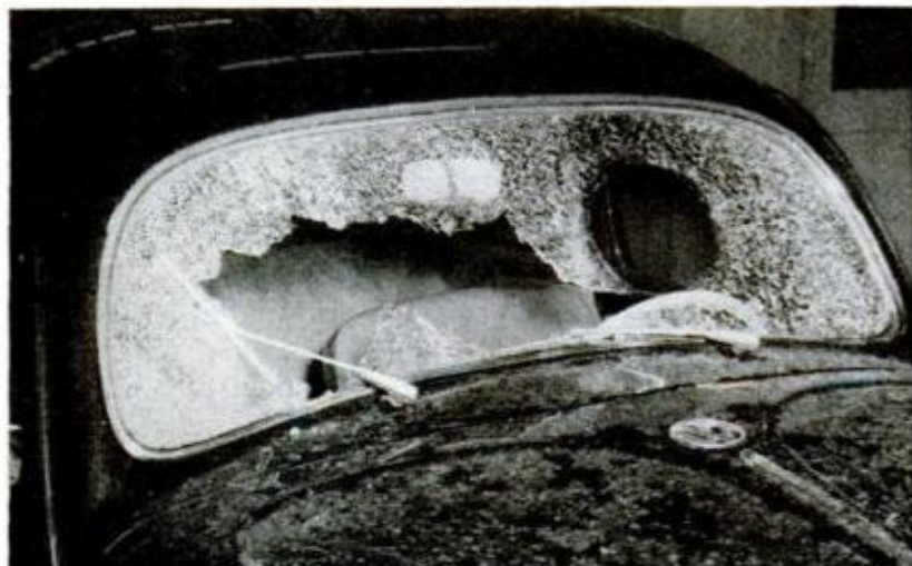
SHATTERED tempered windshield (left). Glass from circular area was found to be not tempered. Cars sold in U.S. have laminated windshields. At right, note fragments of shattered tempered glass on seat
