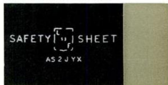
1957 Plymouth sidelight was laminated but not windshield optical quality, so label (below) is AS-2
