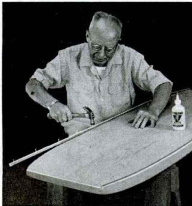
GLUE AND NAIL matching wood strips along top edges
