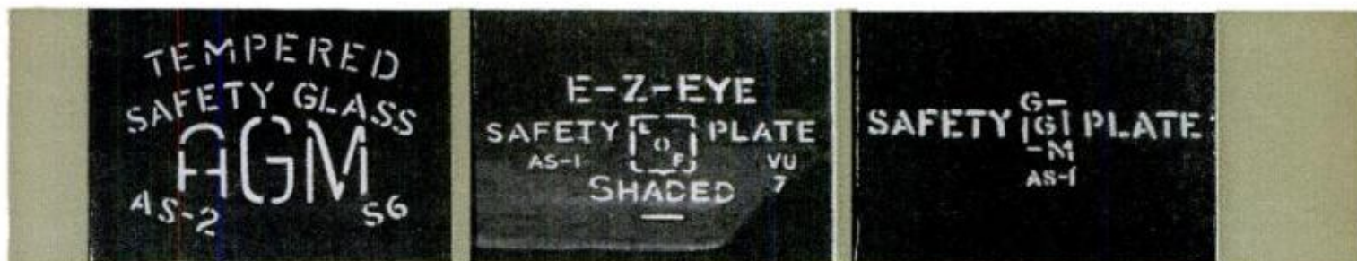
WINDOW from new Rambler (left) is frankly labeled tempered. Center and right, AS-1 laminated windshield and laminated replacement sidelight both have passed optical distortion and laminated glass impact tests
