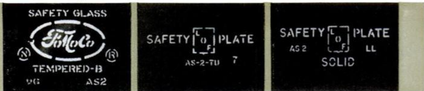
PHOTOS of labels from 1961 Comet tempered vent pane, and 1961 Pontiac laminated vent and tempered window. AS-2 means either tempered glass, or laminated which doesn't have to pass windshield optical tests
