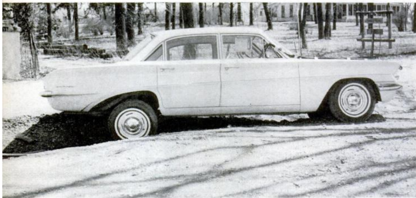
F-85 STRADDLES A 15-INCH-DEEP DITCH without a belly scrape, despite its low clearance and 13-inch wheels
