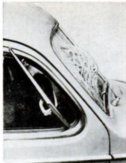
LAMINATED glass backers say it is easier to break and remove it with your hands (left) if you should be trapped inside by an accident. Right, laminated glass may provide more cushioning when impacted by head
