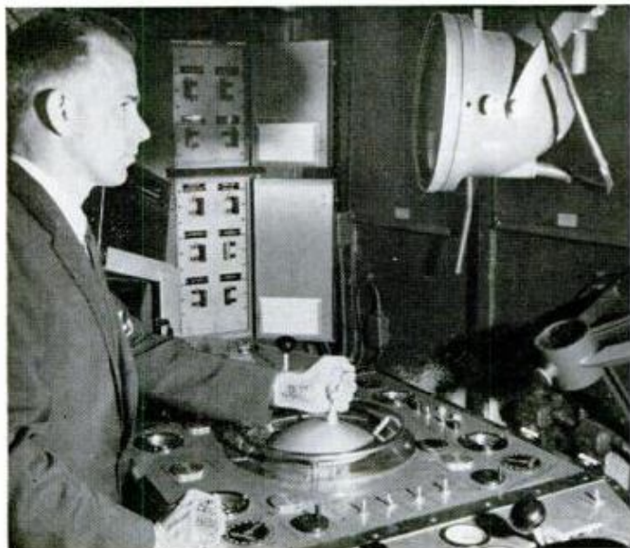
OPERATOR holds ship over hole by positioning four outboard motors with this stick in the wheelhouse
