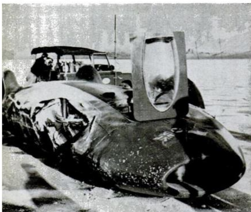
CAMPBELL'S BLUEBIRD , most promising of recent cars to try for record at Bonneville, lies bent and torn after 350-m.p.h. skipping slide along Salt Flats. More than 70 companies invested $4,500,000 in it, and supplied 20 support vehicles
