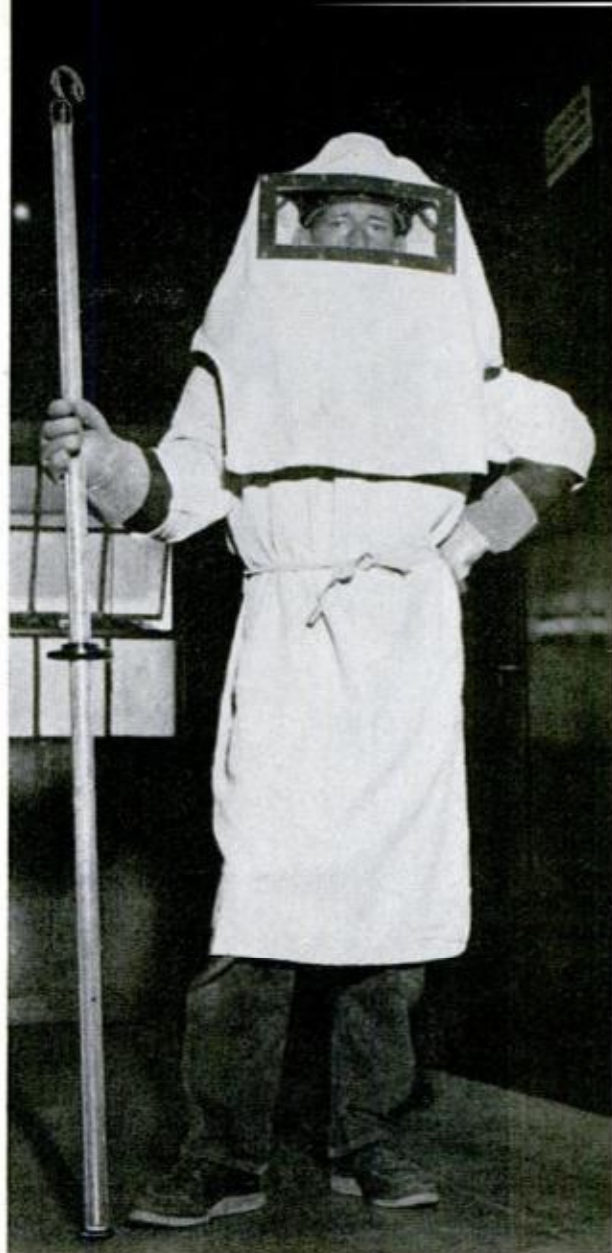
SAFETY SMOCK of asbestos includes rubber gloves and plexiglass window. They are used in manholes
