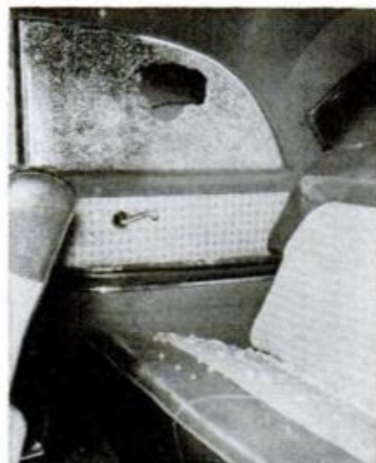
SHATTERED tempered windshield (left). Glass from circular area was found to be not tempered. Cars sold in U.S. have laminated windshields. At right, note fragments of shattered tempered glass on seat
