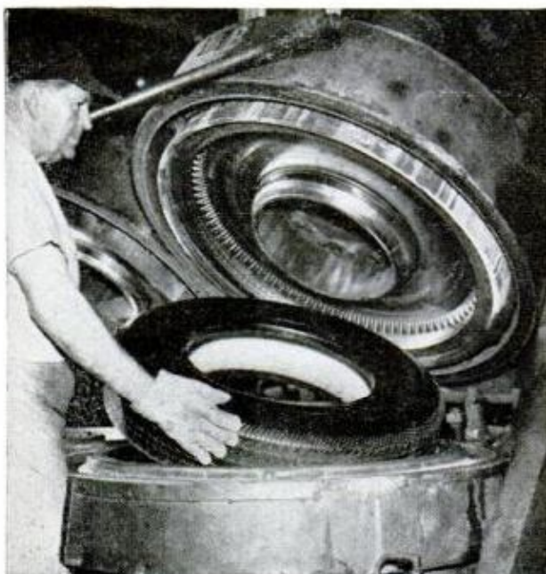
5. FINISHED TIRE comes out of curing machine after baking for 1 hour and 20 minutes at 350 degrees F.
