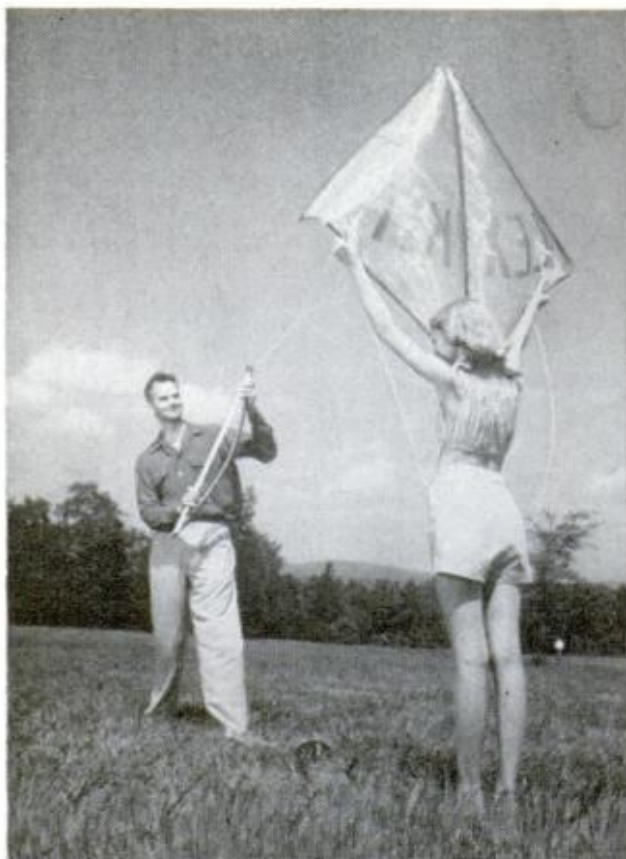
NEWEST KITE is nonrigid Flexkite, made of flexible plastic. Its inventor, Dr. Francis Rogallo, is at left
