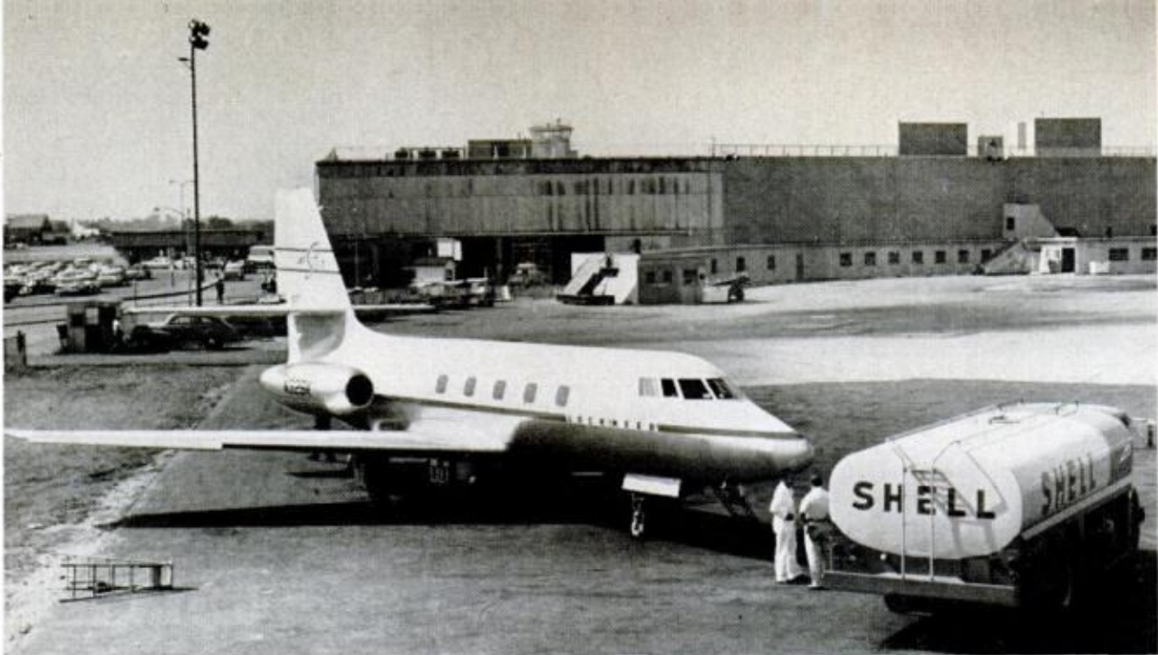
LOCKHEED JETSTAR , another recent jet addition to business fleet, is in 600-m.p.h. class. It can fly 1700 miles nonstop or, with additional wing tanks, more than 3000 miles. There is also a four-engine model
