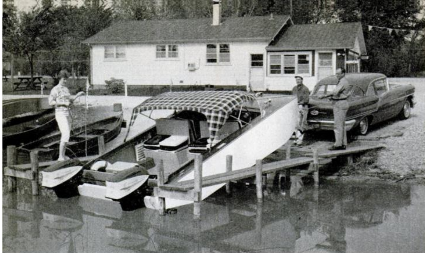
TILT-BED catamaran trailer permits easy one-man launching and retrieving of Pop-Cat without wetting feet
