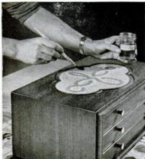
5. SILICONE SEALER brushed on tile and grout after latter is dry, below left, keeps tile bright looking longer. Right, photo shows how some of the tile must be shaped in order to work out particular mosaic design
