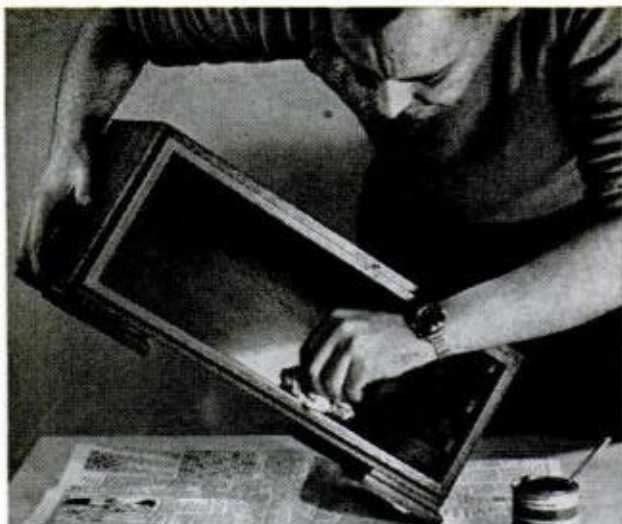
3. RED STAIN is rubbed well into mahogany grain prior to giving case three coats of spar varnish
