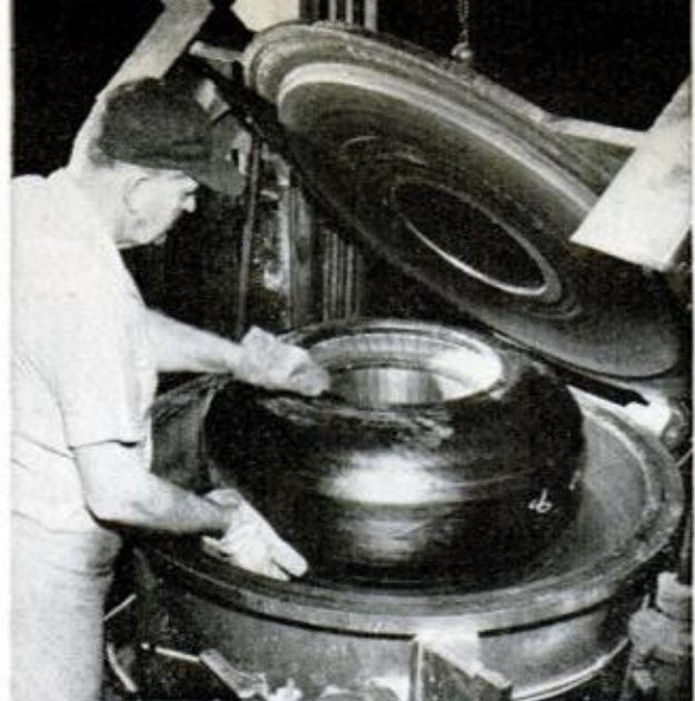
4. AFTER FORMING MACHINE has pressed the soft "green" tire around the doughnut, it is ready for curing
