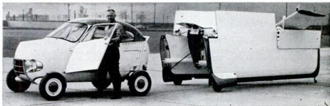
AUTO-AIRPLANE has detachable wings and tail assembly. On the road, these can be hauled behind the cab, or left behind and the cab used as a two-seat compact car. The car can do 60 miles an hour and the plane 100
