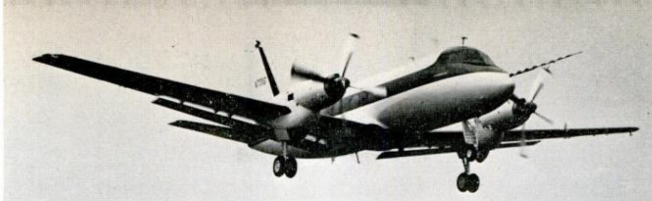
NEW TURBOPROP , Grumman Gulfstream, was first propjet designed specifically for business-flying market. It can carry up to 19 passengers at a cruising speed of 370 m.p.h. and a maximum altitude of 36,000 feet
