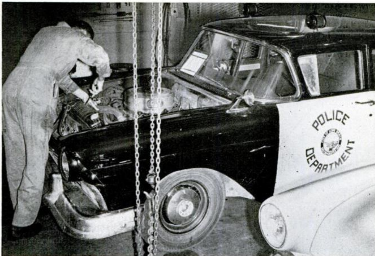
MECHANIC BEGINS ENGINE REMOVAL on Long Beach, Calif., police car. A uniform oil-change program more than doubled the mileage interval between major engine overhauls on the entire fleet of city-owned cars
