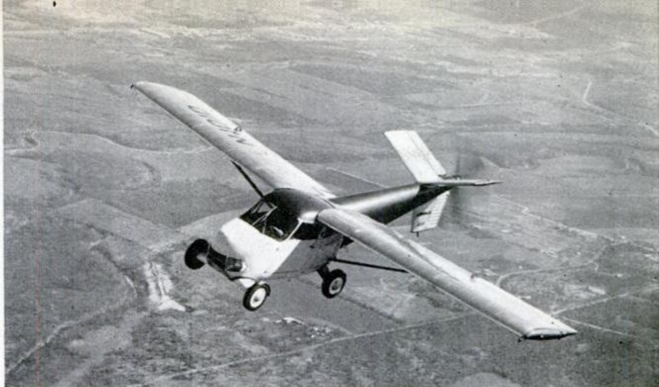
AUTO-AIRPLANE has detachable wings and tail assembly. On the road, these can be hauled behind the cab, or left behind and the cab used as a two-seat compact car. The car can do 60 miles an hour and the plane 100
