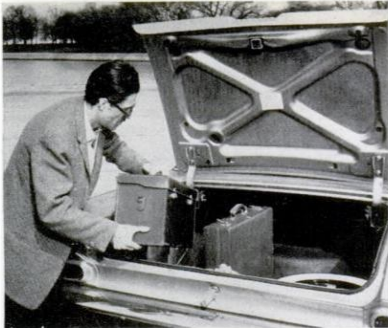
TEMPEST'S LUGGAGE COMPARTMENT is fairly roomy and wide but the spare tire placed flat on the floor usurps valuable space
