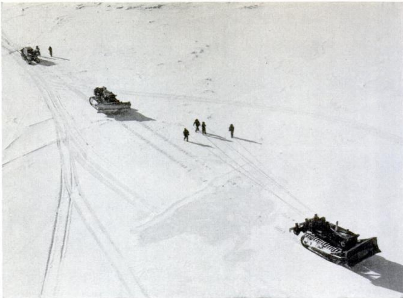
THIN ICE! Drivers guide 35-ton tractors across thin sea ice with reins—just in case one falls through
