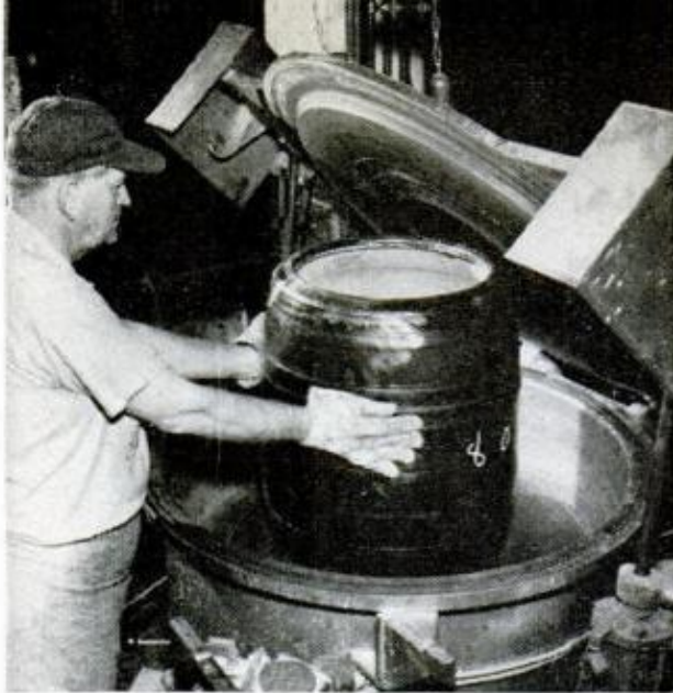
3. "GREEN" TIRE just off building drum goes into forming machine, with rubber doughnut tube inside
