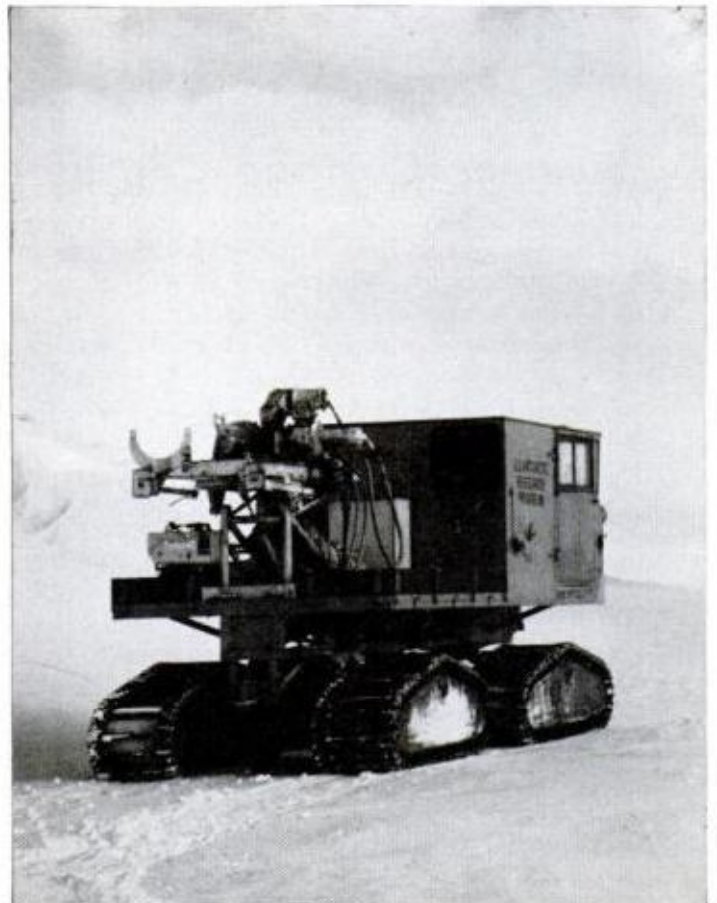
CORING CAT is newest snow vehicle for glaciologists. It is equipped to drill into ice and take samples
