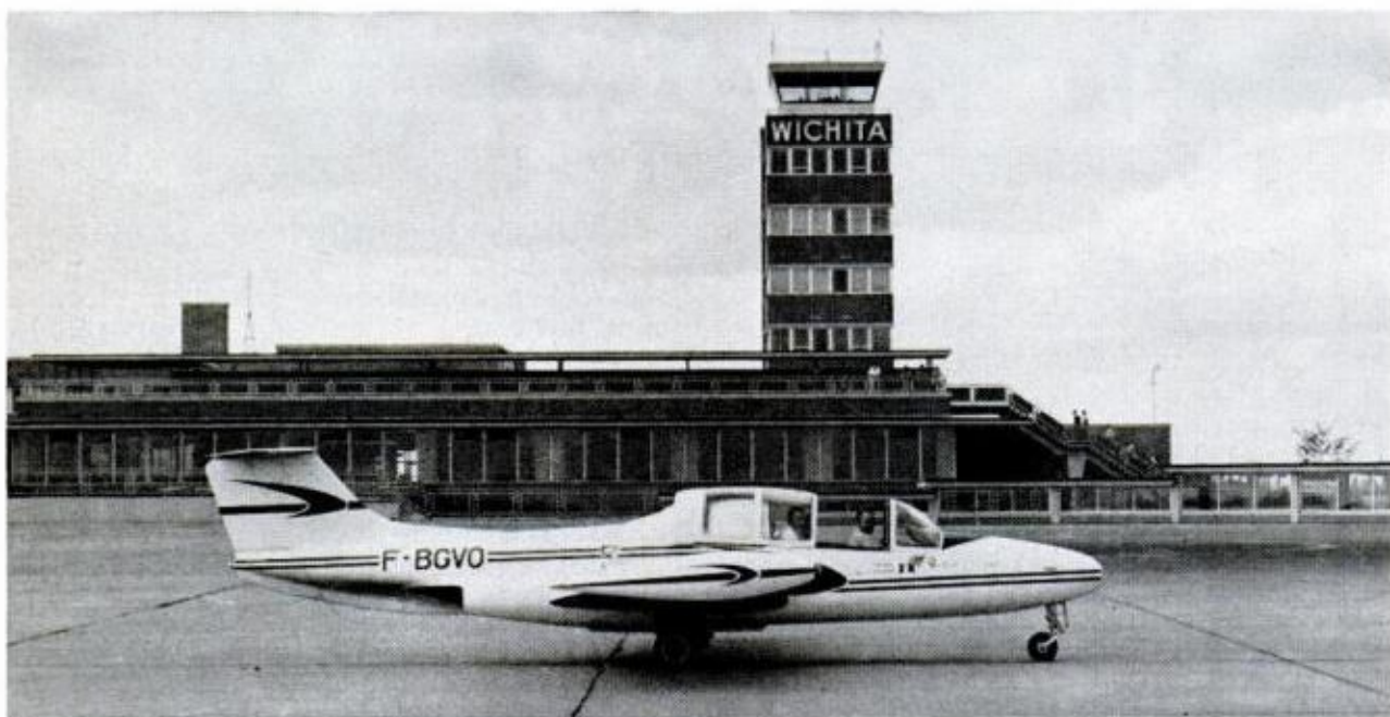
FRENCH JET , Morane-Saulnier 760, became first turbojet to join U.S. business fleet when it was imported by Beech Aircraft Corp. M-S 760, a four-place pressurized aircraft, is capable of speeds above 400 miles an hour
