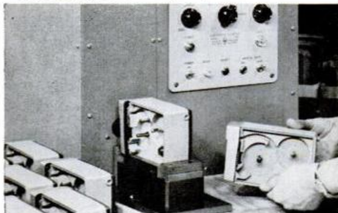
ELECTRONIC FRAME-COUNTER checks film travel—assures movies that move at correct speed.
