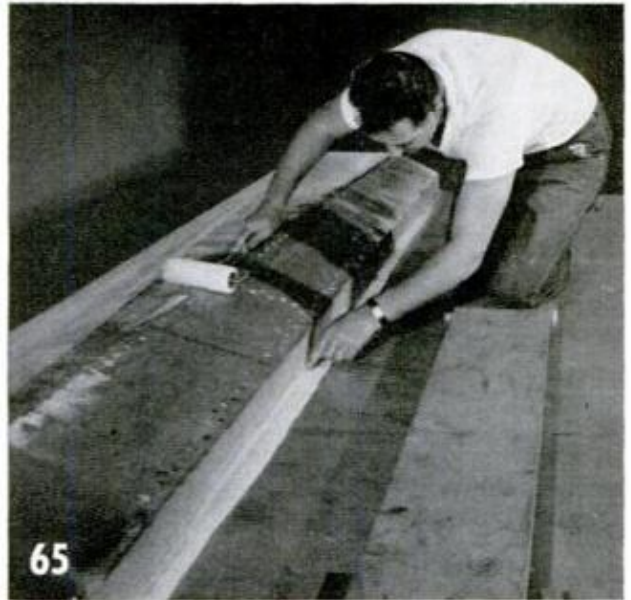
PLANK PLACED ON glassed wing deck prevents grit from being worked into it while working on chines
