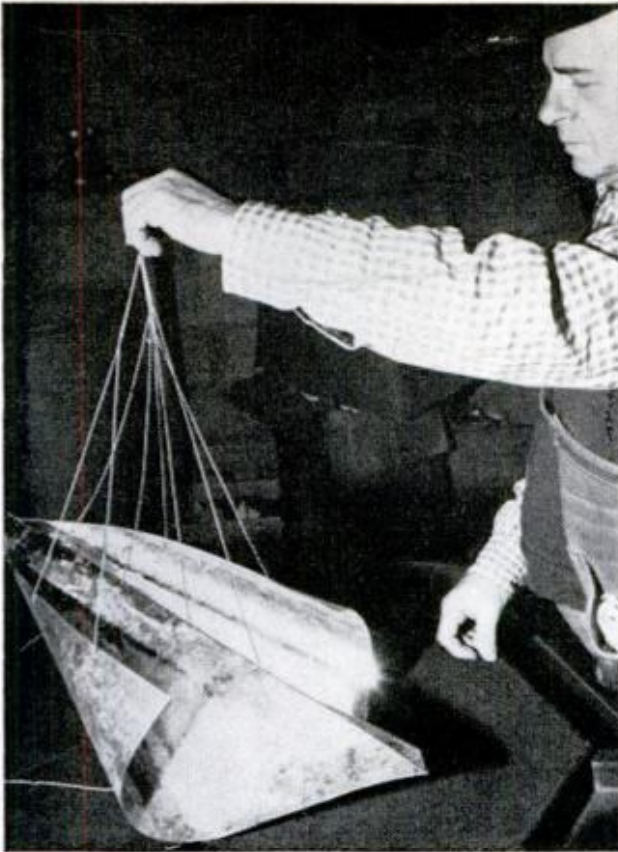
FLYING SHAPE of Flexkite is demonstrated by Yolen. As shroud lines gather, kite assumes proper angle
