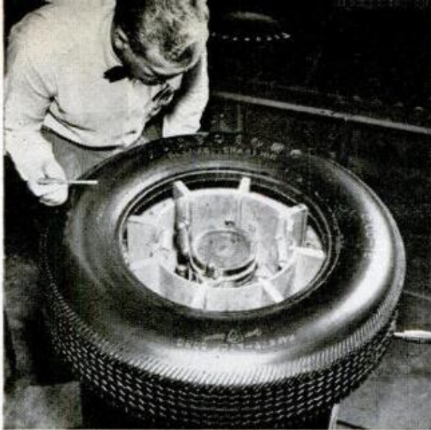
7. STATIC BALANCING of the finished tire with special spirit level checks possibility of heavy spots
