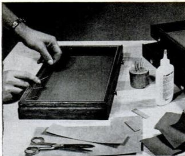
4. FELT LINING glued on inside surfaces of drawer, is held in place with straight pins until glue sets
