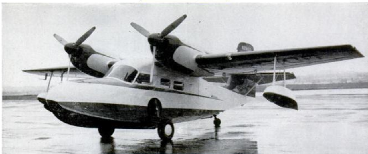
SUPER WIDGEON is direct ancestor of four-engine Golden Goose. It is powered by twin 260-horsepower engines
