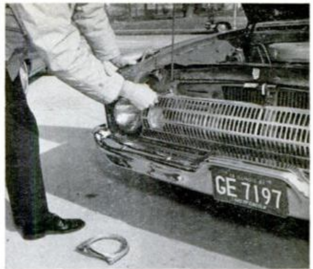
SIMPLICITY SAVES money on replacement parts, labor in cases like Falcon's one-piece grille, single lamp
