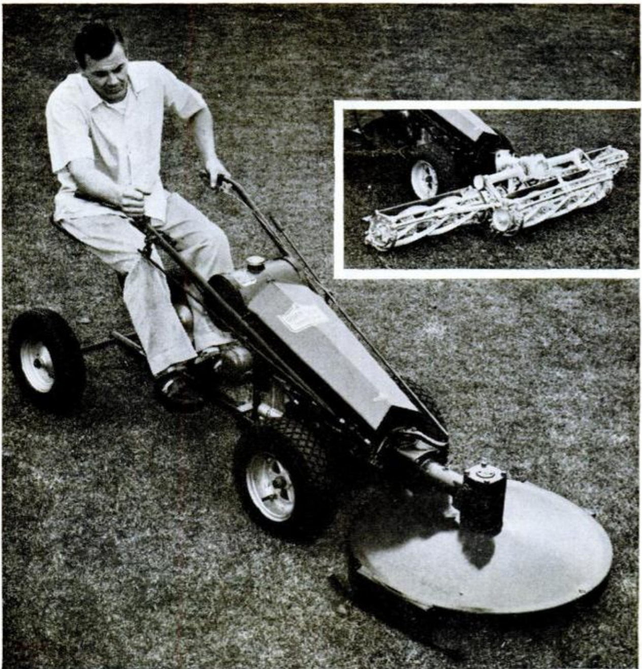
CONVERTIBLE POWER UNIT makes a real workhorse for the enthusiastic gardener. The unit can be used either as a walking or riding mower. Besides using reel or rotary mowing units, suitable attachments can be added to do such jobs as cultivating the garden, grading a new lawn or clearing away the snow in the winter
