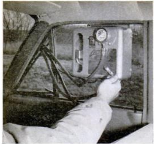
FUEL FLOWS by gravity from 1/10-gallon burette to electric pump, then to carburetor
