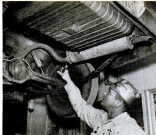
COST OF LABOR on muffler replacement is about equal between big six and compact, but compact part is less
