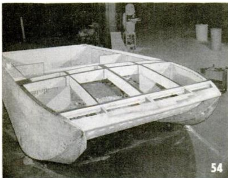
DECK FRAMING and subdecks, above, have been faired and are ready for planking. Below, foredeck panel is nailed from center outward
