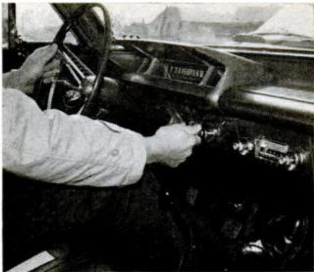
MANUAL CHOKES on Pontiac Tempest, Corvair, Falcon enable skillful operators to save on fuel, repairs
