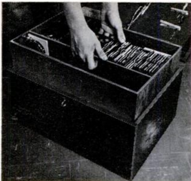
INNER CASE lifts out of combination box and leaves a light-tight unit for loading and changing films
